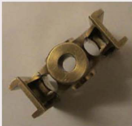
Mike's brass pattern for the lost wax stainless steel early type GWR crosshead castings.
