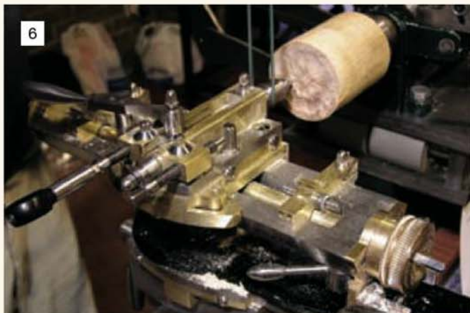
6 The demonstration of rose engine turning by Michael Bain of the Society of Ornamental Turners was fascinating to watch.
