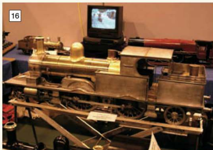
Seen on the Stoford Miniature Locomotive Society stand was this 7 1/4 in. gauge 4-4-2 Adams radial tank engine by member Dave Cox.
