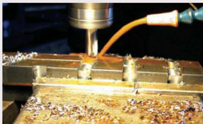
Initial stages in machining a batch of five lamp bodies.
