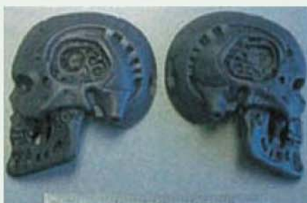
Solid model of a patient's skull obtained using the output from body scanning equipment.
