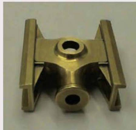
Mike's brass pattern for the lost wax stainless steel early type GWR crosshead castings.
