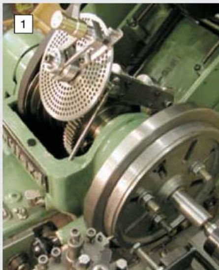
The attachment in use to cut the degree divisions on a Universal Pillar Tool table.
