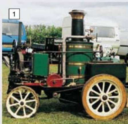
Eddie Lancaster's fine 6in. scale 'special light traction engine' complete with wood block back wheels.
