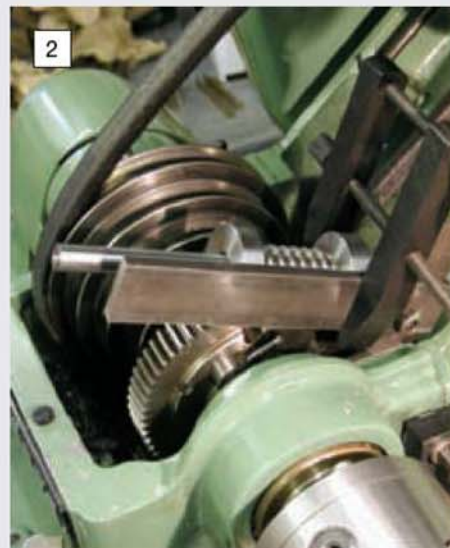
Setting the best angle for the attachment to engage the bull gear.
