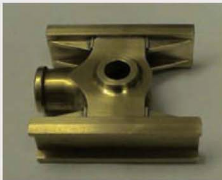
Mike's brass pattern for the lost wax stainless steel early type GWR crosshead castings.
