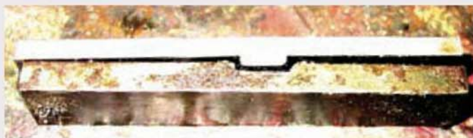
Side mounting brackets are best formed up using a simple bending fixture.
