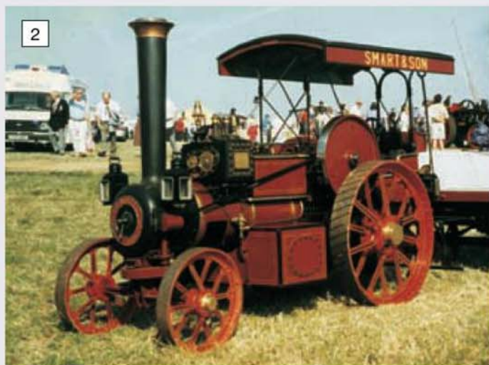
A 4in. model Burrell Gold Medal tractor with direct gear drive steerage. This fine model is the work of John Anyon. Note the pair of 'Meteor' road locomotive headlamps fitted as per the works photograph of the prototype.
