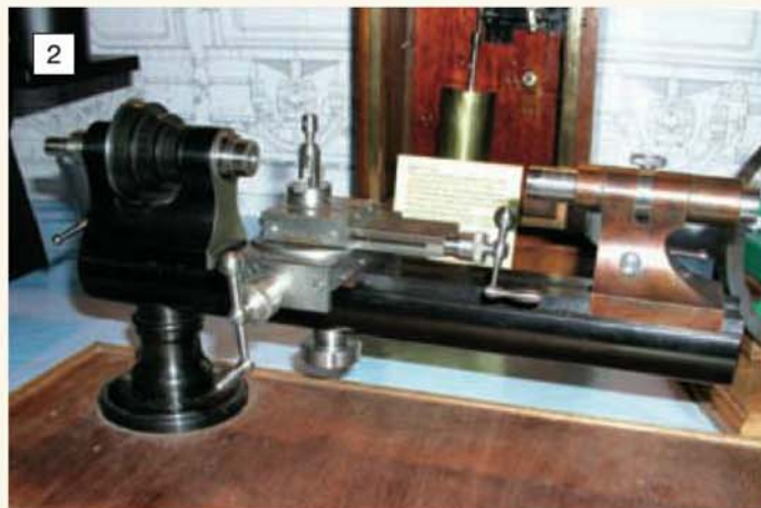
A freelance horological lathe constructed by Howard Harvey of Newport Model Engineering Society.
