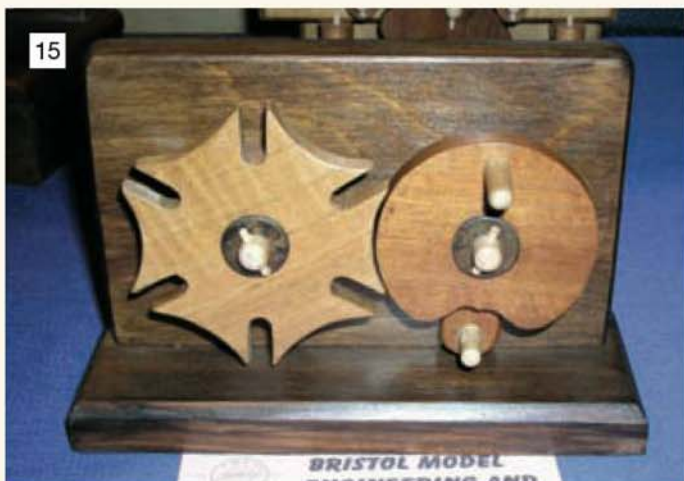
This wooden representation of the Geneva index mechanism was part of an extensive collection of such devices by Edward Addis.
