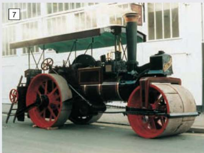
One of the last rollers to be built by Burrells. She is Works No. 4061 and was completed in Jan 1927, only three more rollers were to be made: Nos. 4062, 4067 and 4069, all of 4nhp 8 ton specification.
