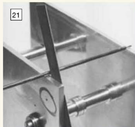
The position of the second pivot is marked using a screw head slotting file.
