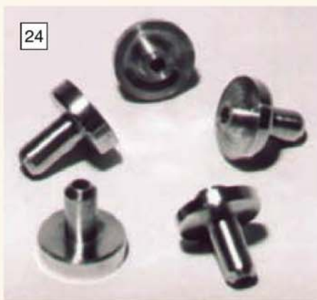
A group of collets; note the undercut face to ensure the wheels seat truly in position.
