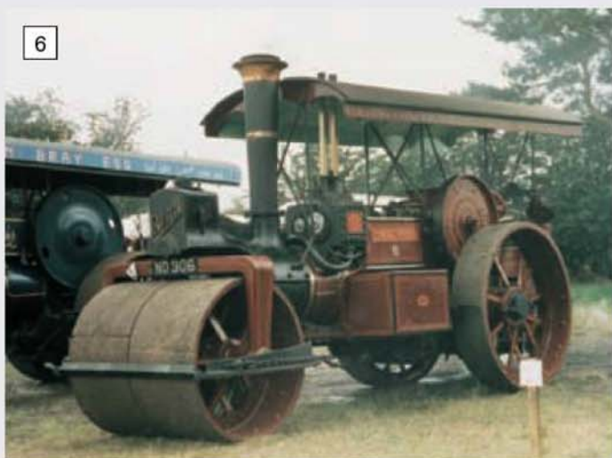
Works No. 3622 was completed in October 1914 and was built as a Gold Medal tractor, being subsequently converted by Burrells to a roller. While 203 tractors were manufactured only 22 rollers were ever made.
