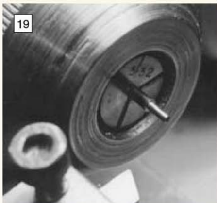
To ensure concentricity, the arbor pivots must be turned using a collet or 4-jaw chuck.
