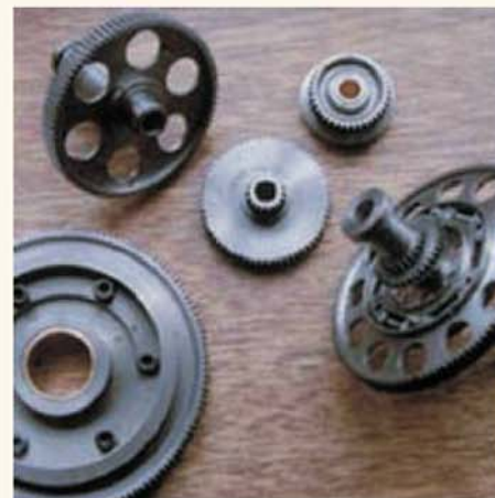
The timing and supercharger gears. The teeth on the large bevel had not been cut at the time of the photograph.
