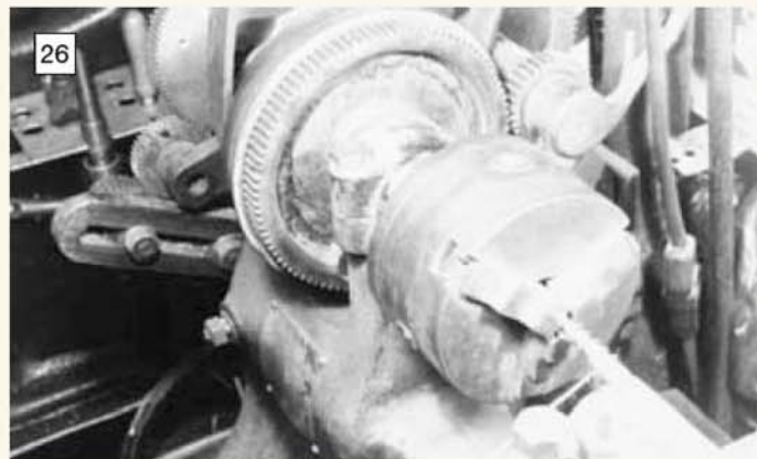
26 Winding a worm helix on a mandrel mounted in the lathe chuck. The lathe is set up for screw cutting and provided the correct lead.
