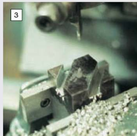
Gashing the dovetails in the steel block using a parting-off tool borrowed from the lathe.
