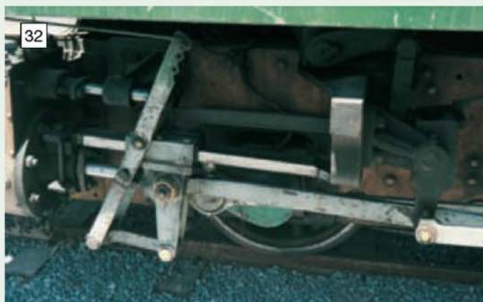
2ft. gauge locomotive Sandy is fitted with Walschaerts valve gear.
