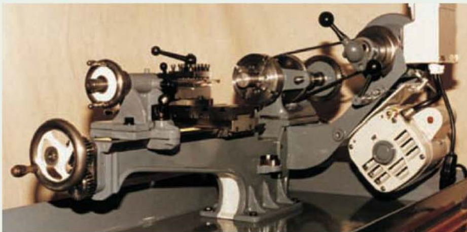
A view from the rear of the Drummond lathe showing the new countershaft bracket assembly, the Hoover motor and the electrical switch gear. This photograph also shows how the drive belt straddles the back gear shaft. Care was taken with the design to ensure it did not foul the shaft on any speed.
