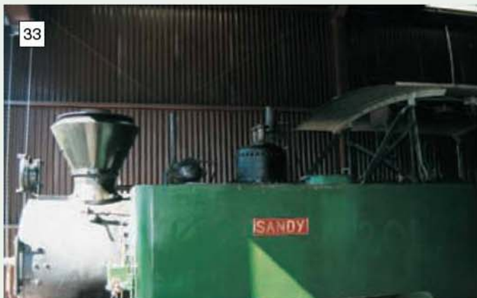
Sandy's superstructure includes a dominant spark arrester chimney!
