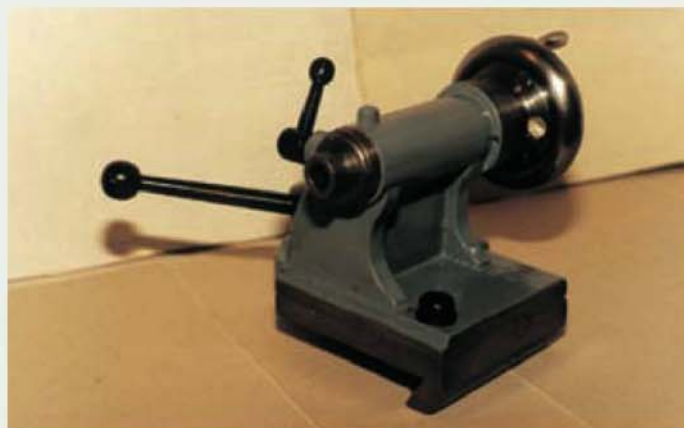
The Drummond tailstock is located on the same bed surfaces as the lathe saddle - a factor which may help even out wear.
