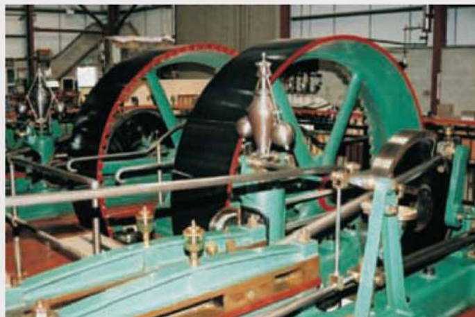
This mirror pair of single cylinder engines with Meyer valve gear was built in 1884 for the Wilderspool Brewery by Thornewill & Warham of Burton on Trent.
