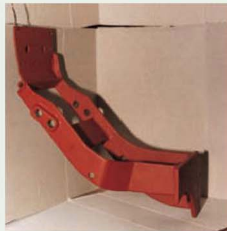
The countershaft bracket after fabrication, cleaning up and painting in primer.
