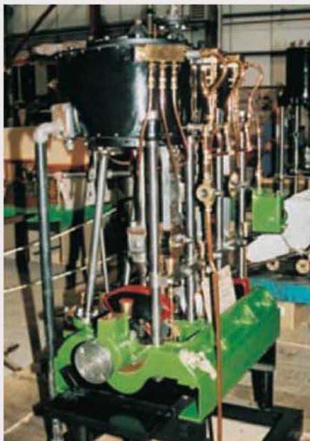
This inverted vertical triple expansion engine with Hackworth valve gear was built in 1927 by Sissons & Co. for a Thames passenger boat.
