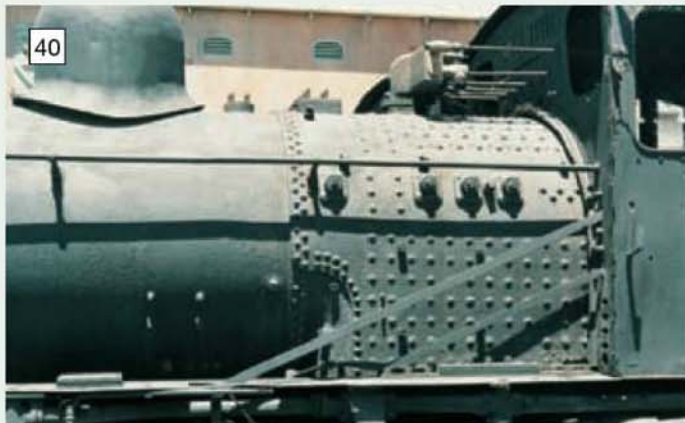
Missing cleading reveals part of the boiler construction at the firebox end.
