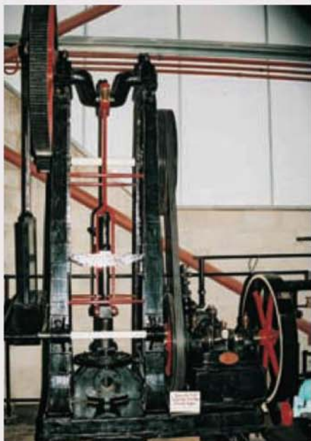
This pump by John Thorn of Patricroft from Tong Dyeworks is powered by a horizontal engine by Robey and Co.
