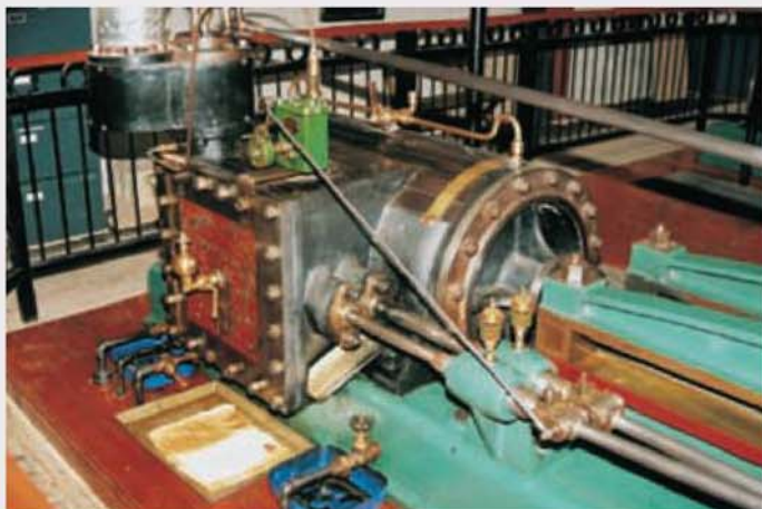
This mirror pair of single cylinder engines with Meyer valve gear was built in 1884 for the Wilderspool Brewery by Thornewill & Warham of Burton on Trent.
