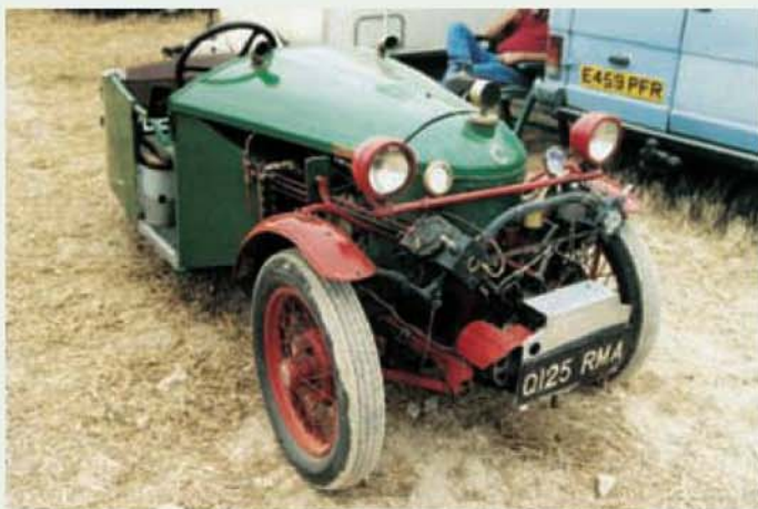
The CEK three wheel steam car Kiswasti built by Mr. Cholton. Incredibly, construction was started in 1947 and it's still unfinished!
