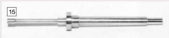
Great wheel arbor with machining completed.
