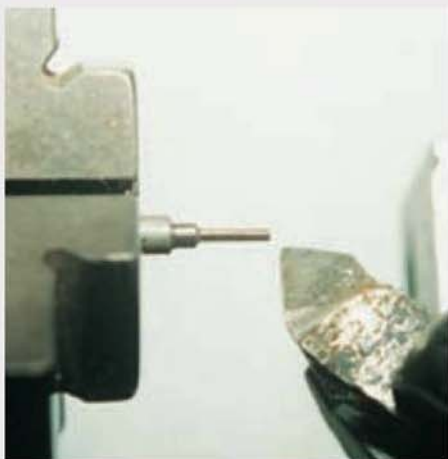
The 0.039in. diameter governor link pivot pins were turned from \frac{1}{8} in. dia. mild steel.
