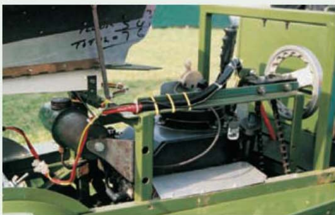
The Diamond T engine compartment with Briggs and Stratton engine.
