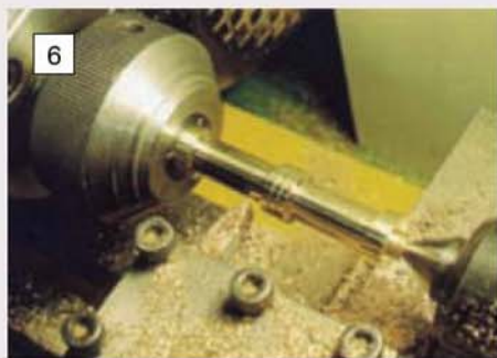
Left: machining the waisted sections of the plate pillars with a round nose brass turning tool.
