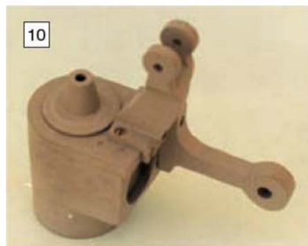
Trial assembly of power cylinder, displacer rod guide, beam bracket and flywheel bracket.
