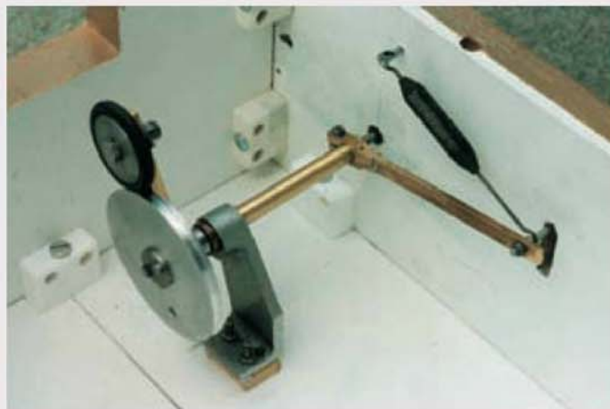
The manual drive mechanism housed in the base. The spring loaded lever brings the tyred wheel into contact with the flywheel.
