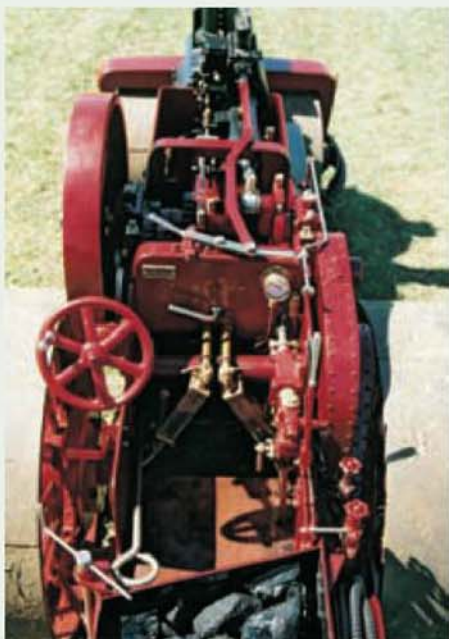
A driver's eye view on the 4in. Garrett Roller seen at the Rushden Rally; note the twin water gauges and the hornplate mounted feed pump on the right-hand side.
