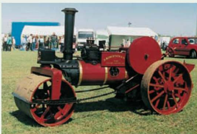
The front fork and swan neck of Dave Robertson's beautifully turned out 4in. Garrett roller were both fabricated.
