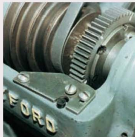
The method used to index the mitre gears while being cut in the lathe.
