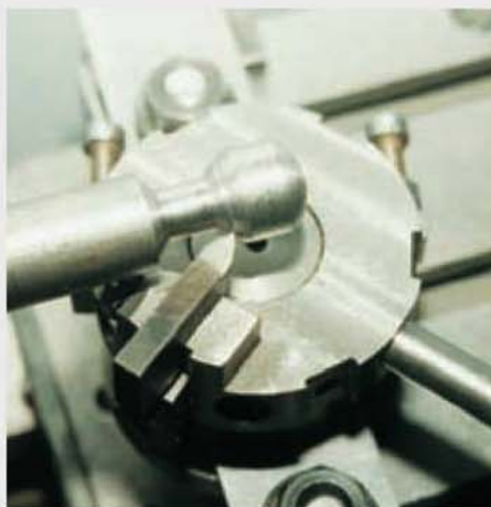
The ball turning device used to turn the governor weights; note the safety advice in the text.
