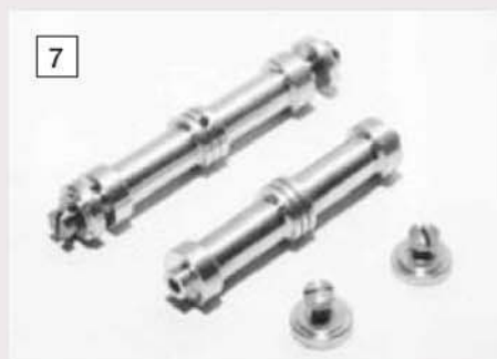
Right: a pair of finished plate pillar sets with screws and washers.
