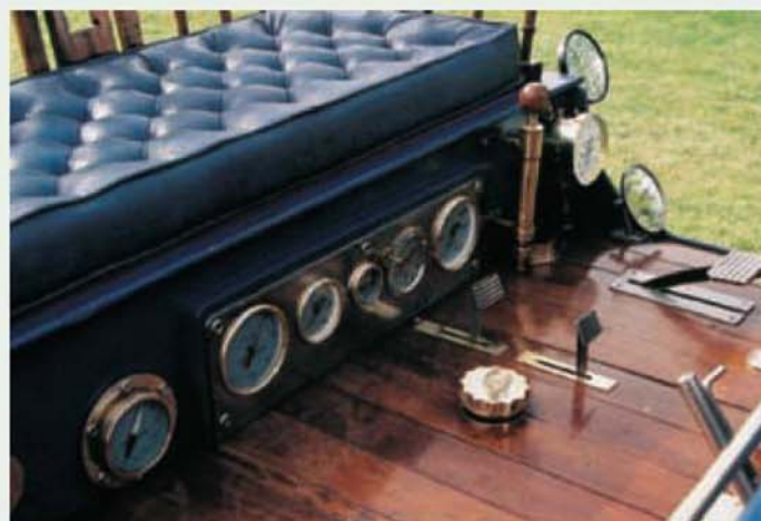
The controls of Ray's steam car. It has tiller steering.
