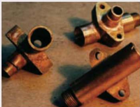
Water valve body (several).
