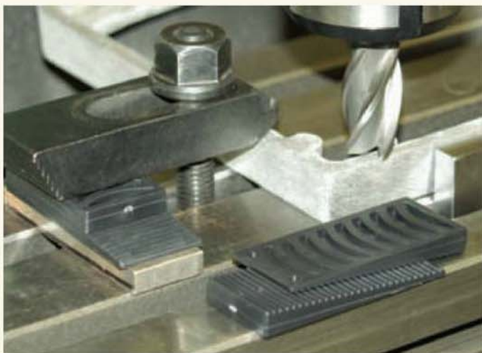
The stepped hard plastic packing blocks to which Mr. D. Dew refers are inexpensive and available in the UK from DIY stores.
