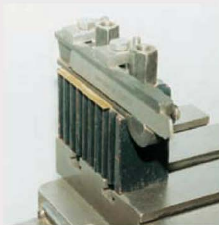
This useful, improvised rear tool post was made from a cylinder offcut.
