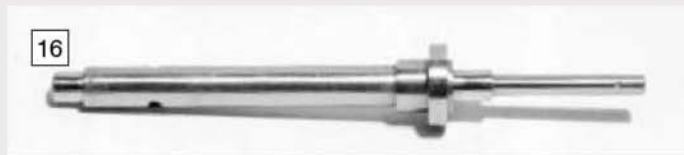
Great wheel arbor cross drilled and brought to length.
