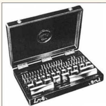
A commercial boxed set of slip gauges. This full set comprises 81 blocks plus two protectors which will permit the user to set dimensions to the nearest 0.0001in.
