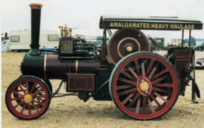
The 4in. Burrell 3-speed road locomotive built by Keith Morris; valve chest name plates have yet to be fitted.
