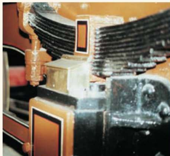
Axlebox details of HR No. 103 at Glasgow Museum; note stirrup link and suspension bracket and the finish of the spring buckle.
