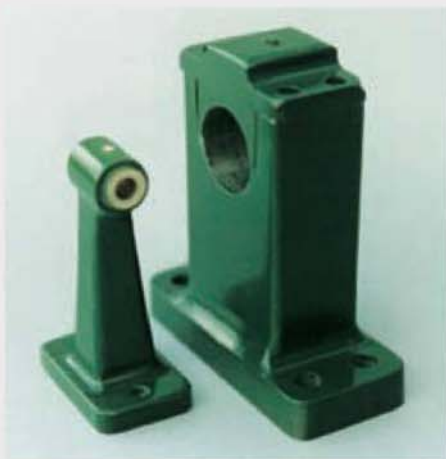
The appearance of items like pedestals was improved by the addition of a body filler fillet.
