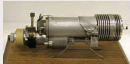
First ever in-line 10cc petrol ignition engine, one of twelve made in 1941 by Augie Savage (USA). The same principle is used in the Glowplug Aero '35' manufactured in 1963 which is also in the auction, as well as Russian in-line examples.
