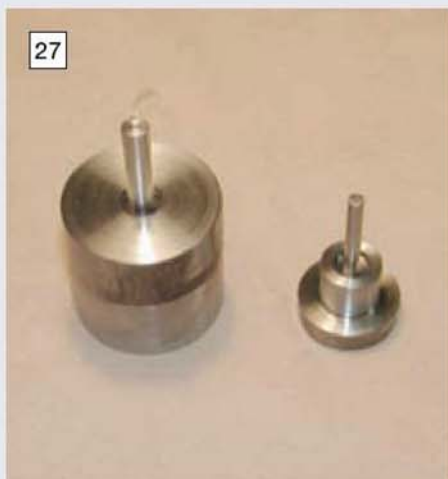
27 The two small fixtures used to align the crankshaft during assembly.
