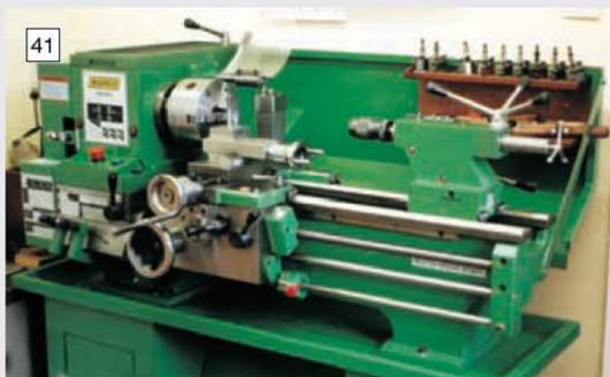
The Author's Warco BH600G lathe complete with the rack feed tailstock described in the accompanying text.
