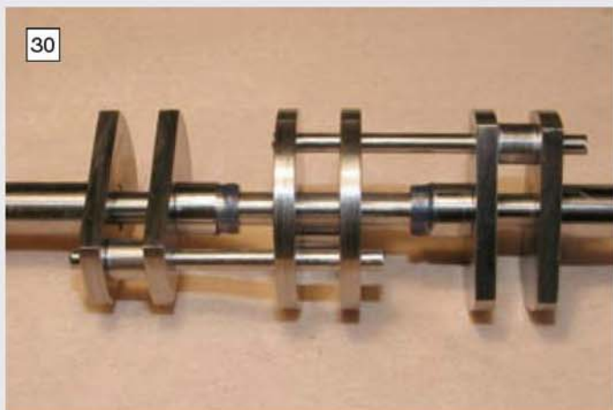
30 The penultimate stage in the crankshaft assembly process; note the rods which ensure correct alignment.
