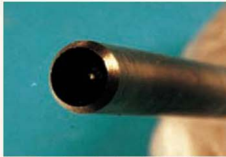
The ball turning tool cutting edge is provided by chamfering the edge to a central hole.
