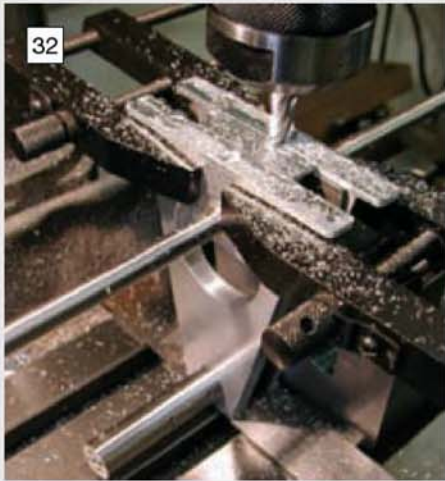
Cleaning off the bases of the supports to ensure that they are all true and aligned.
