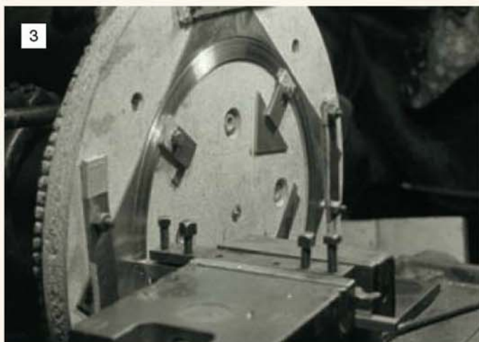
Trepanning out an annular gear ring. This operation was too large for the lathe and was carried out on the milling machine.
