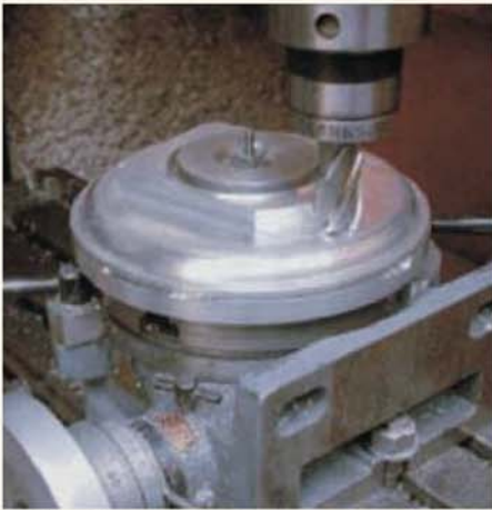
Profiling the rear side of the supercharger cover on the rotary table.
