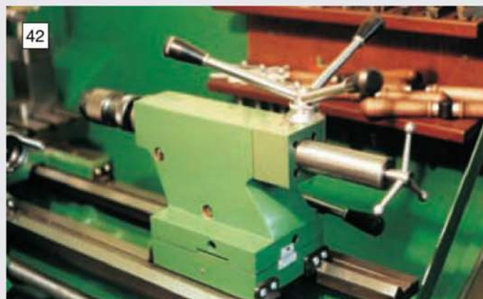
A view of the modified tailstock showing the neat and businesslike appearance of the rack feed mechanism.
