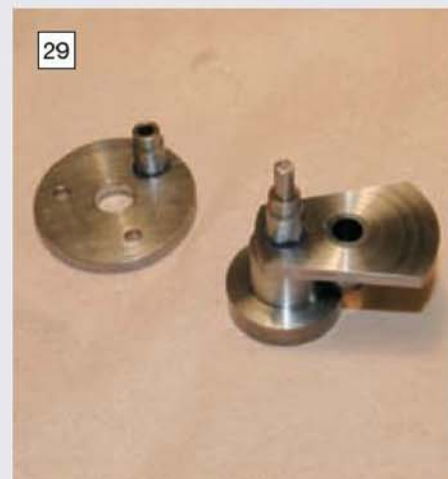
29 The other fixture being used to assemble cranks to webs.
