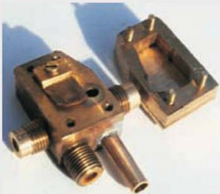
Inside the Author's flap valve injector.
