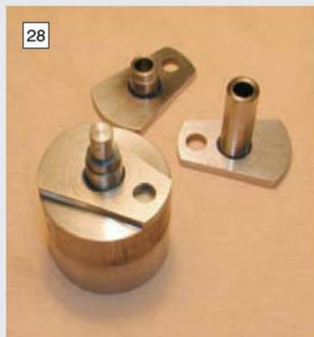
28 One of the fixtures in use to assemble the last journal/web assembly.
