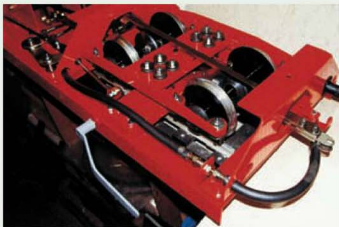
The Author's new passenger car featuring the pivot-less bogie design as displayed on the SMEE stand at the 2003 Harrogate show.
