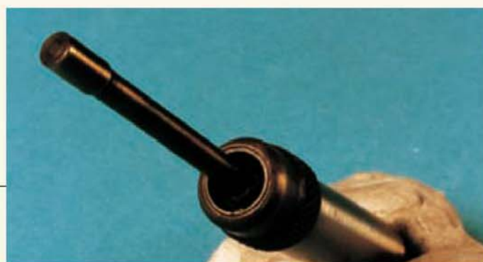
The hollow body of the wobbler houses the ball seating of the probe. A light spring keeps the probe on its seat.
