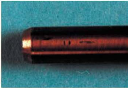
Side elevation of the simple ball turning tool for hand finishing the probe ball seat.
