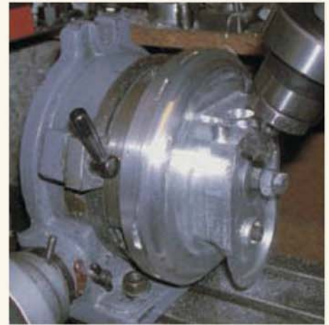
The set up for boring the angled inlet holes in the supercharger cover.
