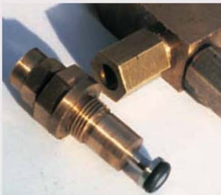
The poppet valve unit of the Author's injector.
