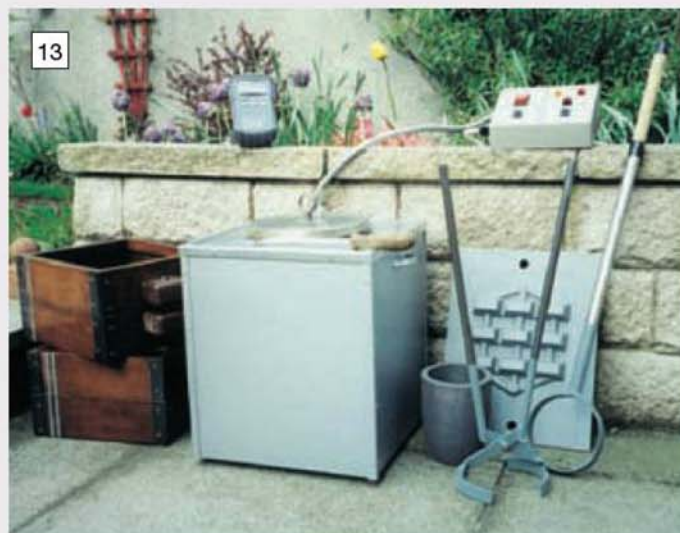
Finished and tested, the Author's small muffle furnace awaits its first melt. Note the tongs, ring shank and moulding boxes all made for the job.
