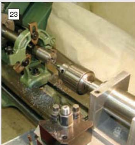
The holes in the webs were drilled using a drilling spindle mounted on the lathe cross-slide.
