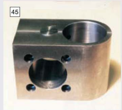
The finished gear housing after cleaning up and deburring but prior to painting.
