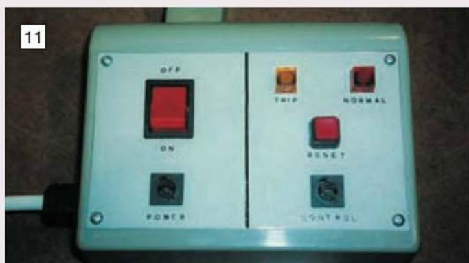
A view of the front of the control box showing switch, indicators, fuses, etc.
