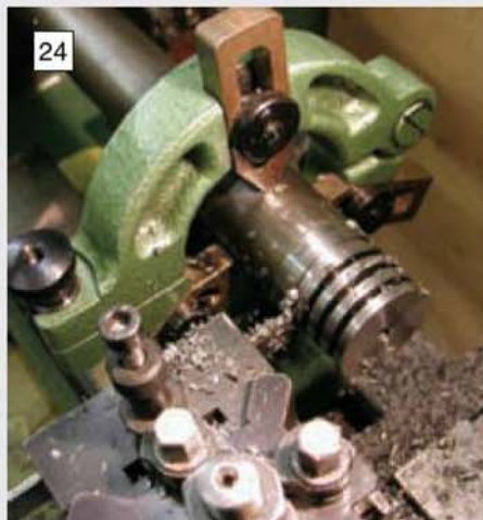
Defining the positions of the last four webs with a parting tool.
