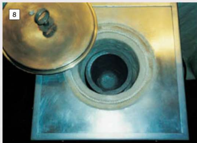
Furnace top showing cover with lifting ring and 6mm hole for the thermocouple probe. Note the glass cord seating for the cover
