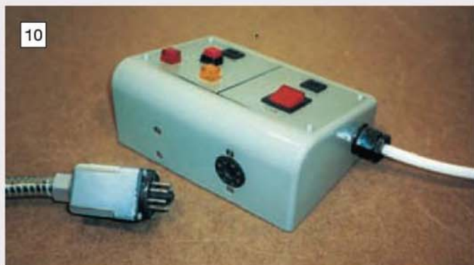
A multi-pin socket is fitted to the rear of the control box.
