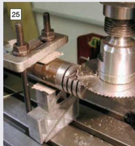
Excess material was removed from the crankshaft webs using a slitting saw.
