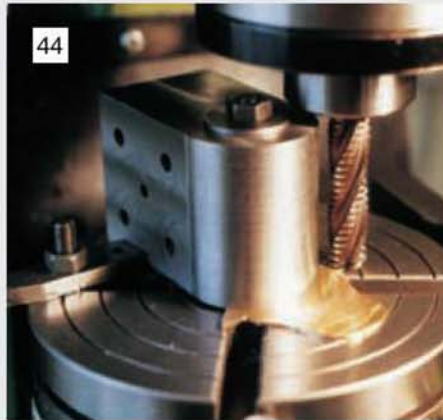
Radiusing the gear housing on the rotary table. Note the brass packing and method of securing.
