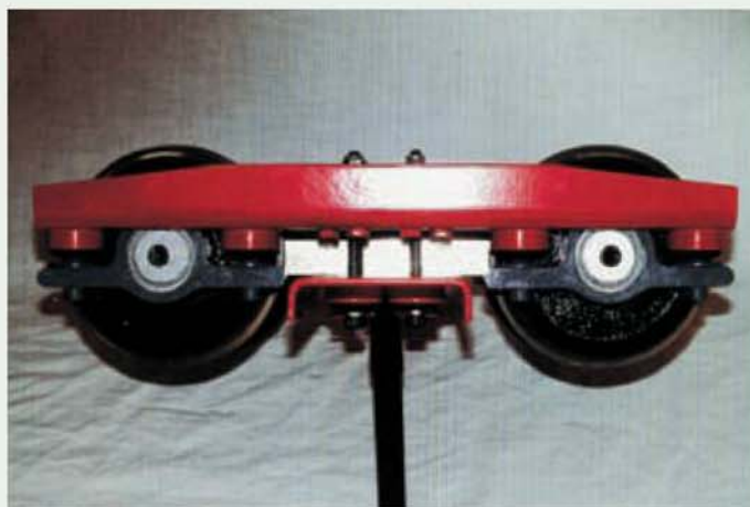
A side elevation of the bogie unit for the new passenger car. The excellent finish was achieved by powder coating.
