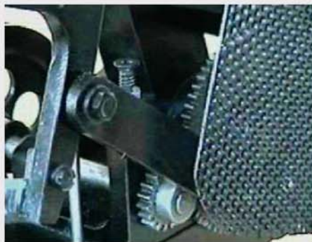
Close detail of the lifting link with the saw in the lowered position. The travel stop screw (centre) is adjusted to arrest downward motion when the cut is completed.
