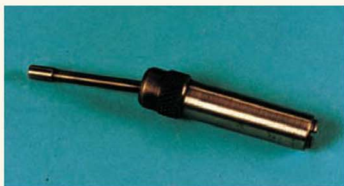
The Author's wobbler. Simple to make, this tool provides an accurate method of positioning features on a work piece with respect to its edges.
