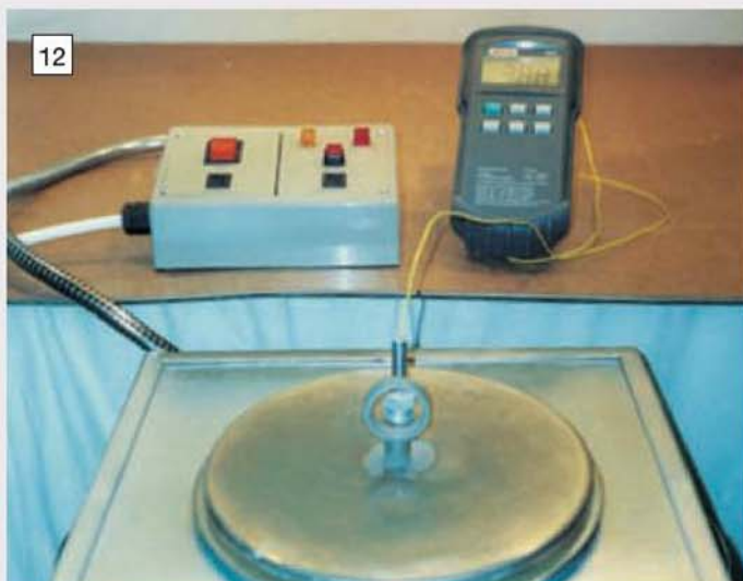
A view of the furnace on test showing the control box, digital thermometer, and thermocouple probe in place through the hole in the cover.
