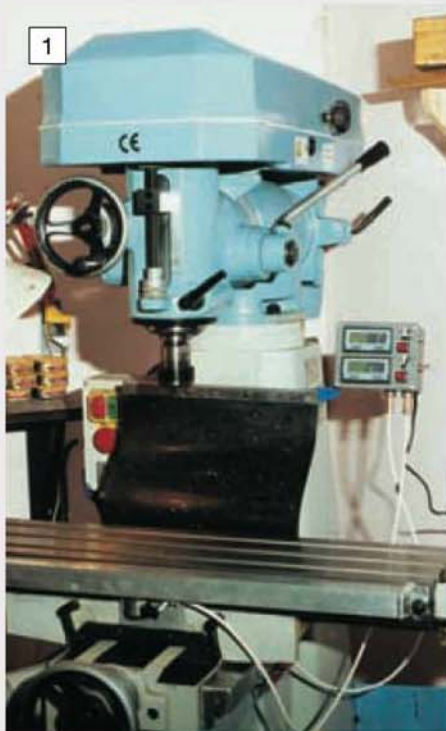
The Author's DRO unit fitted to his own Myford VME milling machine.
