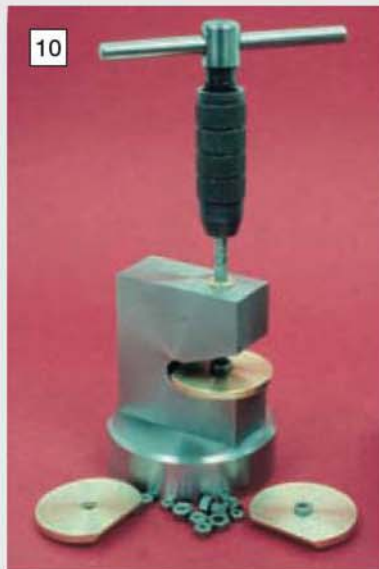
Using a split ring to hold the nut holder blank for turning operations on the lathe.
