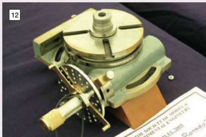
In addition to his fine regulator clock Bob Lilley displayed this neat rotary table built to the design of David Piddington.
