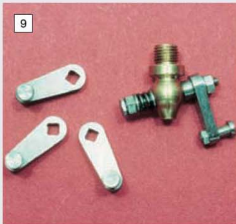
Above: drain cock levers with neat square holes.
