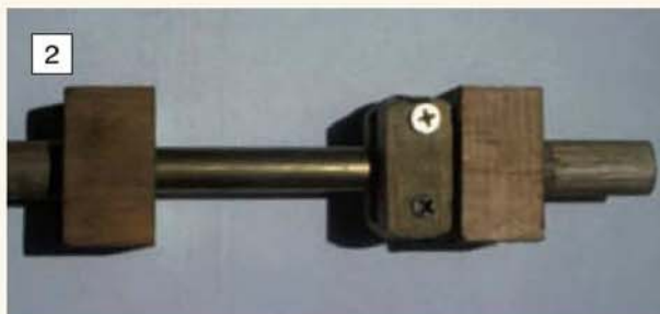
The method used to clamp the cylinder tube for machining the slot in the side wall. Care must be taken to avoid distorting the tube.
