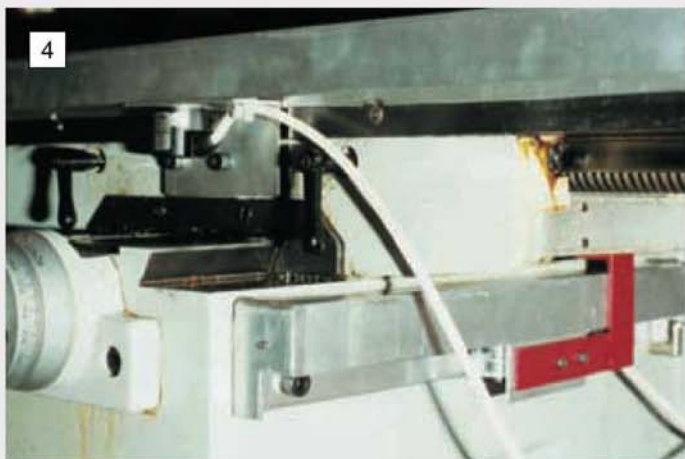
Both the X- and Y-axes are equipped with encoders and, as can be seen here, the installation is neat and business-like and protected from swarf.
