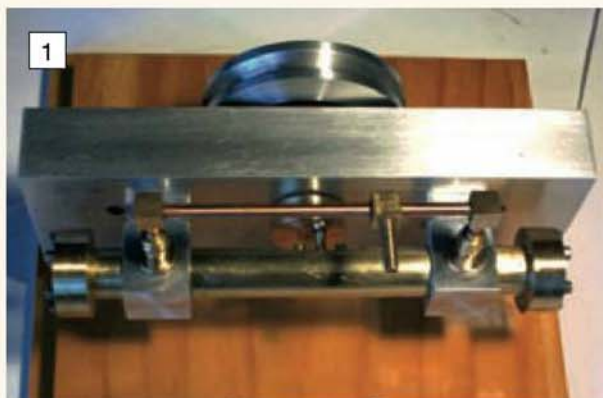
The author's twin-cylinder Twisty, a neat, well balanced and fast running engine of deceptively simple design.
