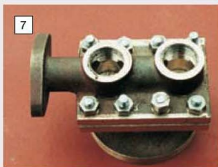
John Freeborne's two machined 4in. scale safety valve castings.
