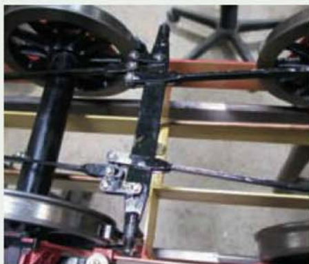
Rear compensating levers, rearmost pullrods, and train pipe again, this time where it crosses from right to left side and is clipped to the frames front and middle. Its rear end is supported from the standpipe, not yet fitted.
