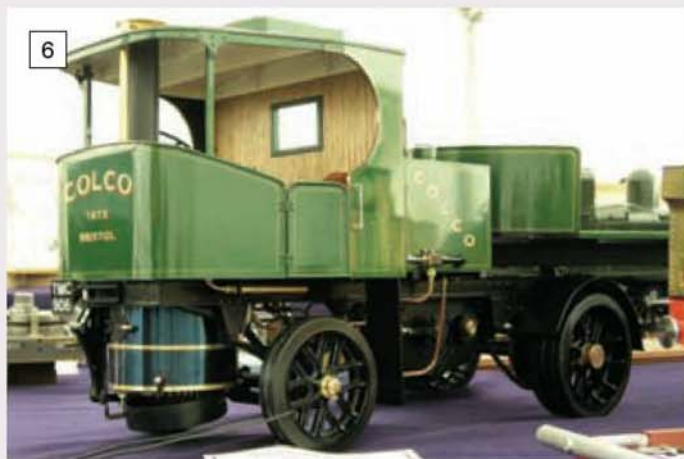
6 This Clayton articulated undertype steam wagon was the work of Tom Collins and looked very refined in its green livery.
