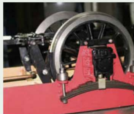
Opposite side, similar details. Note colouring, for these tenders will be coupled behind Bulldogs, and 'Indian red' is used for frames in their prime. Inside I have used 'light buff'.
