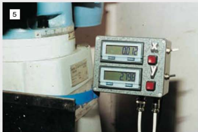
The digital readout box features backlit 12mm characters and is mounted on the right hand side of the machine for convenient viewing.
