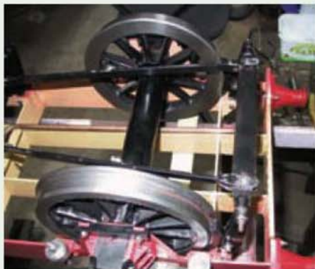
Underside rear end view of the Author's 3000 gallon tender showing the brake gear. Note the 'train pipe' about halfway up the picture. One of the rear brake lever brackets can be seen above this immediately to the left of the crossbeam.
