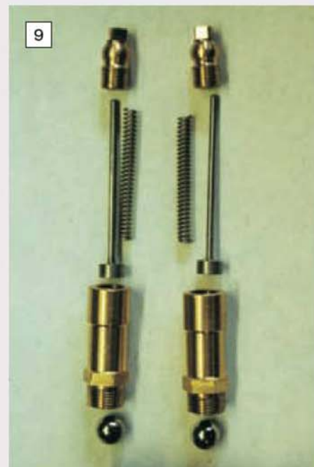
Disassembled chimneys, springs and balls. (Photo 7-9: P. Kybert)
