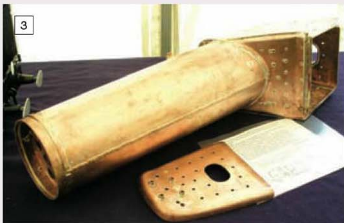
3 The first of three boilers for Lionel Flippance's latest project: three models of the designed but never built British Railways 2-8-2 heavy goods loco.
