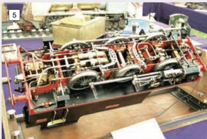
5 A worm's eye view of the gas fired Simplex chassis built by our contributor Peter Heimann.
