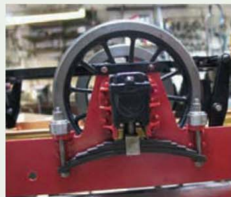
Side view of middle horns, axlebox, wheel, brake levers, springs, springbolts and shock absorbers.
