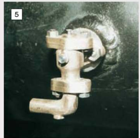
The completed clack mounted on the boiler. Note that the sides of the oval overlap the boiler pad to make a neat, close-scale fitting.
