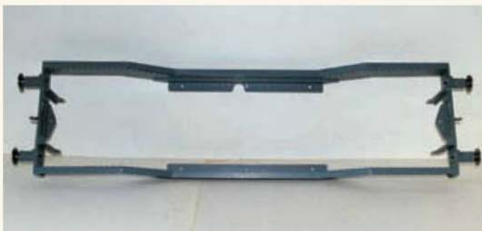
The chassis outer frame and buffer beams after fabrication.
