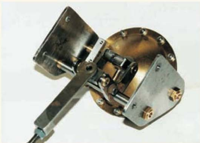
An underside view of the brake vacuum cylinder showing details of the brake linkage.
