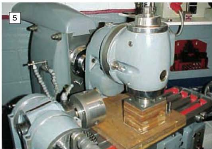
5 The main spindle draw bolt can then be released, the vertical head fixing screws withdrawn and the head brought forward using the cross-slide.
