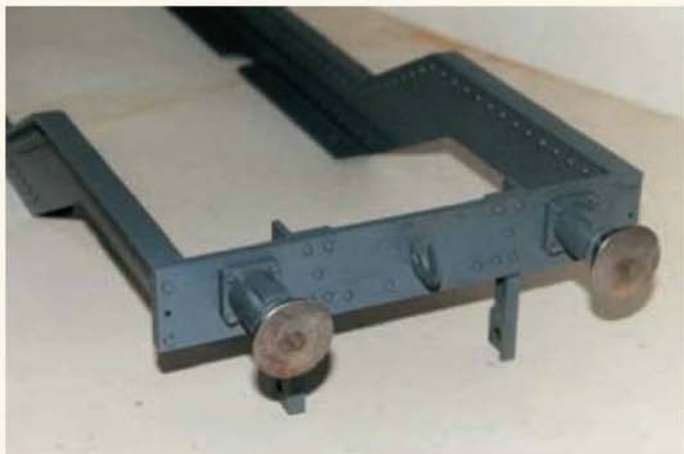
Buffer beam detail. This shot was taken before the chassis spine had been added to the assembly.
