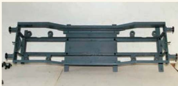
The two parts of the chassis have been united and things are taking shape.
