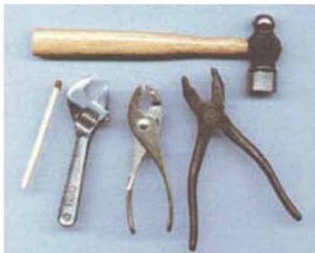
The pliers and the adjustable are steel forgings.
