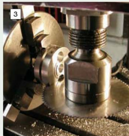
3 The holes having been drilled and tapped, the first pillow block is separated from the bar.
