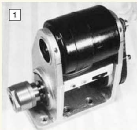
The neat mill/drill built by the author for use on his Myford Super 7 lathe.
