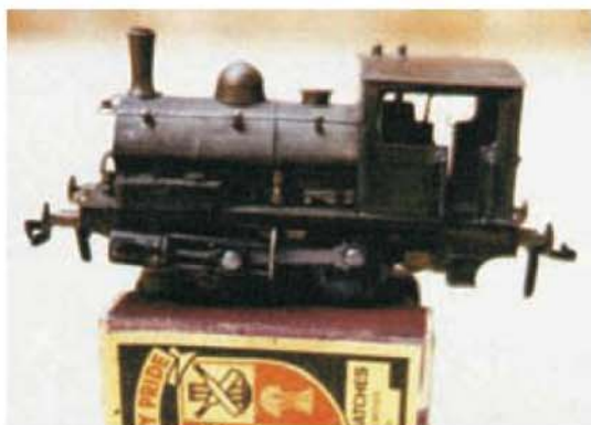
This delightful '00' gauge loco. was made from shim brass.
