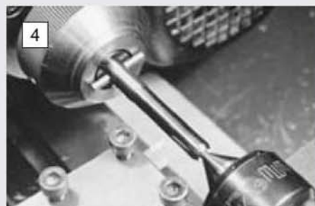
Right (top): the pinion blank is prepared with a leading chamfer and a small cross-pin.
