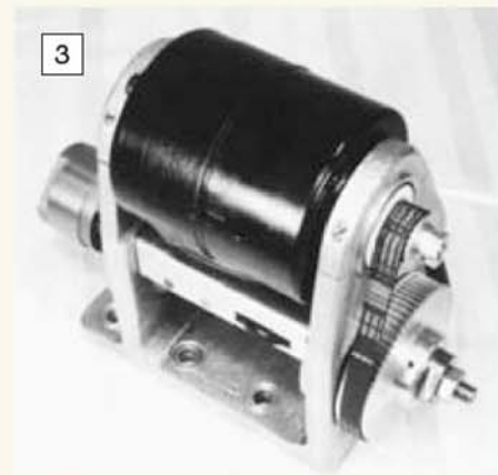
Another view of the assembly showing the toothed belt drive and the speed control knob.
