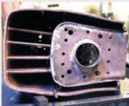
Rear end assembly of a Belpaire firebox locomotive boiler without its backhead during construction showing the firebox, crownstays and part of the foundation ring in place.
