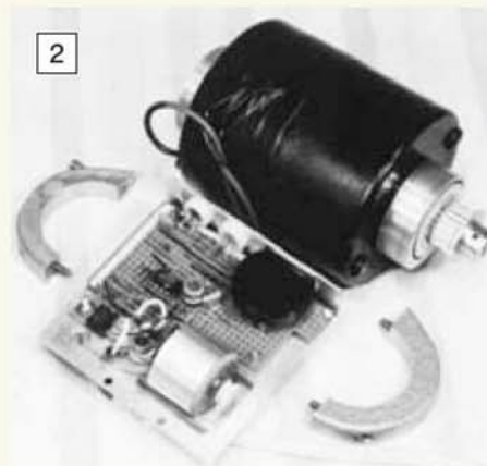
A view of the electronic speed control circuit and the motor used to drive the tool.
