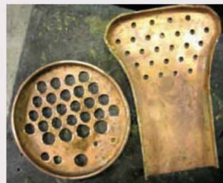
A finished front tube plate (left) and a firebox tube plate (right) for a Belpaire firebox boiler. The pilot holes location the position of the tubes and will be opened out to an easy fit.
