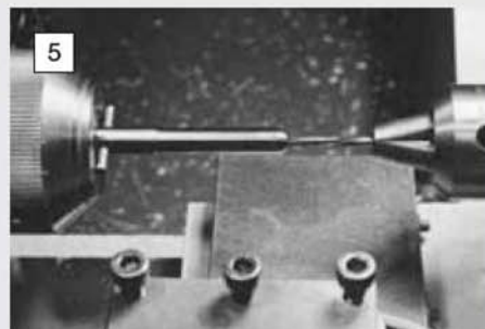
Right (bottom): the pinion blank is drilled and reamed for the arbor on which it will be mounted.
