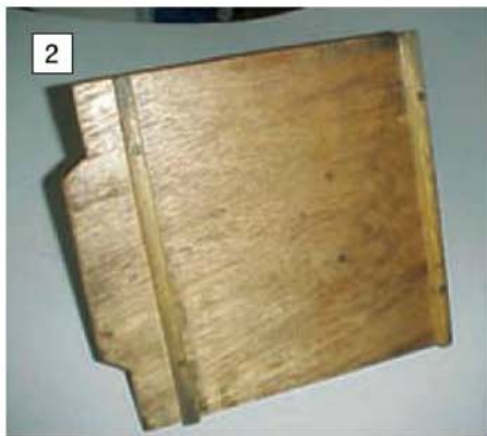
2 Battens underneath the stand locate it laterally on the milling machine table.
