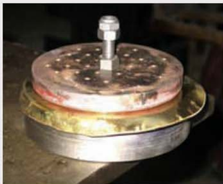
Plate-bashing thin gauge annealed brass sheet. The 'sandwich' configuration helps prevent the brass from lifting in the middle. Note the pilot holes in the tubeplate former (top).
