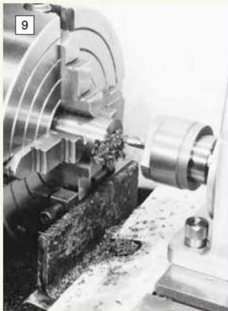
When undertaking milling operations it is wise to lock the lathe spindle. The clamp locking the chuck to the lathe bed can be seen in this photo.
