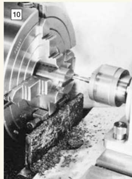
A \frac{1}{4} in. wide slot milled in the end of a work piece using a slot drill. Larger cutters tend to overload the drive motor of the mill/drill.
