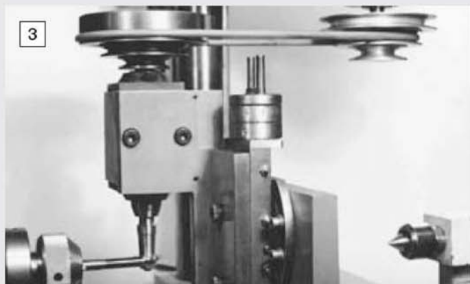
Left: the milling spindle is driven by means of a plastic belt.
