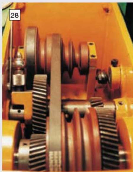
A view inside the headstock of the Author's lathe before the addition of the clutch.
