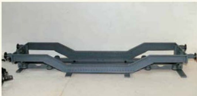
The chassis assembly after the spine and outer frame have been united.
