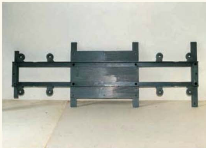
The Lowmac chassis spine and strengthening plate photographed during construction.
