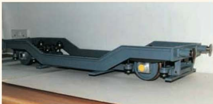
The chassis with the bogies fitted into place.
