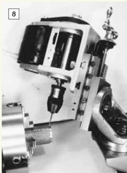
Drilling compound angles using the mill/drill mounted on the swivelling vertical slide.
