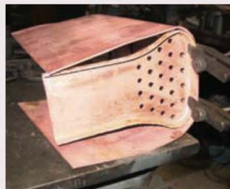
An early point in the assembly of the firebox. The annealed wrapper will be shaped to conform snugly to the front tubeplate profile. Toolmaker's clamps are a useful aid at this stage.
