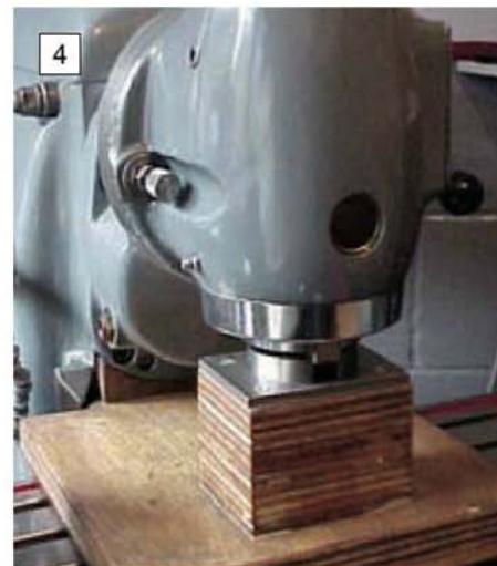
4 The knee is then raised, the spindle orientated to locate the dogs and the draw bolt nipped up.
