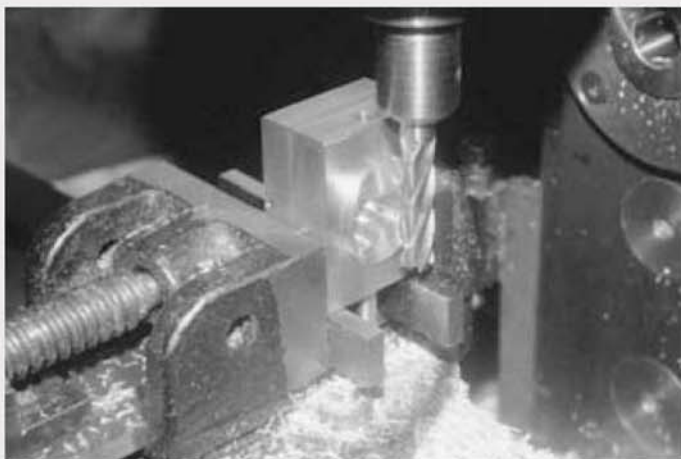
Machining the pistons across the bottom recess clearance. The fixture is a brass block bored to suit the piston. A rod locates the gudgeon pin hole.
