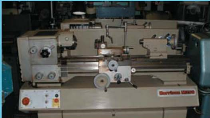
Boxford VSL, 5" x 19", power feeds & gearbox, variable speed to 2000rpm. C/w 3 & 4 jaw chucks, face & catch plate, Q.C. toolpost, tailstock chuck & center. Very late "top of the range" boxford in superb condition. £1475
