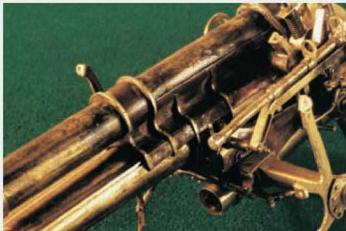
Further details of the barrel cradle, the rocking arm sight, the axletree and shield support brackets.
