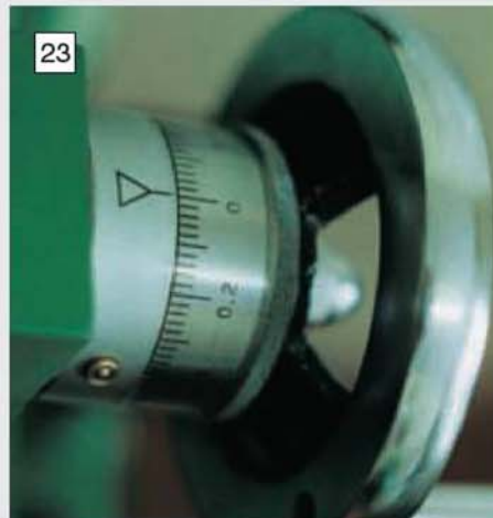
The new tailstock dial fitted to the lathe. All dials were made using G. H. Thomas' techniques.
