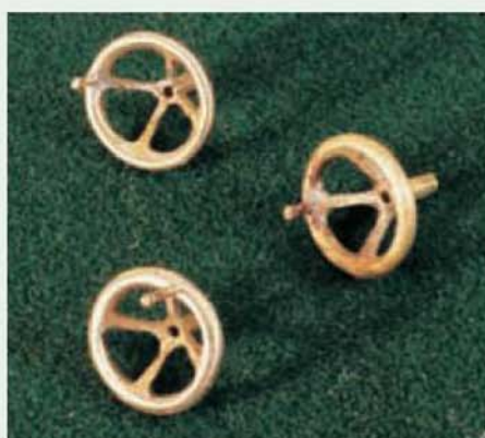
The hand wheels for the elevating and range gear were turned from \frac{1}{2} in. dia. brass bar, pierced and filed to final shape.
