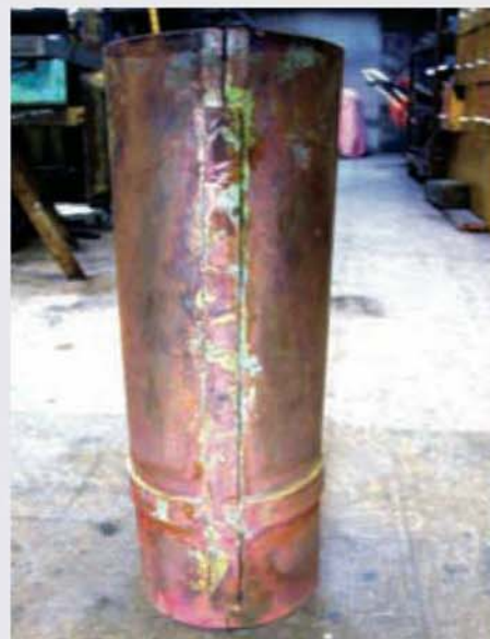
External view of the 7 1 / 4 in. gauge GWR Bulldog boiler barrel during construction; note straps.
