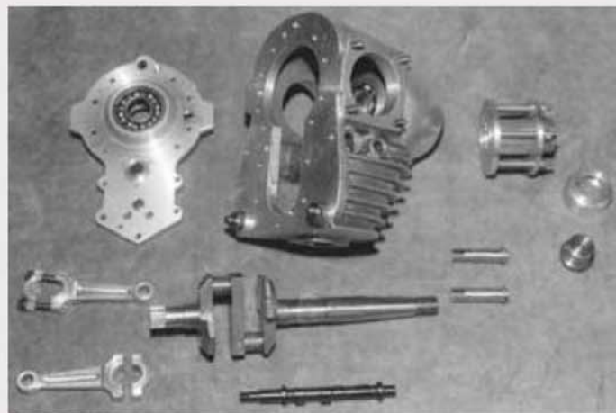
The 'bottom half' of the engine laid out for inspection showing some of the components described so far.
