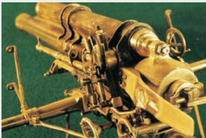
Further details of the elevating and range gear as well as the left hand layer's shield and the breech.
