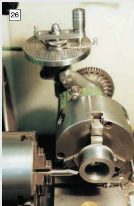
26 Dividing an index dial using a small dividing head on the lathe cross-slide.
