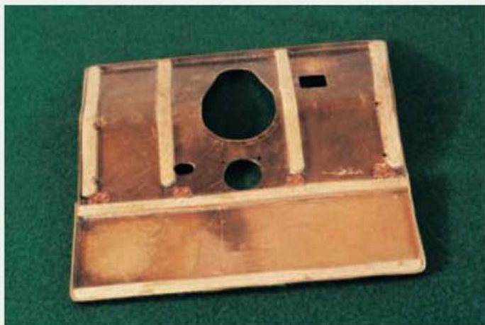
The shield was fabricated from copper sheet stiffened with wooden battens. The edges were beaten over an aluminium alloy former.
