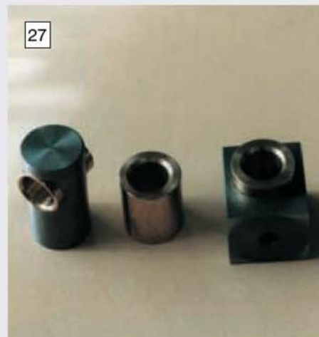
27 The set of new 2mm pitch feed nuts made for the Author's lathe.
