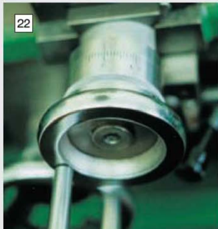
The new cross-slide dial fitted to the lathe. This metric dial shows actual slide movement.
