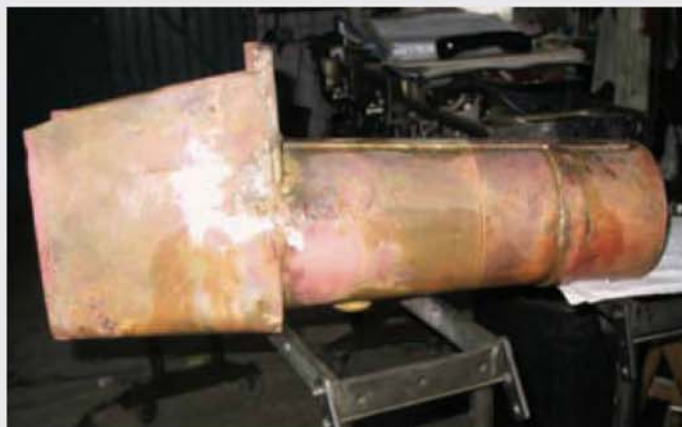
Boiler outer components silver-brazed into an assembly await further work.
