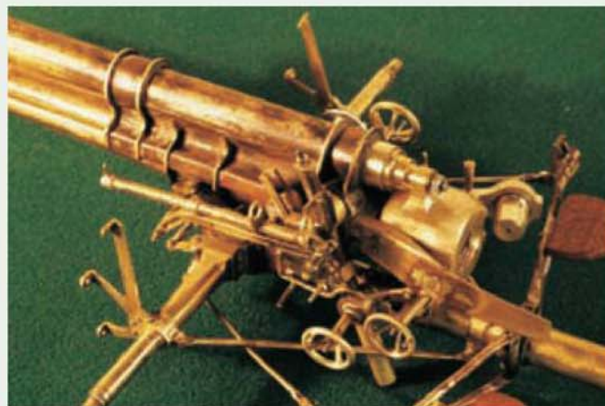
The elevating and range gear mechanism assembled on the model.
