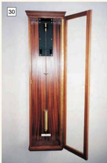
Finished glazed case fitted with the movement mounting fixture and pendulum.
