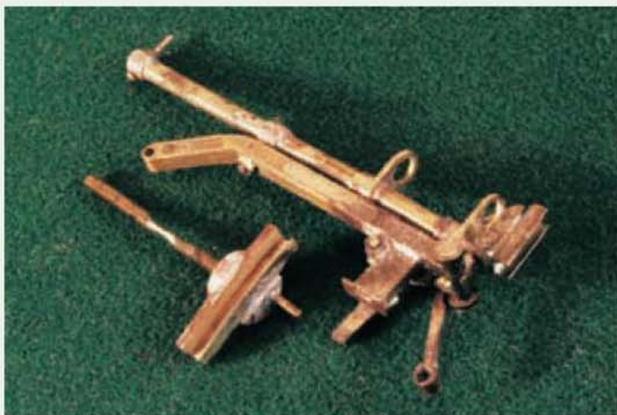
The rocking bar sight with connecting link and curved guide for the range arc.
