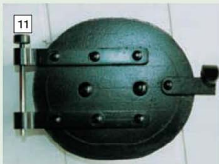
The firehole door should be profiled to fit the opening; in this case John's 4in. model. (Photos 11-12: P. Kybert)
