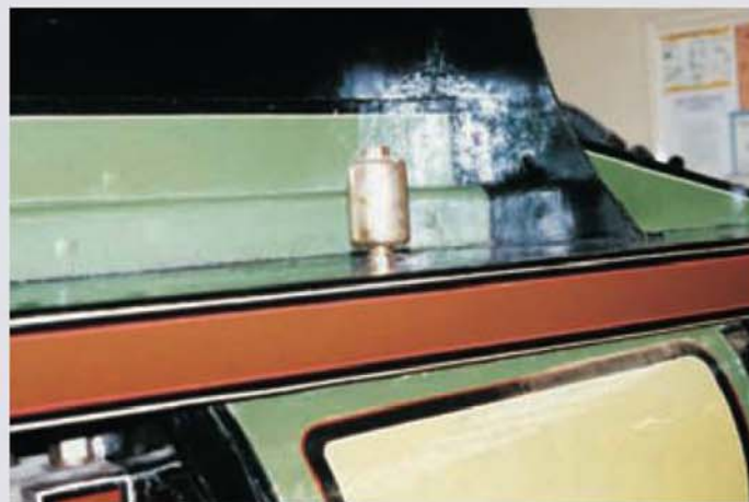
A simple cylinder displacement lubricator is fitted to the 'Big Goods' but the designs varied.
