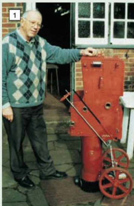
John Freeborne with his 4in. Little Samson . The engine's undignified position here facilitates access when fitting the grate and ashpan.
