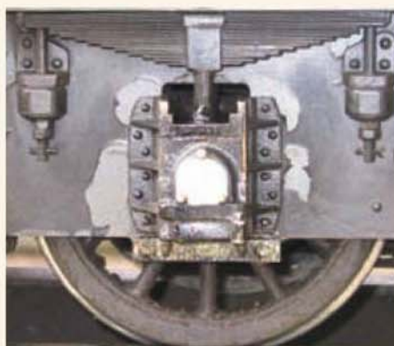
Axlebox, horns and springs on a Hawkesworth high-sided 4000-gallon capacity tender.
