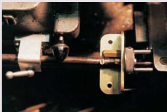
Stripped of its clamps, the device is shown bolted to the regular saddle stop.
