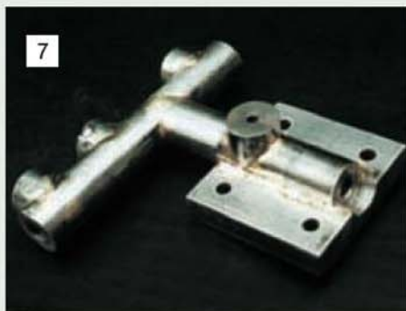
John's manifold after silver-soldering and cleaning up. Note the low profile, necessary to clear the crankshaft and motion.
