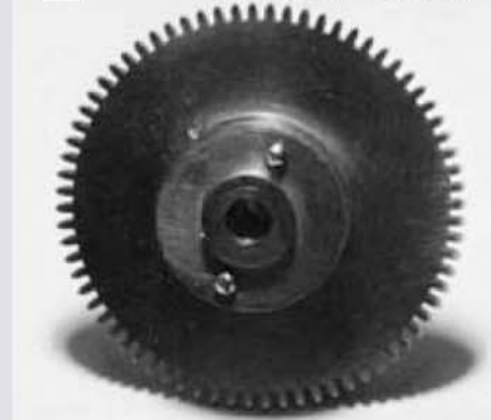
26 The two 10BA fixing screws on the sun/moon bush.
