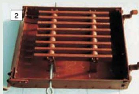
John's grate and ashpan are both fabricated, mostly from stainless steel.
