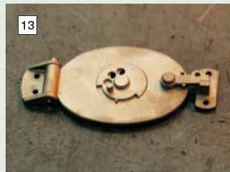
David has fitted a butterfly valve to provide top air over the fire which is claimed to improve combustion. (Photo: B. Camps)
