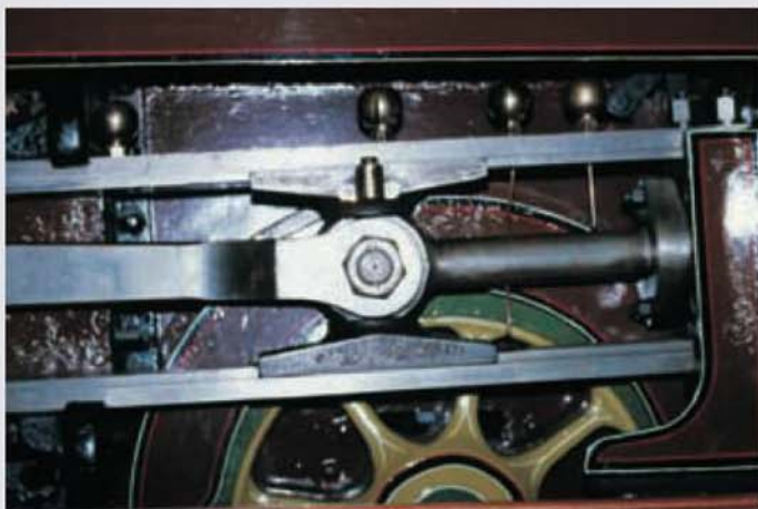
Four lubricators were fitted to the 'Big Goods' slidebars: HR No. 103 was photographed at the Glasgow Museum of Transport and Technology.
