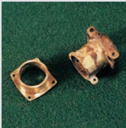
Trail brackets: left for the shield front support, right for the brake arm and tensile stays.
