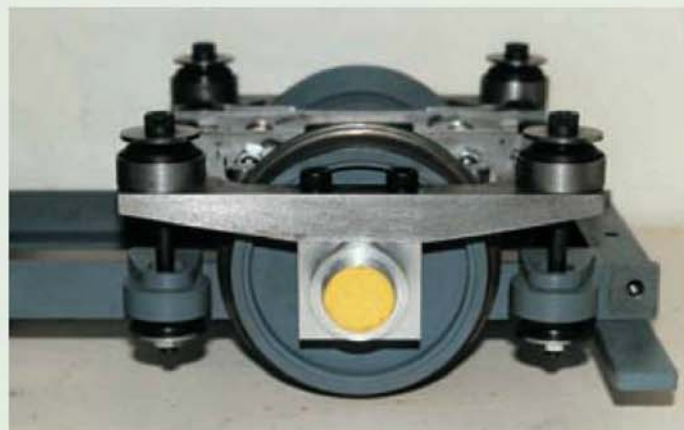
A view of one wheel set showing some chassis details, the axlebox and suspension arrangements.
