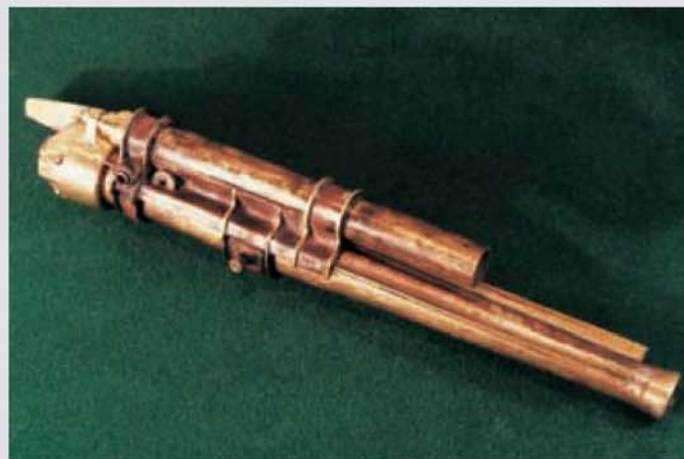
The barrel, breech, cradle and buffer/ recuperator sub-assembly. Note the mounting trunnions and the holes for the elevating and range gear spindles.
