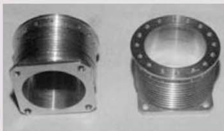
The finished Duralumin cylinders awaiting fitting of the cast iron liners.
