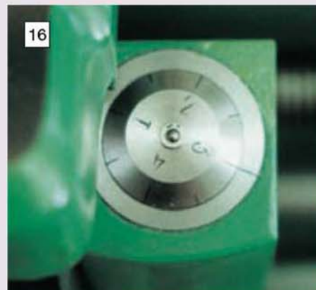
After re-assembly, the modified thread dial indicator is neater and easier to read.
