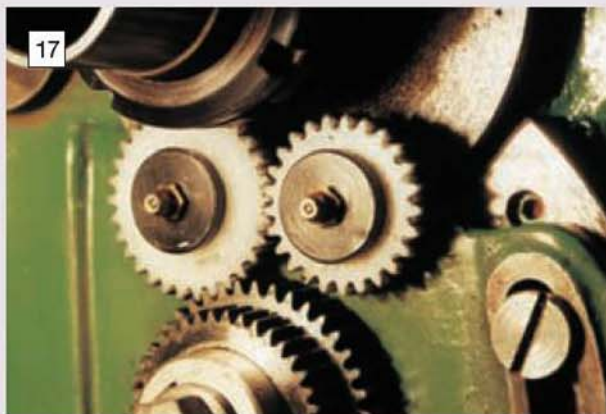
17 Nylon tumbler reverse gears were fitted to give quieter running compared to the standard items.
