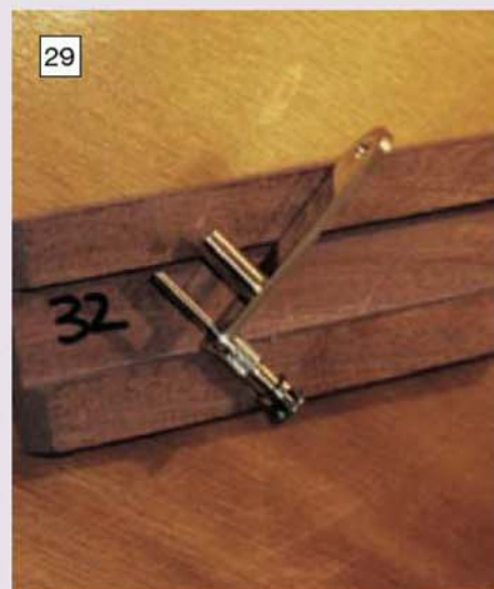
The optional seconds indicator was devised as the author missed seeing the second hand going round in step with the ticks.
