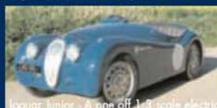
Jaguar Junior - A one off 1:3 scale electric Jaguar XK120 with integrated 'engine'
