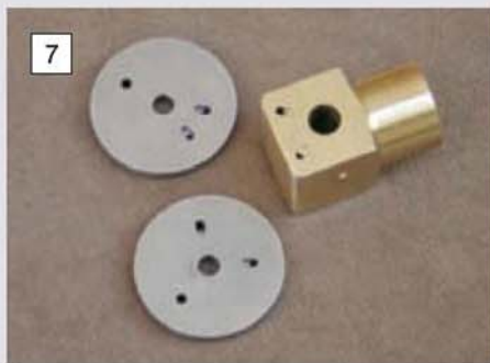
The common cylinder with two varieties of port face for the boxer engine.
