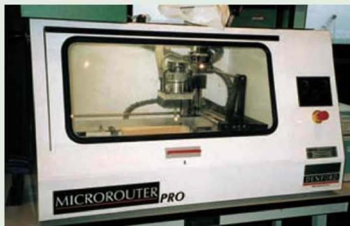
One of the Denford Microrouter CAM machines used for profiling the body.
