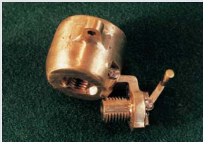
The breech ring with interrupted screw mechanism. The thread used was \frac{9}{32} \times 32\text{tpi} ME thread.
