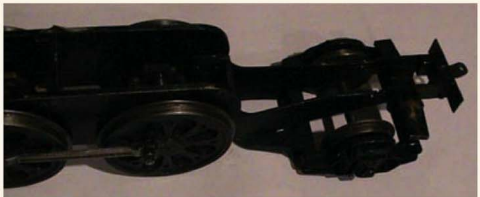
Above: a view of the trailing truck which pivots on the rear frame stretcher as described in the accompanying text. The performance of the model will not be impaired by the omission of outrigger truck bearings.
