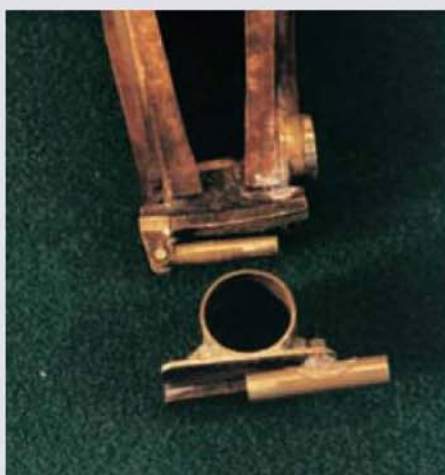
The traversing bracket dismantled to show the method of construction.
