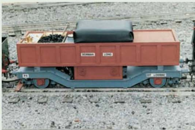
The 'Lowmac' driving car designed by the Author and equipped for use on ground level tracks.
