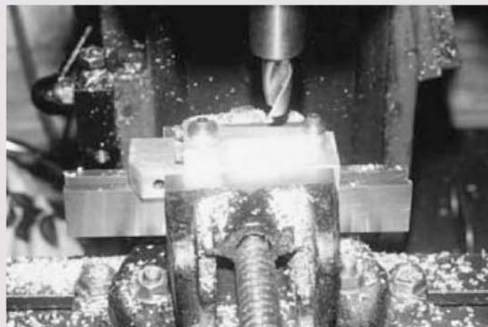
Machining the tapered sides of the connecting rod. The workpiece is mounted on a fixture held in the machine vice.
