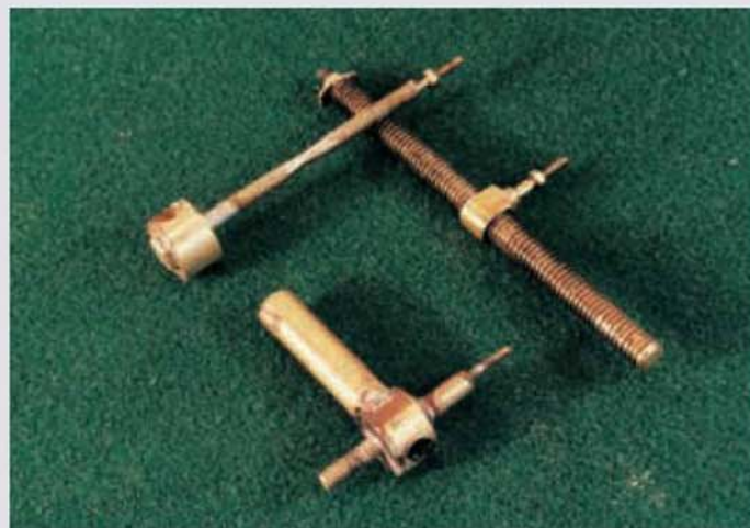
The screws, spindles and gearboxes for the elevating and range gear of the model. The gearboxes are not functional.
