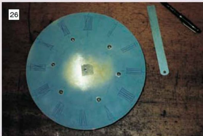
Once the marking out is complete the paper pattern and carbon paper can be removed leaving the image on the grey primed surface.
