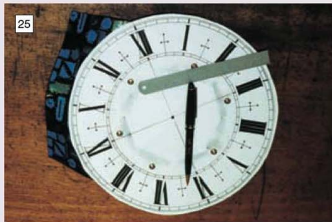
Transferring the numeral layout from the paper pattern to the brass chapter ring using ordinary blue carbon paper, a ball point pen and a steel rule.
