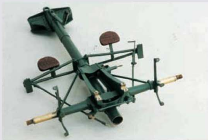
The carriage minus the gun, sights, elevation mechanism and shield during final assembly after painting.
