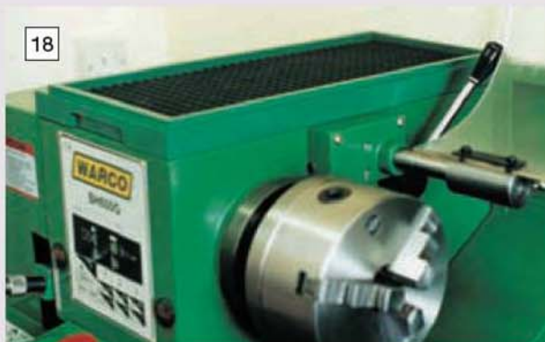
18 The new headstock belt cover was fabricated from aluminium alloy and is much lighter to lift than the standard cast iron one.
