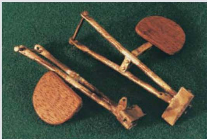
A close up of the two brake arms and brake blocks complete with the layer's seats. The seats were carved from close grained hardwood.
