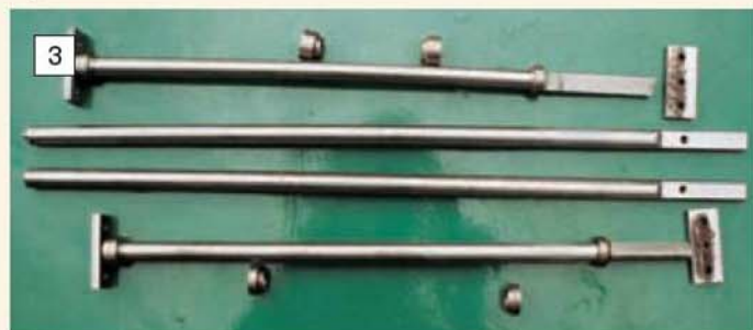
John's canopy stanchions before silver-soldering. The pair on the outside have their collars and plates in place. (Photo: P. Kybert)
