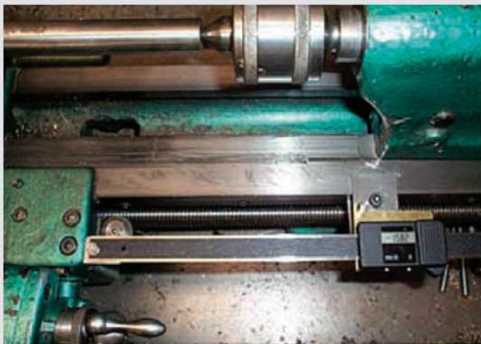
The digital read out slide bar fitted to the longitudinal axis of the lathe. The 8in. long unit is attached to the lathe bed via an adjustable bridge clamp.
