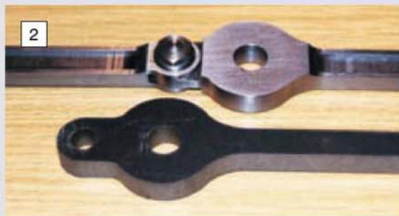
Right: the water cut side rod (bottom) required little work to finish (top)
