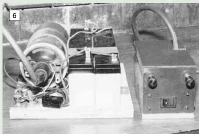
The new buzz box photographed alongside the old, bulky ignition source. The device is neater and less vulnerable to accidental damage.
