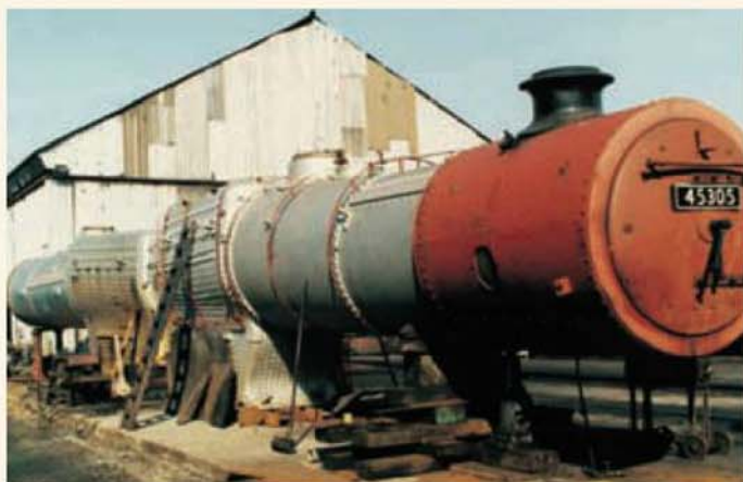
No, it is not a giant double Fairlie but two Black 5 boilers under repair and back to back at the Great Central Railway shed.
