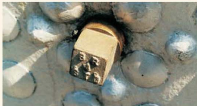
British Railways standard taper thread plugs which were said to be made from lead-bronze castings.
