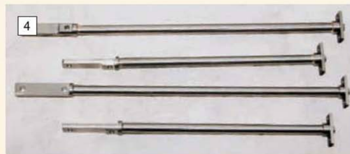
Stan's 3in. scale stanchions are silver-soldered and ready to be fitted. (Photo: S. Nipper)
