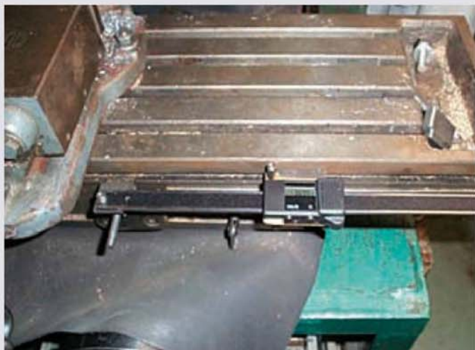
Set up used to mount the digital read out bar onto the longitudinal table axis of the milling machine. Some further simple brackets are used.
