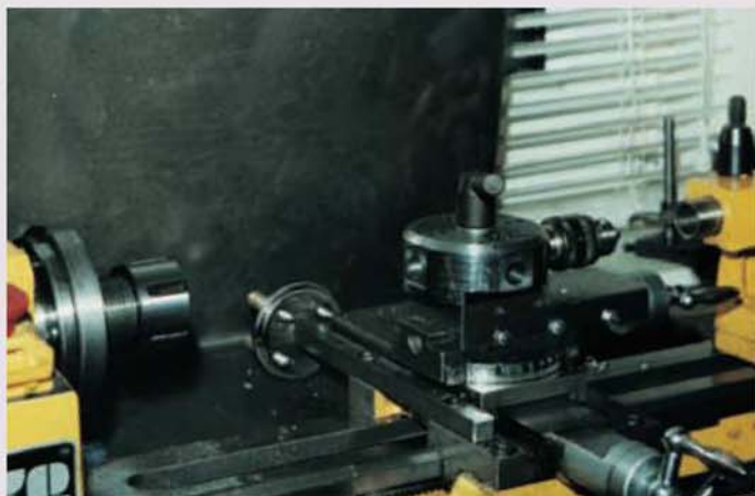
The turret and backstop assembly in use on the lathe. The turret can be indexed to bring various tools into operation, positioned by the backstop.
