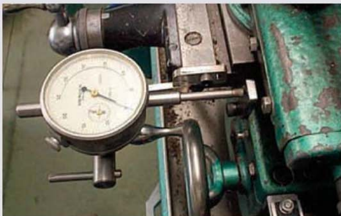
The arrangement used by the author to mount his dial test indicator to the cross slide of his Myford Super 7 lathe. The dti has 1in. of travel.
