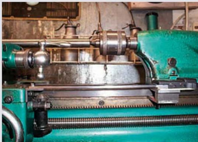
A further view of the slide bar assembly showing the method used to attach the unit to the saddle of the lathe with an angle bracket.
