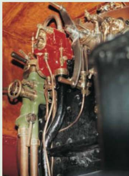
A general view in the cab of 'Big Goods' No. 103 of the Highland Railway on display at Glasgow Museum of Transport and Technology. Note the firehole surround and shelf.
