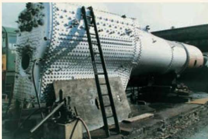
A boiler undergoing a hydraulic pressure test. Just like our model boilers but with everything on a bigger scale.
