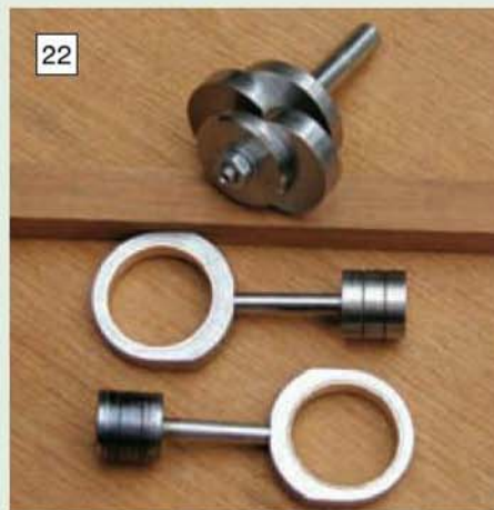
Assembled straight line crankshaft shown with its two piston assemblies.
