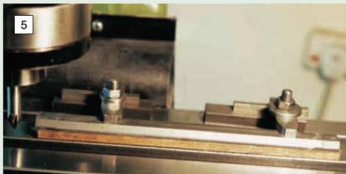
Cutting the bevels on the new gib strip in the milling machine using a 60deg. reverse dovetail cutter (similar to a countersinking bit).
