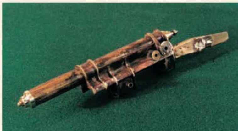
Cradle and recuperator assembly. The trunnion which forms an integral part of the central collar is clearly evident.
