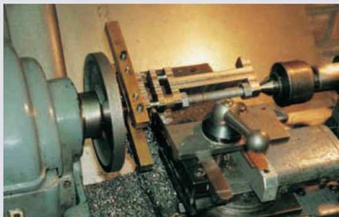
Set-up for turning the crankpins. The tool must be very rigid in order to avoid chatter and to give the best possible finish to the crankpin surfaces.
