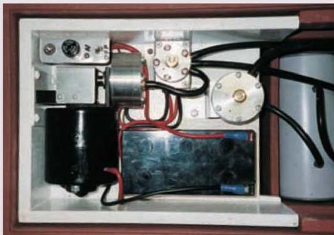
A view of the braking system as installed by the Author in his own driving car. Commercially available components are reliable and easy to replace.
