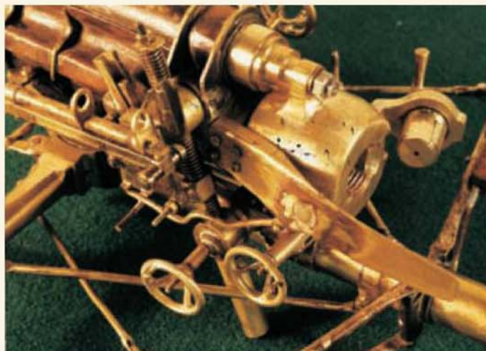
The breech mechanism in the open position. Note also elements of the elevating mechanism described in the accompanying text.
