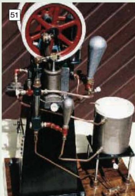
The Author's completed Heinrici hot air engine. The components were primed using an etching primer and finished with Hammerite paints of various colours. The simple air vent needle valve can be seen on the centre line of the engine just below the power cylinder. My trademark handle is scalloped for grip, not knurled. The permanent water tank is on the right of the picture.
