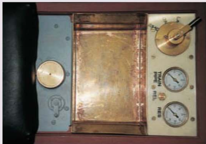
Brake control and pressure gauges. Brakes are applied slowly and surely with the lever set to 'ON' but an 'EMERGENCY' application is also available.
