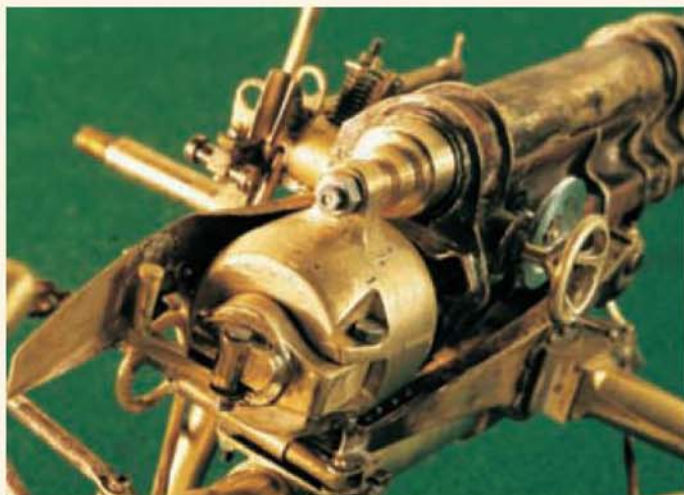
A view of the rear of the part-finished model showing the breech mechanism in the closed position.
