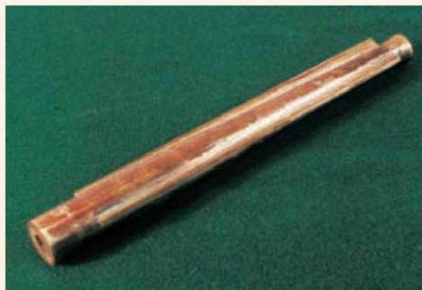
The barrel for the model. The recoil guides can be clearly seen. These form part of the outer jacket of the barrel of the full size gun.
