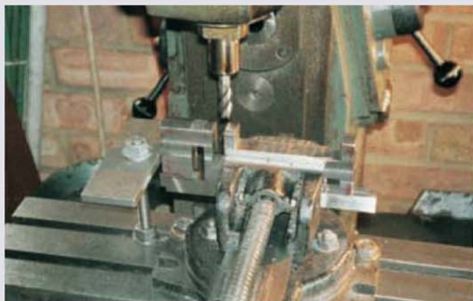
Using the milling machine to further reduce the blank to resemble the finished shape of the crankshaft.
