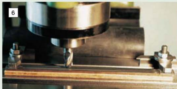
The gib strip was supported on tapered packing to facilitate the machining of its tapered form. It was made over long to facilitate clamping.
