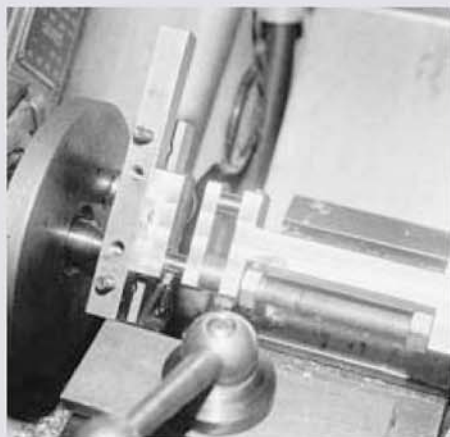
Another view of the crankpin turning operation. Note the brass packing piece and jacking bolt.
