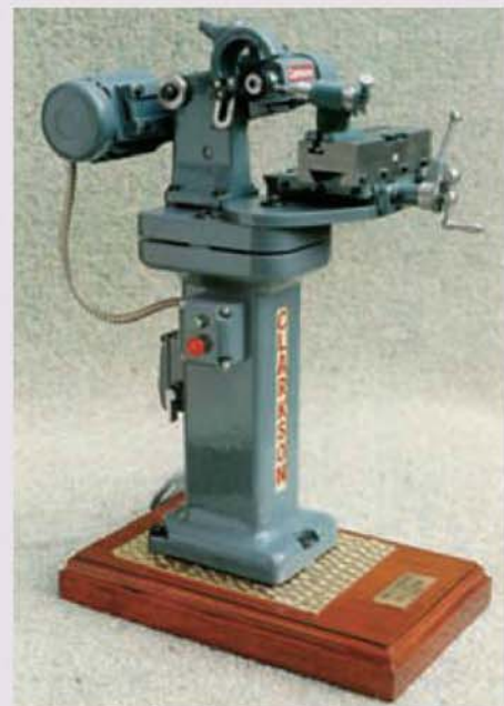
Barry's 1:5 scale Mark 1 Clarkson tool and cutter stands 14in. high and was completed between 24 November 1997 and 18 March 1998. It is made from cast iron billet, aluminium alloy section and mild steel stock without the use of castings.
