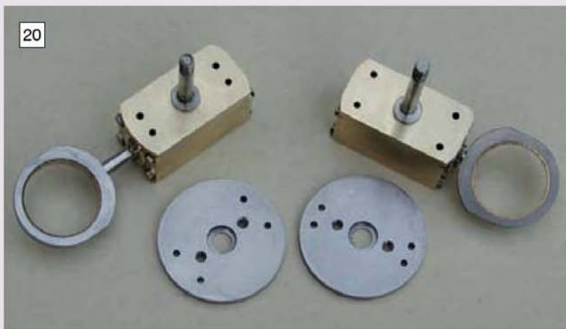
The V-twin cylinder assemblies and port faces. The double port system adopted for this engine can be clearly seen.
