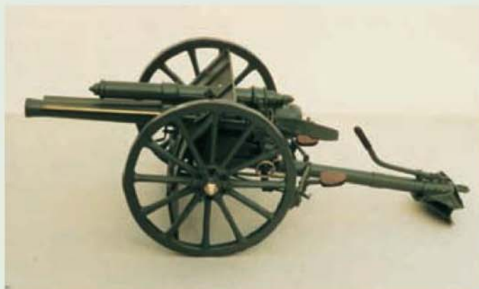
The wheels of the full size gun were constructed from a combination of pressings and timber and the model closely follows this approach.
