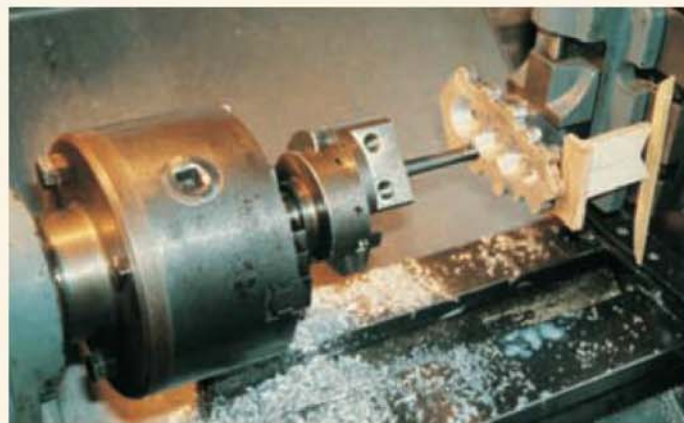
Machining the gear cover plate in the vertical slide. Note the wooden packing at the bottom end.
