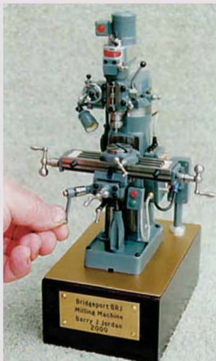
After seeing Jerry Kieffer's miniature models, Barry was inspired to build a smaller version of the Bridgeport. This 1:14 scale model is also functional, although Barry prefers to work in the larger 1:5 scale because his models are able to function more like the originals in that size.
