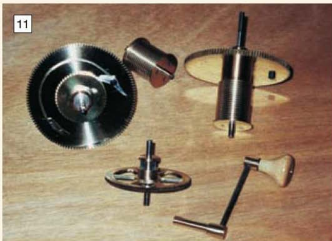
The great wheels assembled with their clicks and springs together with the intermediate arbor and winding key.
