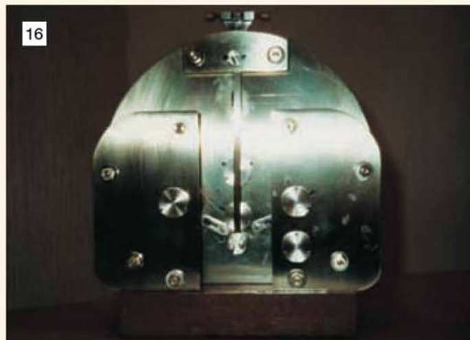
16 Another view of the back of the movement showing the crutch in position. Time to see if there is some life in the movement!
