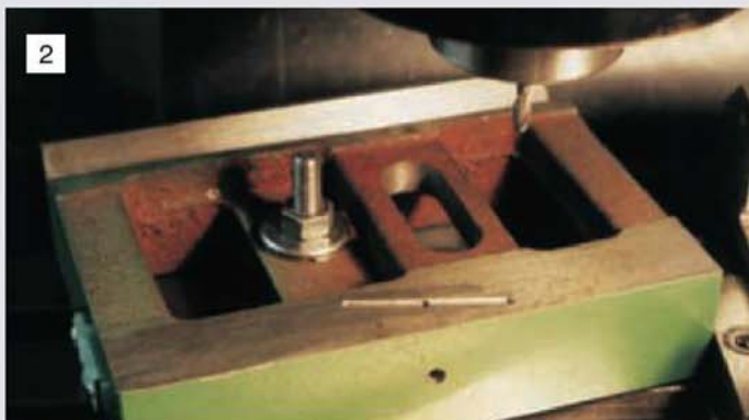
2 Machining an oil groove in the base of the tailstock to improve lubrication between the tailstock and the lathe bed.
