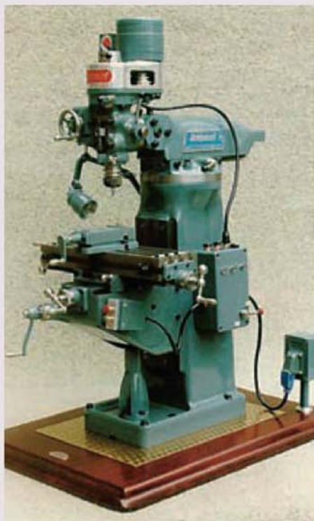
The 1:5 scale Bridgeport mill and machine vice. Barry's first complete project won many awards and was finished just in time for Bridgeport's 100th anniversary in 1997. Fully functional, no castings are used in Barry's models, even parts that look like castings are machined from solid stock.
