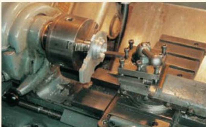
Boring the ball race recess in the back plate. The part is held by means of a turning spigot.
