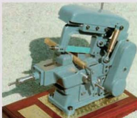
1:5 scale Qualters & Smith Sawmaster 6in. power hacksaw (6 January - 11 March 1999).
