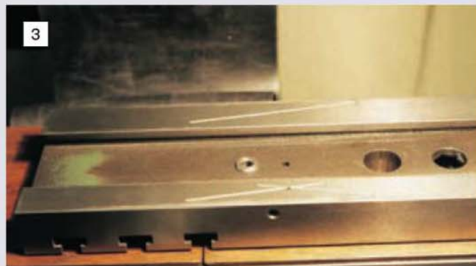
3 Machining the oil groove in the underside of the cross-slide. A small ball nosed cutter was used for this operation and that on the tailstock base.
