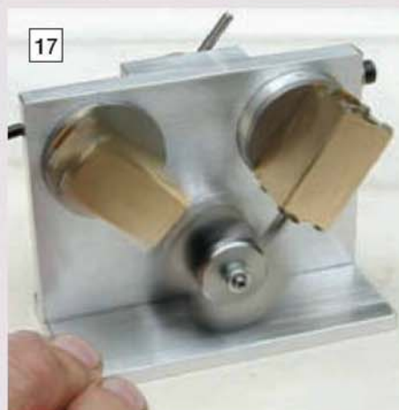
17 The V-twin running. The fifth engine to be built, this was an adaptation of engine T4.
