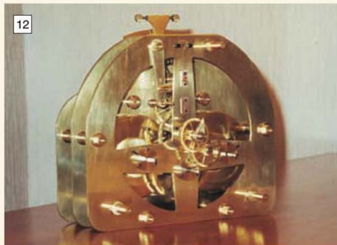
A front view of the clock movement assembled for testing prior to fixing the barrels to their arbors and other final adjustments.
