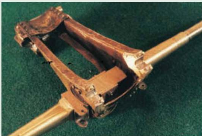
Top view of the carriage showing the method of attachment of the trail yoke to the axletree. Note the curved flanges to permit traversing.
