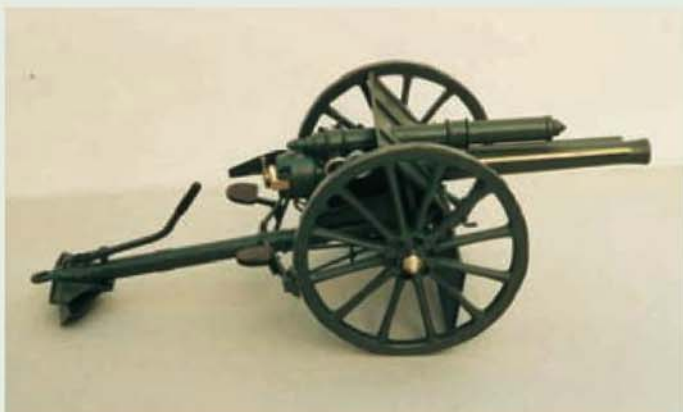
The model of the 18 pounder QF gun built by the author. The term QF (quick firing) denotes the use of a brass cartridge case for the propellant charge.
