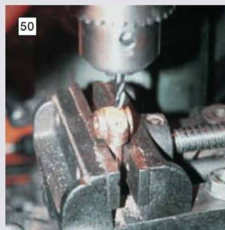
50 Finishing the power piston connecting rod end by counterboring and slitting the bearing.
