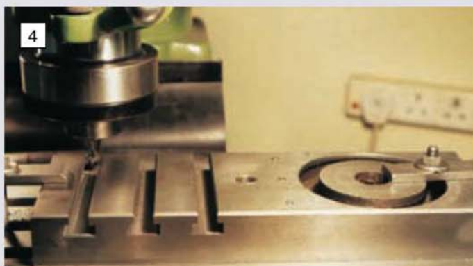
4 Machining an extra T-slot on the cross-slide to give more scope for fitting a vertical slide, dividing head or rear tool post.
