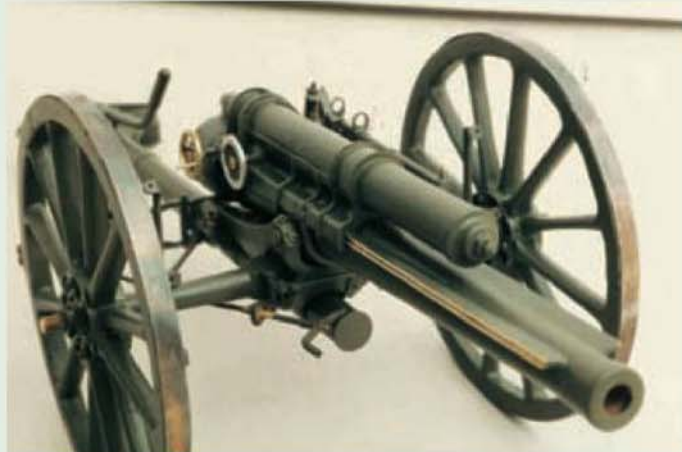
A three-quarter front view of the model without its shield. The provision for allowing the barrel to slide in its mounts upon recoil can be seen.
