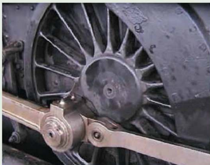
Left-hand Manx driver, note balance weight detail.
