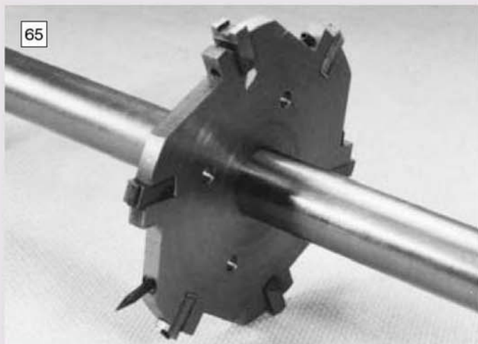
The cutter devised for machining the displacer slots. Note the detachable spur used for setting.
