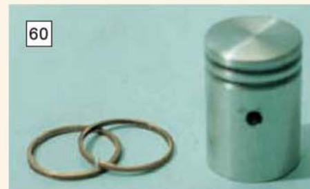
The piston and rings. The rings shown are bronze but cast iron is a better choice of material.
