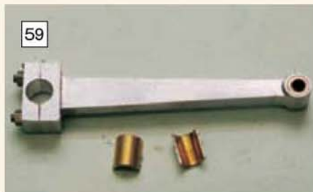
The completed con-rod with pressed in small end bush and big end shells awaiting fitting.
