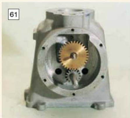
61 The timing gears in position in the timing chest. Note the larger, bronze gear is on the camshaft.
