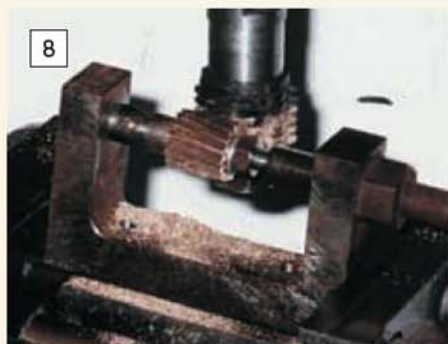
Left: the final tooth profile is formed on the worm wheel by a process known as free hobbing.
