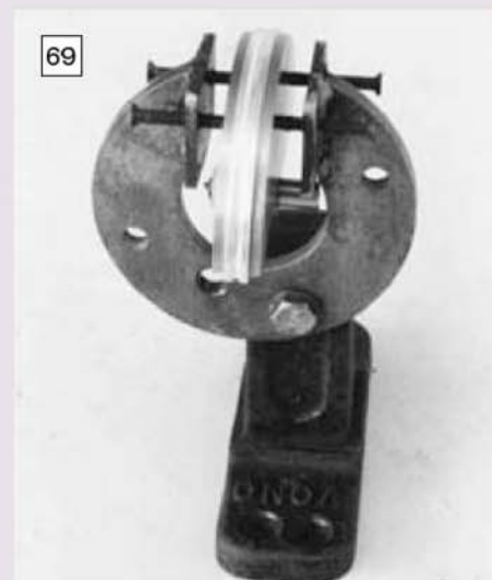
Original fixture used to hold the rotor halves together for welding. This was not a success.
