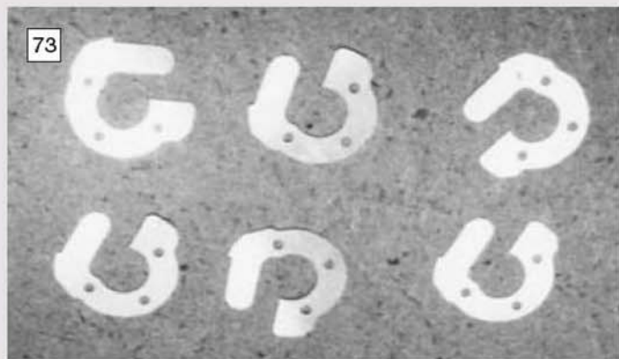
The set of flap valves after being released from their machining fixture. No further work was needed on these items.
