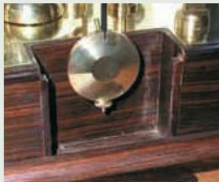
Right: The recess provided for the pendulum with its cover removed.
