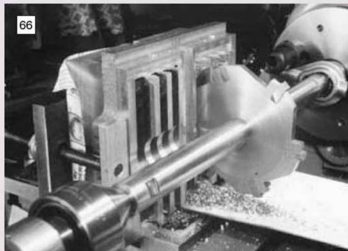
The cutter in use. It is mounted between centres on the lathe and could be used with power cross feed.
