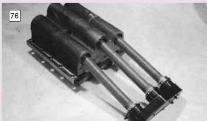
Three of the six electric heater elements withdrawn from their casting for the benefit of the camera.
