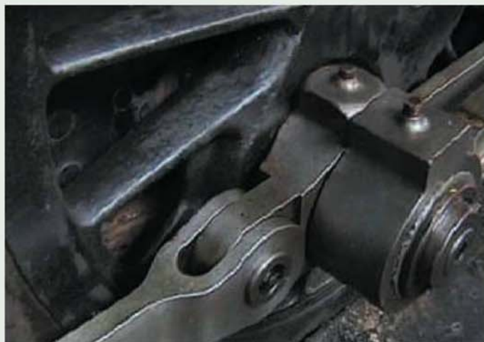
Note the shape of the coupling rod oilbox.
