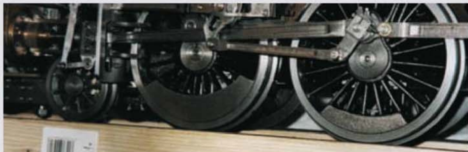
Some of the valve gear on the author's 3 1 / 2 in gauge 4-6-4 L&Y chassis.
