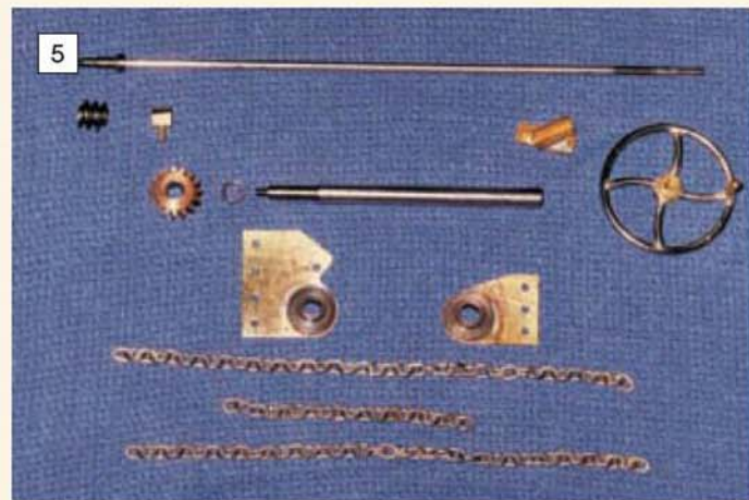
1in. scale steering components. The chain drum is just \frac{3}{16} in. dia. and the steering wheel fabricated from 2mm nickel silver. (Photo: J. Milne-Fowler)
