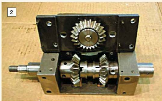
Gearbox assembly with bottom plate and idler gear ready for fitting.
