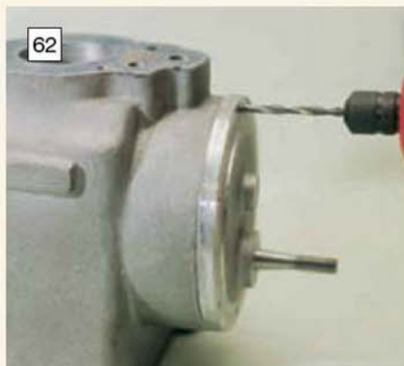
62 Marking the position of the timing cover fixing screws in the crankcase by spotting through.
