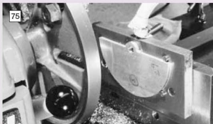
The fixture shown complete with a rotor in place for demonstration purposes. The idea may help someone with a fixturing problem.
