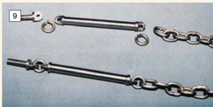
Right: handmade 3in. scale steering chain, spacers, and eyes to connect it to the chain drum. (Photo: S. Nipper)
