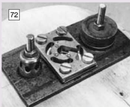
The fixture devised to make the 0.005in. thick flap valves used to control rotor internal pressure.
