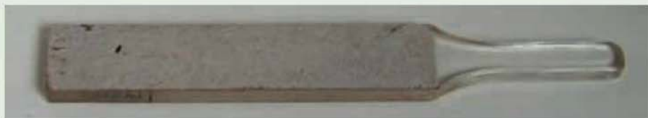
Top: The sandpaper file was made from a scrap length of Perspex.
