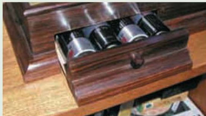
A drawer to the front houses the dry cells which supply power to the Archimedes screw drive motor.
