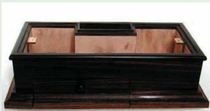
The wooden base constructed for the clock. It is constructed from veneered plywood and hardwood mouldings.
