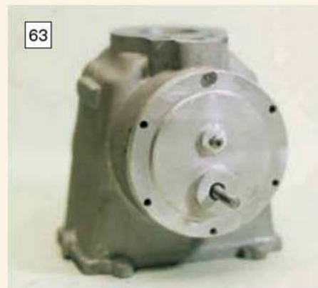
63 The cover temporarily attached to the crankcase with one screw.
