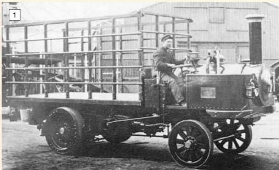
The Savage Universal Carrier was built with three types of boiler: the locomotive type (illustrated), a conventional vertical boiler or a water tube boiler. This contemporary photograph reveals that there is plenty of room for a dummy load containing a motor and battery (see accompanying text).
