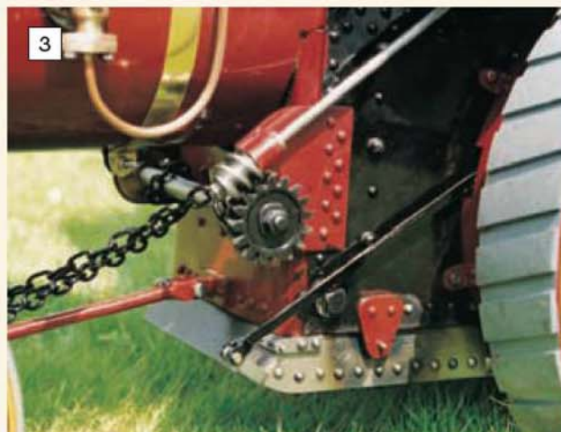
Stan Nipper's 3in. scale steering worm and wheel. (Photo: S. Nipper)
