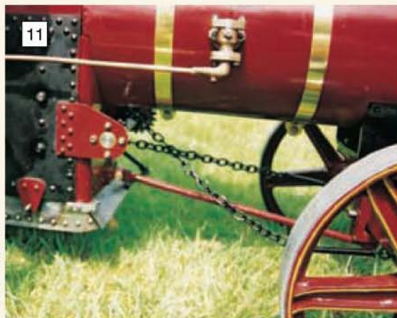
Right: the front axle stay bar connects the front axle to the throatplate. (Photo: S. Nipper)
