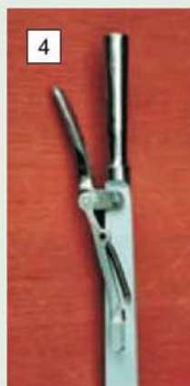
Left: component parts of John Freeborne's 4in. scale Little Samson reversing lever. Centre: the driver's end of John's reversing lever; note the beautiful finish. (Photos 3-4: P. Kybert) Right: the reach rod spans the gap between the reversing lever and the drop arm on the weighshaft. The upward kink is to clear the second shaft. Much of the reach rod ends up behind the second shaft gears and inside the gear casing. (Photo: S. Nipper)
