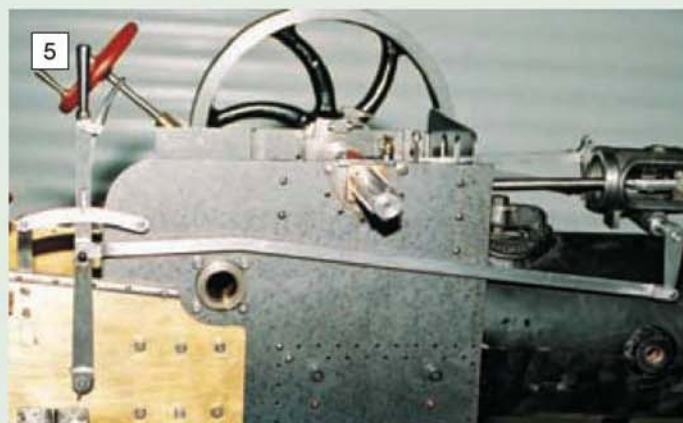
Left: component parts of John Freeborne's 4in. scale Little Samson reversing lever. Centre: the driver's end of John's reversing lever; note the beautiful finish. (Photos 3-4: P. Kybert) Right: the reach rod spans the gap between the reversing lever and the drop arm on the weighshaft. The upward kink is to clear the second shaft. Much of the reach rod ends up behind the second shaft gears and inside the gear casing. (Photo: S. Nipper)
