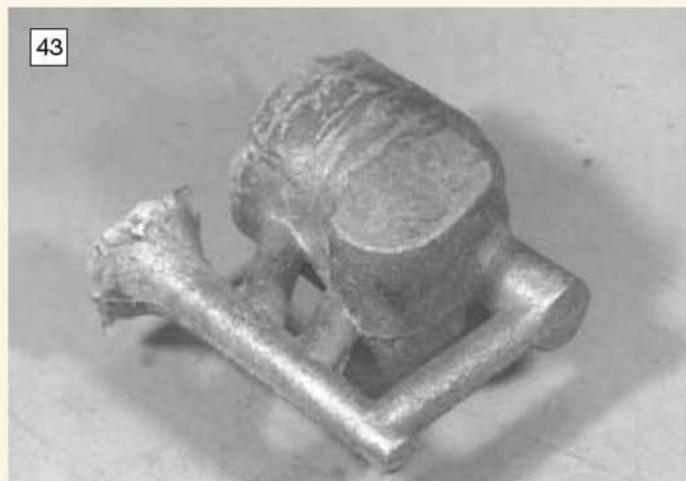
Success at last! This casting resulted from introducing the metal rapidly into the mould and taking care to minimise its contact with atmospheric oxygen.
