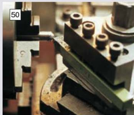
50 Machining the the valve head using a knife tool and the top-slide set to angle of 45 degrees.
