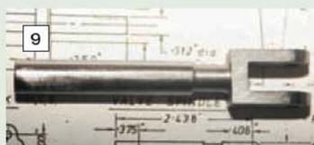
The completed valve spindle. (Photo: S. Nipper)
