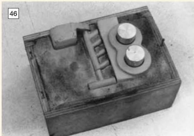
This view of the mould shows the pattern in position and the sand in the process of being rammed up; note the two chills.
