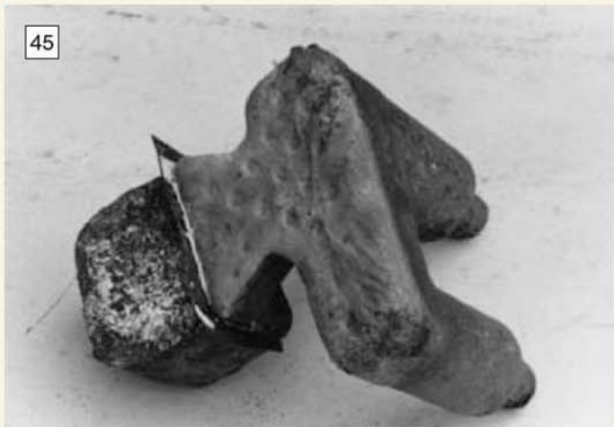
A simple brass casting made using a divided pouring basin (left) which encouraged the molten metal to flow cleanly into the sand mould (right).
