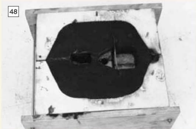
The two halves of the mould box have been securely assembled and the mould awaits its charge of molten metal.
