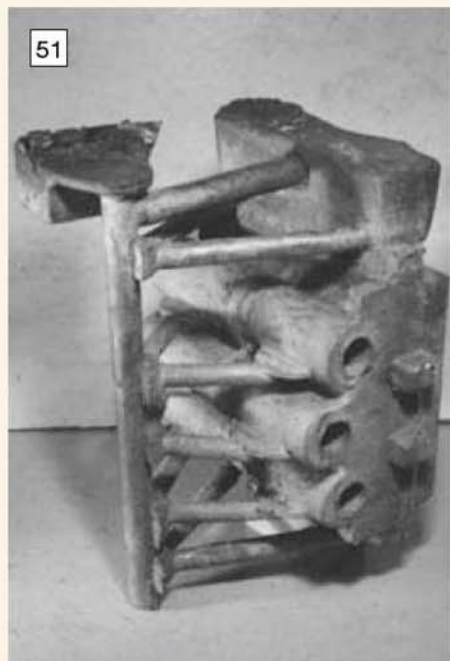
The Mk. 2 engine heater castings turned out very well in gunmetal.
