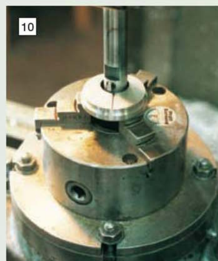
Cutting the keyway in the eccentrics using a milling machine slotting head and a rotary table to deliver the 21deg. angle. (Photo: B. Camps)
