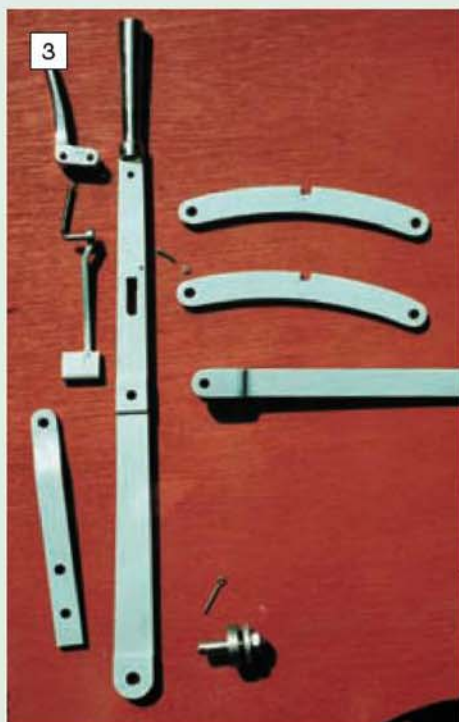
Left: component parts of John Freeborne's 4in. scale Little Samson reversing lever. Centre: the driver's end of John's reversing lever; note the beautiful finish. (Photos 3-4: P. Kybert) Right: the reach rod spans the gap between the reversing lever and the drop arm on the weighshaft. The upward kink is to clear the second shaft. Much of the reach rod ends up behind the second shaft gears and inside the gear casing. (Photo: S. Nipper)
