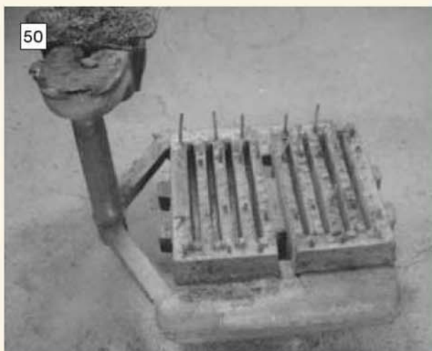
The Mk. 2 engine displacer castings were complex and involved considerable use of cores and a three-part mould with loose pieces.
