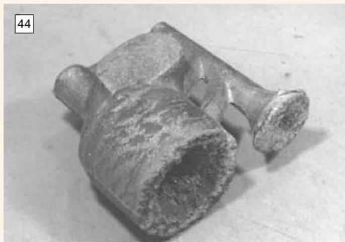
Another view of the successful brass casting; the use of a vertically split moulding box and several feeders also contributed to its success.
