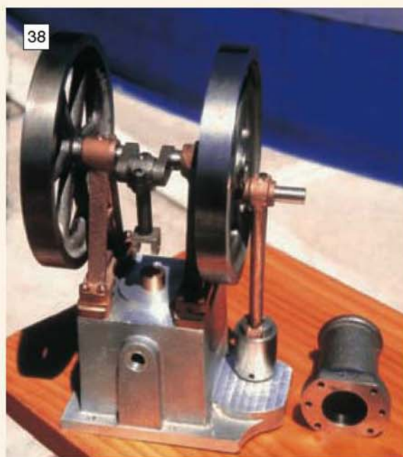
The third assembly of the components which now include the flywheels and 'A'-frame raising blocks. The tapped hole with the shallow counterbore for the outlet fitting from the water jacket can be clearly seen, and also the extended stainless steel crank pin, made deliberately longer than necessary in anticipation of using it somehow to drive a water pump, an idea which was later abandoned for an alternative drive mechanism.
