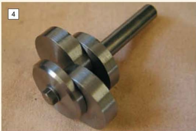
4: A straight-line crankshaft for a twin cylinder engine. The big end offset is obtained using eccentric disks.
