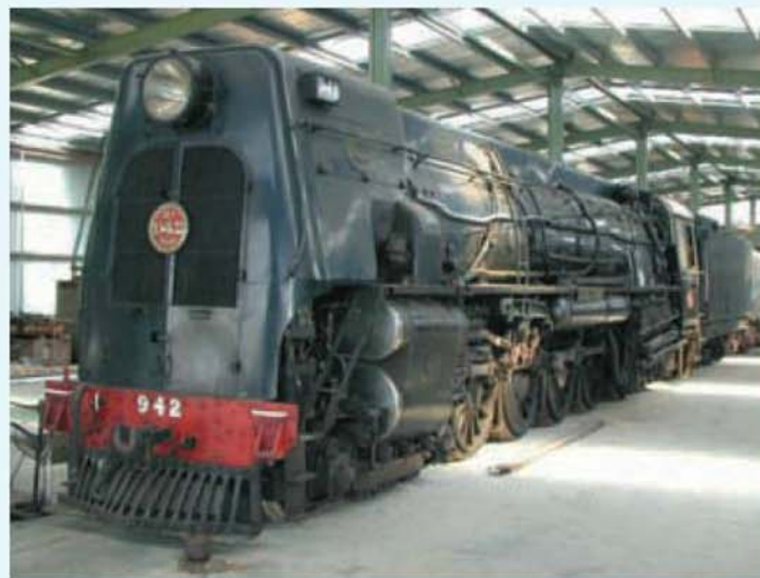
This 'big' engine is a New Zealand Railways Ka class No. 942, 4-8-4 wheel arrangement, built in the NZR Hutt workshops near Wellington.
