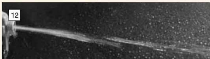
12 This 25psi stream is from an injector which did not work at any pressure. It is no more than a dribble.
