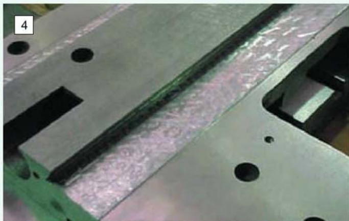
Hand scraped saddle casting for a Super 7 lathe. The distinctive scraper marks are unique to the fitter who made them.
