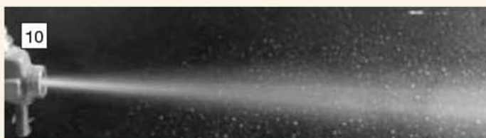
10 At 50psi, the stream is looking better. There is considerable divergence, but this is a good operating stream.
