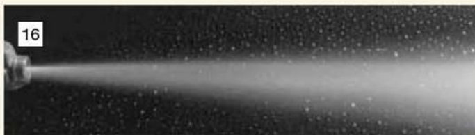
With a proper working injector, the combining cone stream between 120 and 100psi is a mixture of steam and water. The injector still pumps, although there is overflow.
