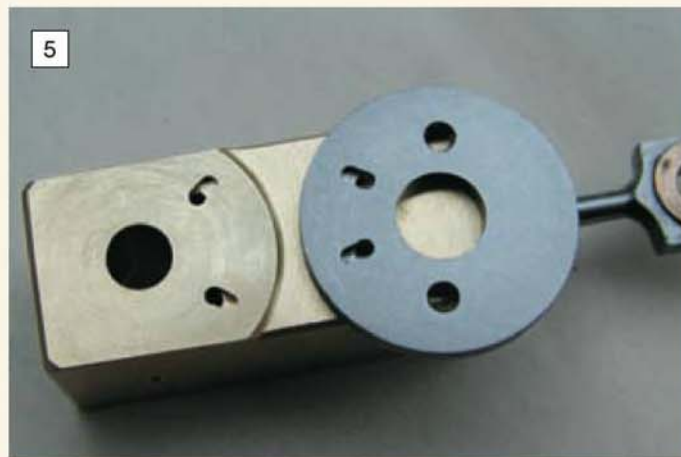
5: End pivoted cylinder with its matching port face disk. The radial port slots described in the text are clearly evident.
