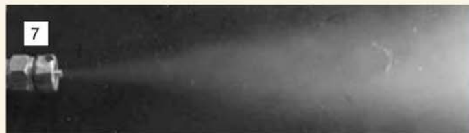
7 After a few seconds, the water starts to clear and the emanating stream of steam still has a good clean form.
