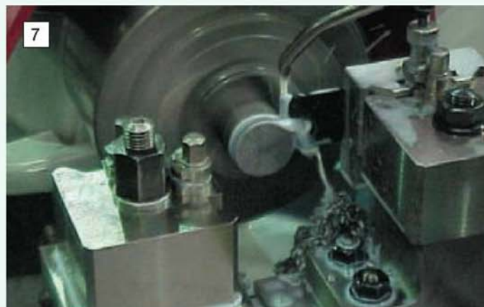
A high speed parting-off demonstration to show the stiffness of the new Myford headstock design and ancillary tooling.
