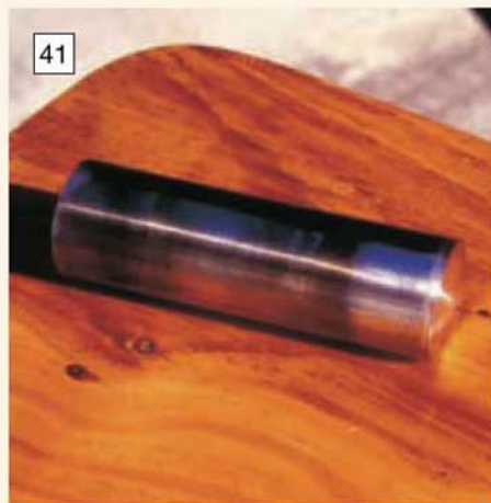
The displacer piston tube with its dished end silver-soldered and trimmed. The displacer end cap received similar treatment but without the need to be reduced to the tube diameter as it didn't obstruct anything and an external silver-soldered fillet could therefore be left in place (see text).
