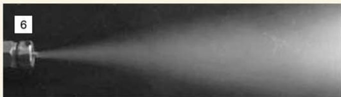
6 The new steam cone in a dummy body shows a good pattern, but with considerable water content when first opened.
