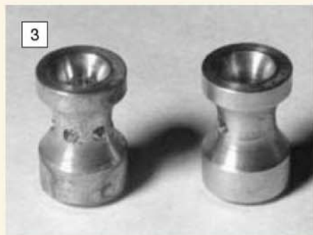
The original combining cone had only one hole. A drilling jig was made and five more of the same size were drilled.
