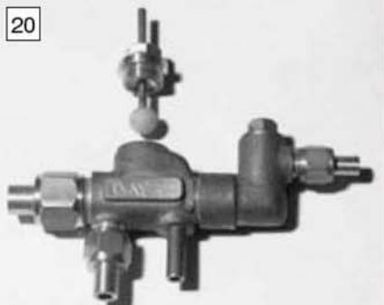
The vacuum around the combining cone was measured with a brass tube pressed into a nylon ball (left). This probe did not interfere with the normal action of the injector. On test (right), the injector behaved just as if it had a steel check valve. The vacuum was measured at 26in. Hg!
