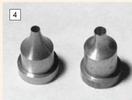
The original steam cone (left) was considerably undersized. The injectors worked with a larger 9deg. cone.
