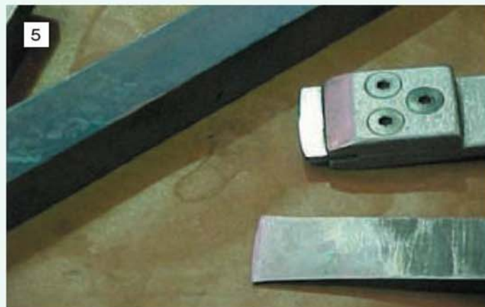
Tools used by Myford machine tool fitters, at the top left is the master surface for checking fit, at bottom right are examples of the scrapers used.
