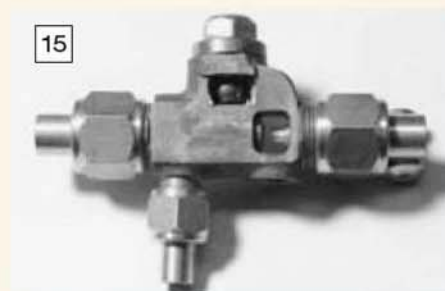
15 Windows were cut in a body to reveal what was happening. It pumped, and the combining cone output could be seen entering the delivery cone, but things were very wet while starting.
