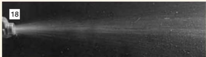
Between 40 and 20psi, the stream is somewhat ragged but the injector is still pumping, although with overflow.
