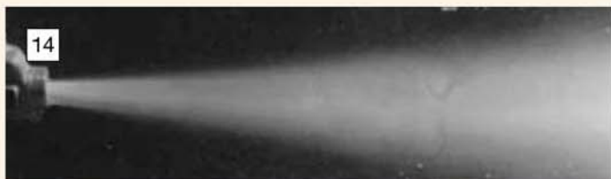
14 At 75psi, this stream would be good for steam cleaning. It is just water and steam from a fire hose.
