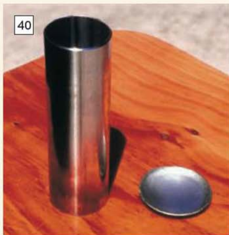
The displacer piston tube with its end cap ready for silver-soldering. The latter was reduced to the tube O/D after silver-soldering so as not to obstruct gas flow in the annular space between the displacer cylinder and piston, this end of the tube was therefore externally chamfered to provide a good fillet of silver-solder (see text).
