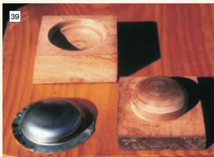
Male and female wooden formers used to press the stainless steel end caps for the displacer cylinder. Squeezing a stainless steel disc between these formers in a vice produced the required curved dish shape, one of which is shown at lower left (see text).
