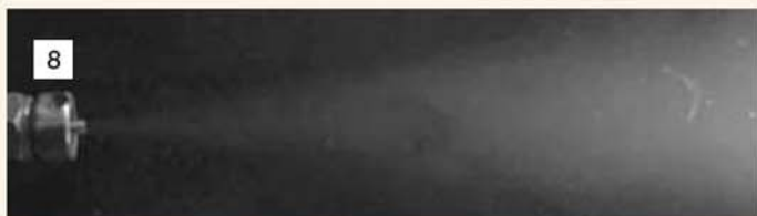
8 After 5 seconds, most of the water is cleared from the jet. Steam lines don't have to be lagged, but it helps to start an injector slowly to clear out water.
