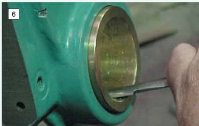
Scraping the bearing bush in a Myford Super 7 headstock to ensure a perfect fit with the front tapered spindle bearing surface.
