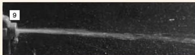
9 With an injector complete except for the delivery cone, the output of the combining cone can be observed. This on a good injector at 25psi.
