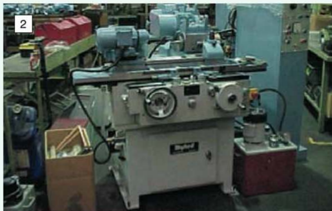
An example of the latest version of the MG12 precision cylindrical grinding machine. Beautifully made and finished.
