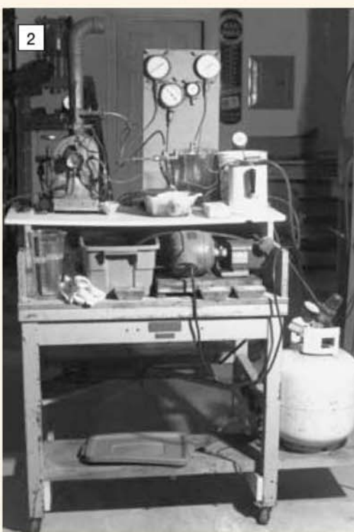
The test stand is on a roller bench and is self-contained. The boiler is propane fired and the feed pump is electrically driven.
