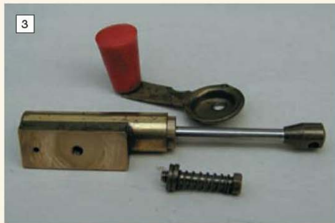
Typical of simple oscillating engine design are these cylinder, pivot and reversing cam from a Mamod traction engine.
