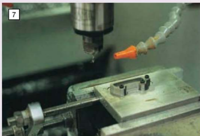
CNC machining a 3in. scale expansion link. Note the stop on the vice to allow the work and sub-table to be mounted and dismantled without losing location. (Photo: B. Camps)
