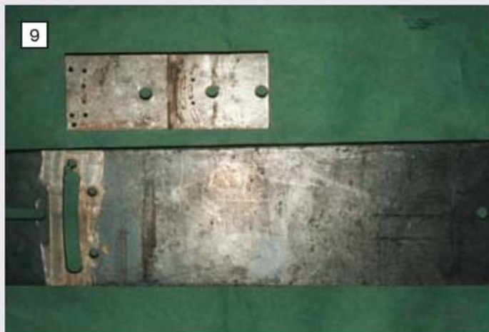
My own jigs for machining the expansion links; these are stored away safely in case the link requires any remedial work in the future.
