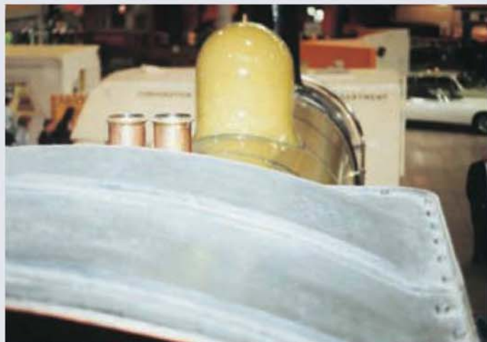
This view of the cab roof of H.R. No. 103 reveals its compound radius form. Painted matt grey, it is bolted to an angle iron surround.
