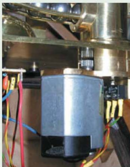
The Buhler 12V motor and its mounting as devised to drive the Archimedes screw and described by the Author for his prototype clock.
