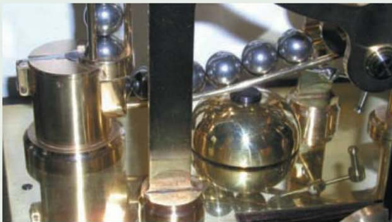
Above: a view of the quarter hour strike mechanism reflected in the highly polished brass base plate of the clock. Note the snug fit of the bell under the track.
