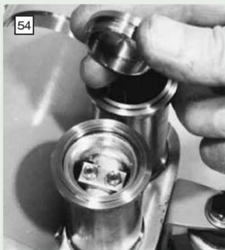
The piston has been attached to its con-rod and the stainless steel cap is about to be fitted.
