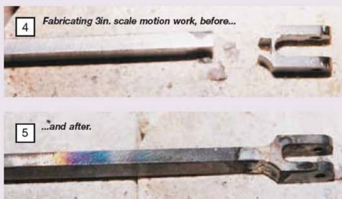
Cutting the forked end of the eccentric rod from the solid, the palm end is to be fabricated. (Photos 4-6: S. Nipper)
