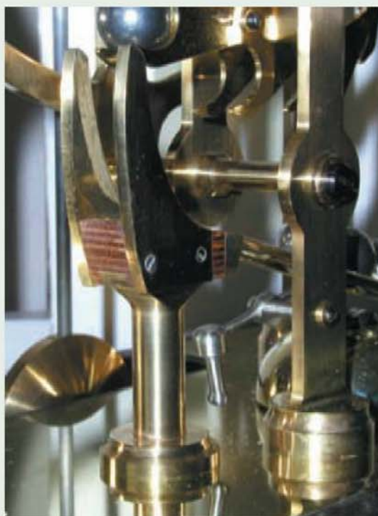
The contact assembly and quarter hour strike mechanism attached to the front time bar.
