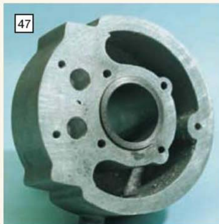
The cylinder liner is fitted into position so that its top is flush with the top of the cylinder block.
