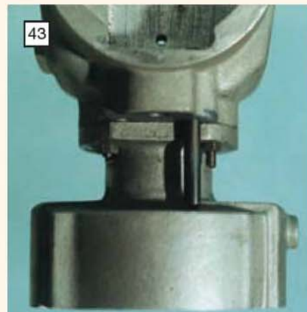
The punch is then pushed right through the tappet hole until it touches the cylinder block.
