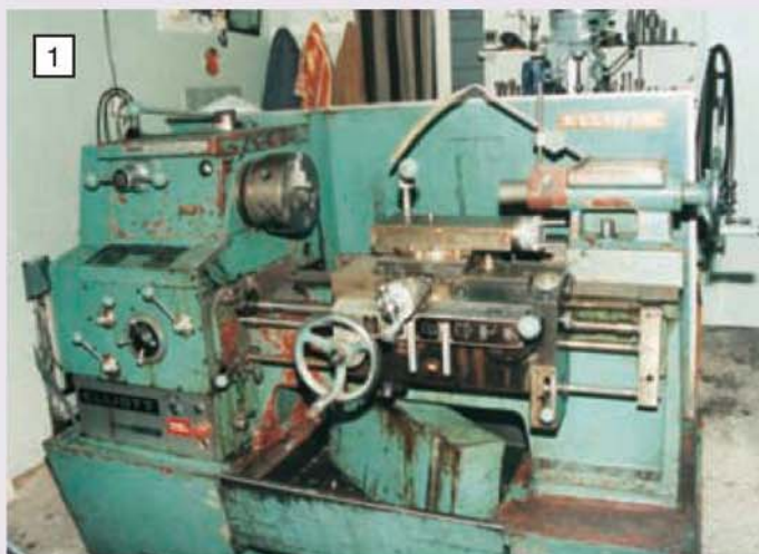
The 15in. swing 'M' series Omni Speed lathe as purchased by the Author. The pumped coolant gear was discarded as was the 3-phase electric, which were replaced by a single-phase motor and switchgear.
