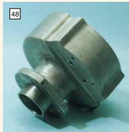
The liner protrudes from the bottom of the block to form a location spigot to fit the crankcase.
