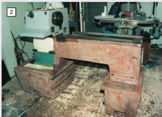
The machine was stripped down as far as possible and cleaned but the headstock drive train was left undisturbed.
