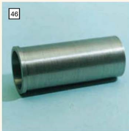
The finished cylinder liner is simply a tube with a flange at one end.
