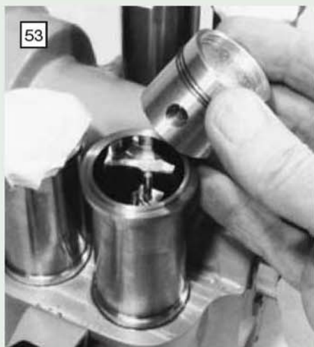
Inserting a finished piston into its cylinder bore; note that it has no top at this stage.
