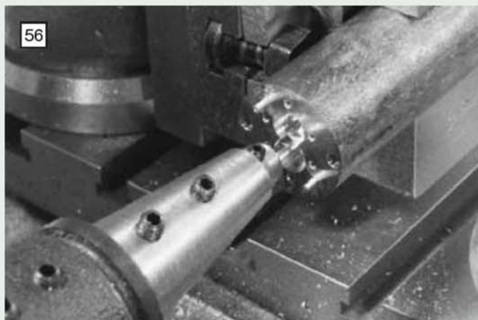
The method used to machine the oil pump. The necessary orifices could be machined using co-ordinates set by the cross-slide and the vertical slide.
