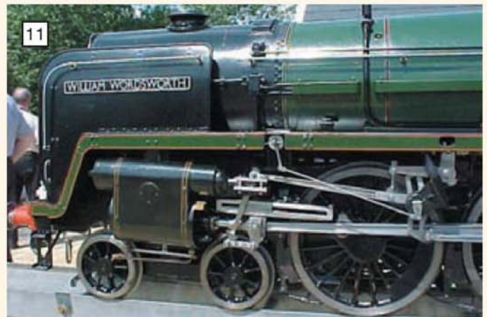
11 The superb motion work and paint finish on John Dalton's Britannia class loco William Wordsworth seen prior to being steamed when its faultless performance matched its appearance.
