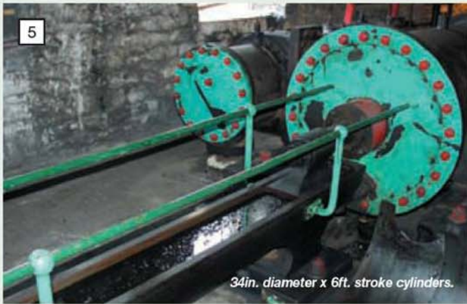
Melling's Patent expansion valve gear.
