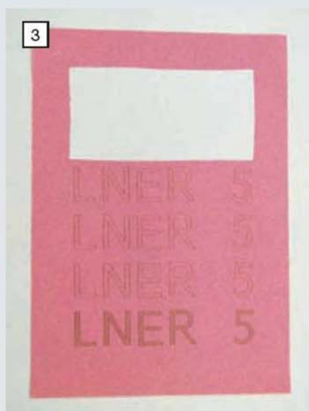
Top: Fig 1 - Artwork for a nameplate, generated on a computer using a CAD program and printed onto adhesive paper.
