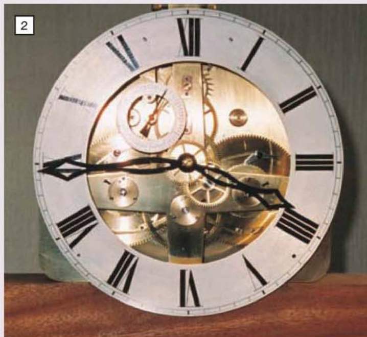
The clock movement removed from its case to reveal the skeletonised front plate through which the motionwork is clearly visible.
