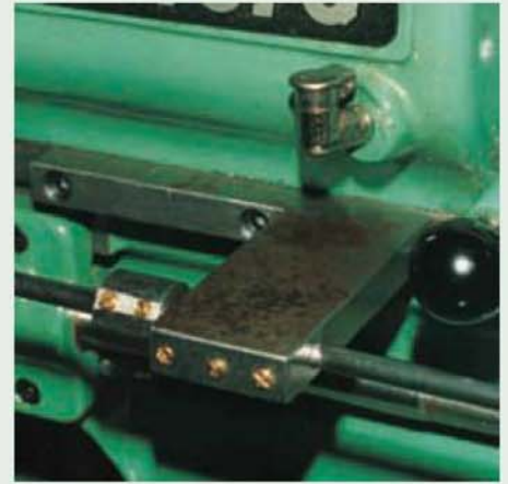
The actuator rod which triggers the release lever is screwed to the front of the lathe, only suitable when no quick-change gearbox is fitted.
