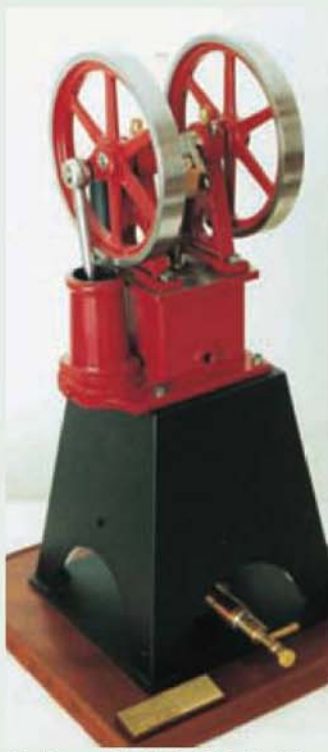
Mr. Norman Barber's Heinrici style hot air engine built without the use of castings.
