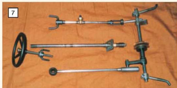
Steering is by worm and half-wheel on a common axle with the rear brakes.
