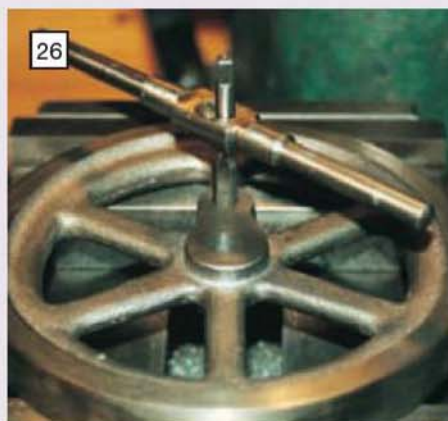
Left: cleaning debris from the \frac{5}{16} in. x 32TPI threaded crankpin hole. A more secure joint results from the choice of this larger thread than the \frac{1}{4} in. BSF specified (see text).
