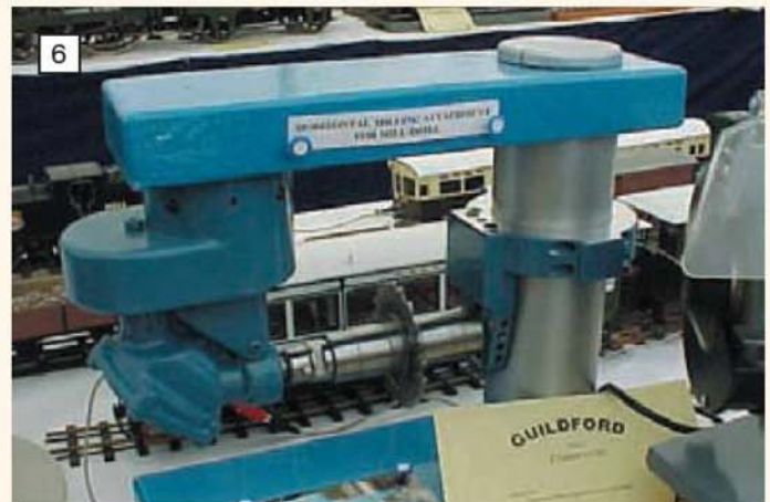
6 The horizontal milling attachment for a vertical mill/drill exhibited by Mr. B. Hatcher showed considerable ingenuity and appeared well made.
