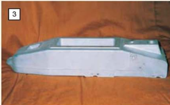
The chassis and crankcase were carved from solid chunk of aluminium alloy.
