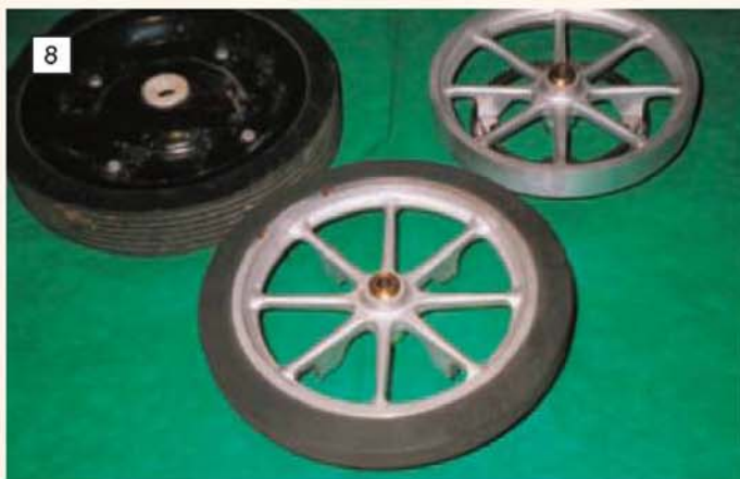
The rubber tyres were cut from old lawnmower wheels (top left).
