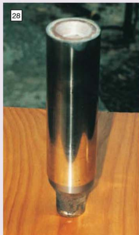
Right: the components shown in photo 27 assembled for silver-soldering the upper cap into the stainless steel tube. The test rod is screwed into the top cap and located in the register hole in the lower insert to provide axial alignment of the thread in the upper cap. Parallelism of this threaded hole with the tube axis was considered to be more important than concentricity. The rolled/seam welded displacer cylinder tube has an internal ridge at the weld and is not truly cylindrical (see text).
