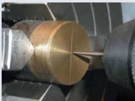
Using a pin to locate the intersection between marked lines aligned with the chuck jaws.
