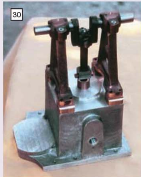
Right: the second part-assembly, with the 'A'-frames on their raisers and the displacer piston connecting rod now clear of the piston rod bush (compare with photo 23, M.E. 4181, 1 November 2002).
