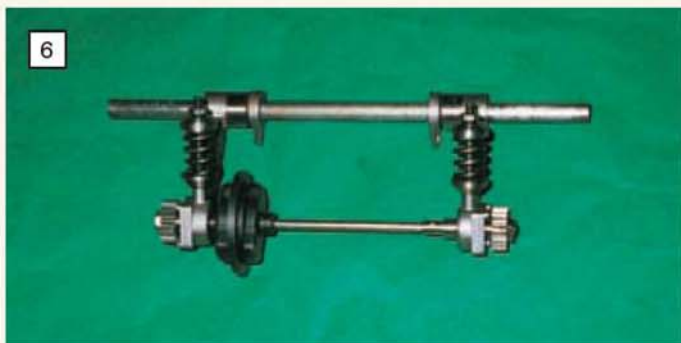
The rear axle with the differential gearbox on the left-hand side.
