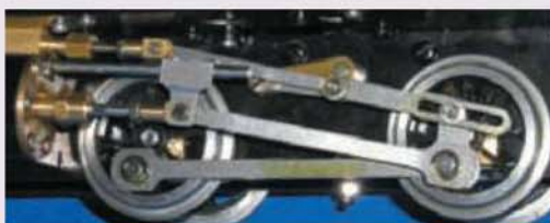
Samson is fitted with a simple but unusual valve gear.
