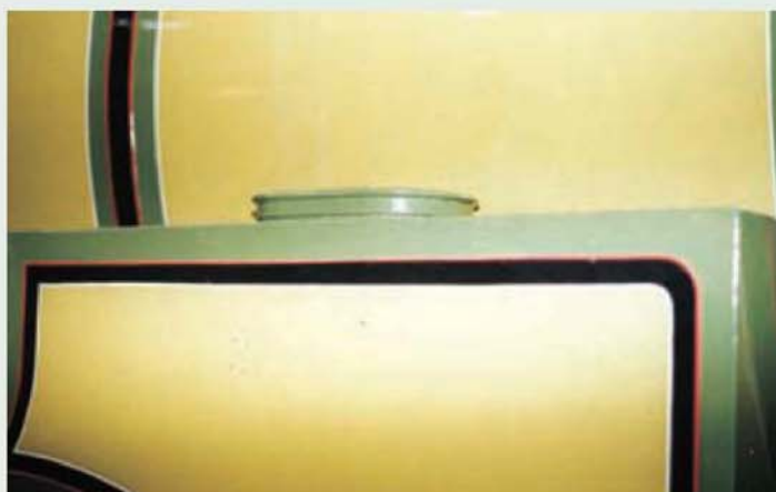
A view of the front splasher of H.R. No. 103 showing the sandbox lid.
