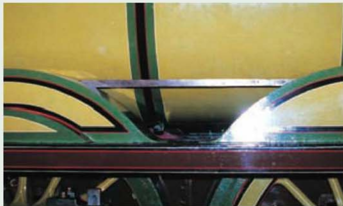
Right hand side of H.R. No. 103. Note the rod for the sanding gear.
