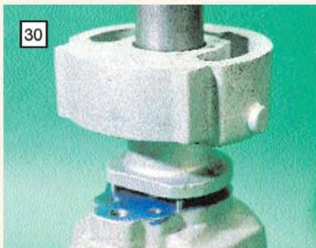
Aligning the cylinder with the crankcase using a length of 1in. dia. steel bar.
