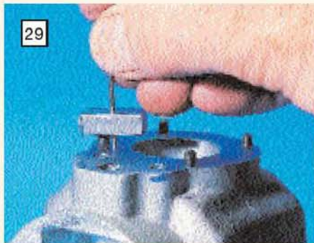
The four punches are all set to the same height and checked with a simple depth gauge.
