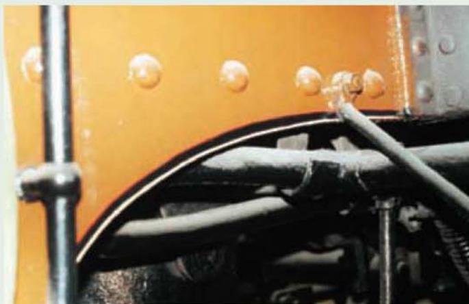
Left hand rear frame of H.R. No. 103 showing the cab steps bracing strut.
