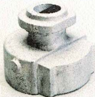
Inverted cylinder casting showing the redundant ring or boss mentioned in the text.
