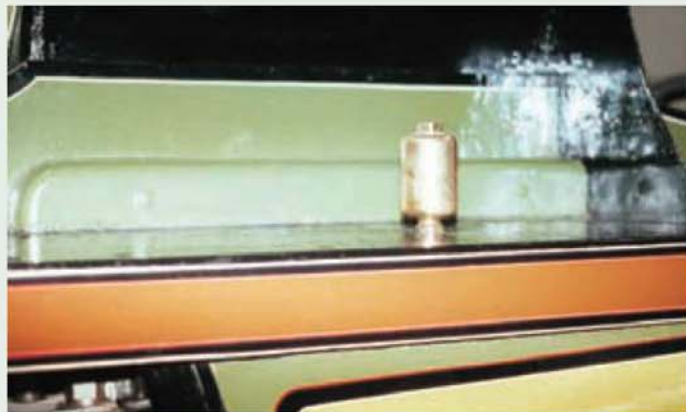
Detail of front platform showing the fairing over the cylinder flange. Note the nearly-flush rivets on H.R. No. 103.
