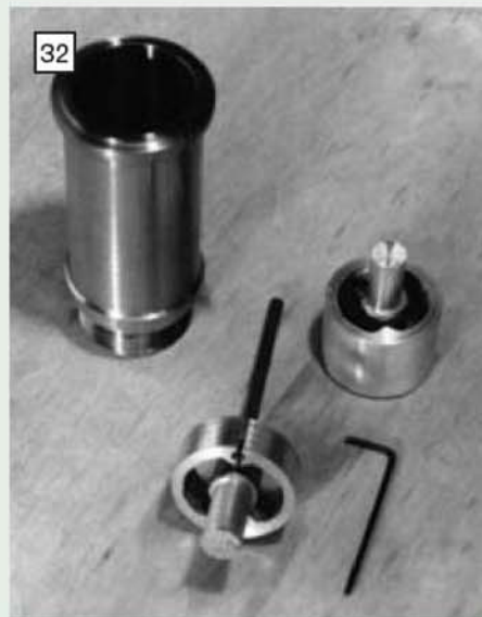
A finished cylinder with the cast aluminium alloy rings used for gauging and lapping purposes.
