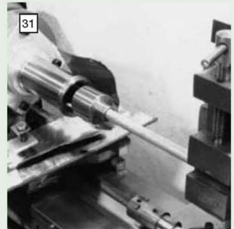
The original lap in use on the lathe before the incident with the dislodged honing stone. The cast aluminium alloy laps proved more serviceable.
