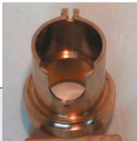
The lifting tube is machined from solid brass, including the hinge lugs, evident in this view.
