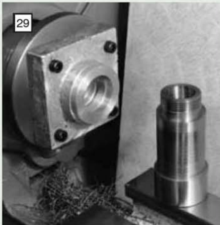
An embryo cylinder roughed out and with the mounting thread turned on the end. This locates in the specially prepared socket on the lathe mandrel.
