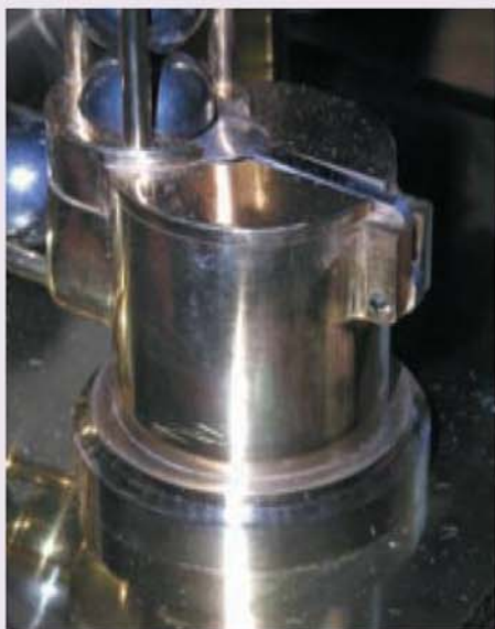
The finished ball lift mechanism showing the lifting tube, cover and entrance bracket. The non-return catch, to be described in a future article in this series, is also shown.
