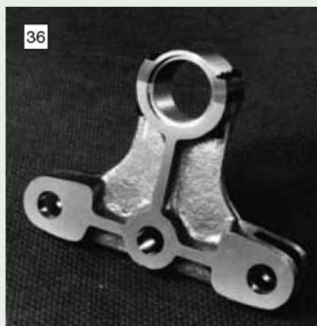
A finished yoke. Note the use of a steel cap, which was chosen to increase the strength of the component in this area.
