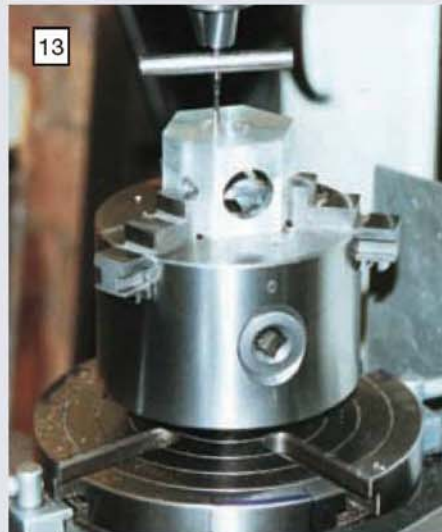
13 The 8BA tap is supported in the drill chuck to ensure it is held perpendicular to the work when tapping for the port flange retaining screws.
