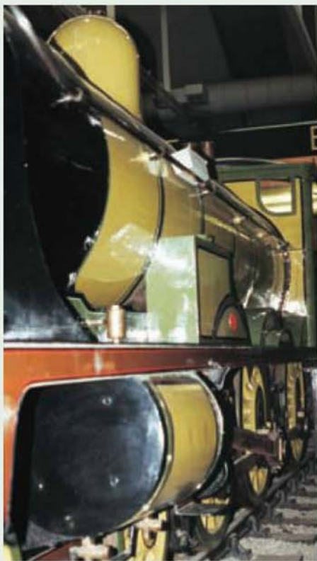
Left hand side view of H.R. No. 103 at Glasgow Museum of Transport. Note the front splash cutaway to accommodate the boiler cladding.
