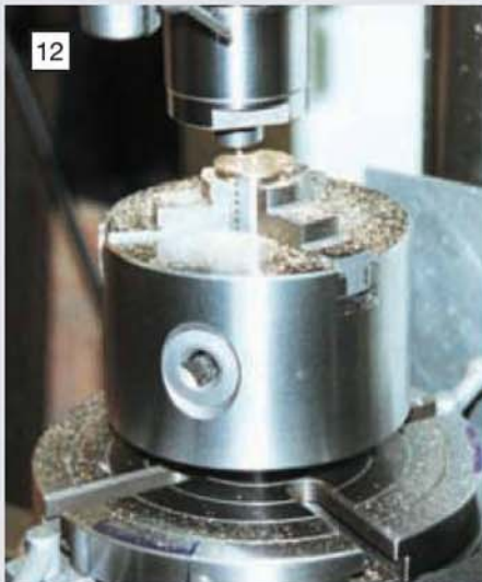
12 Milling the ports in the port flange using the rotary table with the part secured in a 3-jaw chuck.
