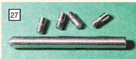
Specially prepared punches are used to transfer hole positions as described in the text.
