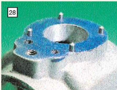
The four hardened silver-steel punches are screwed into the crankcase.
