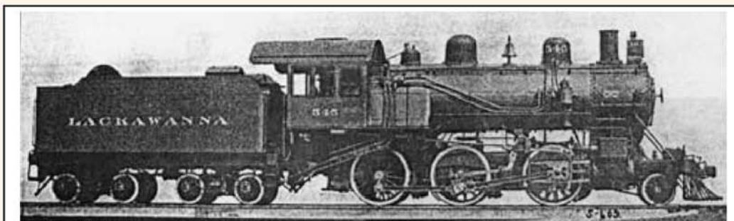
Mogul (2-6-0) Locomotive for Freight Service. Built for the Lackawanna by the American Locomotive Company. Cylinders 20 1/2 in. x 26 in. Steam Pressure 200 lbs. Diameter of Drivers, 63 in. Tractive Effort, 2,948 lb. Heating Surface, Tubes 2,176 sq. ft.; Firebox, 161 sq. ft., Total, 2,337 sq. ft. Grate Area, 53.4 sq. ft. Rigid Wheel Base 15 ft. Total Engine Wheel Base, 23 ft. 10 in. Weight on Drivers, 150,500 lb. Total Weight of Engine 171,500 lb. Fuel, Soft Coal.
