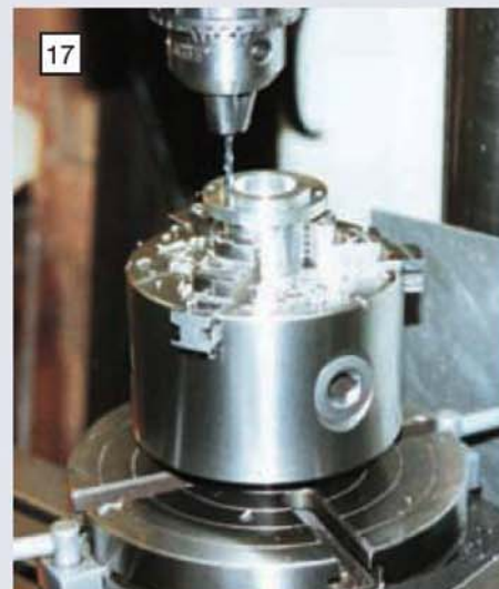
The bearing housing is taken to the milling machine and rotary table for drilling the 6BA clearance holes in the bearing housing flange.
