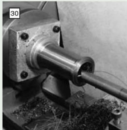
One of the cylinders being bored using a stout boring bar. The fixture ensures that the bore is truly perpendicular to the base of the cylinder.
