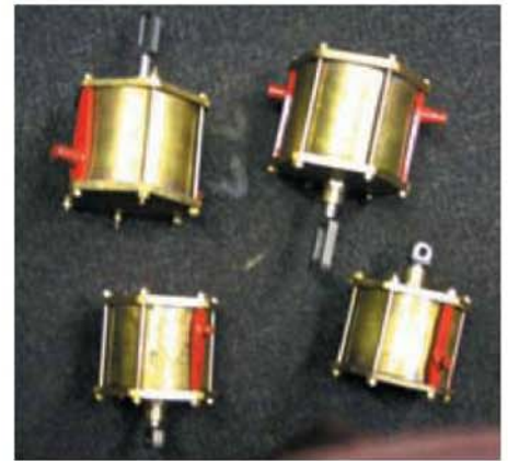
Brake cylinders ready for use. The two at the top are to the 22in. design shown here.
