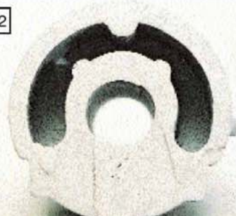
Top view of the cylinder casting showing how the water passages are cast in.
