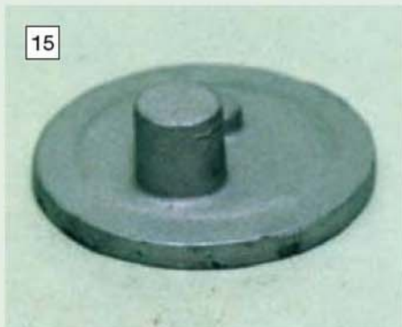
The timing case cover casting showing the extended boss referred to in the text.
