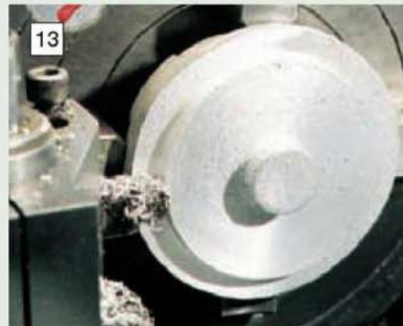
Set up for machining the outer face and bore of the main bearing housing cover.
