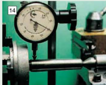
Finding the centre of the bore after reversing the cover in the chuck using a centre and dial gauge.
