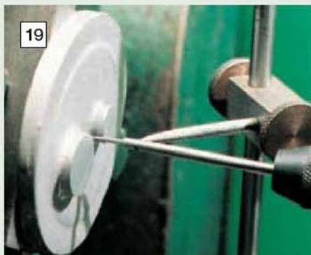
The cover was stuck to a block of steel using double sided tape and the centre picked up.
