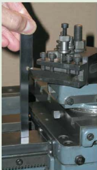
Mr. Paterson's 'minimalistic' tool height setting gauge in use.
