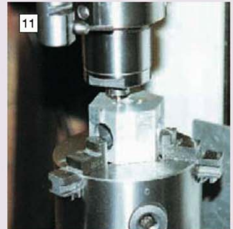
11 Milling the ports in the rear face of the crankcase using the rotary table on the milling machine.
