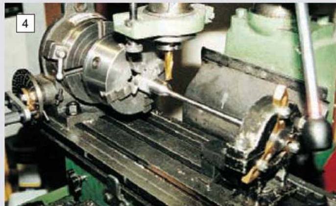
4 Once roughed out, the connecting rod was then mounted in a dividing head, or as here a rotary table 'on edge' to machine the flat surfaces. A Myford fixed steady proved just the thing to serve as a tailstock. (Photo: S. Nipper)
