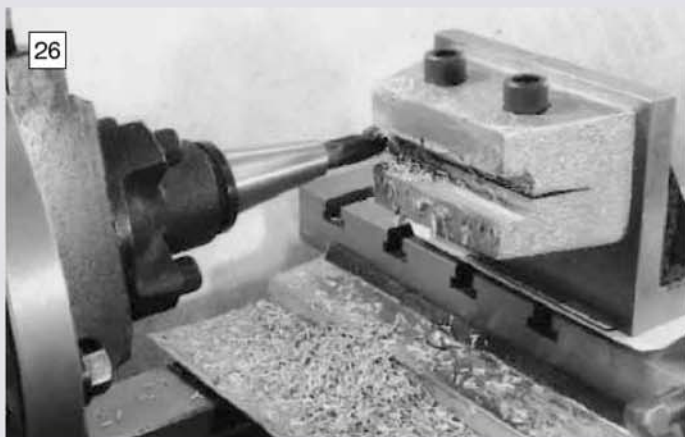
26 Machining the slot in the special aluminium alloy fixture used to hold the slot liners for finish machining.
