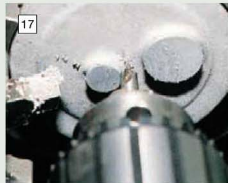
The casting has now been reversed in the chuck and a small centre mark made.
