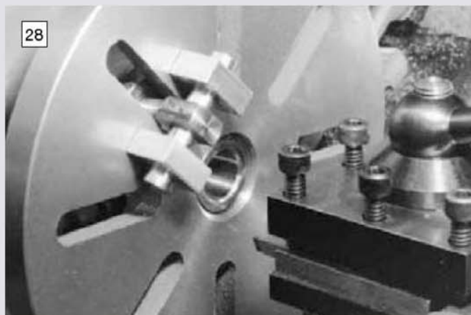
28 Machining the blocks that run in the slot liners using the faceplate. The pair on the opposite side of the faceplate are hidden by the tool post.
