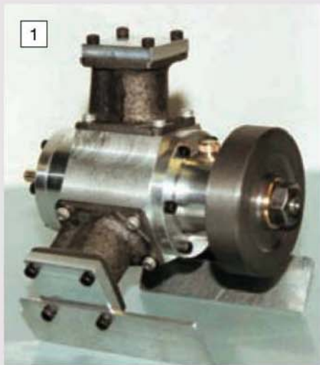
A view of the Author's completed Cygnet Royal steam engine. The three \frac{5}{8} in. bore x \frac{1}{2} in. stroke cylinders of are spaced 120deg. apart around a central crankcase. This configuration makes the engine self-starting.
