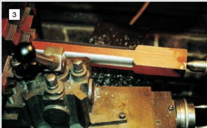
3 John Freeborn machined his 4in. connecting rod from large rectangular stock. EN1A steel is much more difficult to get in rectangular bar form and the intermittent cut must have been unpleasant. (Photo: P. Kybert)
