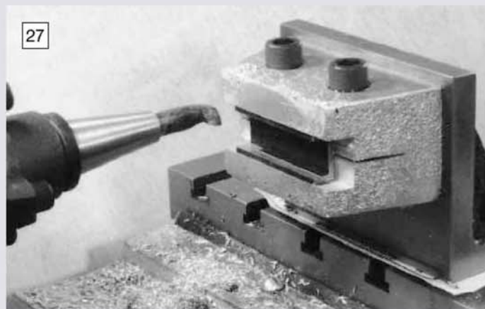
27 Finishing a slot liner gripped in the specially prepared fixture. This device worked well and enabled the parts to be finished without distortion.
