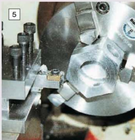
5 The first machining operation on the crankcase. The casting has been fettled and is mounted in the 3-jaw chuck for facing.
