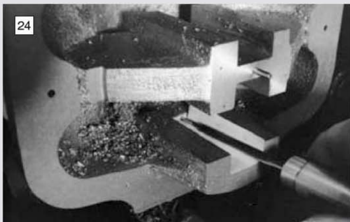
24 Finishing the bottom of the slots with a dental bur. Better attention to casting design would have avoided this by providing a through slot.
