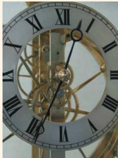
The dial and hands of the clock. The Roman numerals are best engraved mechanically.
