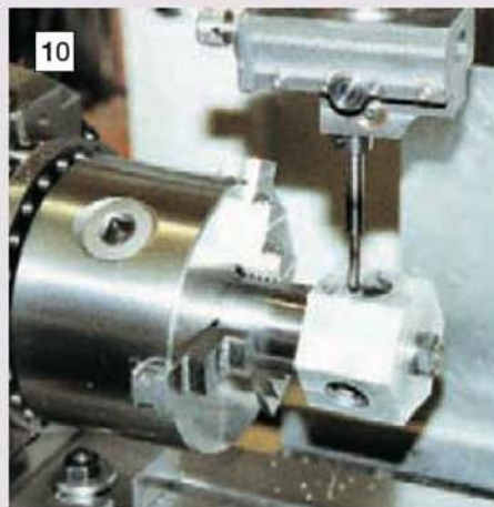
10 While the part is still clamped to the mandrel in the dividing head, the cylinder registers can be machined with an offset boring head.
