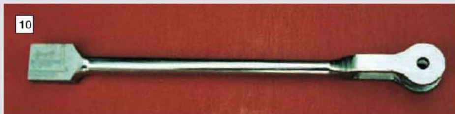
Above: John's connecting rod is now ready for the attachment of the big end strap and bearings. In 4in. scale it is a substantial piece of metal. (Photos 9 & 10: P. Kybert)
