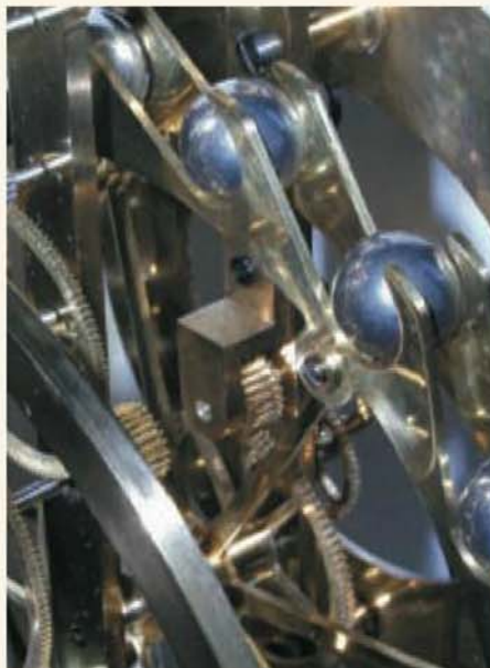
The centre arbor cock in position in the clock together with the respective wheels and pinions.
