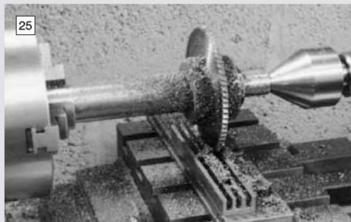
25 Milling the slot liners from gauge plate. This was a nice easy job as it utilised the lathe power cross feed. Table travel is towards the reader.
