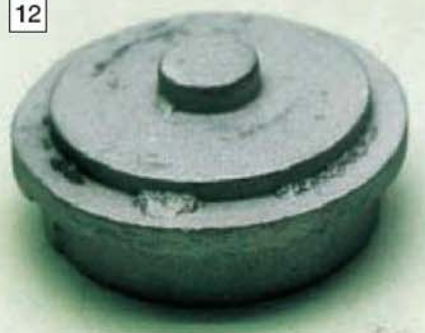
The aluminium alloy casting for the main bearing housing cover was clean and of good quality.
