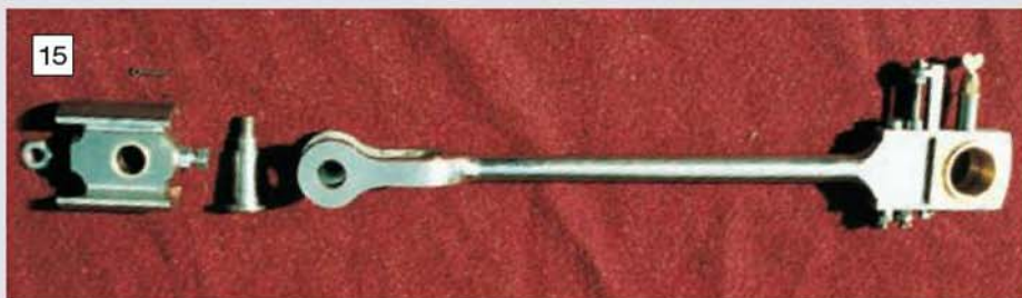
15 A view of John's connecting rod and crosshead. Note that the little end bearing is simply a circular bush which is considerably easier to make and quick to replace if needs be. The little end pin is stepped to prevent the forks being pulled together when the retaining nut is tightened. (Photo: P. Kybert)
