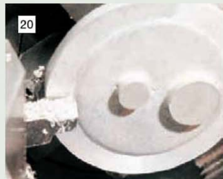
The outer face and edge can now be machined. Cut into the support block to complete the edge.
