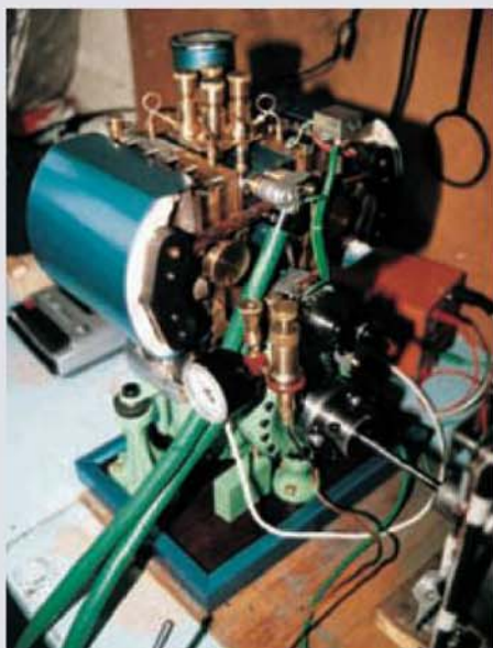
The Author's finished engine on its test bed surrounded by the associated instrumentation.
