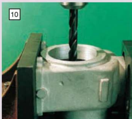
10 After spotting, the three holes were drilled using standard drills which were long enough to reach.
