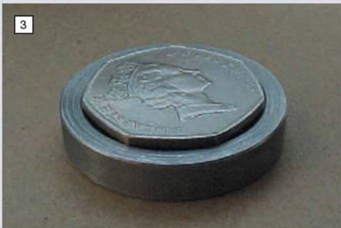
Although the coin is 1.076in. dia. it will not fit in the bore of the ring but rests in the chamfer formed between the bore and the face.
