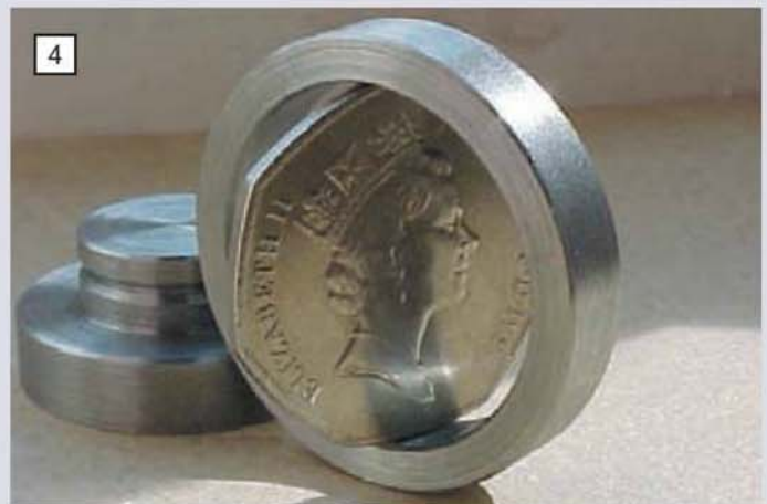
The coin will fit the bore of the ring if inserted in the manner shown. It was actually a snug fit showing that the ring was bored close to nominal size.
