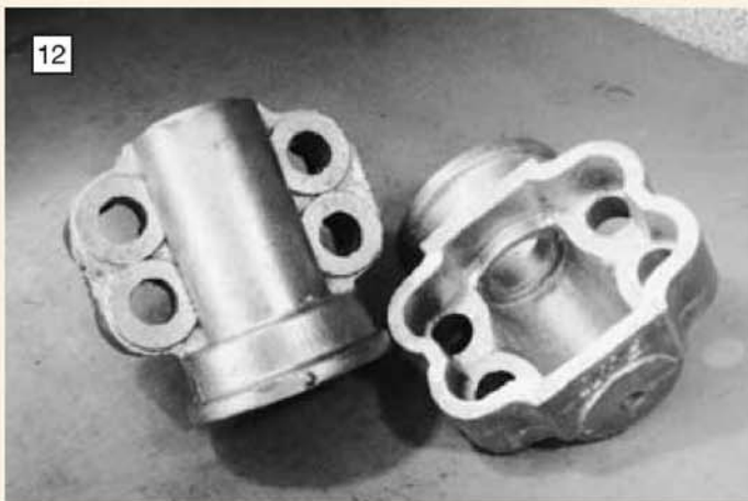
12 The crankcase castings (one to use and one spare) prior to machining and arranged to show the inner and outer surfaces.
