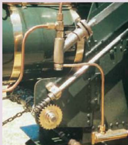
Left hand side detail of the Wallis steam tractor showing the pump and fabricated steering worm.
