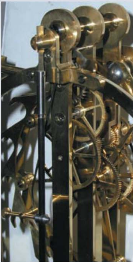
A view of the rear of the clock showing the carbon fibre pendulum rod and pendulum crutch assembly.
