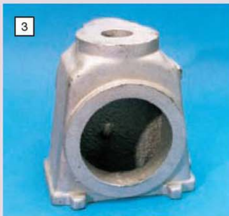
3 A hole on one side of the crankcase gives access to the crankshaft and main bearing.
