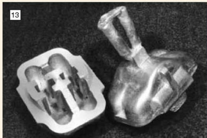
13 The two sump castings. One (left) is showed machined and the spare (right) in the 'as cast' condition. Note the square protrusion for fixturing.
