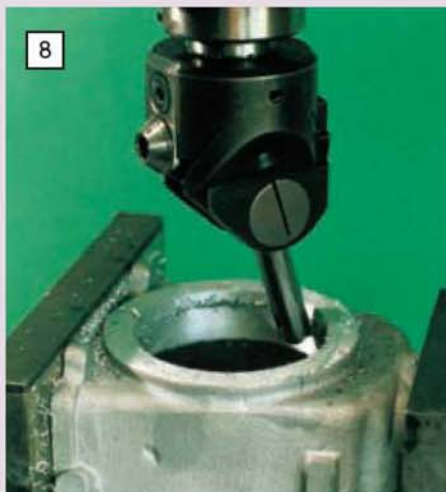
8 The large crankcase access hole was bored with the casting again clamped to an angle plate.
