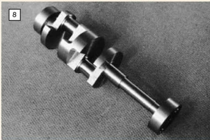
8 The finished crankshaft for the Mk. 2 version of the engine. The chosen material was EN8, a tough steel but one which is easy to machine.
