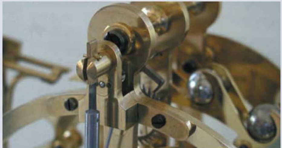
Some of the items referred to in the accompanying text are visible in this photograph. Note particularly the pallet arbor end cap, back cock, pendulum support and pendulum suspension spring.
