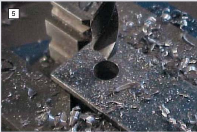
5 A 5/16in. dia. hole has been drilled in a scrap of mild steel bar. It is planned to open up this hole to 1 1/32in. without any special precautions.
