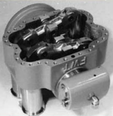
The crankcase assembly shown upside down and in virtually complete form. The protuberance in the foreground is the oil management system casting.
