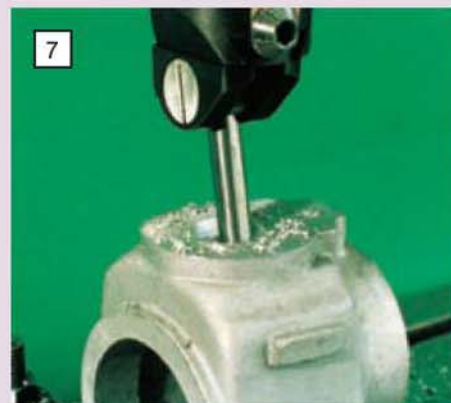
7 Without disturbing the previous set-up, the hole in the crankcase top was then bored.
