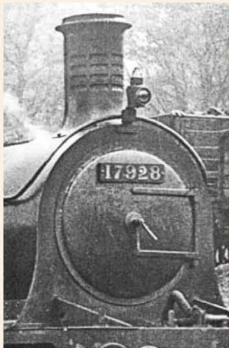
Smokebox door details of HR No. 17928, one of the Jones 'Big Goods' locomotives.
