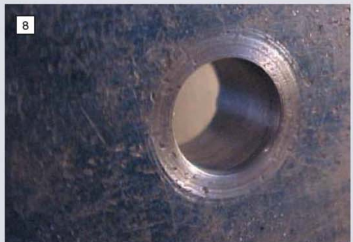
8 The finished 1 1/32in. dia. hole is clean and true without lobes or chatter. The bright ring round the hole is caused by the initial rotation of the emery cloth.
