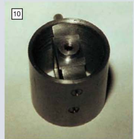
Above: the central crosshead piece is then slid into a tube and secured with a couple of screws ready to be silver-soldered. (Photos 7-10: S. Nipper)
