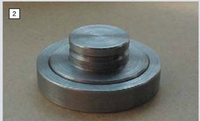
The ring was turned to a snug fit on the plug gauge and is seen here with the plug fitted into its bore.
