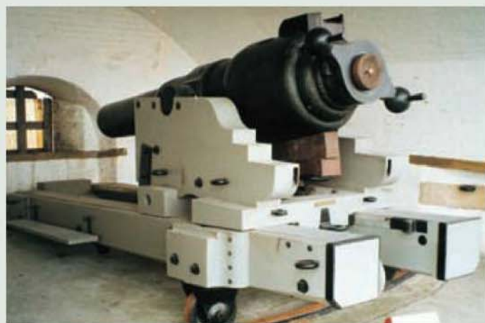
Lieut. Col. D. A. Wilcox based his model 7in. Armstrong RBL on a dwarf traversing platform on this full size version at the Royal Armouries Artillery Museum at Fort Nelson near Fareham in Hampshire.
