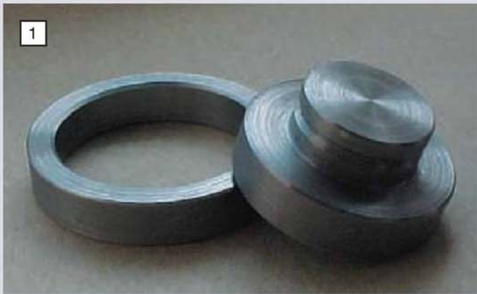
A simple plug gauge and ring were quickly turned up to illustrate the points made in this article. The plug was turned to a diameter of 1.076 inch.
