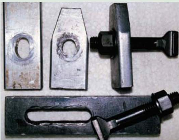
A selection of well used, old and very battered plain 1\frac{1}{2} x \frac{1}{2} in. strap clamps with \frac{1}{2} in. T-bolts.
