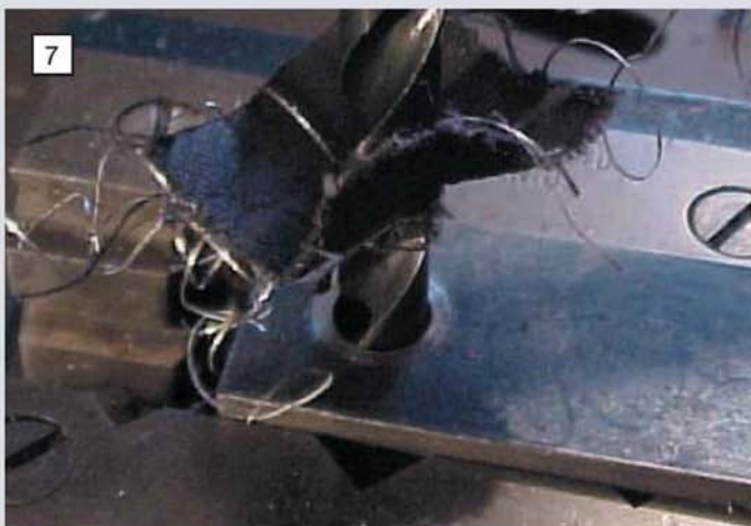
7 The emery cloth starts the drill centrally in the hole and both lips of the drill are cutting evenly. The vice/work is/are clamped before finishing the hole.
