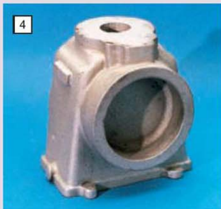
4 A view of the timing side of the crankcase casting. All the castings were of excellent quality.
