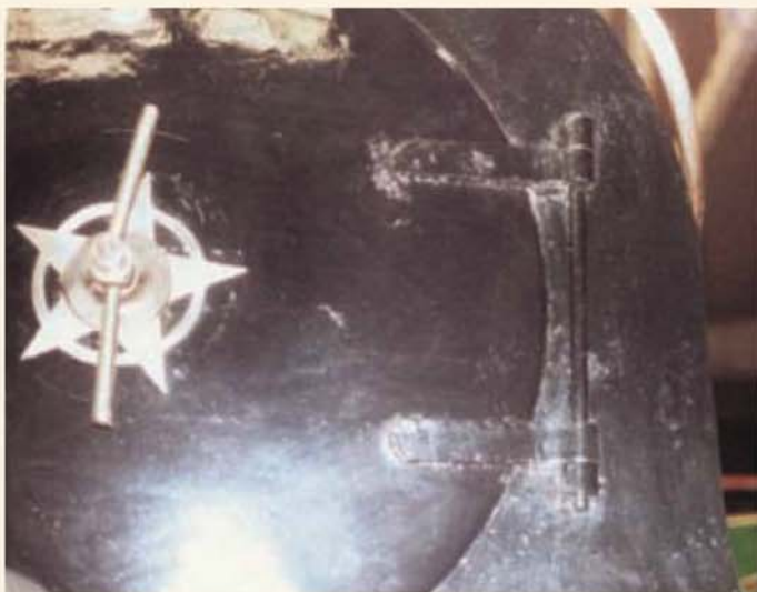
Smokebox door details of HR No. 103, the Jones 'Big Goods' locomotive preserved and on display in Glasgow Museum of Transport & Technology.
