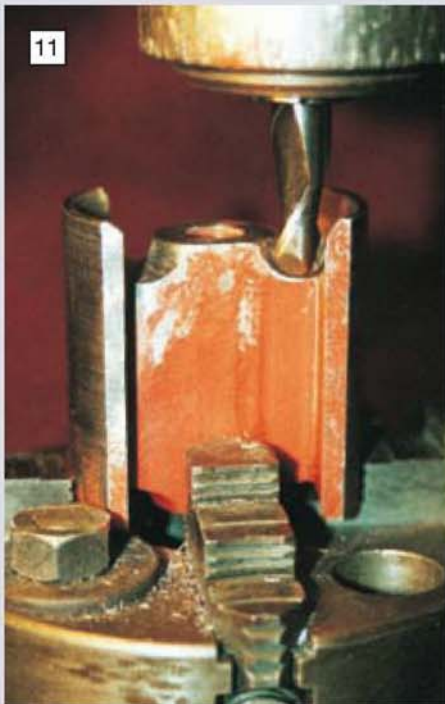
John Freeborn's set-up for cutting the radii in the ends of his 4in. scale crosshead by using a ball nosed cutter and a rotary table. The crosshead was cut from the solid.
