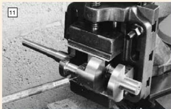
11 Drilling the oil way in the thick central web of the crankshaft at a pre-determined angle on the vertical slide.
