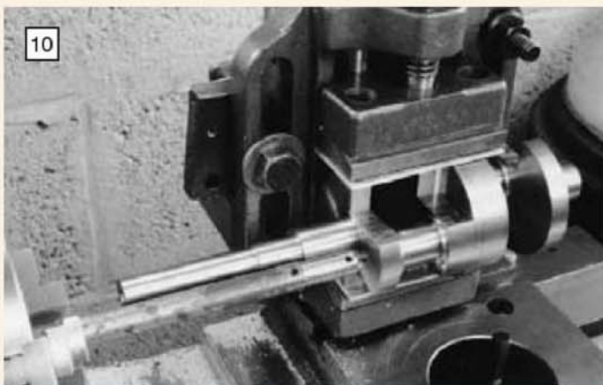
10 Using an extension drill to axially drill the crank pin nearest the drive side of the crankshaft. Redundant holes were plugged with grub screws.
