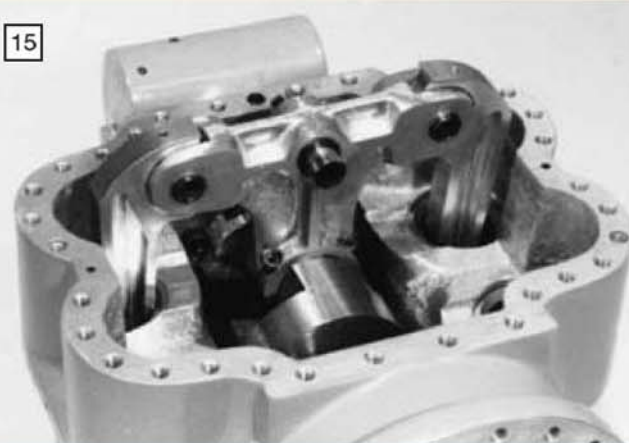
A close up of the big end and yoke assembly. The connecting rod to yoke bearings are hardened steel running in hard bronze bushes.
