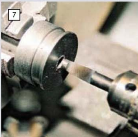
The tapered bore in the piston is formed using a taper reamer. The casting is supplied with a chucking spigot so that the bore and the outside diameter, including the piston ring grooves, may be machined at the same setting.
