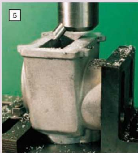
5 The crankcase casting is clamped to an angle plate to machine the base flat by fly-cutting.
