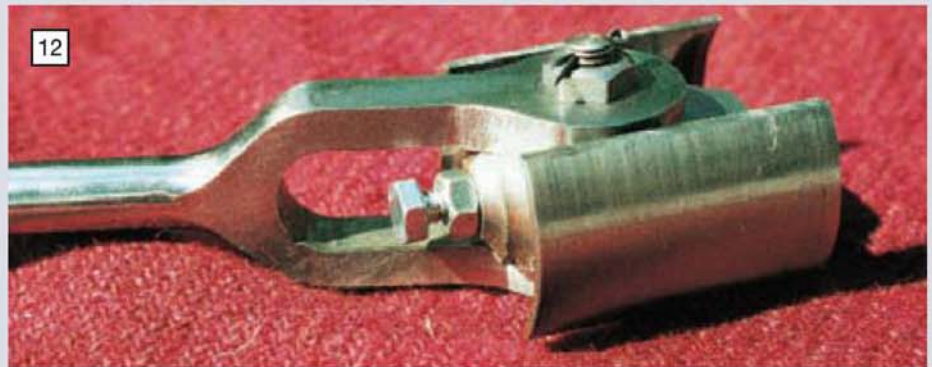
The completed 4in. crosshead is fitted into the connecting rod fork. (Photos 11-12: P. Kybert)
