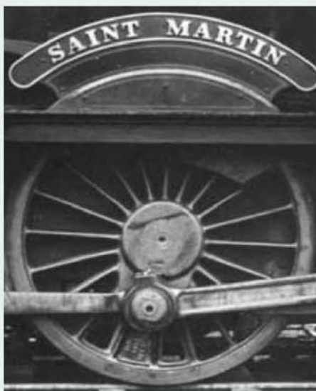
The latest 'Hall' type wheel as fitted to Saint Martin, the prototype for the 'Halls' which was converted from a 'Saint'.
