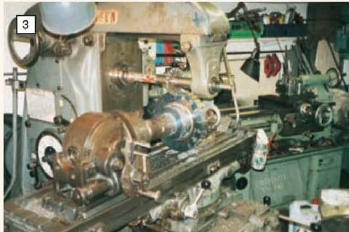
Gear cutting one of the full-size pinions. The cutter is not a form tool but an ordinary side and face cutter. Repeated cuts are taken 'at all points' on the tooth profile until the tooth fits templates of the desired tooth form made in advance. (Photos 1-3: Richard Morgan)
