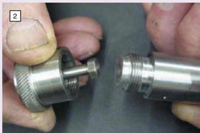
A bolt is inserted into the tool ready for end trimming to length and profile; finger pressure alone on the cap is sufficient to clamp the bolt firmly.
