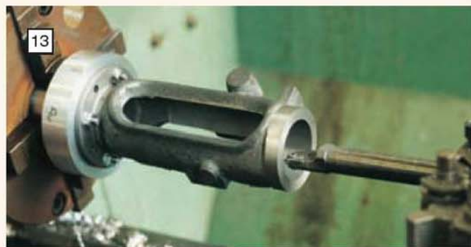
Left: David Hall's 3in. scale trunk guide is mounted in a special collet to guarantee concentricity with the cylinder mounting flange. (Photo: B. Camps)
