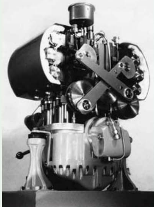
Now in its nineteenth year of development, the Author refers to his hot air engine as a burnt air engine because it runs on air from which the oxygen has been burnt out.
