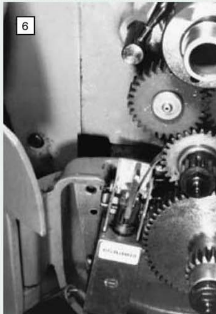
A solenoid indexes a headstock gear to provide the required saw blade feed per cut via the quick change gearbox and cross-slide feed.
