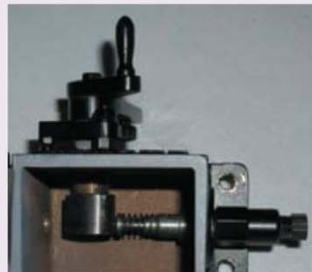
Three views of the Author's high pressure lubricator designed, made and fitted to his 4in. scale McLaren compound road locomotive on which it has worked successfully for some years.
