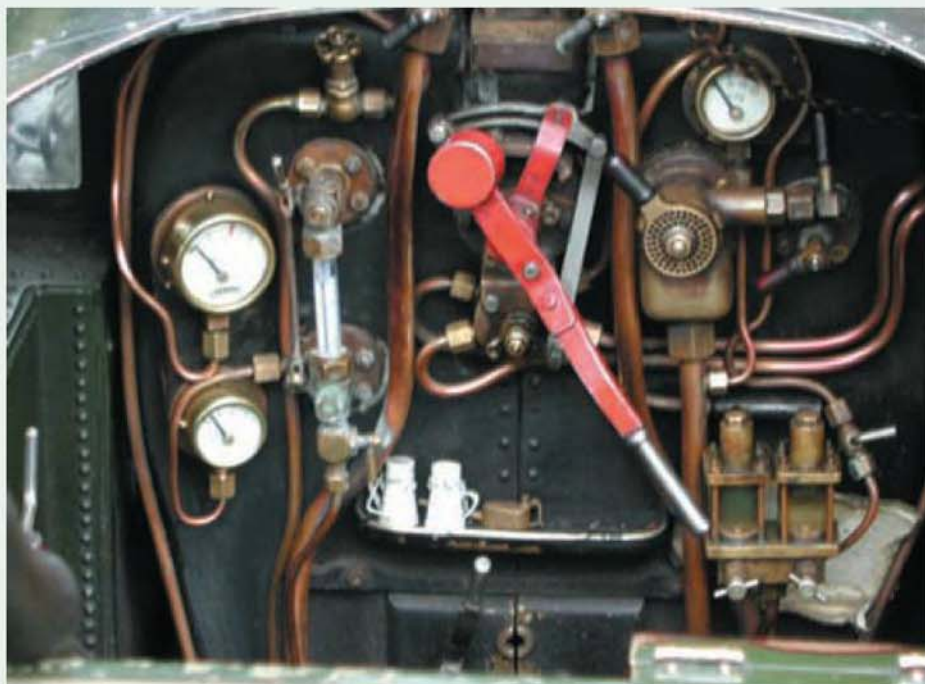
This view of the backhead of Graham Taylor's GW Prairie tank locomotive shows the fittings described in this article and demonstrates that a good looking working backhead is feasible in 7 1 / 4 in. gauge.
