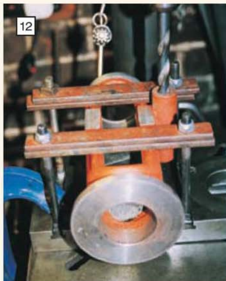
Still safely secured to the cross-slide, the trunk guide has been moved to the drilling machine which had more 'window' than the mill for drilling and reaming the weighshaft hole. (Photos 9-12: P. Kybert)
