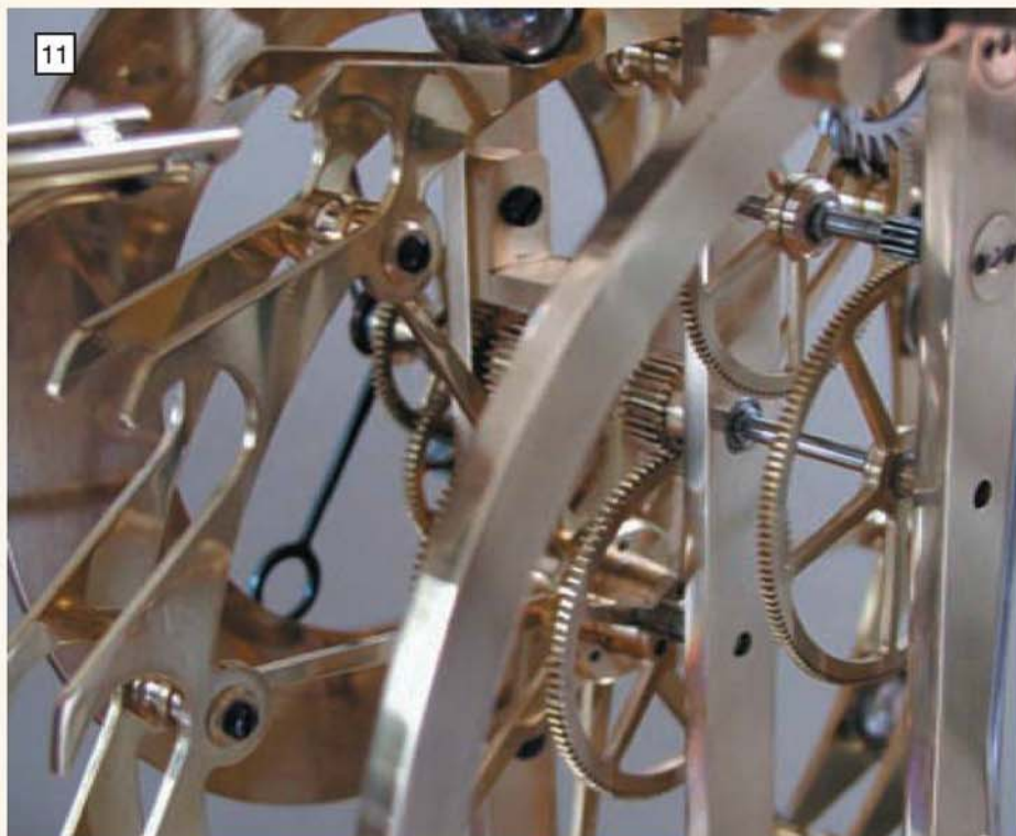
This view shows some of the constructional details of the Ferris wheel clock and the arrangement of the train. Note the method of attachment of the Ferris wheel cages to the spoked support member.
