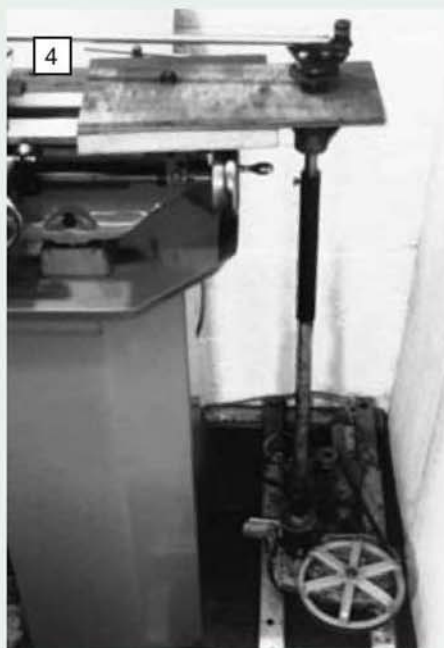
The drive to the hacksaw unit for cutting the heater fins combined parts from a washing machine and a windscren wiper mechanism.
