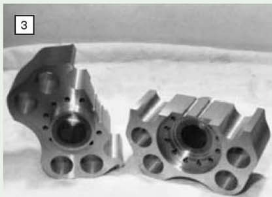
Close scrutiny of this view of the heater castings reveals the finned bores which presented an interesting challenge!
