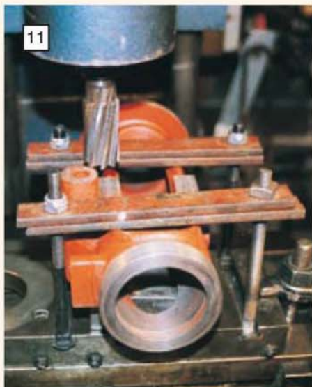
Undisturbed, the trunk guide and cross-slide are mounted on the milling machine table to machine the horizontal surfaces. The cross-slide feed screw assembly has had to be removed so the cross-slide seats properly on the machine table.
