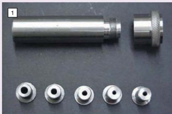
The tool dismantled to show the body, the end cap and five inserts made for different sizes of bolt.
