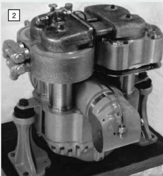
This view of the Mk. I engine shows the oil management housing. The bottom end was used for the Mk. II engine.
