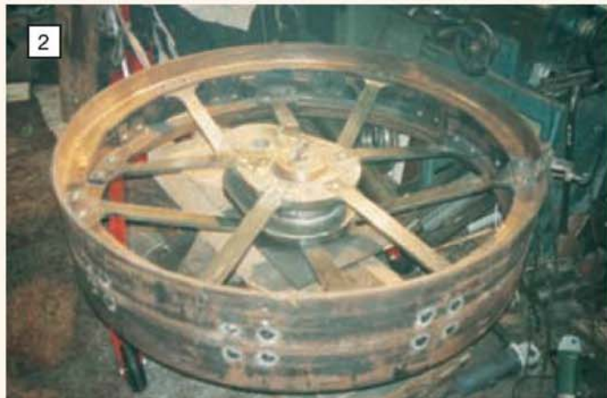
One of the 12in. to the foot back wheels during construction; note that the spokes are welded to the steel hub.
