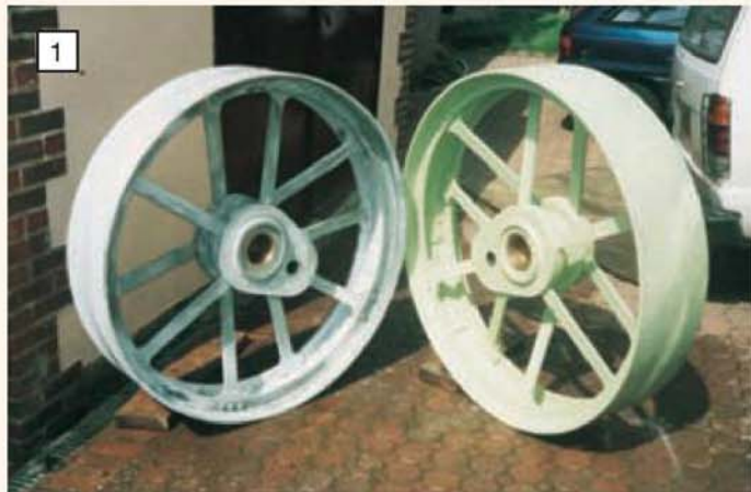
The completed pair of 12in. to the foot Savage Little Samson wheels took twelve months in the manufacture.
