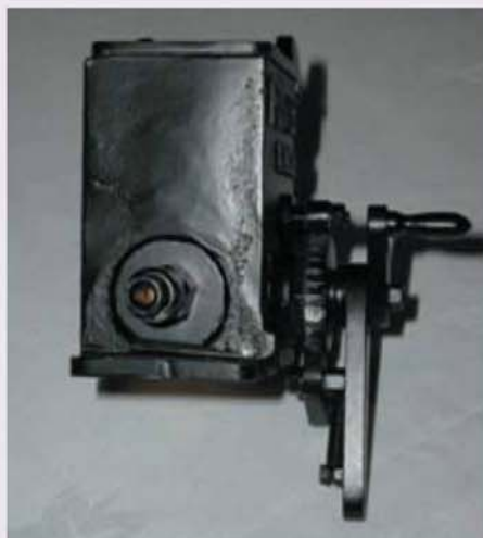
Three views of the Author's high pressure lubricator designed, made and fitted to his 4in. scale McLaren compound road locomotive on which it has worked successfully for some years.
