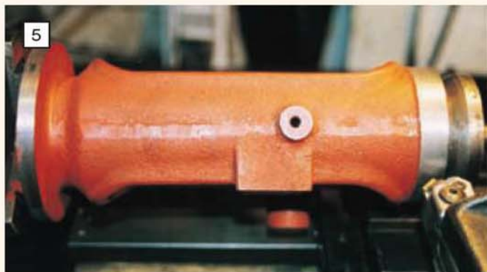
John Freeborne's 4in. scale trunk guide is supported on a cone centre in his Myford lathe. (Photos 5-8: P. Kybert)
