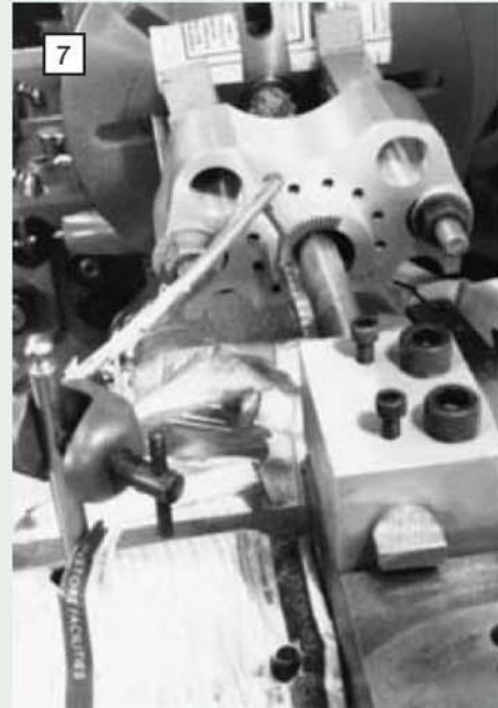
The Author's ingenuity paid off, cutting the fins in the bore of the heater casting is seen here in progress with an air jet to clear the swarf.
