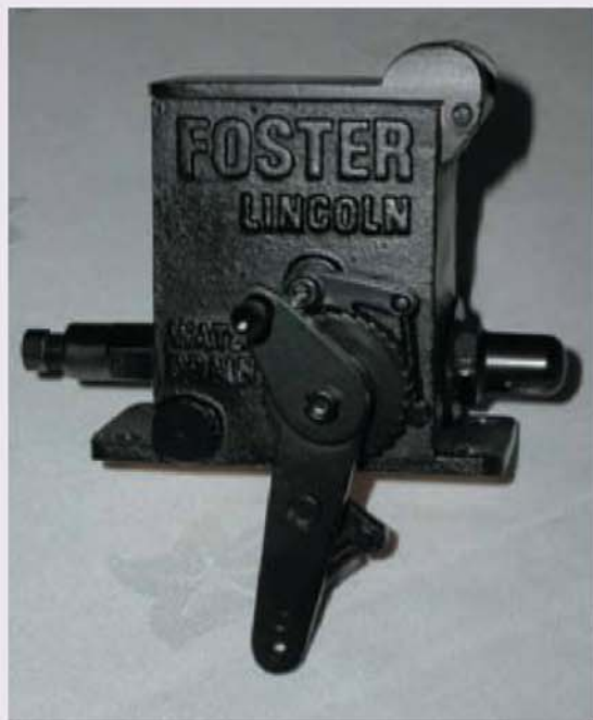
Three views of the Author's high pressure lubricator designed, made and fitted to his 4in. scale McLaren compound road locomotive on which it has worked successfully for some years.
