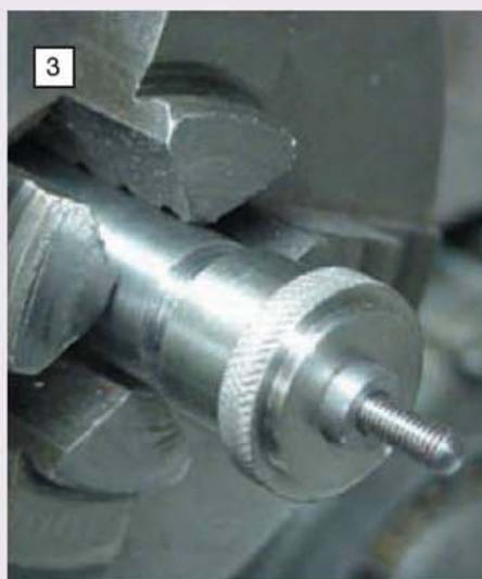
The tool in use. Here the body has been gripped in a self-centring 4-jaw chuck, but any reasonably true running chuck would do.
