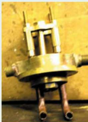
Safety valve and top feed fitting; note the forward facing feed pipes.
