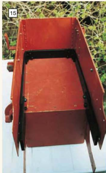
Right: the internals of John Freeborne's 4in. scale tender with his reinforcing straps. (Photo: Peter Kybert)
