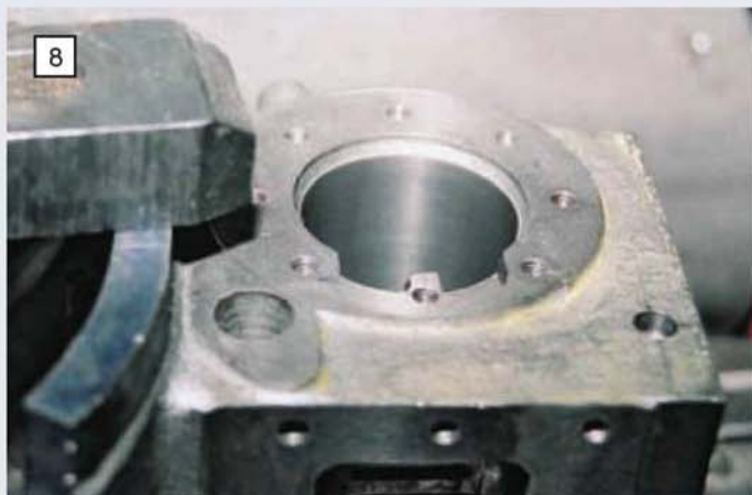
This particular view reveals the quality of the honed cylinder bore and the two recesses for the steam ways with the cover stud hole between. (Photo: S. Nipper)
