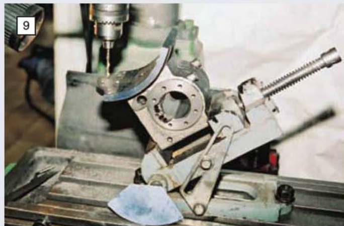
Stan's set-up for drilling the stud holes in the underside of the saddle involves the use of an adjustable angle vice. Note the drilling template resting against the vice. (Photo: S. Nipper)
