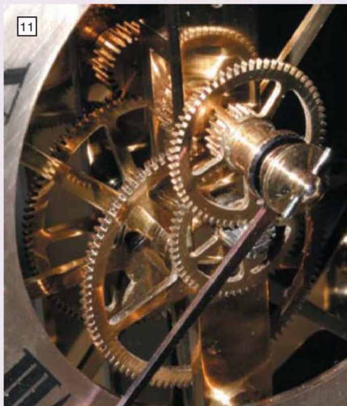
Close scrutiny of the wheels and pinions assembled in the Author's clock reveals the very fine finish obtained on all the individual parts.
