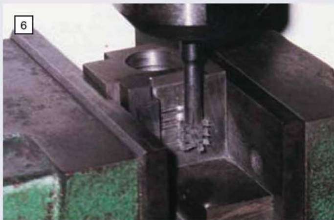
Jonathan's special home-made ganged cutter in use to machine the ports of the cast iron cylinder which has since been discarded in favour of a fabricated bronze cylinder. (Photo: J. Milne-Fowler)
