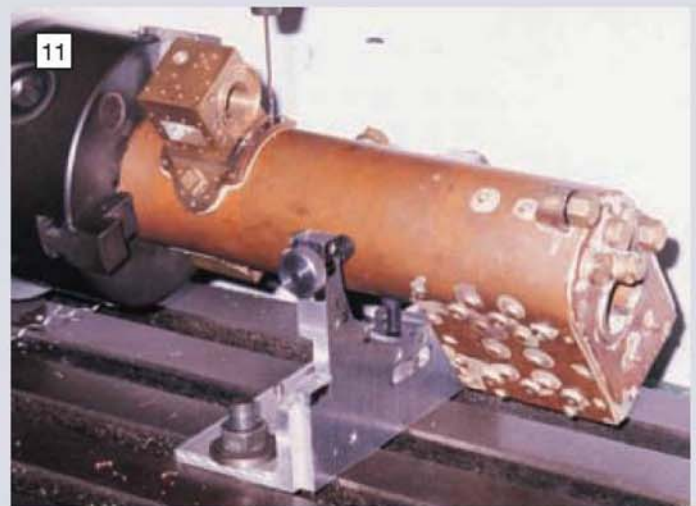
The holes were spotted through to the boiler with the aid of a specially constructed steady. A long series drill was used but an extended drill would have served this purpose as well. (Photo: J. Milne-Fowler)
