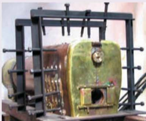
Above: the cladding is an assembly of many separate pieces. Below: assembly is facilitated by the use of a 'gantry'. Right: interlocking lugs retain the backhead cladding.
