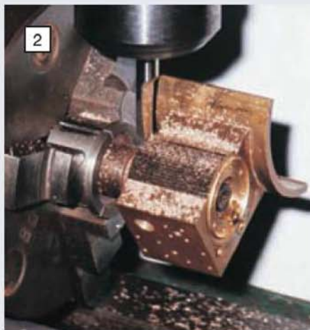
Profiling the 1in. scale cylinder as described in the text to generate a faceted cylindrical surface which can be finished by hand. Note the neatness of the saddle. (Photo: J. Milne-Fowler)
