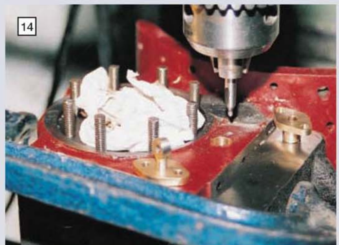
The final operation on the cylinder is drilling the valve spindle hole by jig drilling from the valve rod guide after the trunk guide has been assembled.
