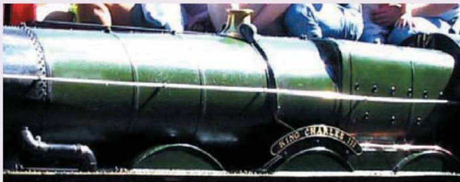
Above: the cladding is an assembly of many separate pieces. Below: assembly is facilitated by the use of a 'gantry'. Right: interlocking lugs retain the backhead cladding.
