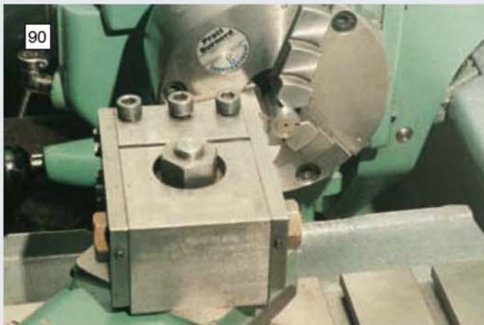
90 Facing off the rollers to thickness. The parts are supported in a fixed bush mounted in the 3-jaw chuck.
