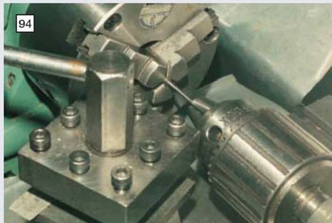
94 The method used to face off the valve rod ends to thickness; the parts are located by a length of \frac{3}{32} in. dia. rod mounted in the drill chuck.
