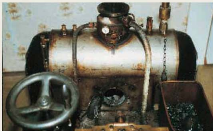
Although externally similar to the original Yorkshire boiler configuration, the casing hides a regular vertical boiler with three cross tubes.
