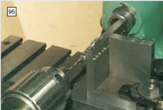
The set-up for drilling and slotting the valve rod ends using a special angle bracket with tailstock support
