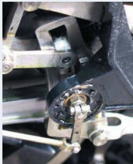
A PTFE die block is fitted to Bob Shaw's Britannia as described in last month's instalment.
