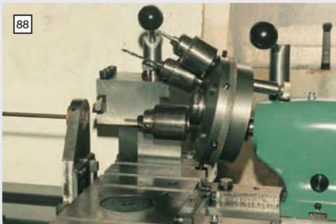
The set-up used by the Author to speed the production of the tappet rods. Note the use of a tailstock turret and the previously described bush steady.
