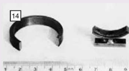
14 The trunk guide (right) was cut from a ring (left) machined to the appropriate dimensions.
