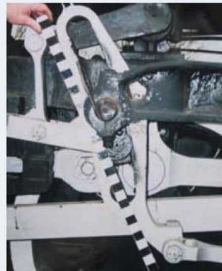
The full size expansion link together with a stick of inches against which to judge dimensions.
