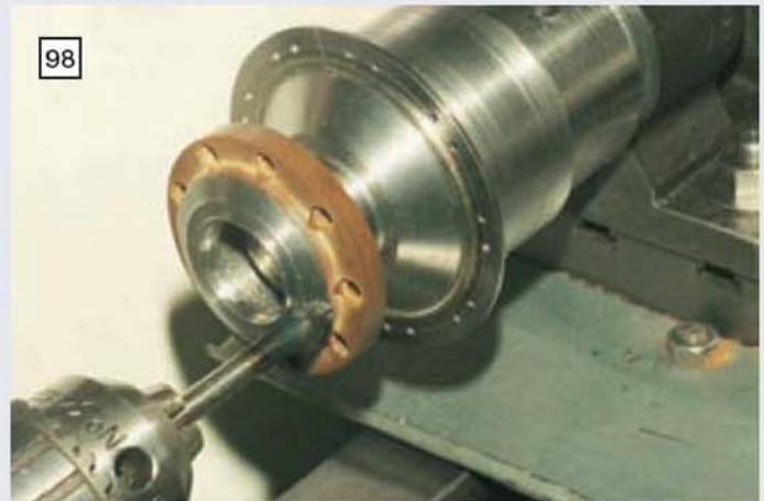
Drilling and boring the commutator ring with the workpiece mounted in the dividing head bolted to the lathe saddle.
