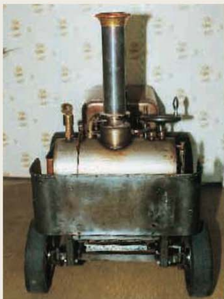
The boiler is a good steamer, a feature which may be due to the internal chimney venturi profile.
