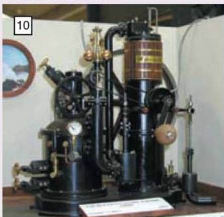
10 Cedric Mell's caloric engine made to the design of Buckett and seen on the SMEE stand.
