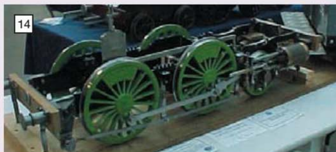
14 Seen on the 7 1 / 4 in. Gauge Society stand was this chassis for a LSWR 2-4-0 WT Beattie tank locomotive by Chris Rayward.
