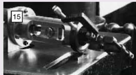
15 The trunk guide bracket is clamped in place to locate the position of the fixing holes.
