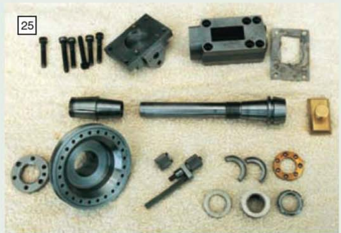
25 Components of new headstock. Top row: dovetailed base, headstock body and shim. Centre row: bearing sleeve, mandrel and cover plate. Bottom row: sleeve nut, pulley, tapered cotter, thrust bearing, spacer ring and lock nut.
