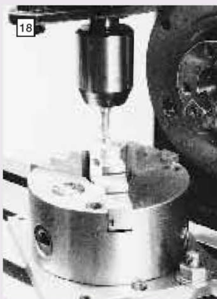
18 The cavity for the connecting rod little end is milled into the crosshead using a slot drill.
