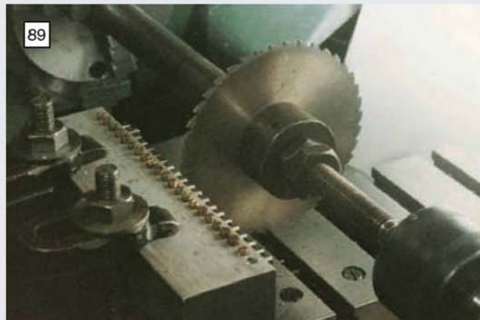
The block used for the relatively heavy slotting operation needed on the tappet rods is much stiffer than an angle plate.
