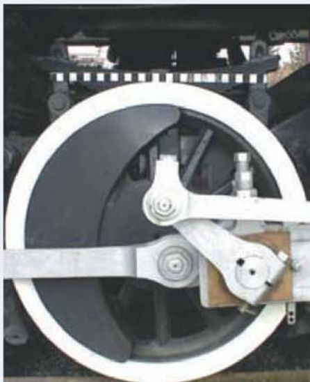
The return crank is keyed and clamped on the full size engine; the key will be omitted in the model.
