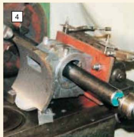
John Freeborne machined his 4in. scale liner bore after machining the saddle as previously described. (Photo: P. Kybert)
