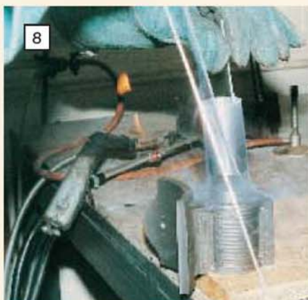
8 The cylinder liner has been immersed in liquid nitrogen at -196deg. C, ready to be dropped into place. Note the protective gloves to guard against dangerous contact with the very cold metal.
