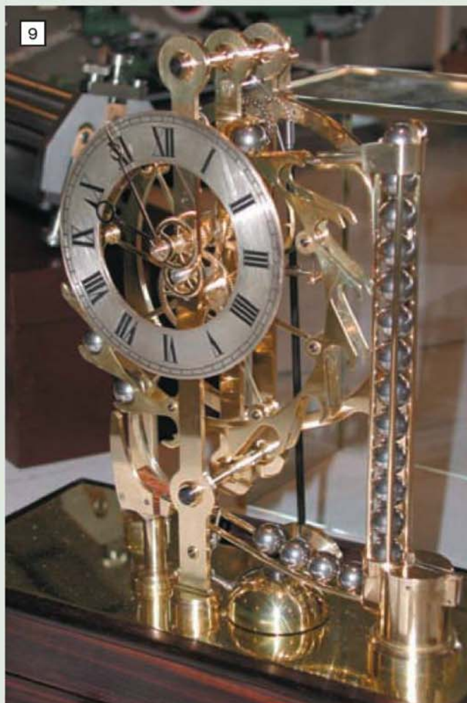
A view of the Author's prototype Ferris Wheel Clock, showing the column of driving balls being lifted to re-enter the Ferris wheel and so drive the mechanism. The three frame members which hold the clock together are also apparent and are described in this article.
