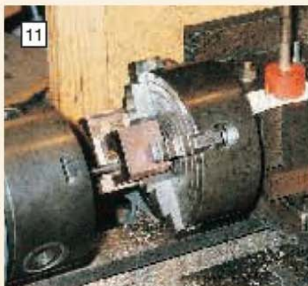
Jonathan's set-up to machine the internal steam uptake in his fabricated 1in. scale cylinder block. (Photo: J. Milne Fowler)
