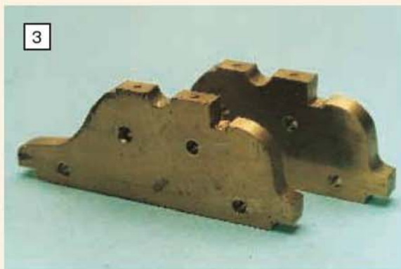
Stan made his frames by soft-soldering 16swg brass sheet together. If you have some spare 1/4in. material to hand, so much the better.
