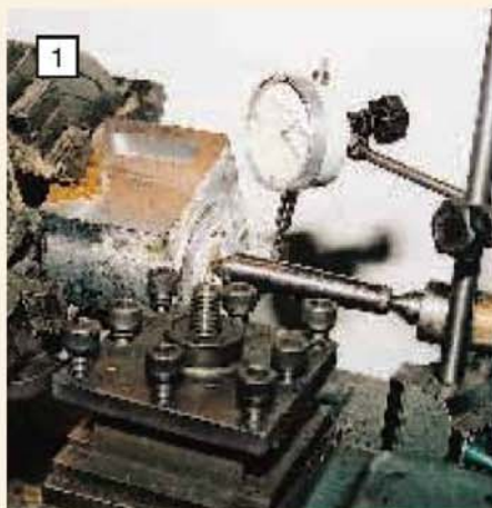
Setting a 3in. scale cylinder casting in the 4-jaw chuck using a 'floating' centre and dti. The casting must also be set square to the chuck.
