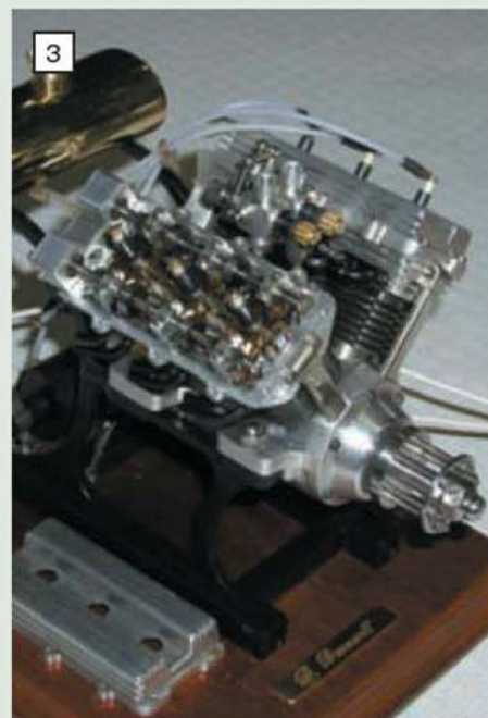
Dave Bramwell had removed a cover from his 18cc V6 aero engine to reveal the valve gear.
