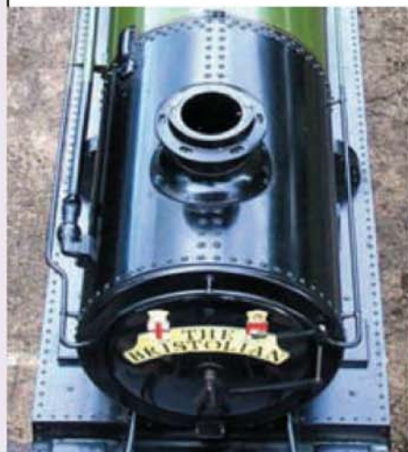
An 'overbridge view' of the 47xx smokebox reveals the longitudinal joint at the top (see text).
