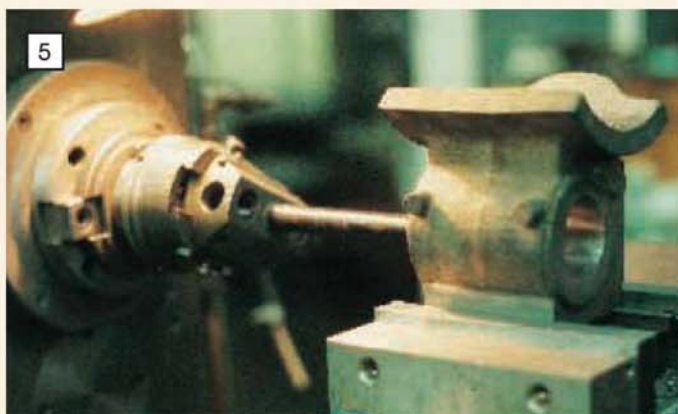
David's 3in. scale Little Samson cylinder was machined on a horizontal milling machine with the aid of a boring head. Note that the tool is relatively slender, limiting progress to light cuts.
