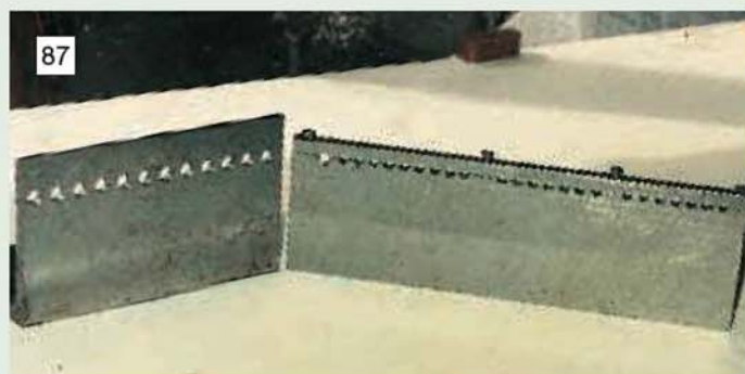
Above: two of the special angle plates used by the author for slotting screw heads and similar work.
