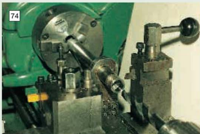
74 The lathe set up for machining the valve cage locking rings. The bush steady is used together with both the front and rear tool posts.
