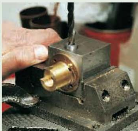
Using fixture 1 to drill the valve bodies. Note that the fixture is held in a vice which is rigidly clamped to the table of the drilling machine - a wise precaution when drilling brass
