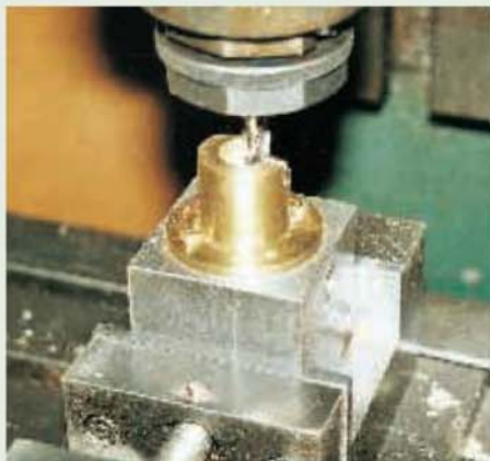
Fixture 1 is also used to hold the valve bodies during milling of the top quadrant which forms the stops for the operating lever. The fixture fits conveniently into the machine vice.
