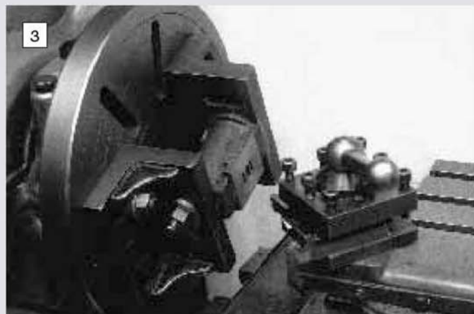
A rigid and balanced set-up for machining the cylinder valve face involves mounting the block between a pair of angle plates bolted to the faceplate.
