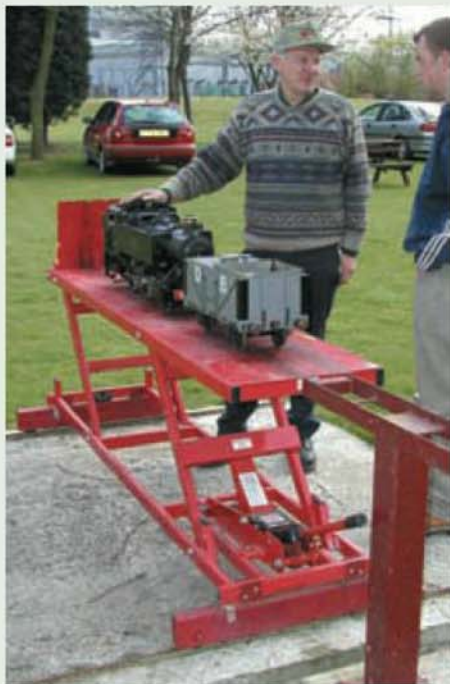
Locomotive handling is facilitated by the club's hydraulic lifting traverser.
