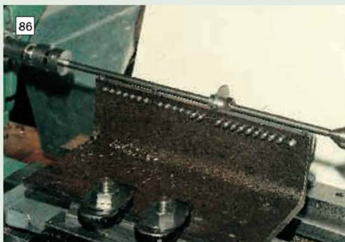
Left: the special angle bracket used to machine the screw slots in the wrist pins. It was made from a piece of angle iron machined on the outer faces.
