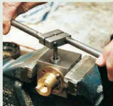
After drilling has been completed fixture 1 can be used as a tapping aid thus ensuring that the threads are automatically cut perpendicular to the surface of the valve body.
