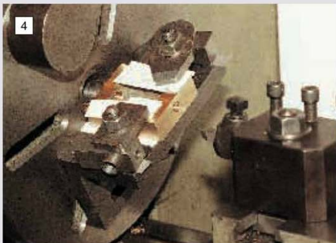
Left: final stages in machining the cylinder valve chest. Note the packing to prevent damage to the clamped surfaces.
