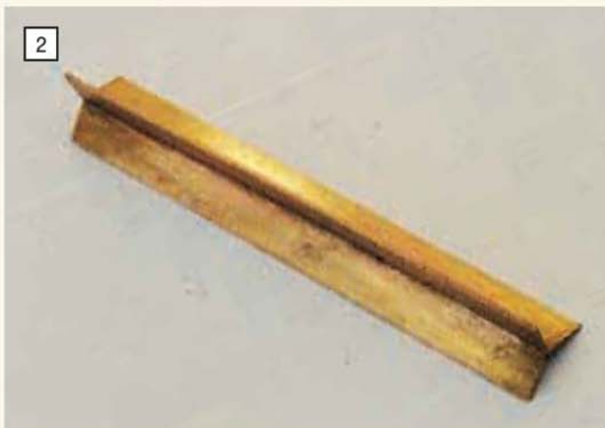
The Spider is shown here after silver-soldering and pickling and ready to be re-mounted between the End Formers for turning between centres.
