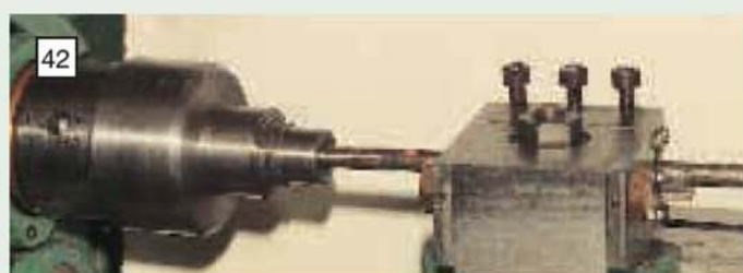
Above right: the cylinders were bored to leave 0.001in. stock on diameter for honing to a finish.
