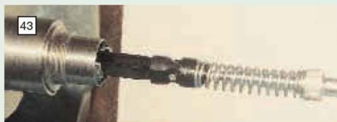
Below right: honing the cylinder bores to size and finish using a hone from Bruce Engineering.
