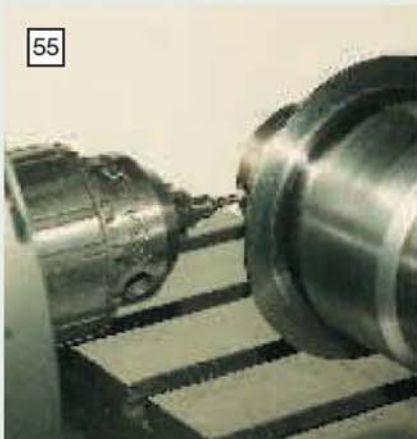
A spindle mounted cutter was used to cut the keyway in the rear ball race housing.
