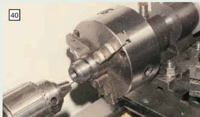
Drilling the vertical transfer ports from the headstock, with the workpiece held in the dividing head mounted on the lathe cross-slide
