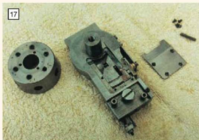
The turret indexing and locking mechanism is concealed beneath a cover plate. The small tappet which is pushed out to engage the stop bar operating lever can be seen on the right hand side.
