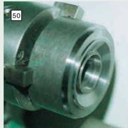
50 Rear ball bearing housing in the crankcase face being machined with the workpiece gripped in a 4-jaw chuck.
