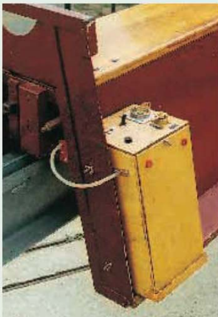
A Frimley Lodge MR pattern vacuum generator unit made by members of Guildford MES. Seen here mounted on a passenger car, its design has been arranged to suit the general lines of the vehicle.
