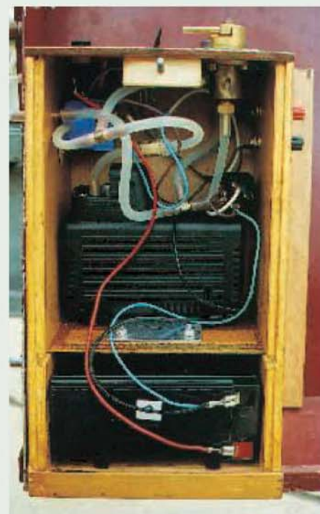
Inside one of the Guildford MES vacuum boxes. This view reveals the battery, pump, valve and pipe work. Individual components can be identified by reference to the drawing (left).
