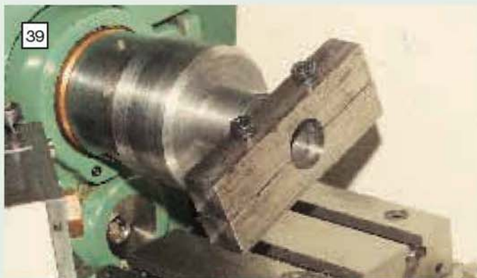
The cylinder removal device, designed to assist with the removal of tight cylinders from the master and slave chuck.
