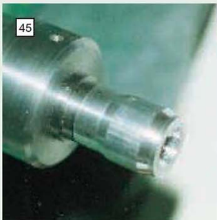
45 Stage two in machining the cylinder heads; here the outside profile is receiving attention.
