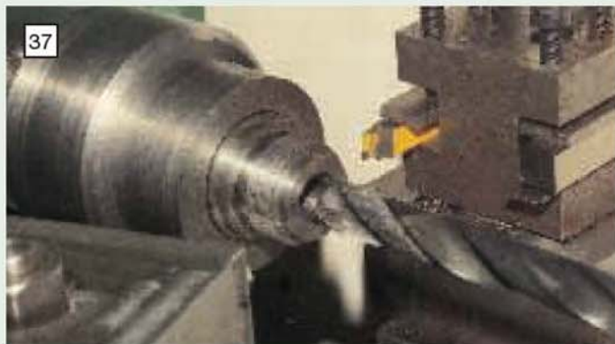
The lower part of the cylinder liners is machined using a knife tool in the main (front) tool post, a screwcutting tool and a parting-off tool in the indexing rear tool post and a drill in the tailstock.
