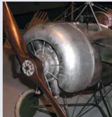
John Siddall's 1:4 scale flying model represented a 1916 Fokker AIII of the Austro-Hungarian Air Service. Radio controlled and powered by a Laser 180V engine, the Flair engine cowling shielded a dummy 9-cylinder rotary engine.
