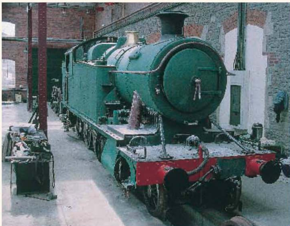
2-8-0T locomotive No. 4247 nears the completion of its restoration at Swindon Works which is part of the Steam Museum.
