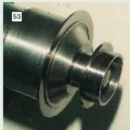
Rear ball race housing with all turning work completed
