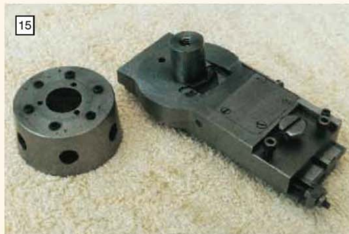
Turret slide with turret removed; the end of the intermediate slide and gib strip is visible at the right hand side. On the top of the slide is the cover plate over the turret indexing mechanism.
