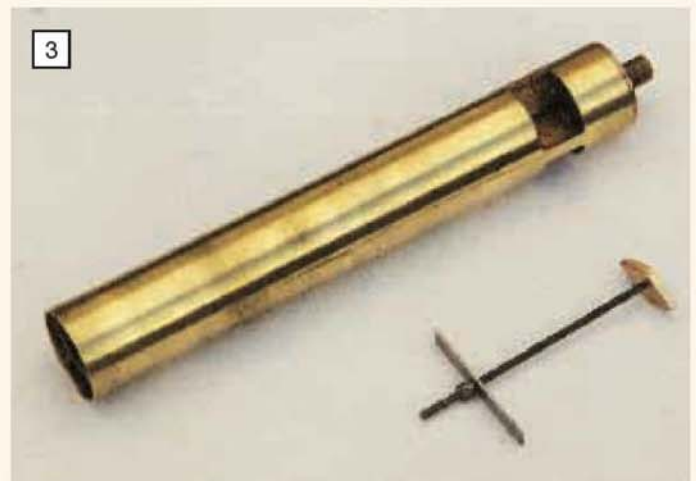
The finished Whistle; alongside is a tuning stop with its 4BA studding, locknuts and crossbar, set for the correct depth.
