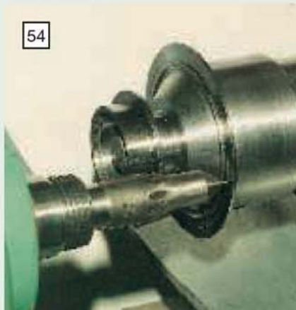
Marking the Top Dead Centre positions on the rear ball race housing.
