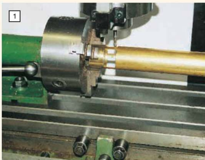
Dividing head set-up for machining the voice slots in the Whistle Tube. The snug-fitting steel plug to prevent distortion by the chuck jaws is clearly visible. Note also the table stops set to limit travel.
