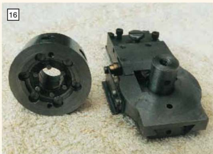
The turret slide and a view of the underside of the turret showing the indexing ring and tool clamps.
