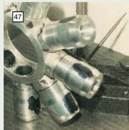
47 The second stage of marking out for the sparking plug locations.
