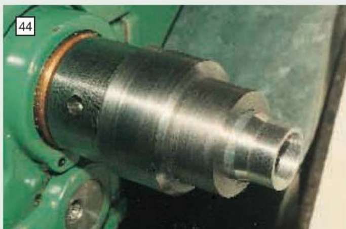
The first stage in machining the cylinder heads, once more using the master and slave chuck.
