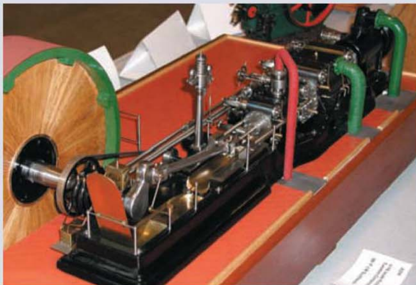
Left: Peter Southworth's magnificent 1:16 scale model of a Pollit & Wigzell tandem compound steam engine showing the wood panelled flywheel and crankshaft.
