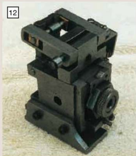
Shape turning cam assembly with hexagon cam fitted. The cam follower is just visible under the cam. At the top is the tilting roller frame with its roller. Just visible is the top of the cranked lever which transmits the movement of the cam follower to the roller.
