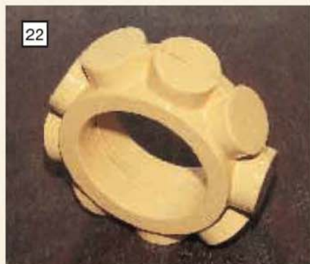
The modified crankcase pattern. This pattern avoids the use of a core.
