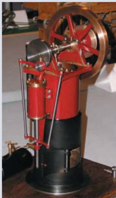
Anthony Mount's model Bailey's Vertical Engine. The characteristic 'V' connecting rods are evident in this view.
