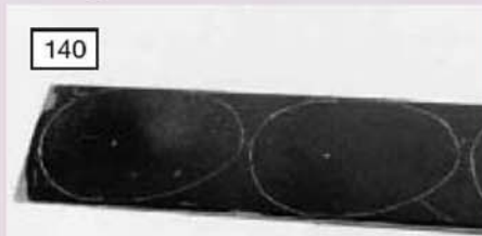
The 'egg' shields can be marked out on a strip of 1 x 1/32in. brass.
