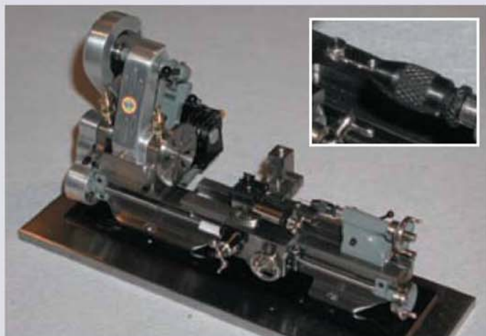
Left: Don Hoey's delightful 1:6 scale Myford ML7 centre lathe with (inset) a close-up of the tailstock drill chuck illustrating the superb detailing.
