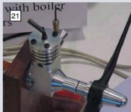
Mr. John Carter's diminutive 0.8cc diesel engine was to be found on the Guildford MES club stand.
