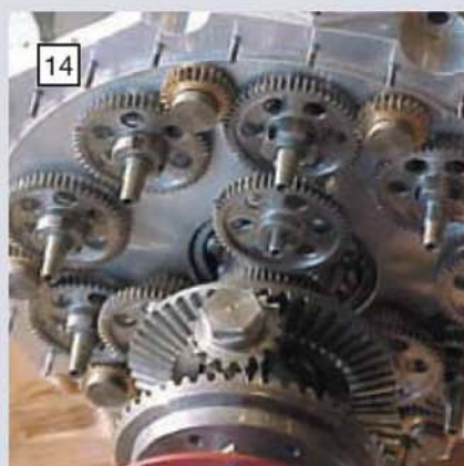
Below left: this 12-cylinder aero engine must sound splendid when running. Below: Brian Perkins' Aquila engine has recently been described in these pages; these views are of the sleeve valve gear train and the engine casing.
