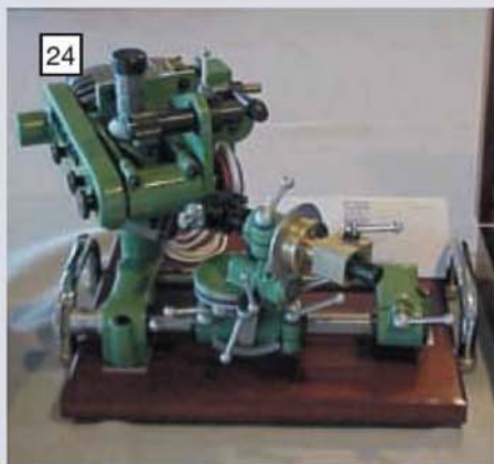
Mr. Graham Tyler's tool and cutter grinder to the original Quorn design by Prof. Dennis Chaddock was a Medal winner at a previous M. E. Exhibition and therefore was presented in the loan section of MEX 2001. Superbly finished, it was accompanied by a comprehensive boxed set of accessories.
