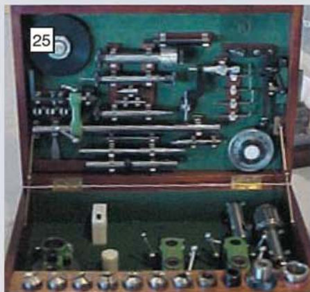
Mr. Graham Tyler's tool and cutter grinder to the original Quorn design by Prof. Dennis Chaddock was a Medal winner at a previous M. E. Exhibition and therefore was presented in the loan section of MEX 2001. Superbly finished, it was accompanied by a comprehensive boxed set of accessories.
