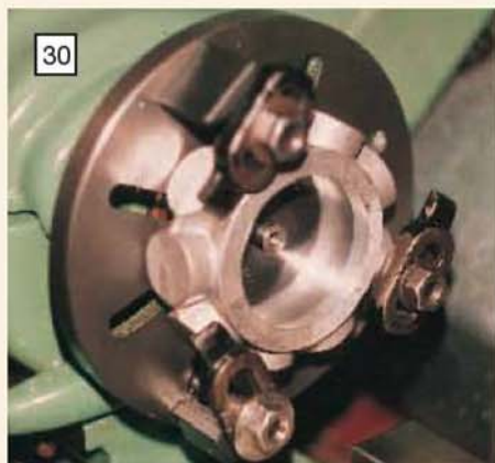
Crankcase reversed for machining the other face. Note the use of the locating disc.
