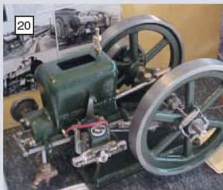
Mr. R. Field's barn engine was displayed on the Ickenham DMES club stand. Ignition is by means of a Minimag magneto.
