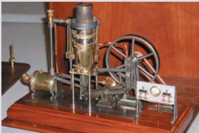
Also by Brian Marshall, this model demonstrates the principles of operation of the Reverend Stirling's original engine of 1816.
