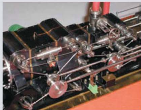
Left: Peter Southworth's magnificent 1:16 scale model of a Pollit & Wigzell tandem compound steam engine showing the wood panelled flywheel and crankshaft.
