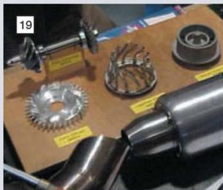
The component parts of a gas turbine engine include a rotor shaft assembly (in the cradle), a diffuser (front left), a vaporiser stack (centre), and a nozzle guide vane (front right).
