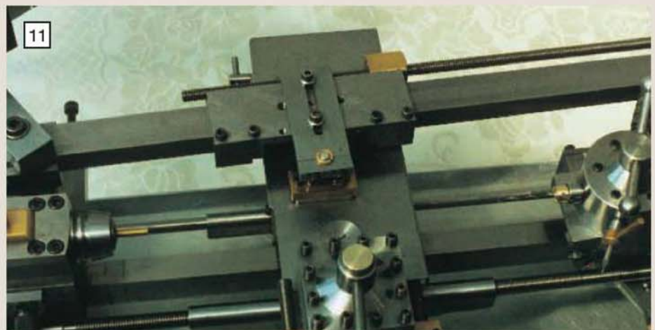
This view shows the connection between the cross-slide and the long slide on the auxiliary bed for turning long tapers. The connecting link is a ball joint.
