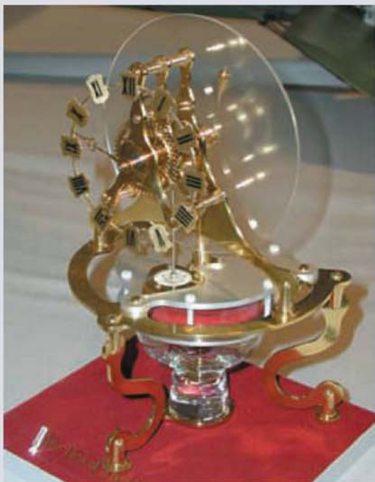
A novel hot air engine powered clock was exhibited by Wilfried Vermeiren and bore the label: Time files at a heartbeat.
