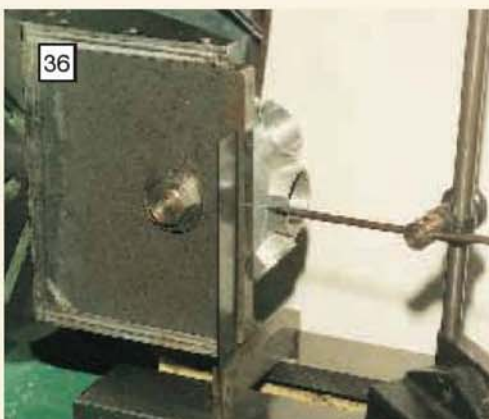
Marking the crankcase top dead centre positions. Note the use of a square on the lathe bed to ensure the faces of the crankcase are vertical.
