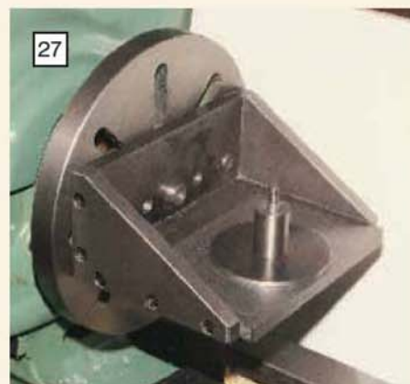
Crankcase machining angle plate in position on the faceplate with locating disc and mandrel.
