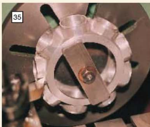
Final facing off of the front and rear of the cylinder seats.
