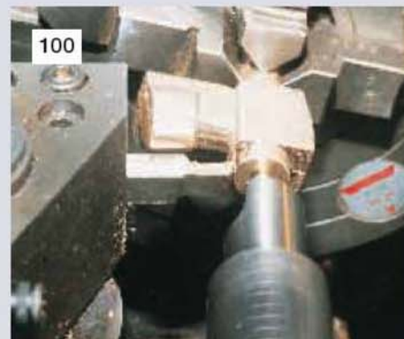
100 With the casting held by the chucking piece, the body is drilled, counterbored and tapped, and the boss machined at the same setting.
