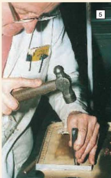
David Hall is seen here riveting up his tank sides. Note the quality of the rivets, even when out of sight, and the beautiful radius achieved on the angle without any notches.
