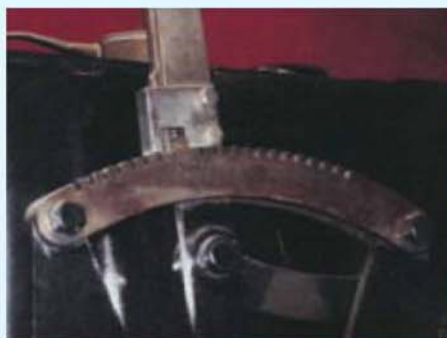
Details of the reverser on the full-size Jones 'Big Goods' at Glasgow's Museum of Transport.
