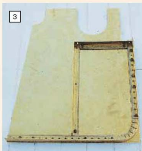
Left: John has laid the brass angle on to the tank side and drilled through for fixings.
