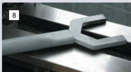
Mac uses a special spanner to remove the unit from the lathe spindle nose.
