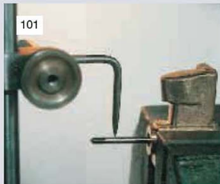
101 The casting is transferred to the milling machine and set by using a scribing block to check a steel rod inserted into the drilled bore.
