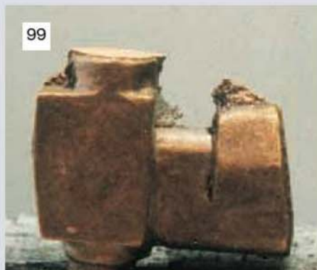
99 The chucking piece can be used to hold the casting in the bench vice for careful fettling work with suitable files.
