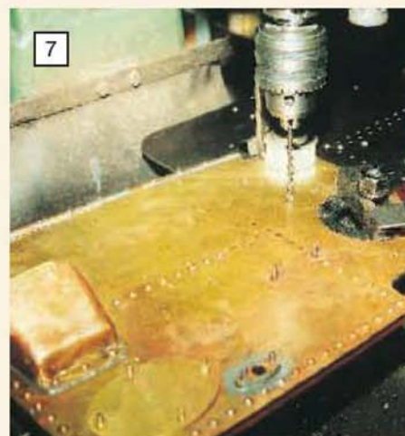
Above left: I have always had an instinctive dislike for hand held power tools and, given a chance, will always reach for a proper machine tool. It is good to see Stan Nipper using his milling machine here to drill the holes in the tank back/bottom plate. No doubt they are being co-ordinate drilled and are bound to come out in a beautifully straight line.
