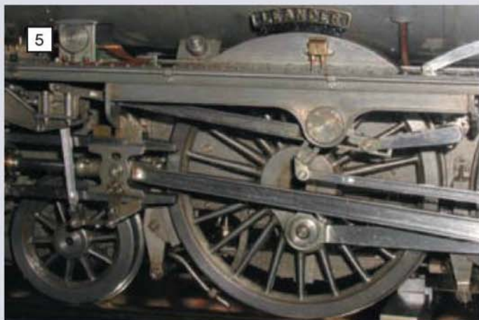
The wheels on Mac's 4-6-0 Leander were all fabricated; no castings at all were in fact used in the construction of this magnificent model.
