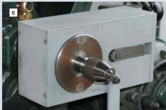
A view of Mac's high-speed milling and drilling head in situ on his own Myford Series 7 lathe.
