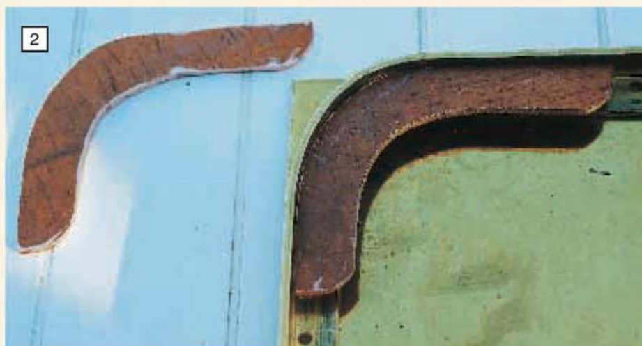
Above: John Freeborne cut notches in his \frac{1}{2} \times \frac{1}{2} in. brass angle to help it around the 2\frac{1}{2} in. radius on his 4in. scale Little Samson backtank.
