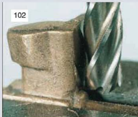
102 Once correctly set, the base of the pump body can be machined using the peripheral teeth of a sharp end mill. A blunt cutter will raise burrs.
