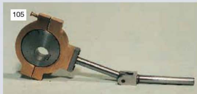
105 The pump ram or plunger is operated via the pump connecting rod which attaches to the eccentric strap shown here on its eccentric sheave.
