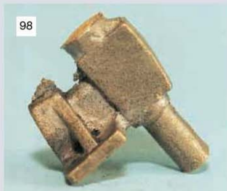
98 Pump body casting as supplied, seen here resting upon the useful chucking piece. A little cleaning up is required before machining begins.
