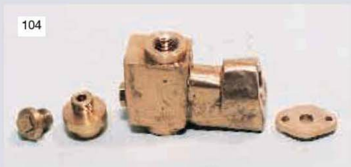
104 A view of the finished pump components including (left to right) top cap, valve seat, valve body and gland.
