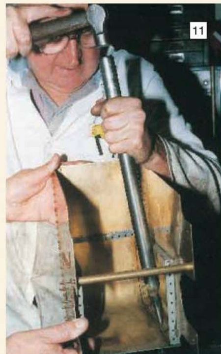
Final riveting up in grand style. An extra pair of hands comes in very handy. Yet another pair of hands was needed to take the picture.
