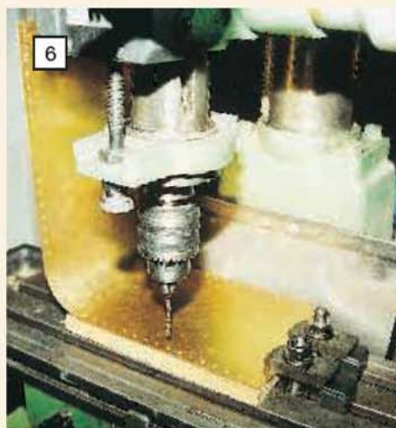
Above left: I have always had an instinctive dislike for hand held power tools and, given a chance, will always reach for a proper machine tool. It is good to see Stan Nipper using his milling machine here to drill the holes in the tank back/bottom plate. No doubt they are being co-ordinate drilled and are bound to come out in a beautifully straight line.
