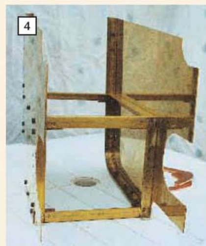
Left: John has laid the brass angle on to the tank side and drilled through for fixings.
