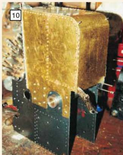
Above left: John's 4in. scale backtank is held together with an assortment of toolmaker's clamps prior to the spotting through of further holes.
