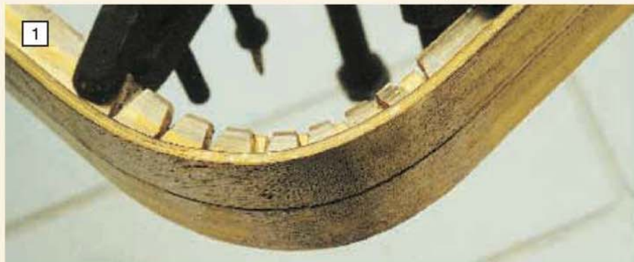
Above: John Freeborne cut notches in his \frac{1}{2} \times \frac{1}{2} in. brass angle to help it around the 2\frac{1}{2} in. radius on his 4in. scale Little Samson backtank.
