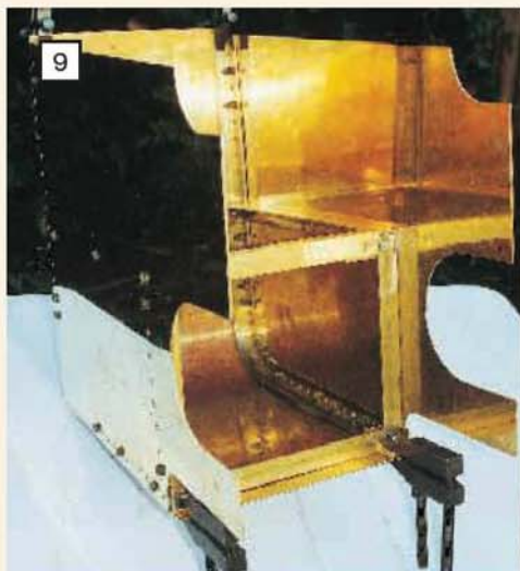
Above left: John's 4in. scale backtank is held together with an assortment of toolmaker's clamps prior to the spotting through of further holes.
