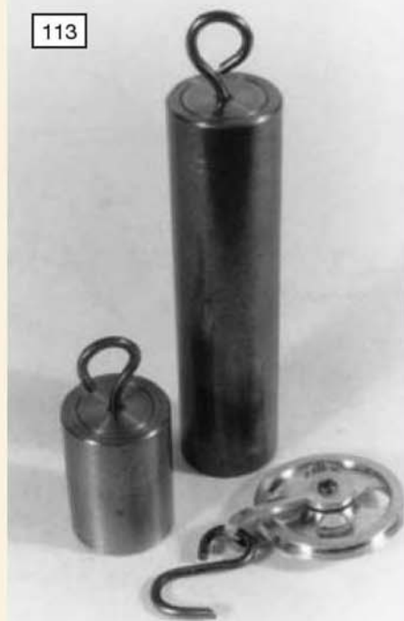
The driving and jockey weights with the pulley.
