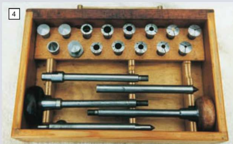
Above: the right-hand drawer of the two-drawer cabinet contains collets, draw tubes and two tailstock runners together with three collet blanks and a headstock centre.
