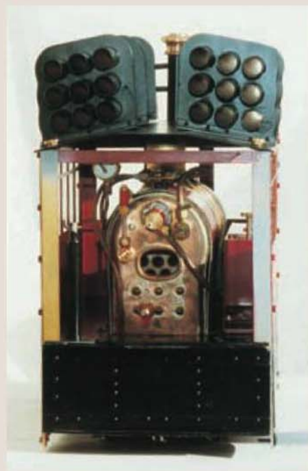
A driver's eye view of Burrell that also shows the layout of the condenser to advantage.
