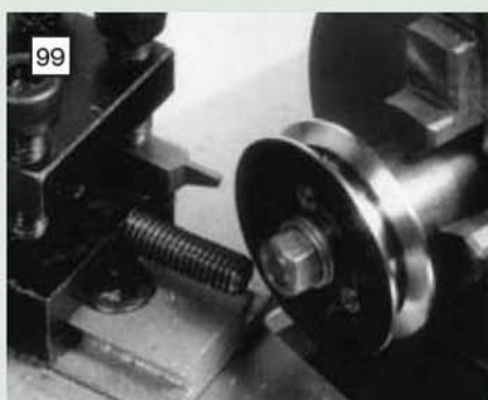
Machining the bevel edges on the pulley flanges.
