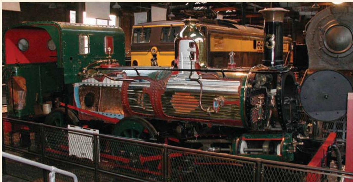
No. 3 Pender was built in 1874 for the Isle of Man Railway and now resides in the Power Hall of the Museum of Science & Industry in Manchester, sectioned so that the workings of a steam locomotive can be studied. Locomotive Lion (of Titfield Thunderbolt notoriety) can be found further down the hall.
