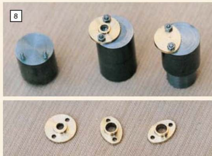
8 A simple machining technique followed by a minimum of hand work with a file produces glands of a neat elliptical form.
