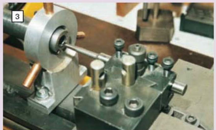
A fixed steady is used to support the workpiece while boring the No. 1 MT barrel nose taper which is finished with a suitable taper reamer.
