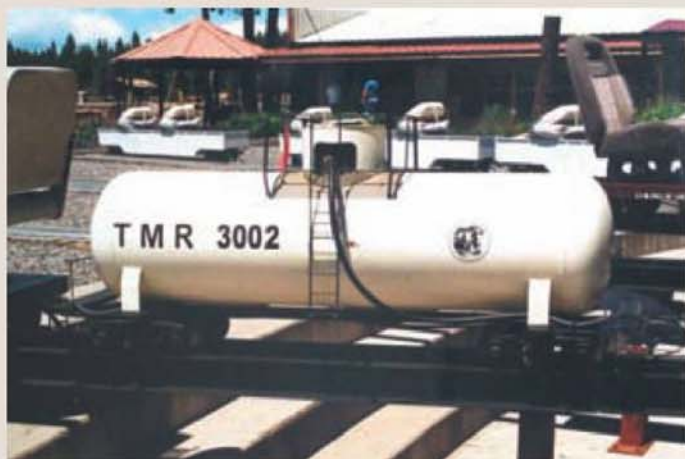
Just one of the 25 propane vehicles used to power the majority of steam engines on site. Each wagon contains 25 gallons of propane.
