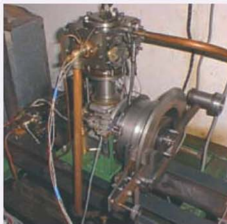
The single cylinder 50mm bore x 32mm stroke vertical engine used to obtain the results shown in the accompanying text.
