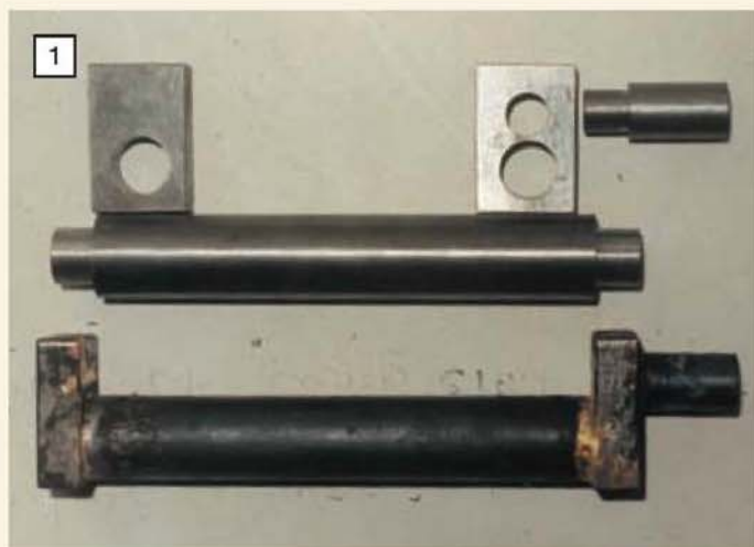
The main crankshaft assembly is shown here before and after brazing. The steel specified for the crankshaft is EN8 and slow cooling after brazing is recommended to avoid subsequent machining problems.
