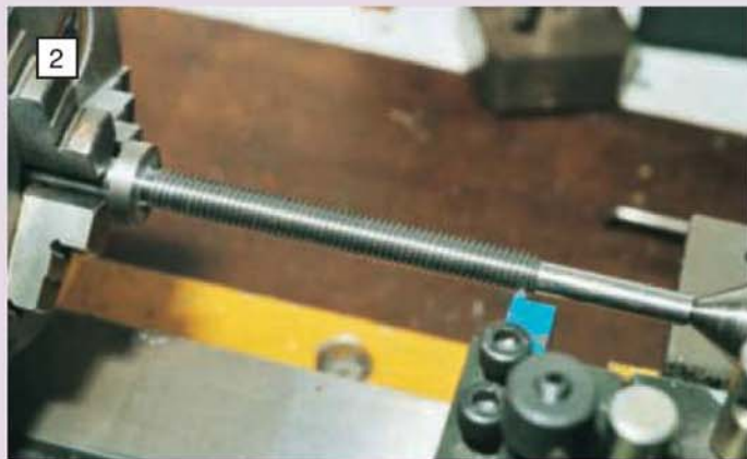
Screwcutting a left hand thread is always less trying than cutting a right hand thread because the tool travels away from the spindle during the cut.
