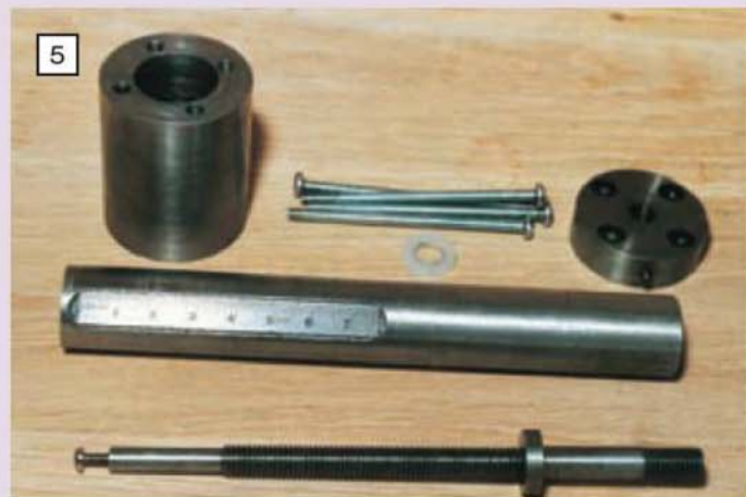
The new components with a steel rule in position in the groove machined for it and the pan head screws obtained from a local DIY store.
