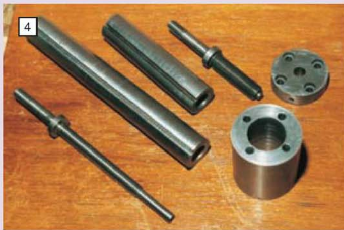
The new components (from lower left) and those which they replace (top centre). The original tailstock spindle featured a right hand thread.
