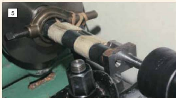
Above right: drilling the centres. In this photo, the main shaft has been drilled and the lathe cross-slide moved over to allow drilling of the crank pin.
