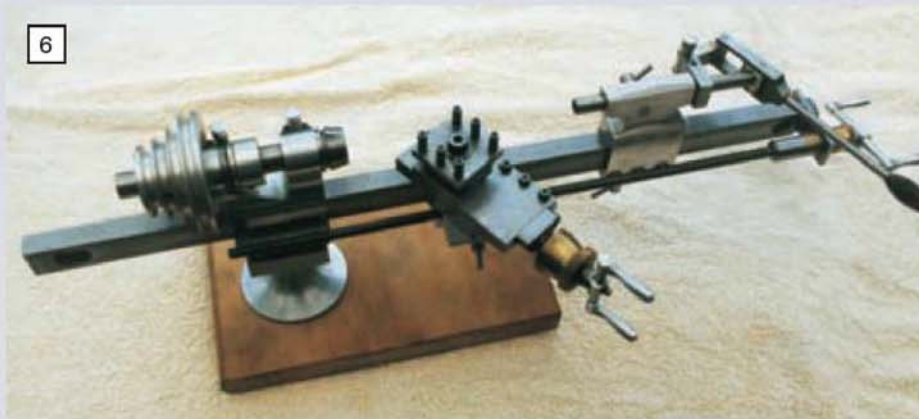
The lathe in its original concept form with bed extension at left for holding in vice but before adding screwcutting facility or mounting on the two drawer cabinet. Not 100% accurate but as near as now can be achieved.
