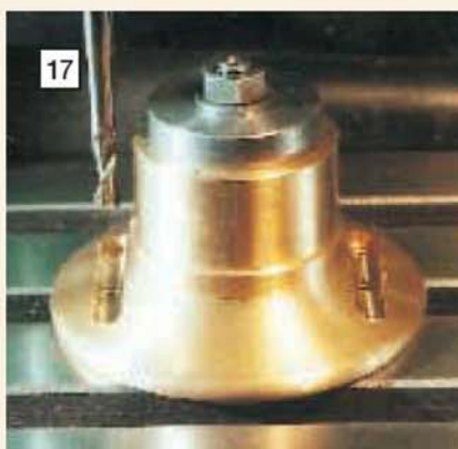
17 Two slots for the bearing bracket feet are carefully cut using a long series slot drill.
