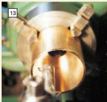
A large boring bar is used to finish the inside diameter of the cast gunmetal water jacket.
