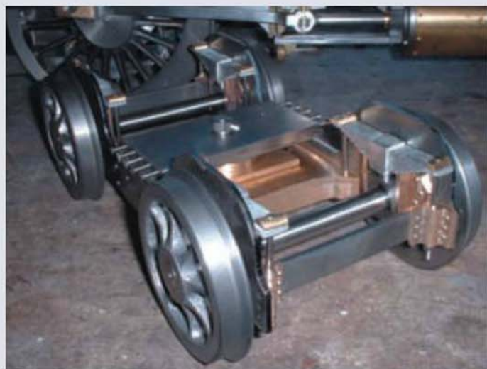
The bogie too is making good progress; prospective builders are invited to observe the close-to-scale wheel spoke profile.
