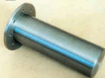
This finished hot cap took the Author some ten hours to machine from solid stainless steel bar!
