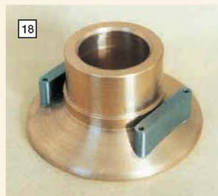
18 Completed water jacket cap with bearing bracket feet fitted using cheese head screws from below.
