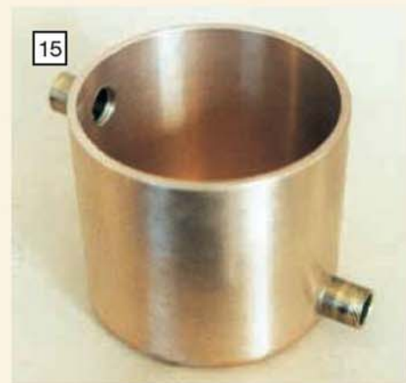
The finished water jacket is fitted with short lengths of thick wall brass tube.
