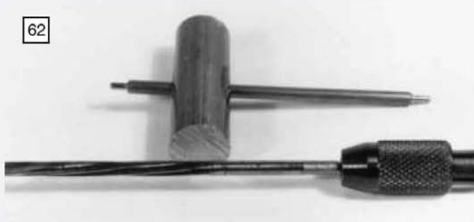
Showing a 1/8in. hand reamer.
