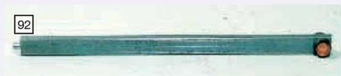
The eccentric rod with dowel and filing buttons attached.
