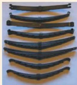
Some of Doug Hewson's springs made up from annealed spring steel and then hardened and tempered.
