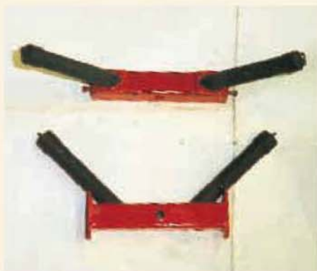
The sandboxes are fabricated from square box section material.
