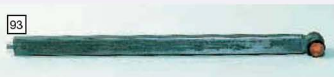
The radiused end has been filed and the bar suitably necked ready for final machining.
