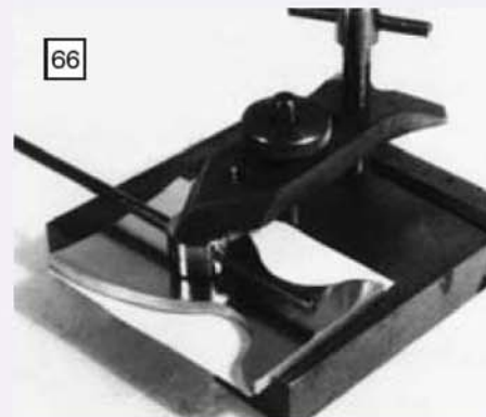
Using the jack screw of the holding clamp to press the collet home.
