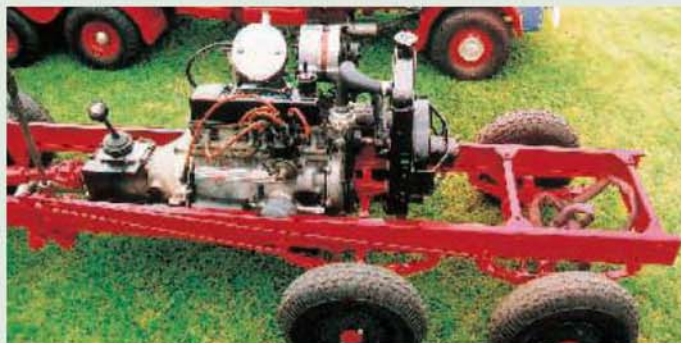
Very much under construction, Ray Stevens' eight-wheel Atkinson lorry. The engine came from a Reliant Robin and fits neatly between the frames.
