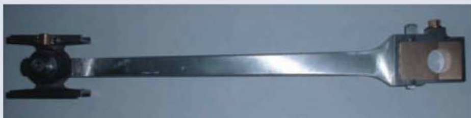
Construction continues apace; this con-rod and crosshead is for 'Loch' but differs from that for the 'Big Goods' only in length and lack of the fish bellied profile associated with the longer rod.
