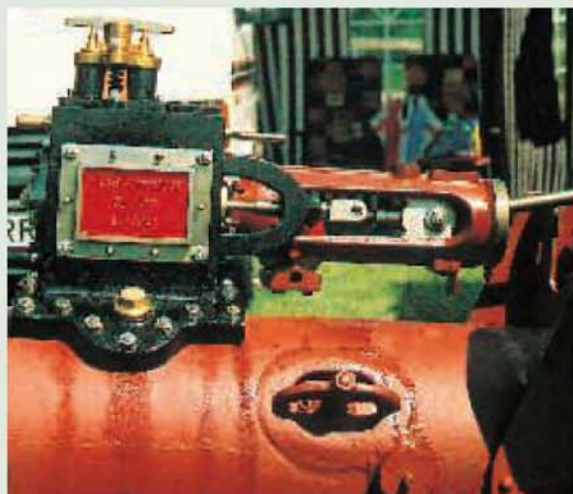
Right: Roy made his own patterns for this cylinder assembly. There is a lot of metal in the cylinder, which is topped with an elegant safety valve. A robust casting supports the valve spindle. The round bracket on the barrel is for the pump.
