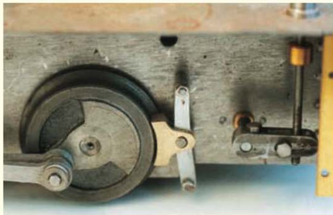
A close-up view of the brake gear. The large hole over the brake hanger is for the ash-pan dump pin.
