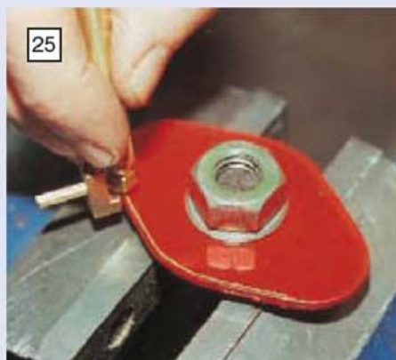
Left: the edge guide is used when the required line is controlled by an edge profile.
