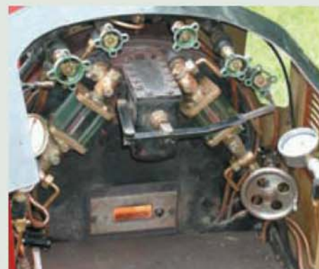
Neil Simkins runs down the grade towards Weston Central Station at the controls of No. 5901 Mt. Kenya completed in 1979 for William Heller by Milner Engineering and now resident at the NRM, York. The cab view (right) reveals, clockwise from left to right, the brake handle, boiler pressure gauge, steam valves for the whistle, large injector, blower, atomiser and cylinder drains, atomiser pressure gauge and reversing wheel. The fire is visible through the window at the bottom of the backhead.
