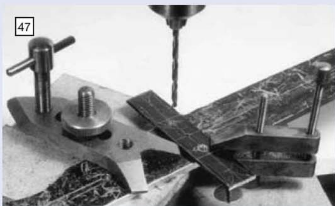
47 Drilling the front bridge piece. Second toolmaker's clamp removed for clarity.
