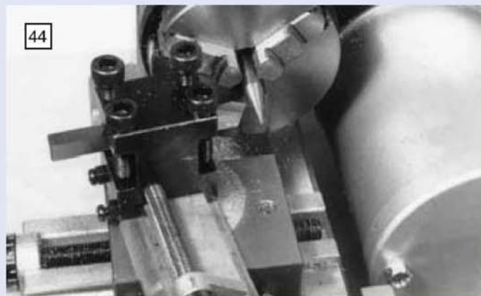
44 Taper turning one of the spurs.
