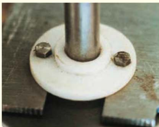
Left: the PTFE axle boxes bolt directly onto the frames. There are no hornkeeps, although they would be very easy to fit.
