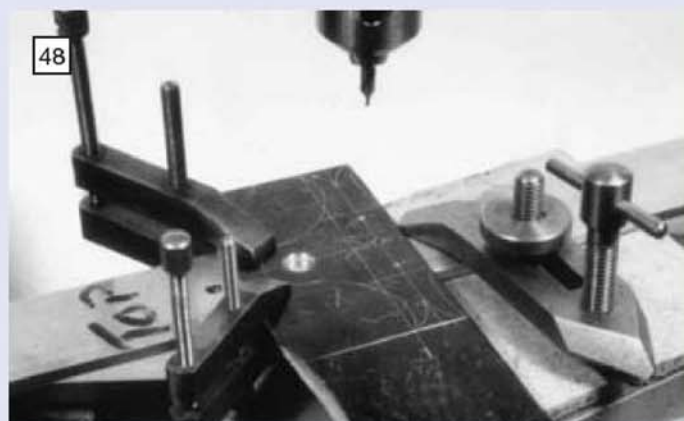
48 Using the centre drill to start the holes in the rear bridge piece.
