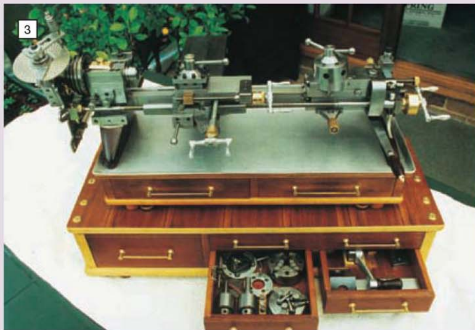
The lathe in its present form mounted on the original 2-drawer cabinet with integral drip tray. Underneath is the 5-drawer storage cabinet with two drawers open to show stored accessories. Note the dividing head mounted on the headstock.
