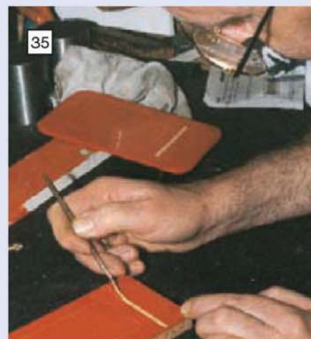
The viscosity of the paint used and the attitude of the fletcher to the work were variables which had to be right before success could be assured.
