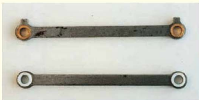
Above: two variations of the coupling rods. The top is a conventional type with oil bosses and bronze bushes. The lower is the type actually fitted with PTFE bushes. Both items were CNC marked and laser cut.
