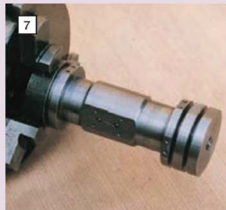
The cylinder components were machined as a group, leaving the stock material undisturbed in the 3-jaw chuck for as long as possible.
