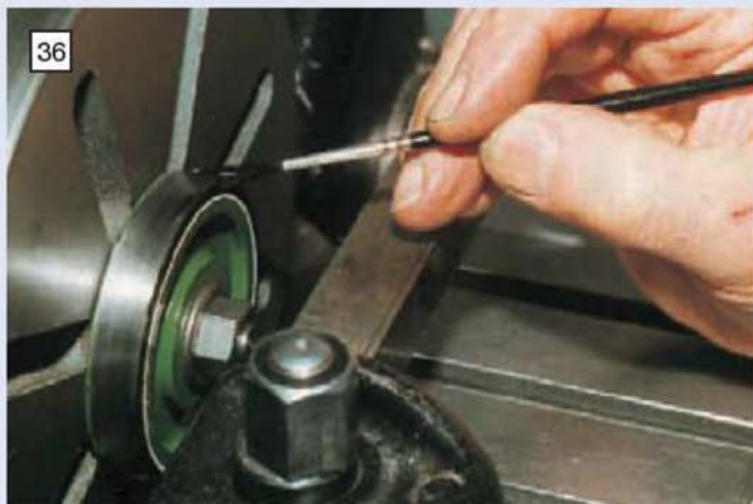
Frank preferred to use a small brush and found it easier to hold it like a pen when applying colour to a wheel mounted on the faceplate.
