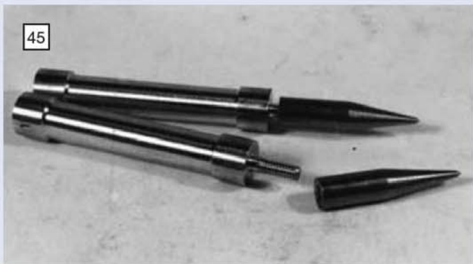
45 The completed dial pillars and spurs.
