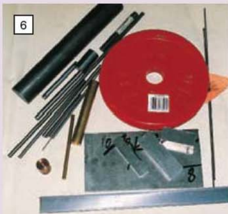
Most of the components for the writer's model were prepared from this group of materials. The large red cast iron weight became the flywheel.
