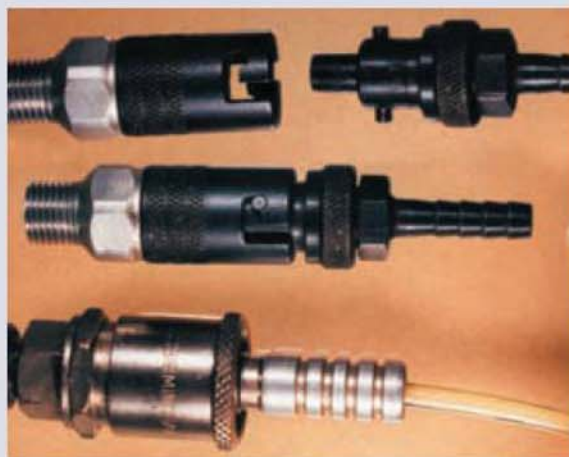
Right: Air line couplings. Top, push and twist; bottom, an 'Enots' brand push and click. Many types are available, both larger and smaller.
