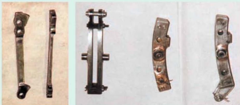
The subject of some frustration, the combination levers (left) had to be remade while the expansion links (right) are fabricated using separate pivot pins secured in place by brazing.
