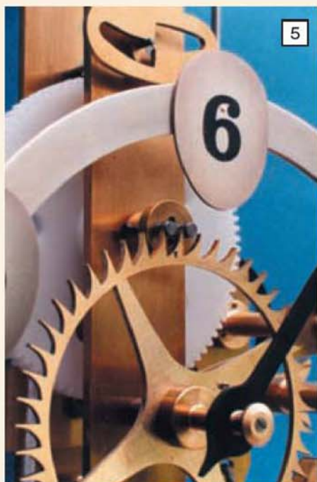
Close-up of the escapement and 2-pin suspended lantern pinion.
