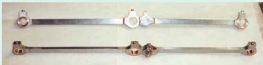
Below: The coupling rods were machined from bright mild steel. They are not fluted but are fitted with oil cups as per the prototypes.
