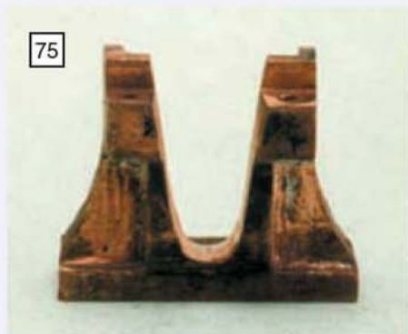
Bottom left: the support bracket for the guide bars. Apart from machining the base to get it flat, it is finished by hand filing.
