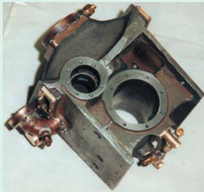
Top left: The three cylinders which are fitted with cast iron liners, represent a considerable amount of work.
