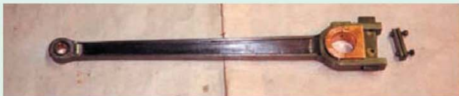
Above: The inside connecting rod is fluted on both sides and is shown here fitted with its big end bearing and locking plates.
