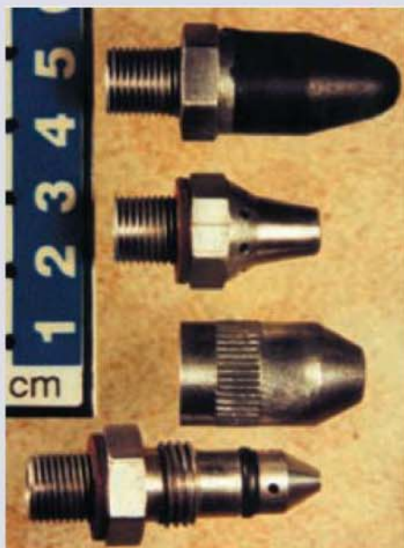
Air line jets. Top: a plain rubber tipped jet, useful to clear pipes, etc. and to avoid damage to polished work. Centre: so-called safety air jet; eight sideways jets deflect grit and swarf from the user. It is not, however, foolproof. Bottom: this two-part jet can provide a variable flow and is also suitable for spraying liquids.
