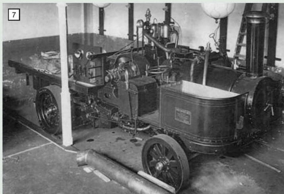
This wagon was fitted for electric light generation for the West Country showland proprietors Marshall Hill and photographed at the 1904 Smithfield show. Other pictures taken on the same occasion show an extension chimney to carry the smoke away and the globe lights above illuminated. This wagon has a locomotive boiler and a number of recognisable Little Samson fittings including the steering wheel and chimney cap. The engine for electric light generation was a duplicate to the engine underneath but direct coupled to the generator.
