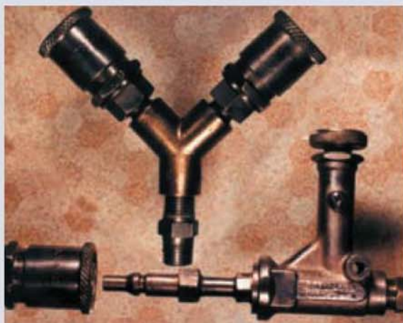
Left: Air line couplings. Two sockets are fitted to the 'Y' fitting which is connected to the air supply. The needle valve can be used to reduce the rate of flow, useful to supply an air/reducing valve or an air/gas muffle furnace.
