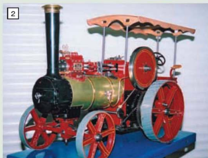
Stan Nipper's very handsome Little Samson approaches completion. Still to be fitted are the gear casings and motion covers. The canopy with its curvy sideboards transforms the engine.
