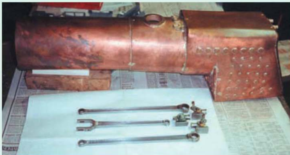
The boiler was built by Priory Boilers in Warwickshire. The outside connecting rods seen here are in mild steel and are shown with the fabricated crossheads described in the accompanying text.
