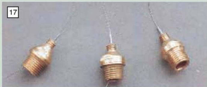
Lining nozzles made from hypodermic syringe needles
