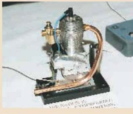
First Place in the Stationary Engines Section went to P. P. Decker for his 4in. Barr & Stroud sleeve valve motorcycle engine.
