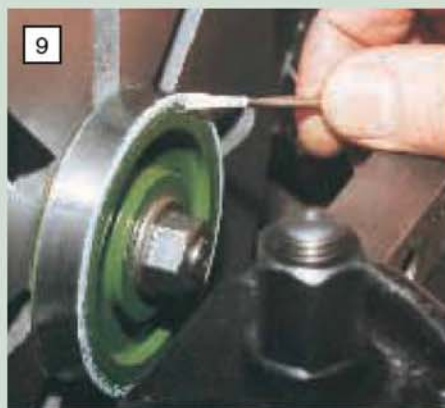
Applying the white line. Note the method of application
