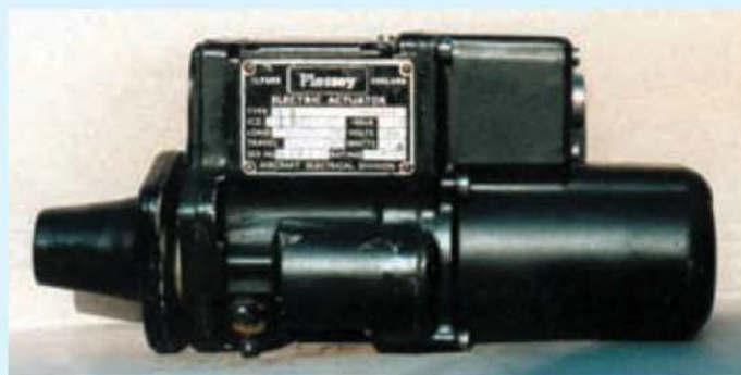
The 24V motor as used by Derby SMEE for point operation.
