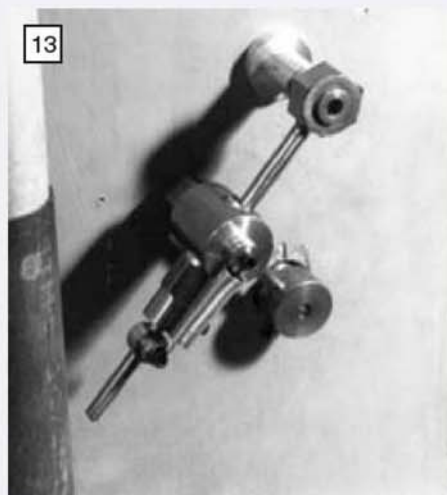
13 Linear bearings removed excess friction from the mechanism and the extra inertia helps it get it over centre.
