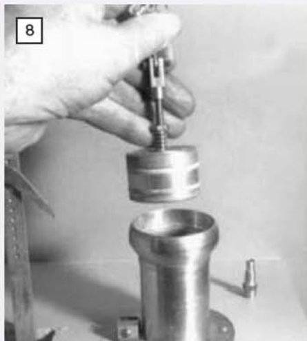
The piston has two 'rings' and 0.015in. clearance. The spring and nut provide for delicate adjustment of friction versus sealing.
