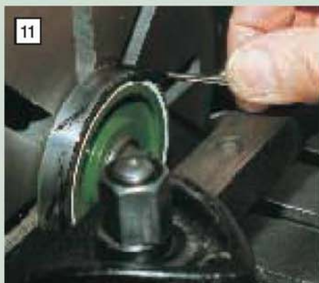
Applying the black line after the white line has dried and the position has again been knifed
