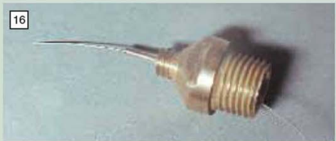
Lining nozzles made from hypodermic syringe needles
