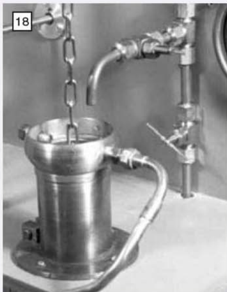
18 Water is dripped onto the piston to seal the rings. The second valve is to feed the boiler. The clamp on the cylinder avoids possible distortion due to soldering.
