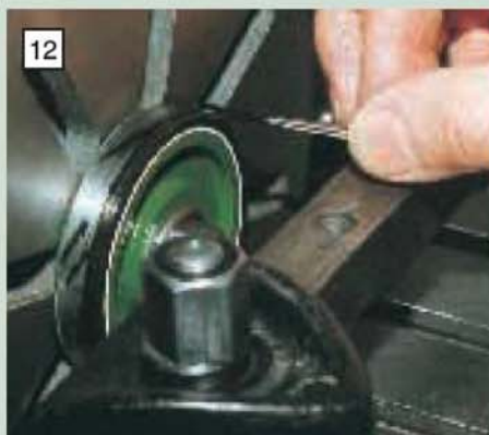
Applying the black line after the white line has dried and the position has again been knifed
