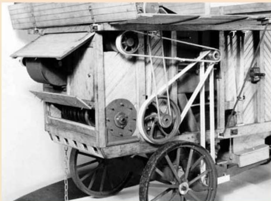
Above: This Ransomes 54in. threshing box model illustrates the author's remarks regarding belts — "Despite the many open and unguarded belts, with open flywheels and pulleys, accidents were very rare indeed. Everyone handling threshing tackle, from the farmer downwards was aware of the dangers which could arise so easily". Below: An oil painting showing Steam threshing on the farm.
