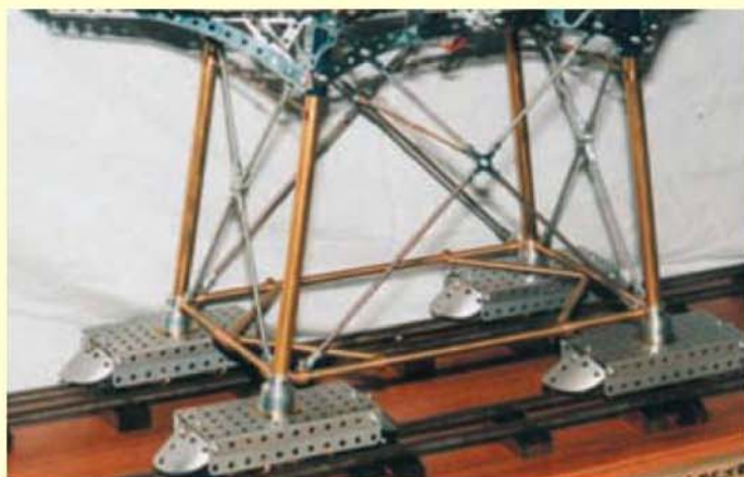
Lower leg construction and frame bracings. Also seen to advantage are the aluminium adapters and modified wheel disc sole plates for the leg mountings.
