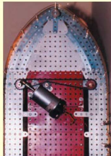
The motor upper reduction gearing by worm and pinion and the cross drive to the opposite down shaft by chain and sprockets.
