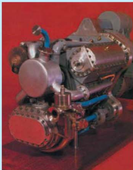
The last opposed piston model known to the author is Roy Amsbury's superb Deltic type locomotive engine.
