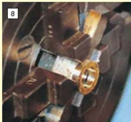
Turning eccentric strap with spacer behind it in the 4-jaw.
