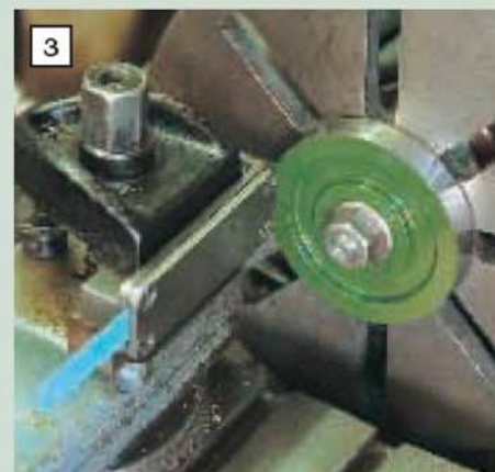
The knifing tool in the special holder
