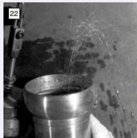
22 The spray of water from the injection nozzle was enough to reach the bottom of the piston and shuts off about half-way down.
