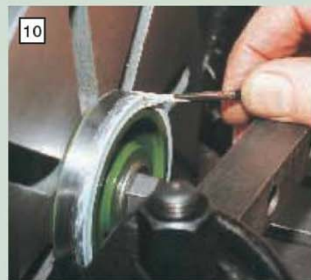
Finishing the white line. The heel of the brush is now well down
