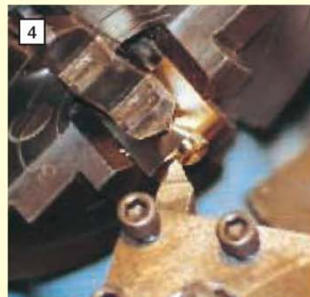
Machining the valve spindle bosses on the ends of the steam chest.
