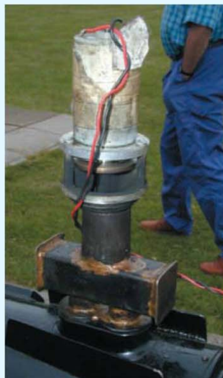
Typical 12V dc electric fan type blower adapted to suit the double chimney arrangement of LBSC's Heilan' Lassie. Some users of this type of blower have ingenious arrangements for speed control.
