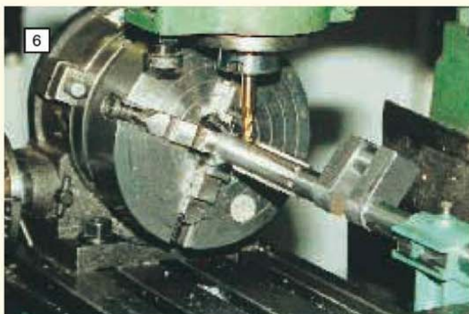
Left: The crankshaft splines are machined with the crankshaft held in the 4-jaw chuck and supported on a steady. The rotary table is used to index the crankshaft to produce the six splines. (Photo S. Nipper)
