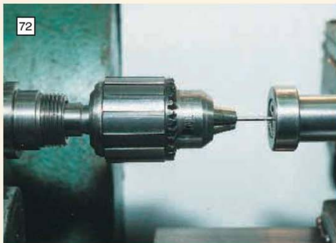
Small diameter work is not always firmly gripped in a 3-jaw chuck, particularly when threading with a die when forces can be considerable. The tailstock drill chuck is designed to grip small diameters and when fitted in the headstock will hold small diameters much more securely.
