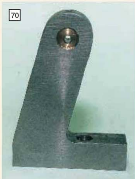
As well as being threaded, the end of the valve spindle is reduced in diameter to act as a guide. This small diameter is difficult to machine without support; shown here is a suitable device as previously described in these pages. The brass bush is drilled from the headstock to suit the diameter of the work, and a new bush is fitted each time it is used. Rigidity is assured by machining as close as possible to the steady.
