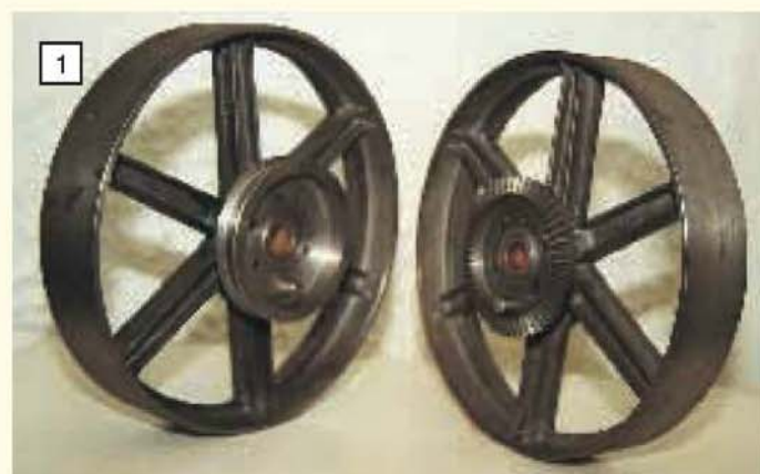
Left: A pair of 3in. Little Samson back wheels. One has the brake drum fixed to it and the other a differential bevel gear. Note the end of a driving pin visible on each (Photo: S. Nipper)
