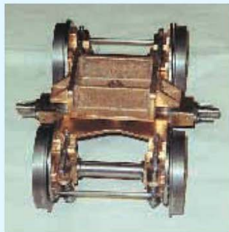
Two views of the writer's front bogie, with which he says he is well pleased. The bogie frames are in 1/8in. steel as shown on the drawings and needle roller bearings have been fitted. Castings are available from M. J. Engineering, deep in S.R. territory.
