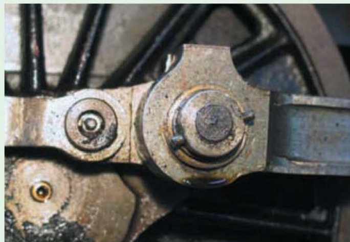
The coupling rod joint is secured in a similar fashion to the crosshead pin, utilising a 5BA nut in a recess big enough to accept a box spanner.
