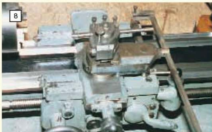
Left: An internal keyway cutting set up on a 4 1/2in. Boxford lathe. The feedscrew has been removed from a topslide to convert it into a planing attachment.
