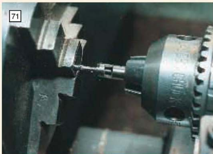
The writer's own running down tool in use for machining a small diameter. Sometimes called a rose bit, it steadies the workpiece while reducing its diameter to a size predetermined by the bore of the cutter which features cutting teeth on the end facing the lathe headstock.
