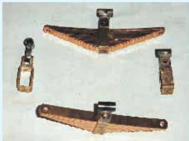
Above: The horn blocks and keeps were carefully finished before being assembled into the frames; an approach which required much corrective afterwork!
