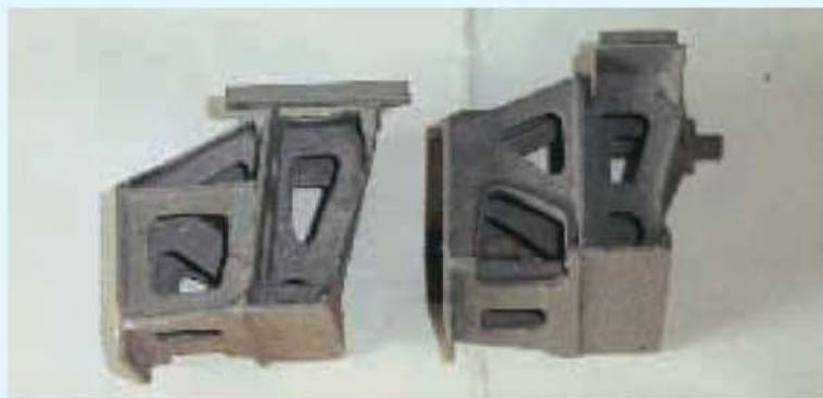
Above: The parts for the superbly detailed outside guide bar brackets were assembled by silver-soldering; regrettably they are to the West Country design! Left: The inside motion bracket required modification as described in the text.
