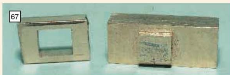
Above: the two parts of the valve; the rectangular section standing proud on the larger piece locates the cut-out to prevent movement during silver-soldering.
