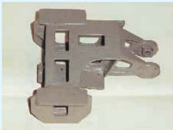
Above: The parts for the superbly detailed outside guide bar brackets were assembled by silver-soldering; regrettably they are to the West Country design! Left: The inside motion bracket required modification as described in the text.
