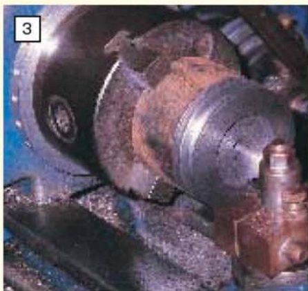
3 Components for the smaller models may conveniently be cut from the solid. Here a 1in. scale brake drum is being machined from a solid billet of cast iron. (Photo: J. Milne-Fowler)
