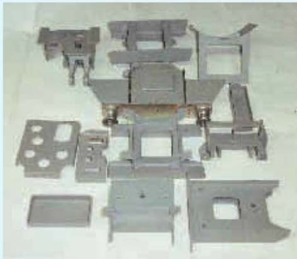
Left: Stretchers, stays and buffer beam for GSN were made up with a few alterations as described in the text and posed for a photographic record.
