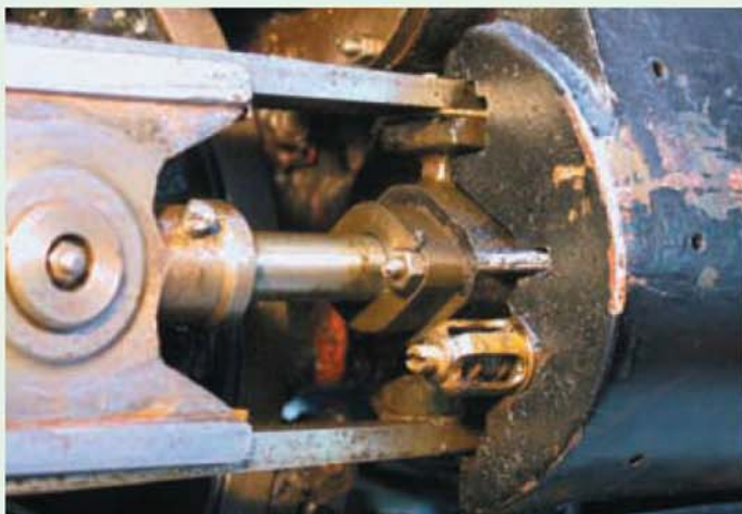
A view of the rear face of the cylinder showing the packing gland. The studs should be set at 45deg, but would incur additional patternmaking costs.
