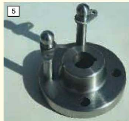
5 This driving boss serves as a stand for two completed driving pins. (Photo: S. Nipper)
