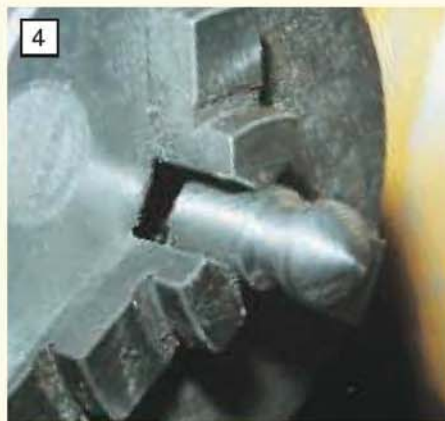
4 Close inspection of the machined surface of this ball end of a driving pin reveals rings resulting from the co-ordinate work in initial turning. (Photo: S. Nipper)
