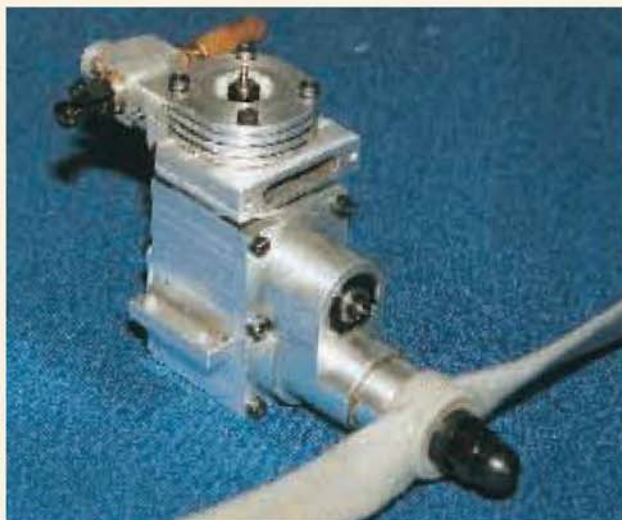
Left: A 6.5cc sleeve valve engine built by the author to the Nicholson design.
