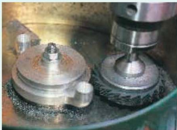
Left: After several false starts, the fins were machined into the inlet manifolds using a stack of saws mounted on an arbor.
