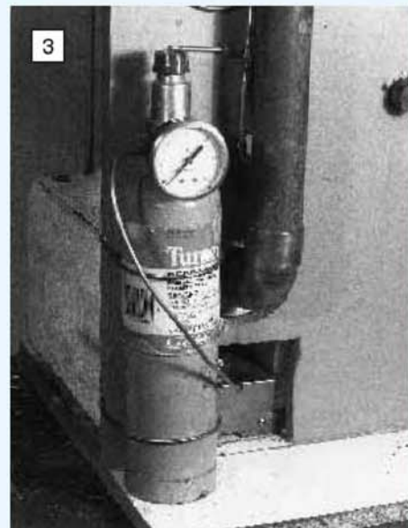
Fuel is propane supplied through a pressure regulator. To maintain 1/2psi in the boiler, only 2psi is required on the fuel.
