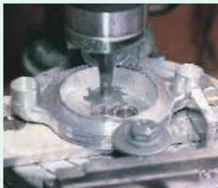
The inner cavity was machined into the inlet manifold using a home-made cutter and offsetting the workpiece on the rotary table.
