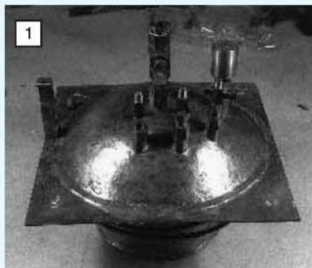
The boiler is made in three pieces. An exercise in copper forming, the dome was finished by hammer forming over a bowling ball.
