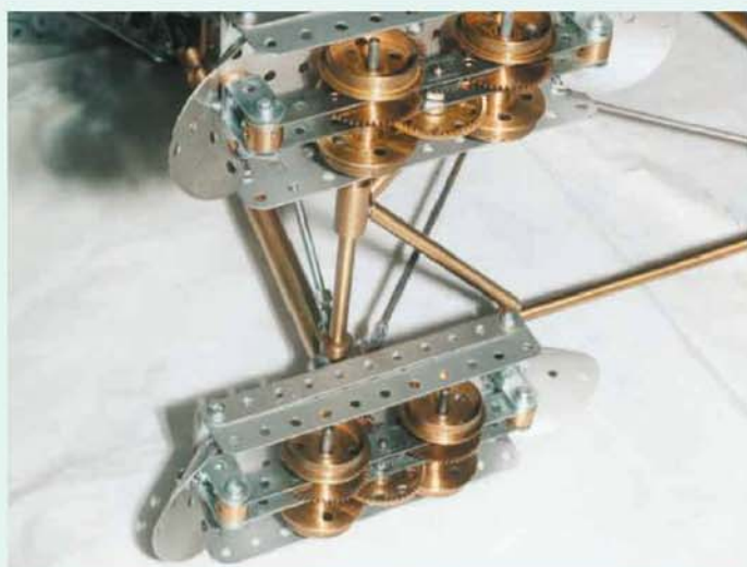
A view of the 'O' gauge powered bogie constructions in the sponsons which feature components made by the writer.
