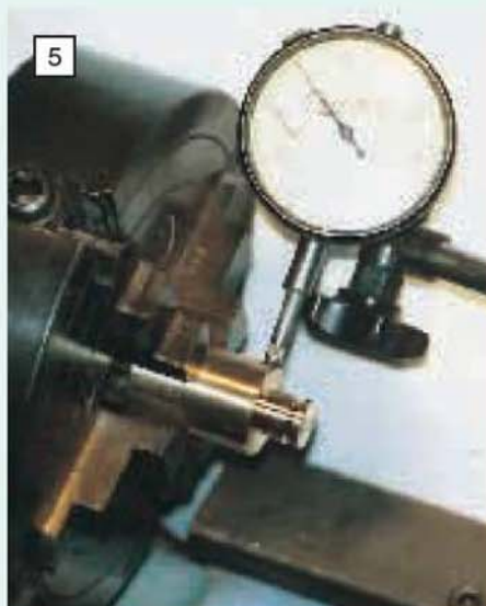
Centring the piston and rod in the turning fixture with the aid of a plunger type dial gauge.
