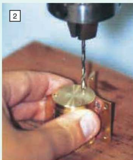
Spotting through the drilled front cover holes to locate screw holes in the cylinder.
