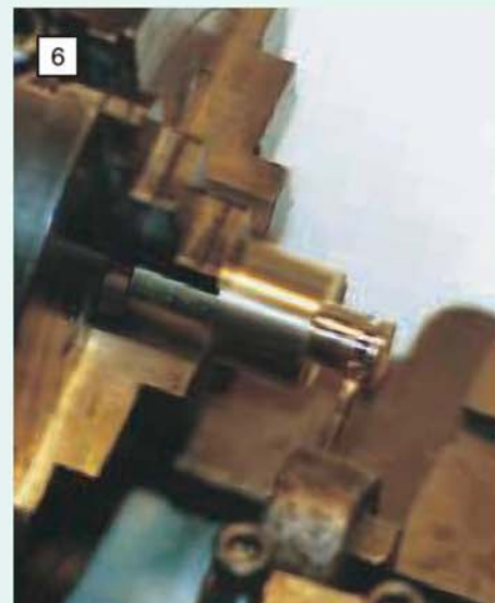
Machining the piston packing groove while the piston and rod are held in the mounting fixture.
