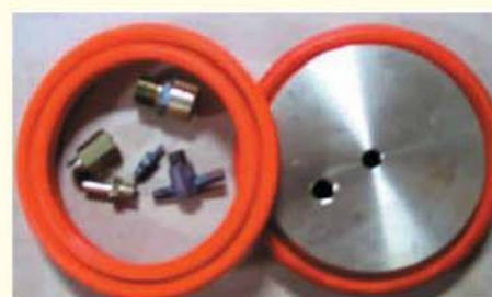
A U-section ring seal for the brake cylinder piston permits greater dimensional tolerance on the components.
