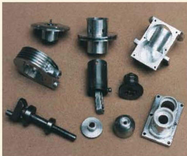
Right: Component parts of a modified Nicholson sleeve valve engine by Bob Dunn.
