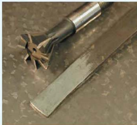
A 60deg. dovetail cutter (top) and the cutting edge of a commercial flat scraper; note the scraped texture on the surface plate on which they stand.
