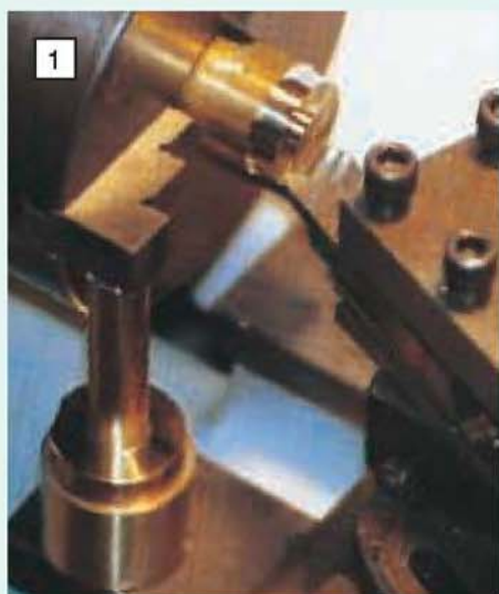
Using a stop under each jaw in turn to index for three screw hole positions.
