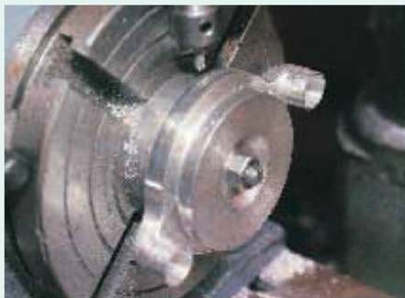
Right: Surplus material between each pair of inlet manifolds was relieved with the job clamped to a vertically mounted rotary table.
