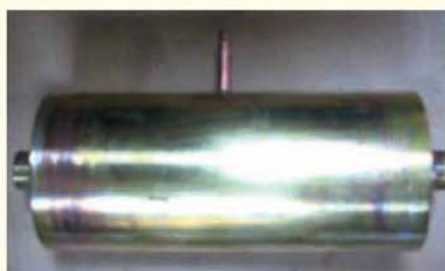
A vacuum reservoir improves braking efficiency by increasing the effective volume above the brake cylinder piston.
