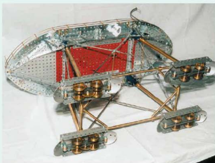
A view of the underframe showing the underside of the deck plus the lower gearing to the two powered sponsons.
