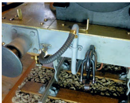
Photo 12: Standard installed with dummy pipe.
