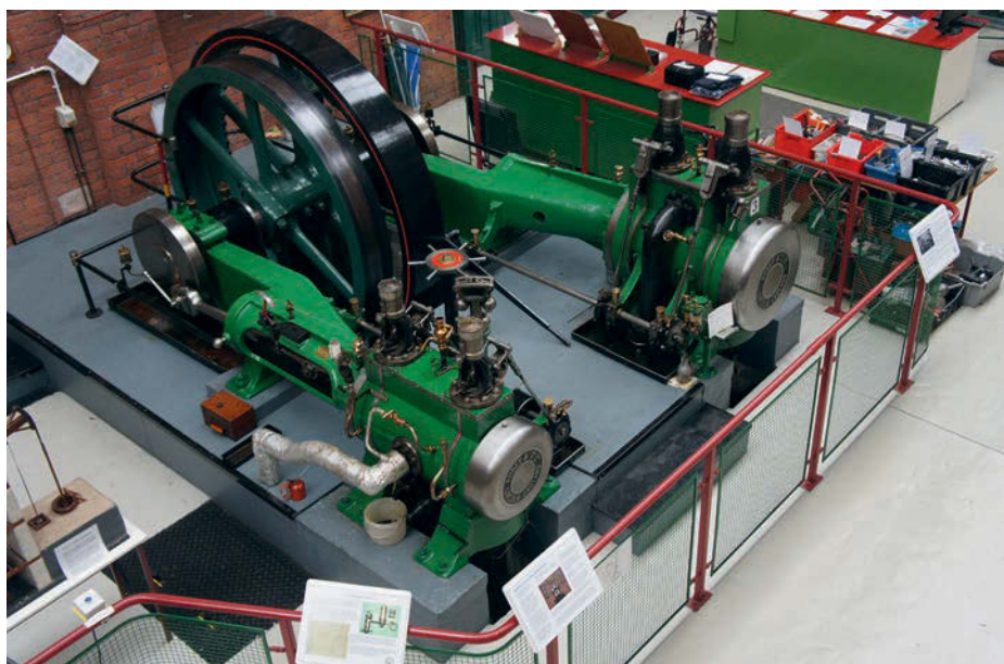
Photo 23: Twin cylinder Robey compound was built for demonstration and experimental purposes in a college.
