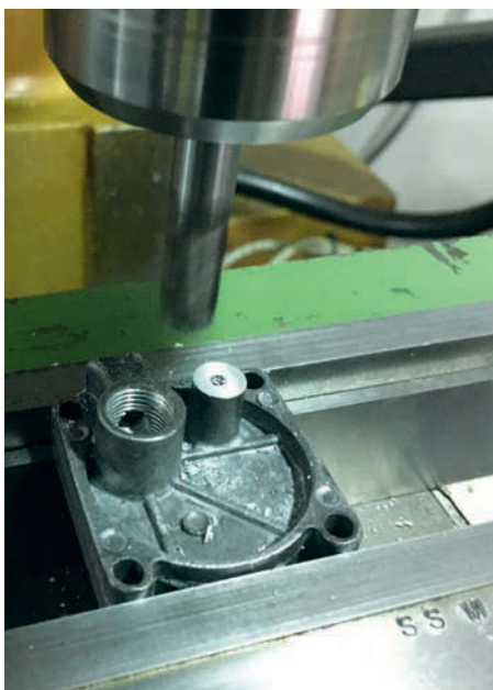
Photo 21: Milling off the handle locating lug was easy because this mazak die casting was not resistant at all.
