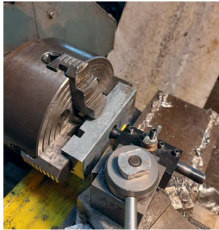
Photo 4: Boring the hole for the shaft.
