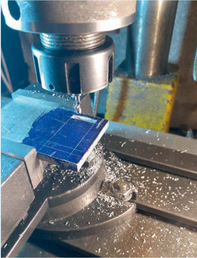
Photo 2: Machining the new end stop from plate.
