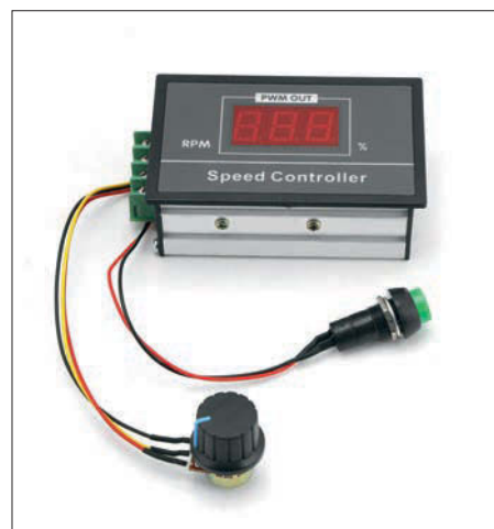
Photo 24: Well worth the price for the convenience of having a digital readout, this is the speed controller with an on/off switch and a rheostat already attached.
