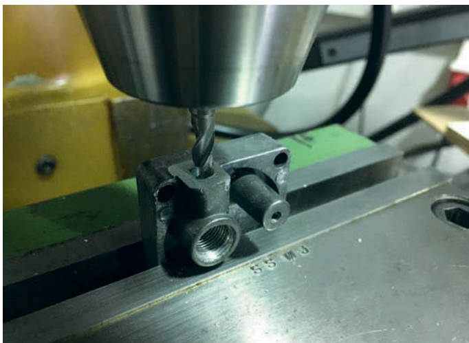
Photo 19: About to take the plunge to create a circular section 5mm diameter hole to tap M6.
