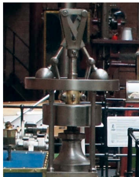
Photo 29: The cross-arm governor is an unusual design, one of just three known examples.
