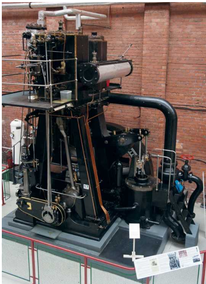
Photo 21: Diamond rope works engine seen from the side showing the beam operated condensate pump.
