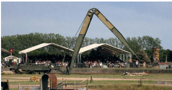
Photo 18: The Titan Armoured Bridge Layer can set up a 25 metre bridge in minutes.
