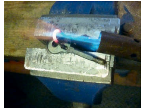
Photo 8: Annealing the links to remove spring back.
