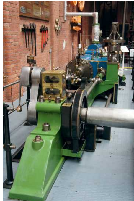
Photo 28: Crankshaft bearing and lubricators. Mill engines needed regular oiling at many points.
