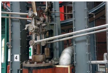
Photo 17: Rather than use crossheads and slides to guide the piston rod the Kenyon engine uses an adaptation of Watt's parallel motion devised by Phineas Crowther in the North East that was much used for colliery winding engines.
