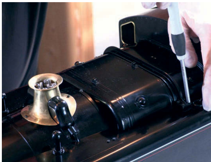
Photo 11: Installing fire box top over.
