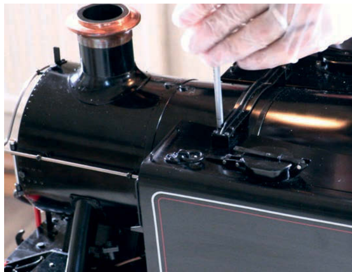
Photo 12: Securing the boiler to side tanks.
