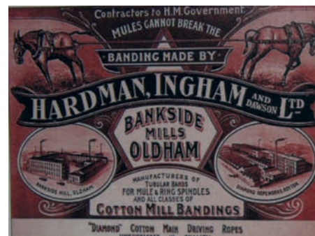
Photo 20: Advertisement for the Diamond rope works. One of their products, cotton rope, was much used in cotton mills to drive line shafts. Cotton rope was strong and quiet in operation.
