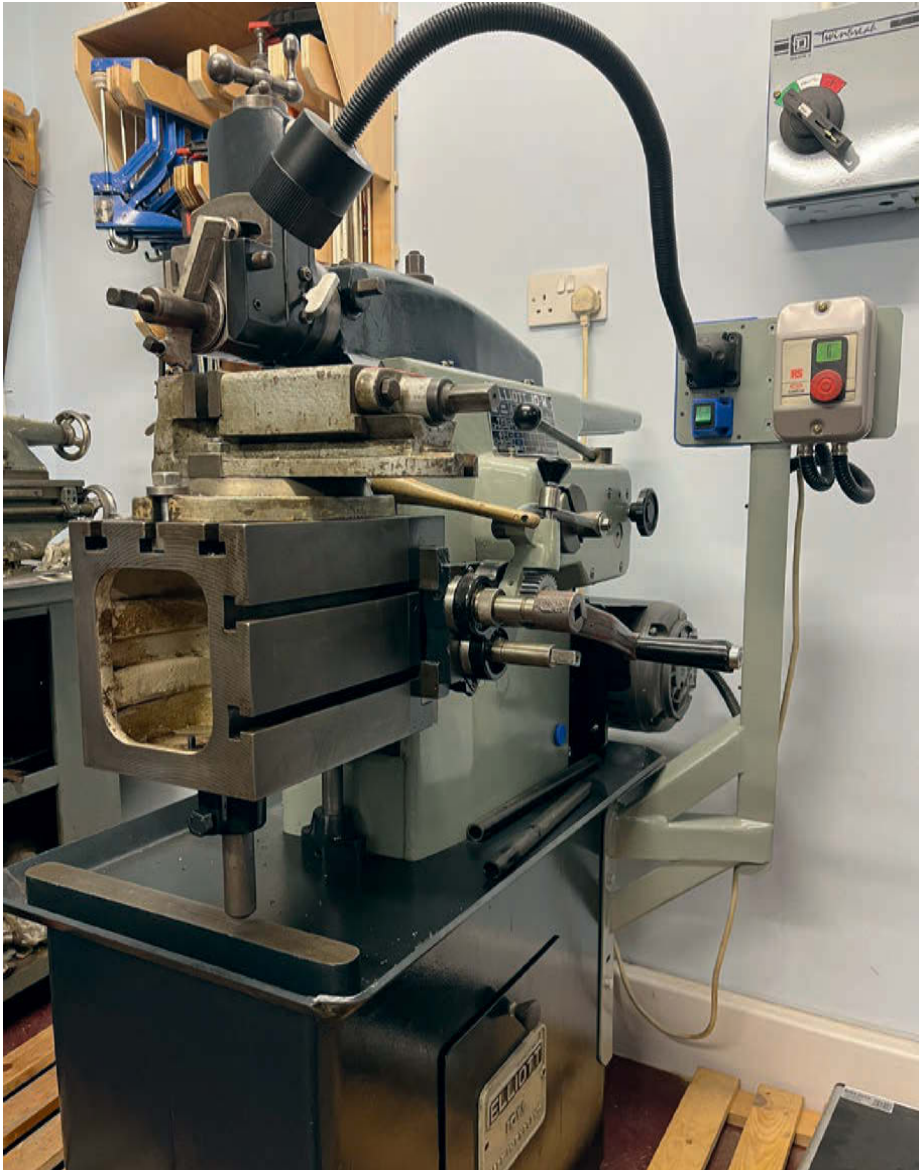
Photo 35: Elliot 10M Shaper refurbishment and improvements.
