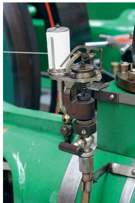
Photo 25: Taking an indicator diagram was an essential part of a mill engineer's work. A diagram would show if the engine was working efficiently. It is hoped to feature more about indicators in a future article.
