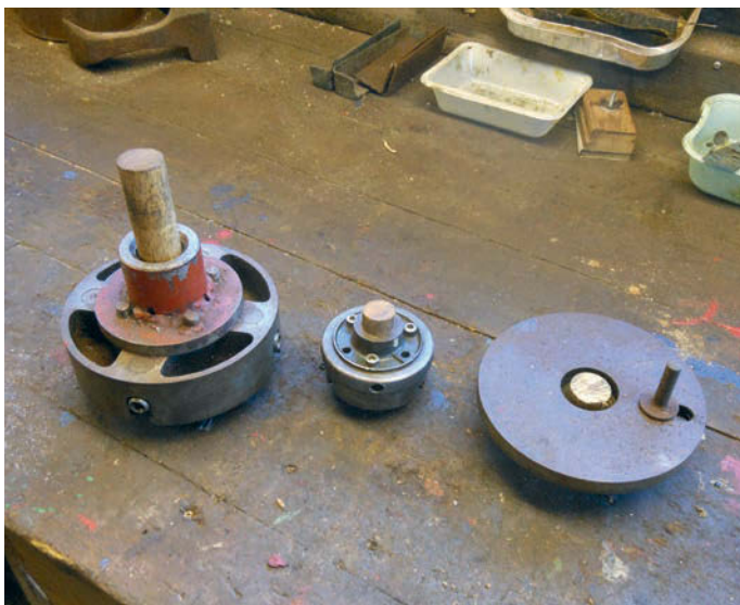
Photo 2: Wooden plugs to protect chuck threads.
