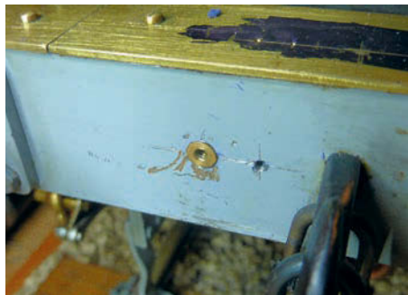
Photo 10: Bush repair after grinding out a broken tap.
