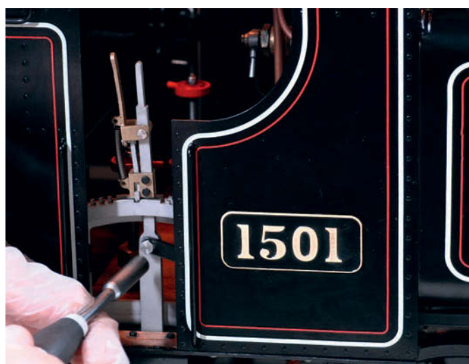
Photo 14: Securing the reversing lever to reach rod.
