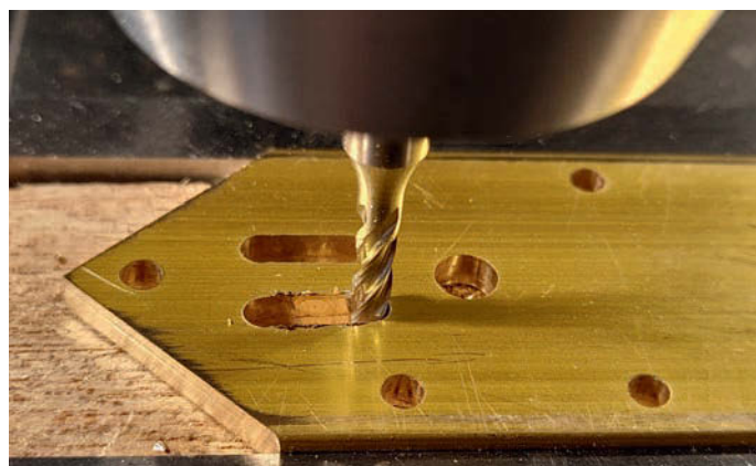
Photo 12: Machining slots in the port plates.
