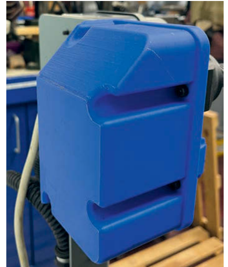
Photo 36: Electrical housing installed on the control column.
