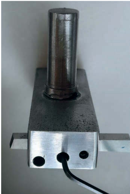
Photo 3: Three holes drilled and taped for 4 mm grub screws.
