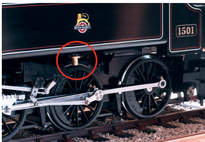
Photo 10: Location of water balance pipe.
