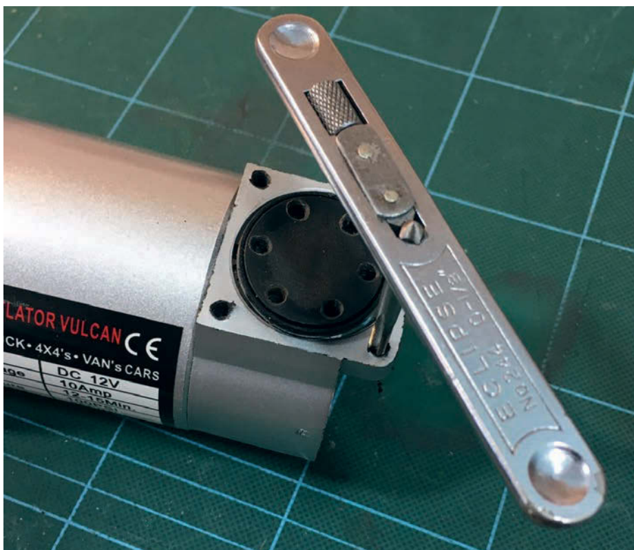
Photo 13: To keep this finely crafted compressor from possibly blowing its own head off, here's a snap of the wood screw holes being retapped M4 for proper bolts that will actually hold the cylinder head in place. The black disc with six holes is the piston.
