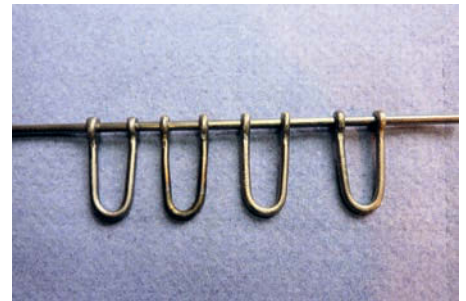
Photo 7: Links with holes lined up using 3/32" rod.
