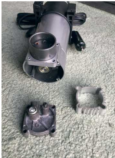
Photo 14: With the head removed and holes tapped, I popped the cylinder back on for this shot, but the end plate has now been removed, revealing the crankshaft end and conrod.
