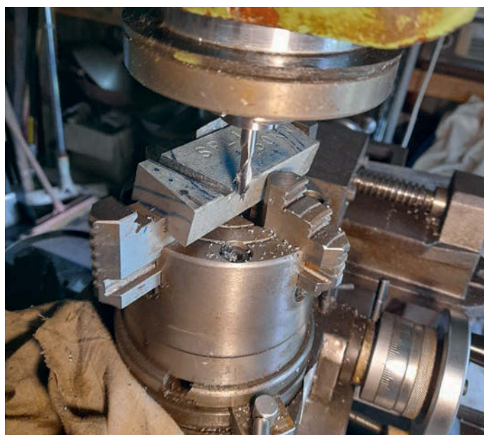
Photo 2: Milling the slot.
