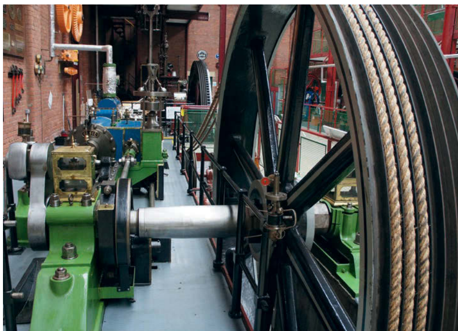
Photo 27: Wasp engine crankshaft and flywheel. Ropes from the flywheel pulley operated line shafts powering machinery in the mill.
