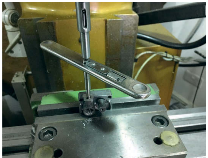
Photo 20: And here's the tapping operation under way.
