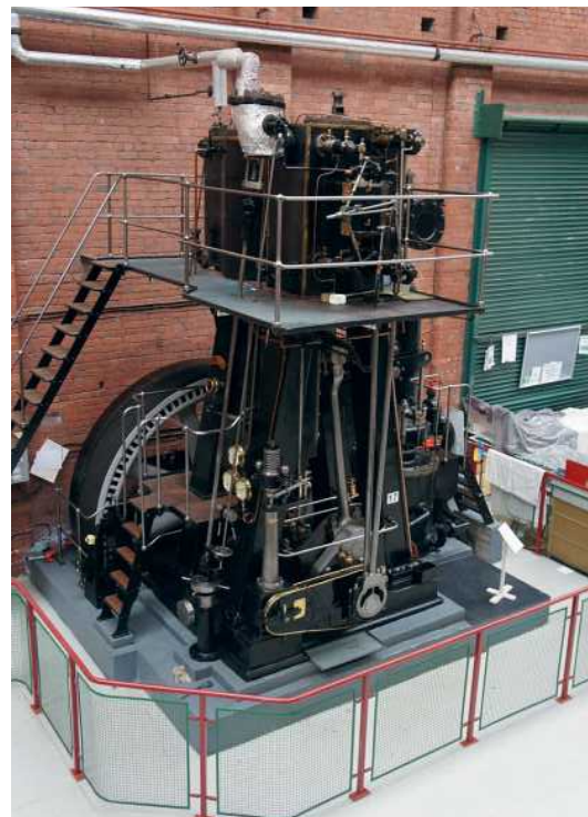
Photo 18: The two cylinder vertical compound built by Scott and Hodgson of Guide Bridge for the Diamond Rope Works around 1914-15.
