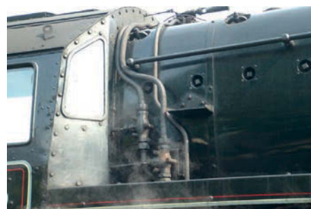
Photo 308: Valves on right side of firebox.
