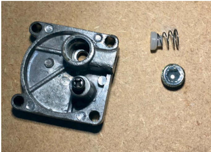
Photo 17: This is the top surface of the Cylinder head, die cast in Mazak alloy.
