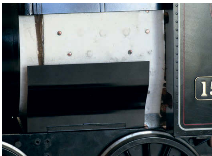
Photo 8: Fire box heat deflector.
