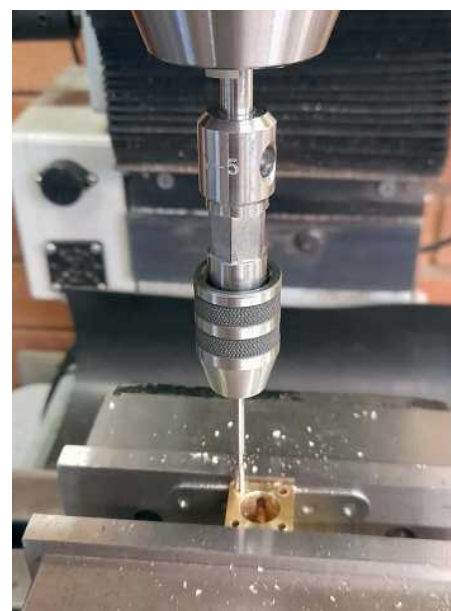
Photo 16: Tapping holes in the ends of a cylinder.
