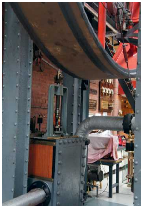
Photo 16: The flywheel pulley drove mill machinery via a leather belt to line shafts.
