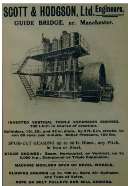
Photo 19: Advertisement for one of Scott and Hodgson's triple expansion engines. These were much used in ships but some found their way to cotton mills as they took up less space than the horizontal engines generally used.
