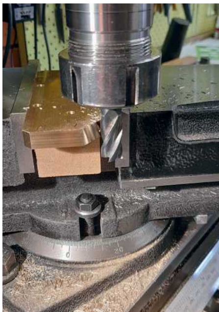
Photo 7: Milling the edges of the manifold.
