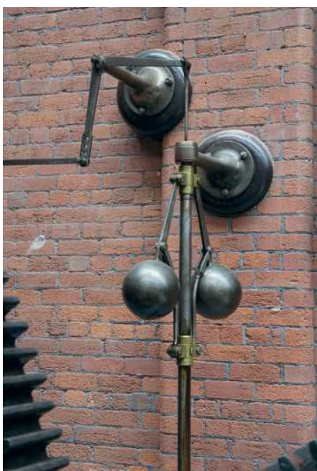
Photo 5: Basic Watt type governor on the Crossfield engine
