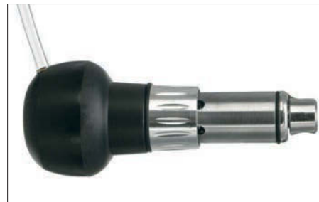
Photo 5: This is a typical air powered engraving handpiece, with its bulbous palm handle, fluted locknut securing the shaft with radial air holes, and a collet at the front, ready to accept a graver.
