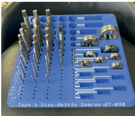
Photo 26: Metric tap and die storage block.
