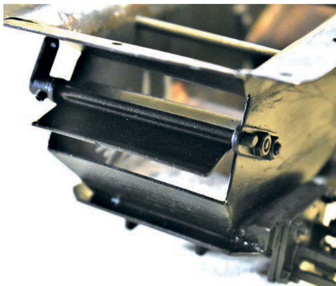
Photo 304: Front damper door; photo - John Arrowsmith.
