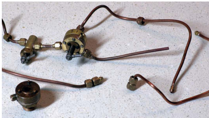
Photo 8: Back head and smokebox pipework.
