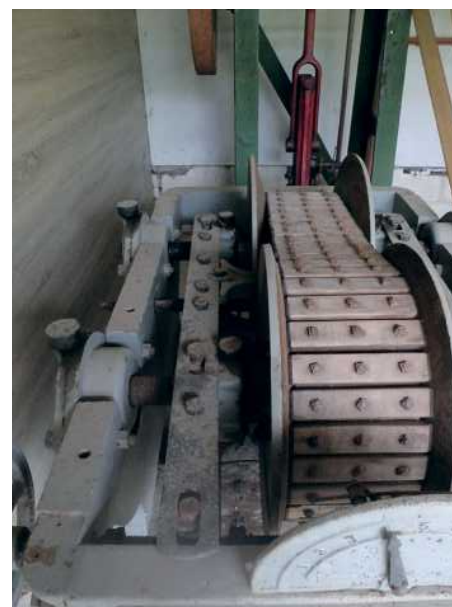
Photo 3: Variable speed transmission at Wortley Top Forge).
