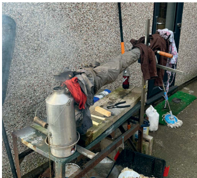
Photo 10: An improvised wood steamer.
