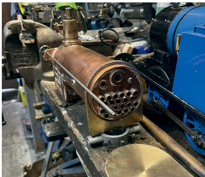
Photo 8: Routing the reverser rod.
