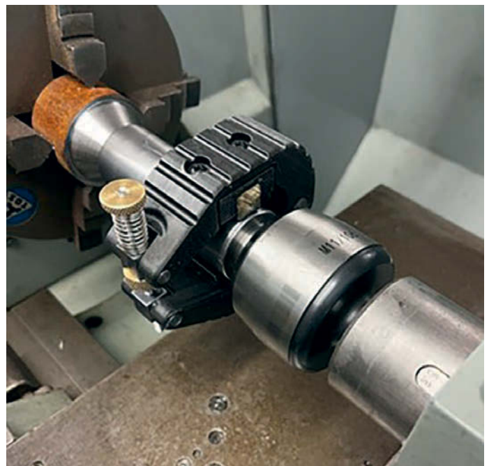
Photo 18: The 3D printed external hone in use.
