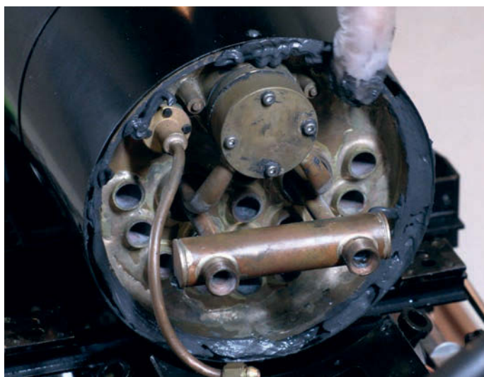
Photo 12: A very messy job with Fireweld.
