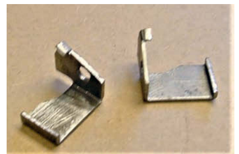
Photo 300: Grate locks from 16 swg sheet.
