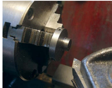
Photo 9: Using a mandrel to machine the sawn faces of the two outer eccentrics.
