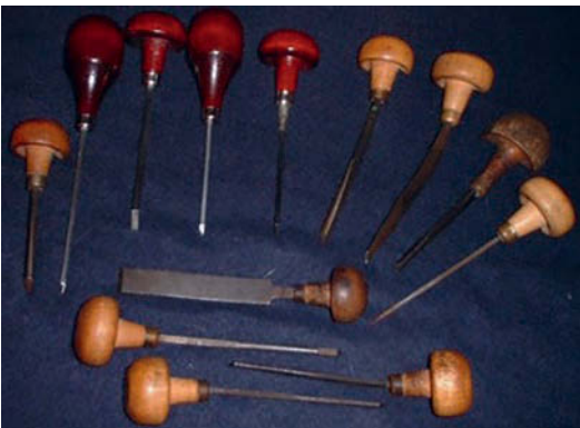
Photo 3: An array of traditional push engraving Gravers. This selection would cover the majority of the shapes and widths of line that an engraver would require to produce his work.
