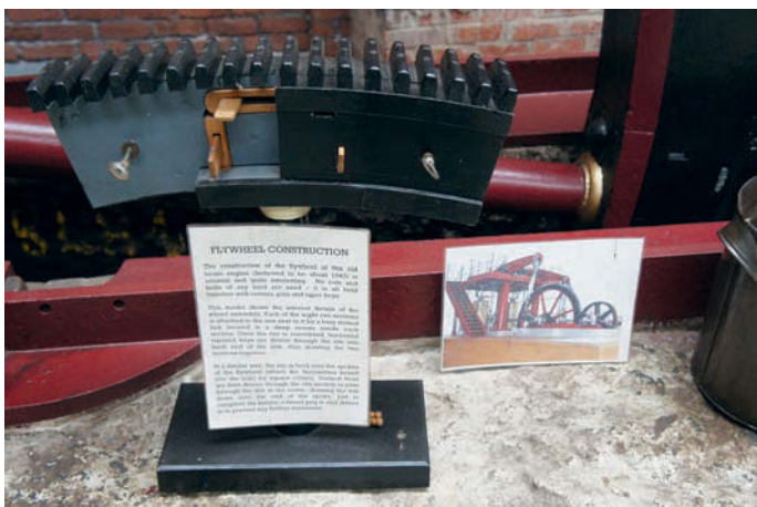
Photo 6: Large flywheels were not cast in one piece but assembled from parts with the rim keyed and cottered together. Shown in one of several excellent displays in the museum.
