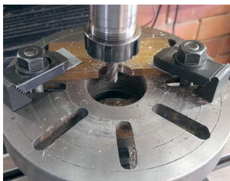
Photo 6: Milling the manifold circular cut-out. Faceplate mounted on rotary table.
