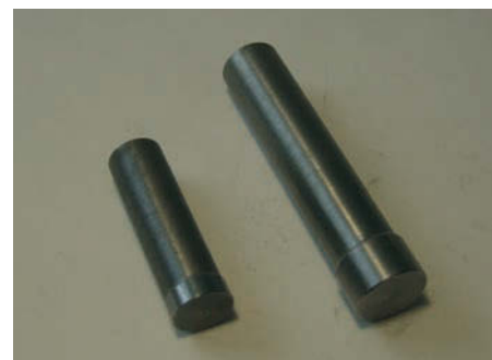
Photo 6: The two gauges for the boring operations.
