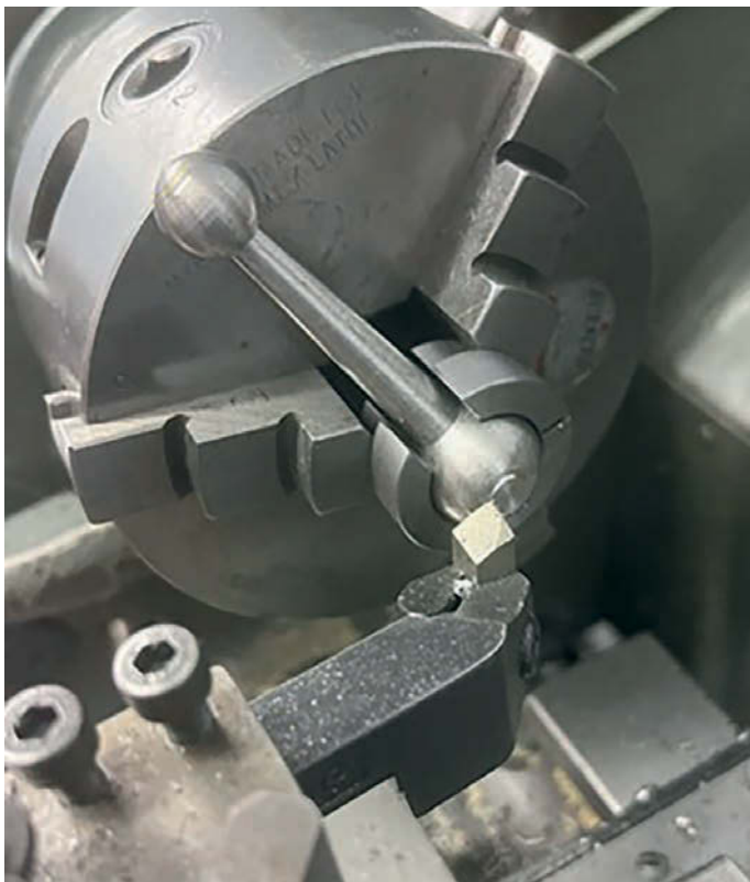
Photo 13: Machining the flat on one of my larger ball-ended handles.
