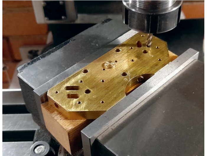
Photo 9: Milling slots in the manifold.
