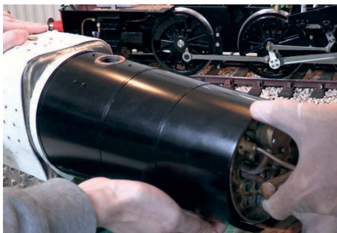
Photo 5: Fitting the wrapper.
