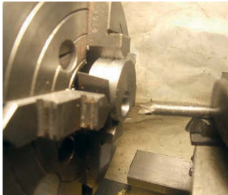
Photo 8: Drilling and machining the eccentric bores.
