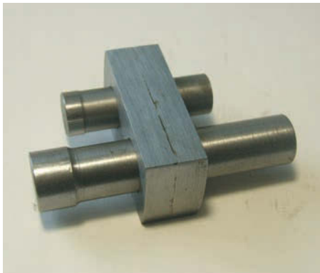
Photo 7: A bored pair of crank webs with their gauges.
