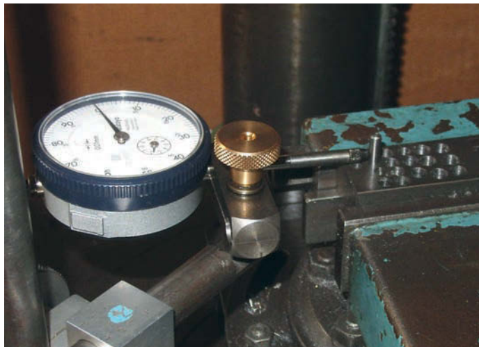
Photo 2: Testing the fit of a pin in a reamed hole.
