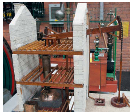
Photo 2: Newcomen engine model. The first practical engine design to use steam - which was condensed to make a vacuum powering the piston. It was extensively used in mine pumping but could not be used for rotary motion and hence was not useful for textile mills.
