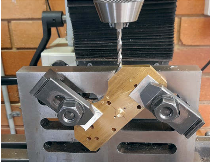
Photo 8: Drilling internal passages in the manifold.
