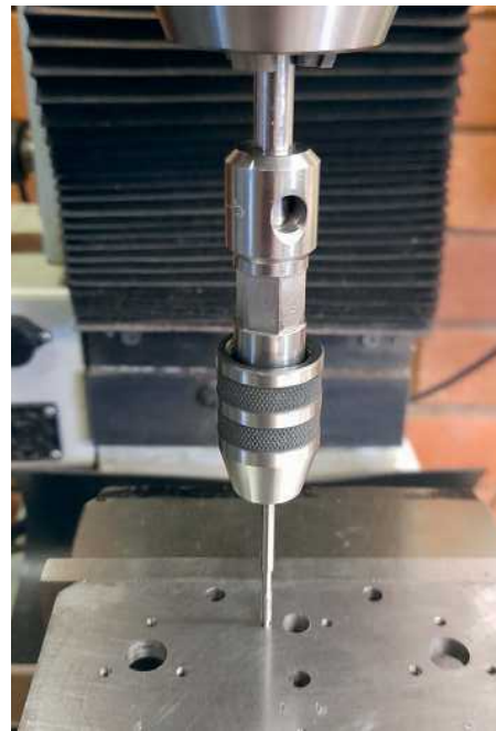
Photo 5: Tapping holes in the rear endplate using a DIY tapping guide.
