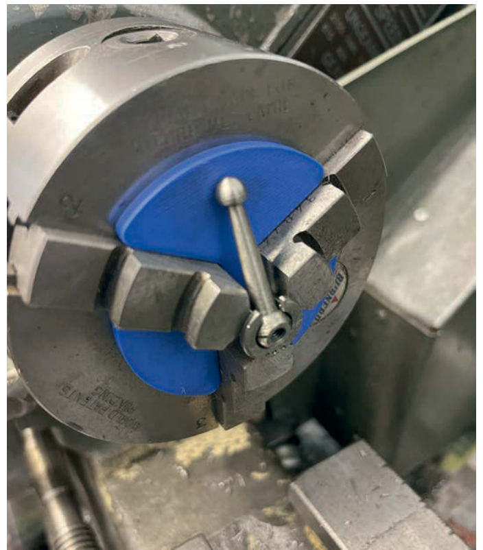
Photo 14: The special spider in use machining a flat on an M4 ball handle.
