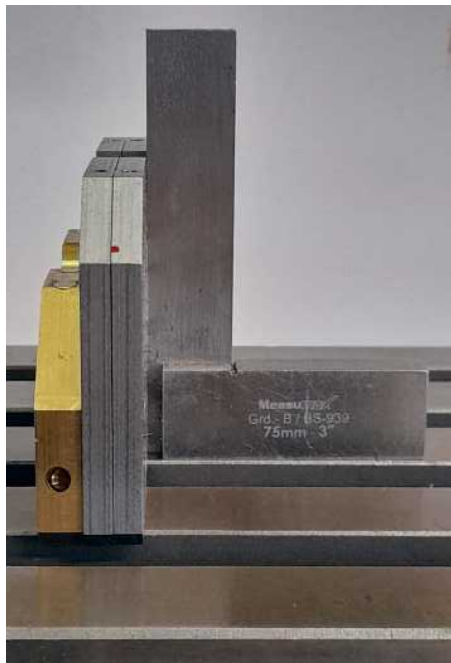
Photo 3: Squaring the plates for clamping.
