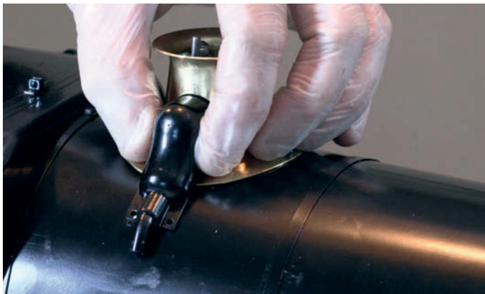
Photo 7: Test-fit of the top feed pipe cover.
