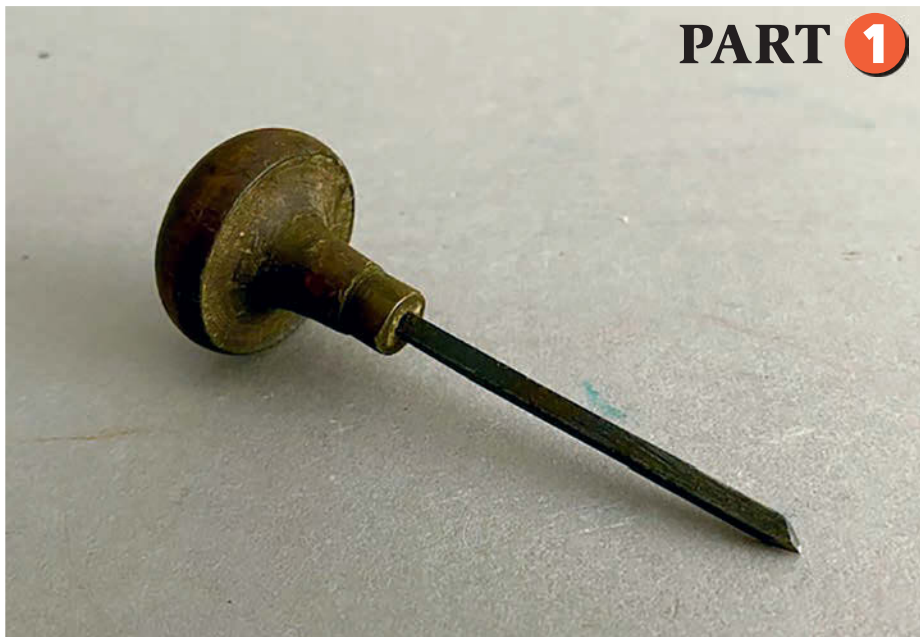
Photo 1: A typical palm-pushed engraver's push Graver.
