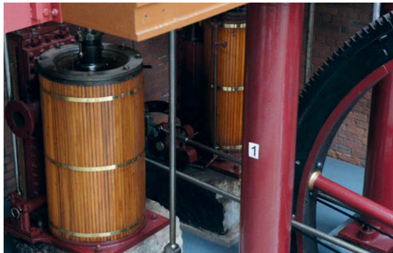
Photo 4: Crossfield engine cylinders lagged with wood. The high-pressure cylinder is on the right.
