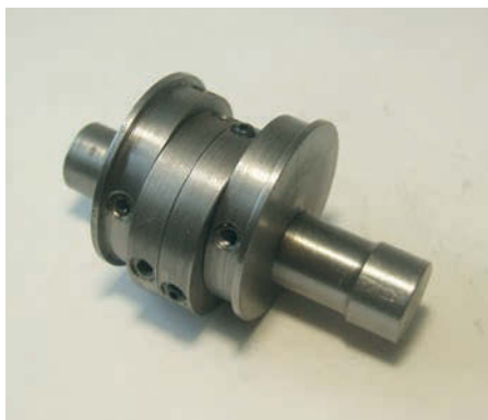
Photo 11: The four completed sheaves on their shaft.
