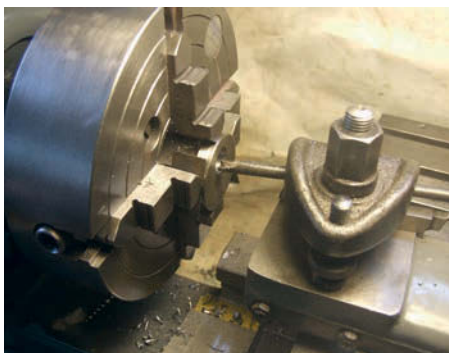
Photo 10: Holding the shouldered pair of eccentrics in the lathe is simpler.
