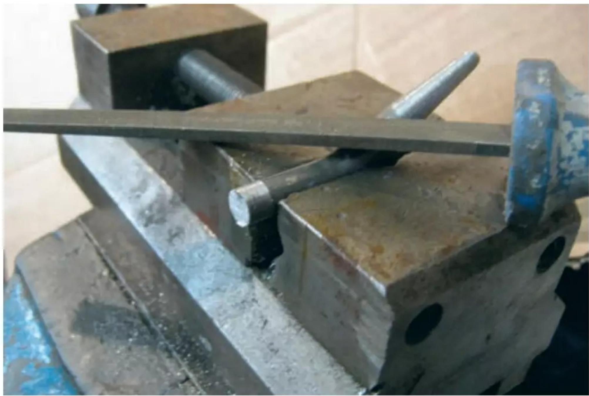
Photo 21: Filing oversize spigot.
