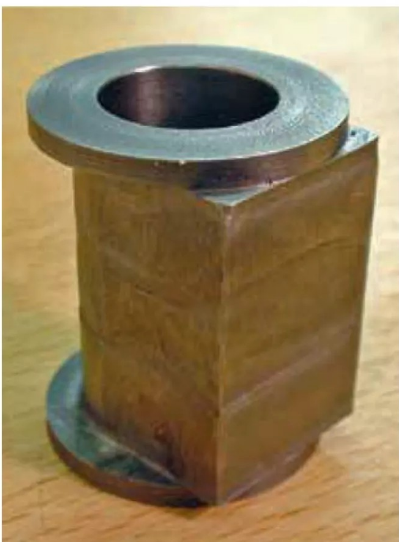
Photo 6: Basic cylinder machined from cast iron bar.
