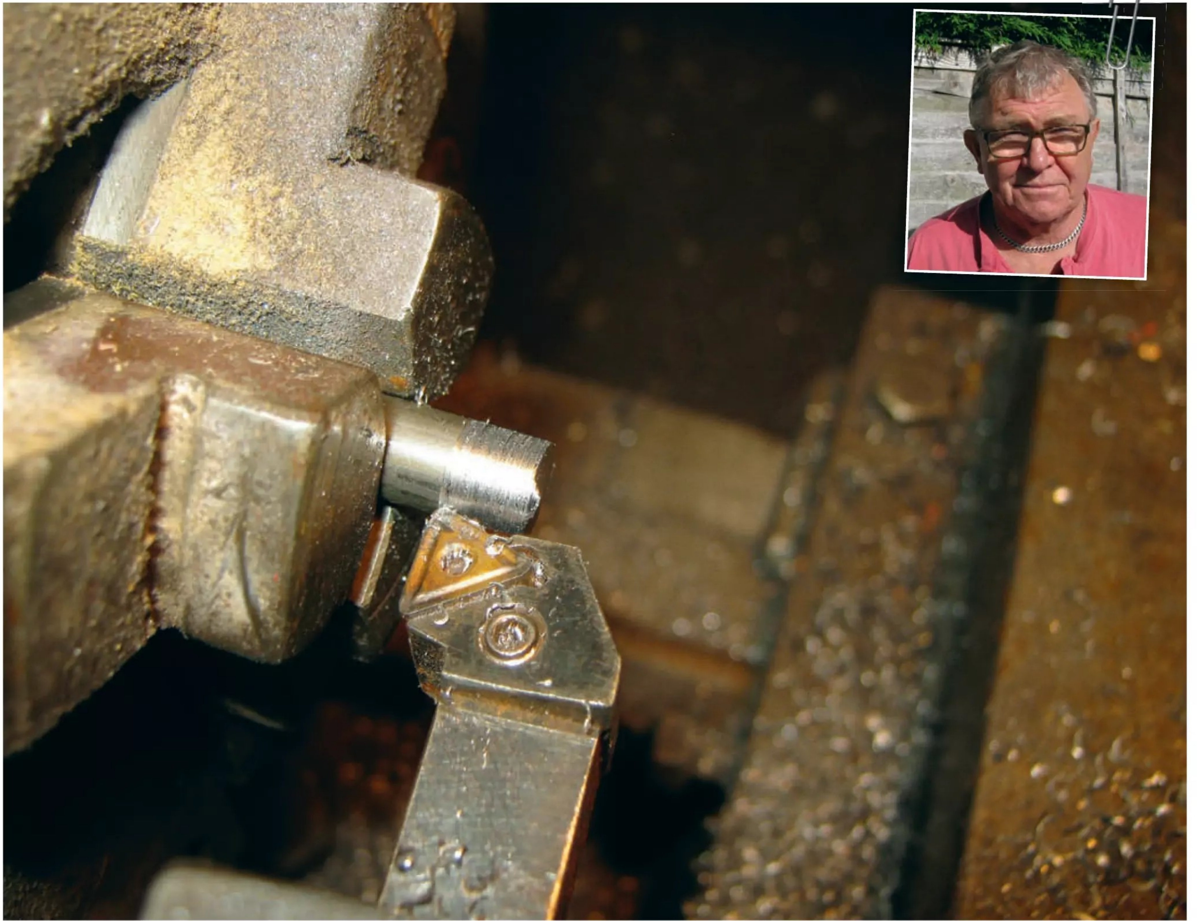
Photo 13: Turning down the opposite end.
