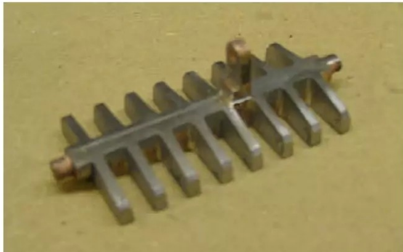
Photo 284: Stainless steel grate casting.
