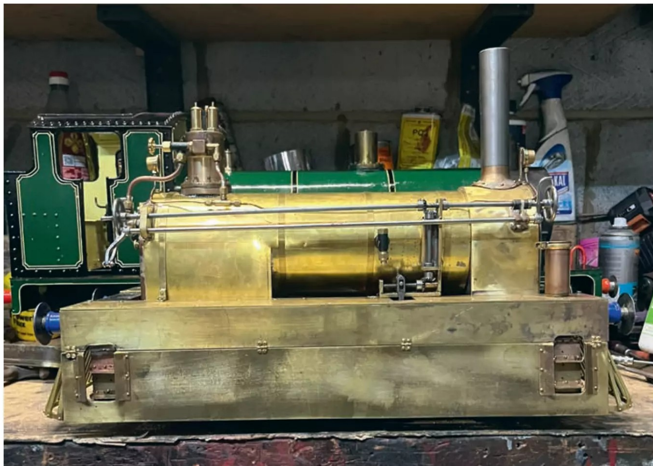
Photo 1: The unpainted chassis and boiler, cutouts for the steps declare it to be a C53.
