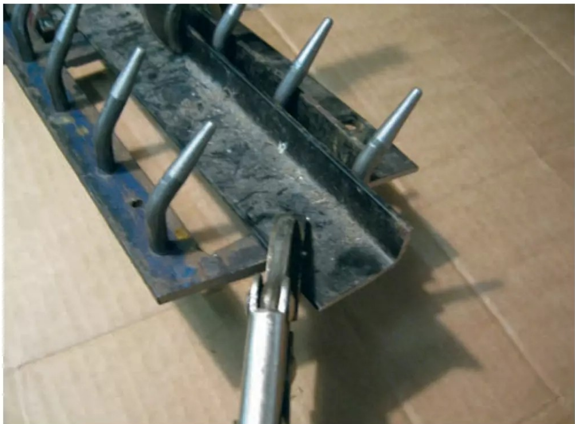
Photo 23: Clamping to keep tines aligned.
