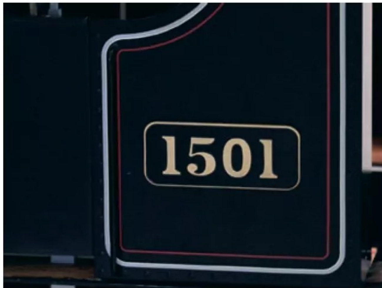
Photo 18: Etched brass running number plate & lining decals.
