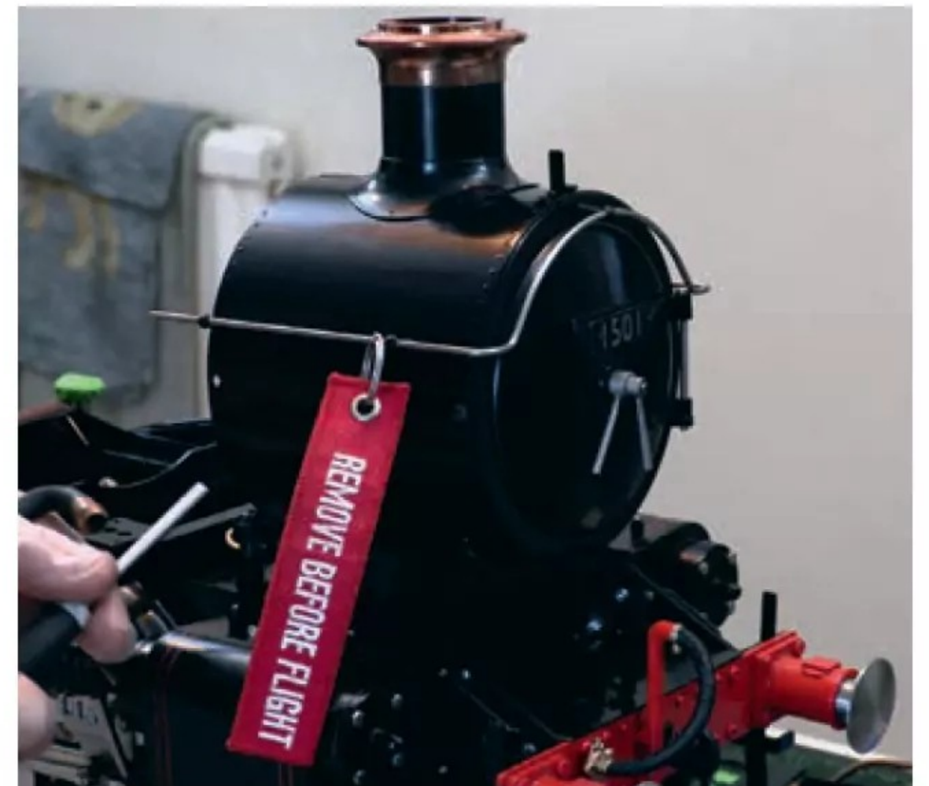
Photo 16: Bolting in the smokebox.
