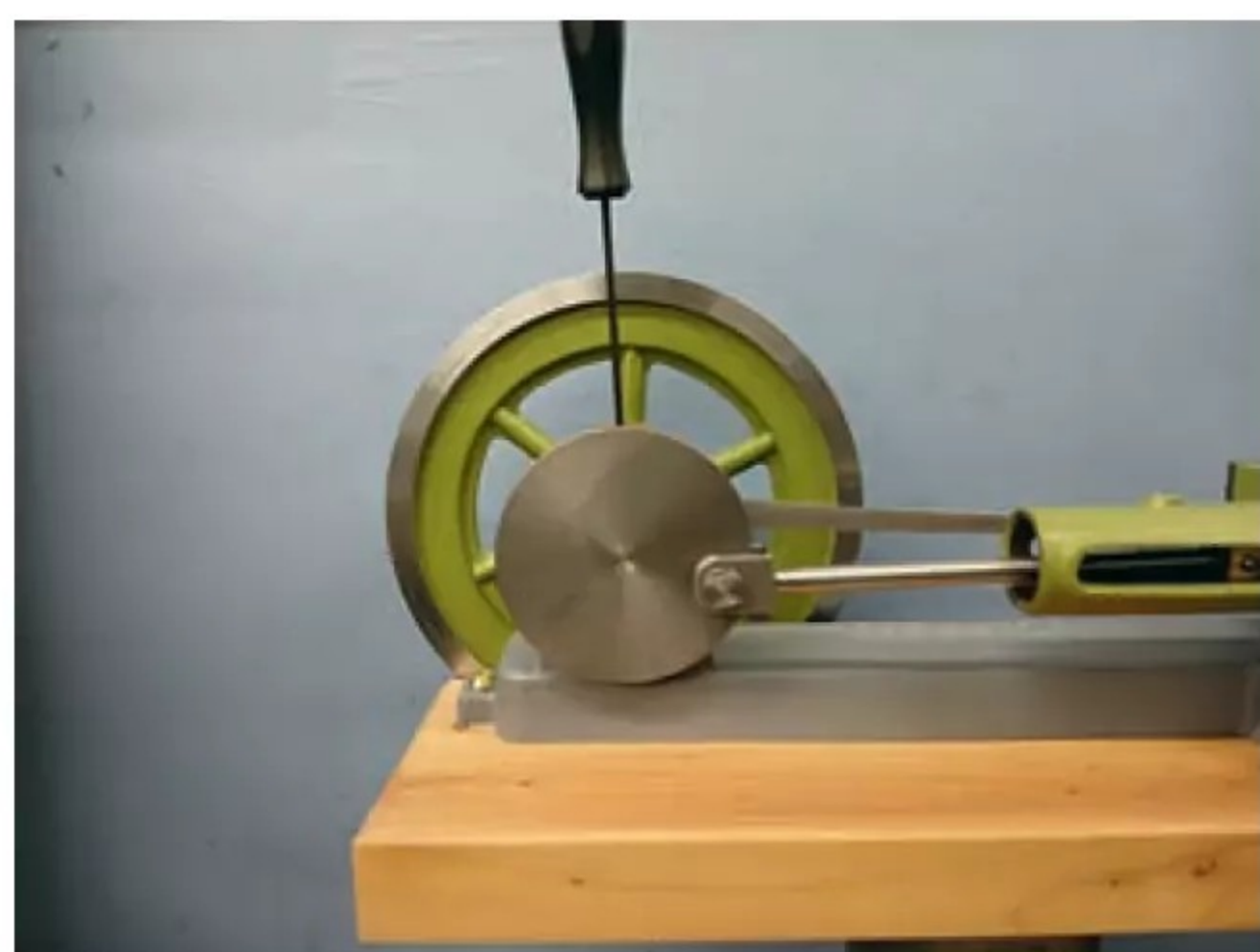
Photo 68: Setting the timing
