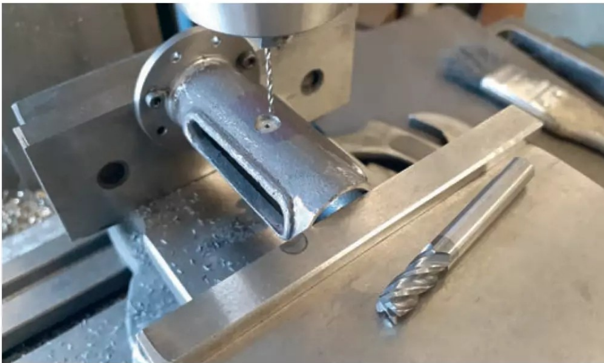
Photo 64: Adding oiler boss to trunkguide
