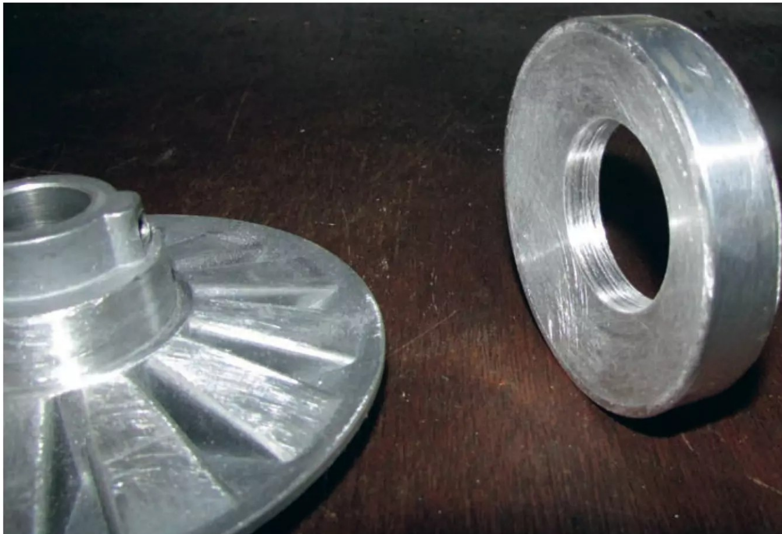
Photo 8: Completed part. Bonding surfaces have been roughened with abrasive to help the bond.
