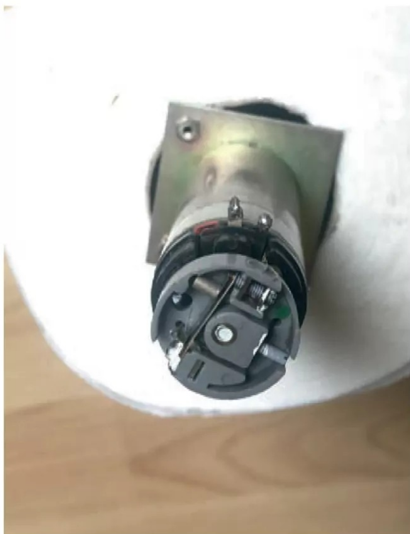
Photo 1: Motor with built-in centrifugal switch.
