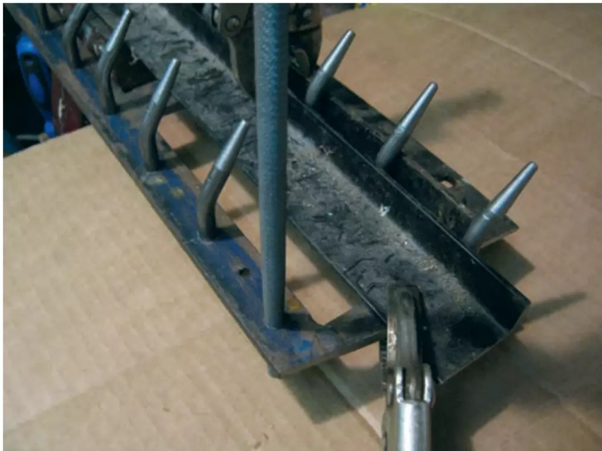
Photo 22: Opening up hole with round file.
