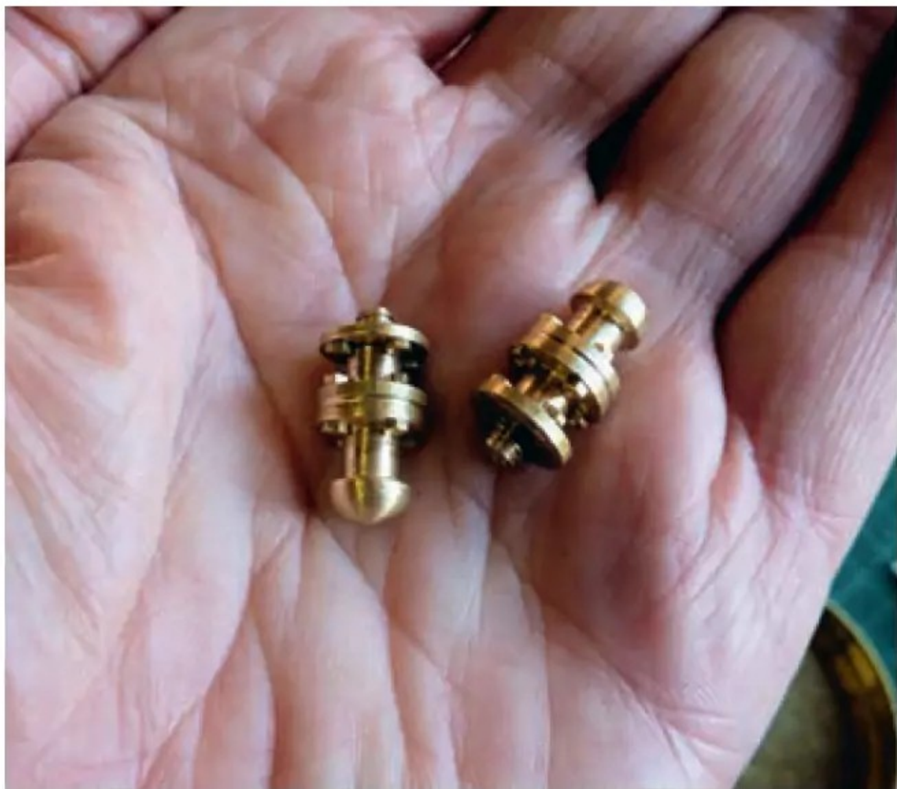
Photo 3: Tank vents in the hand.
