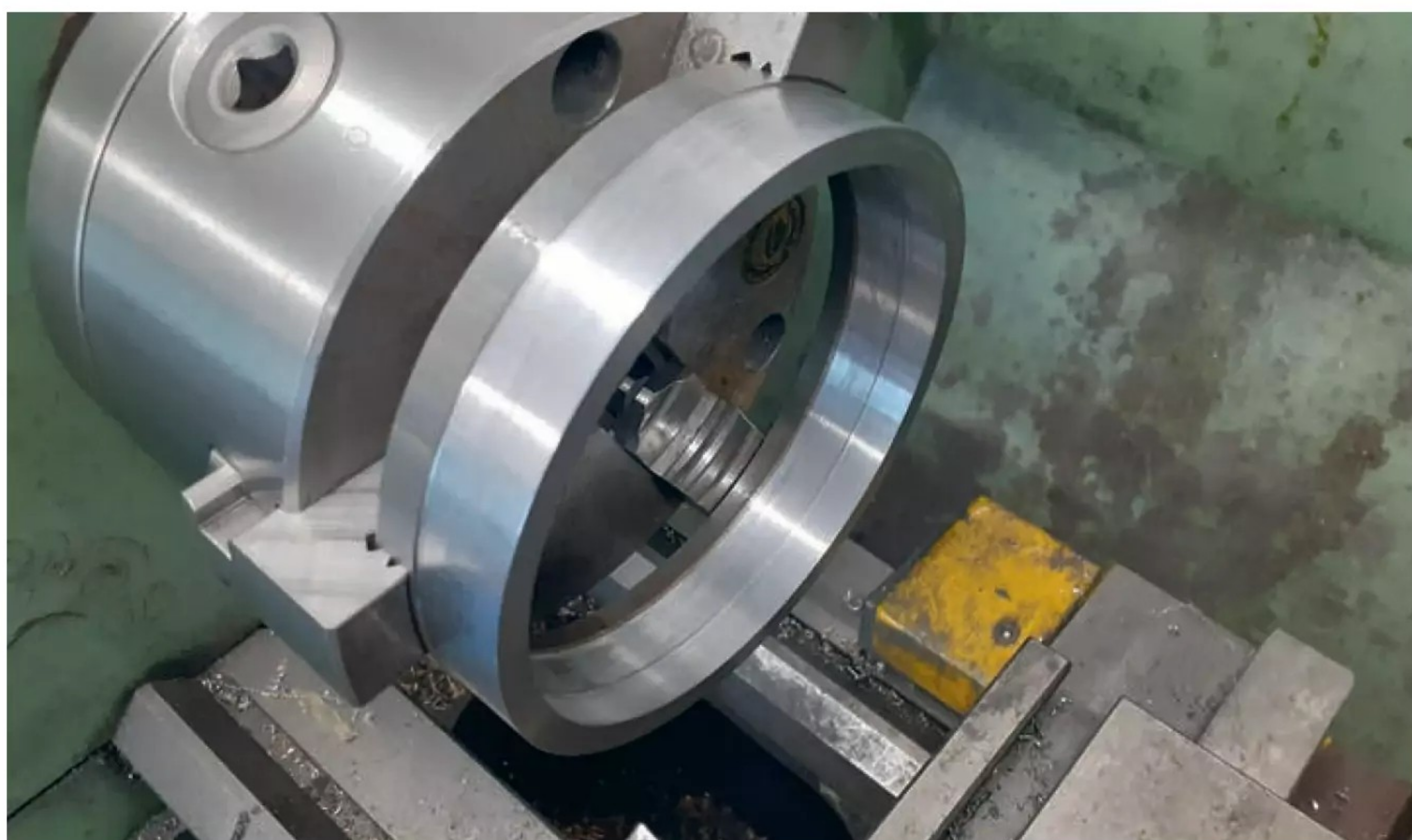
Photo 61: Turning flywheel rim from thick wall tube
