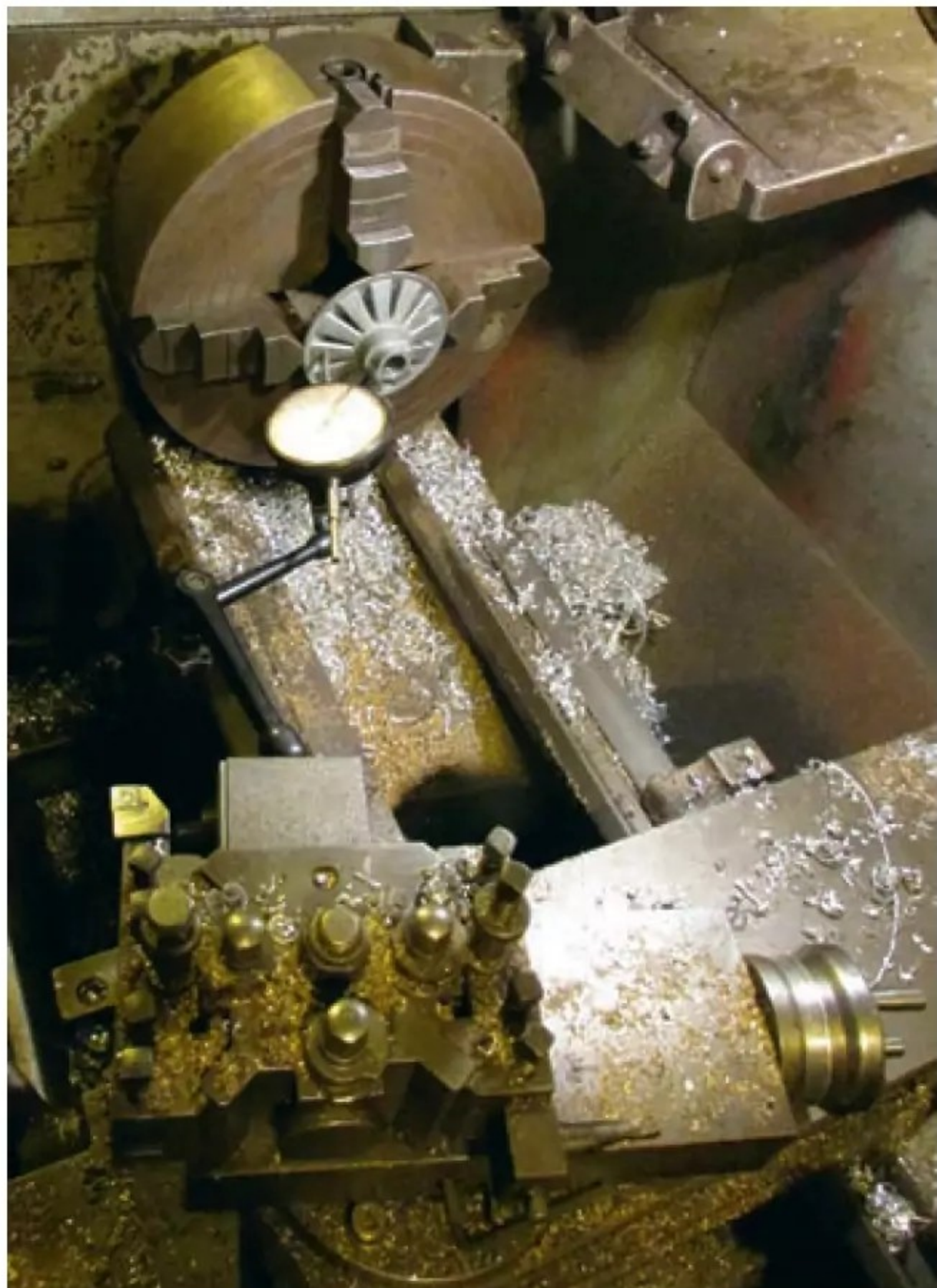
Photo 7: Determining the angle of the spokes by use of the compound slide. The relatively small size of the pulleys may not have been obvious before this picture.
