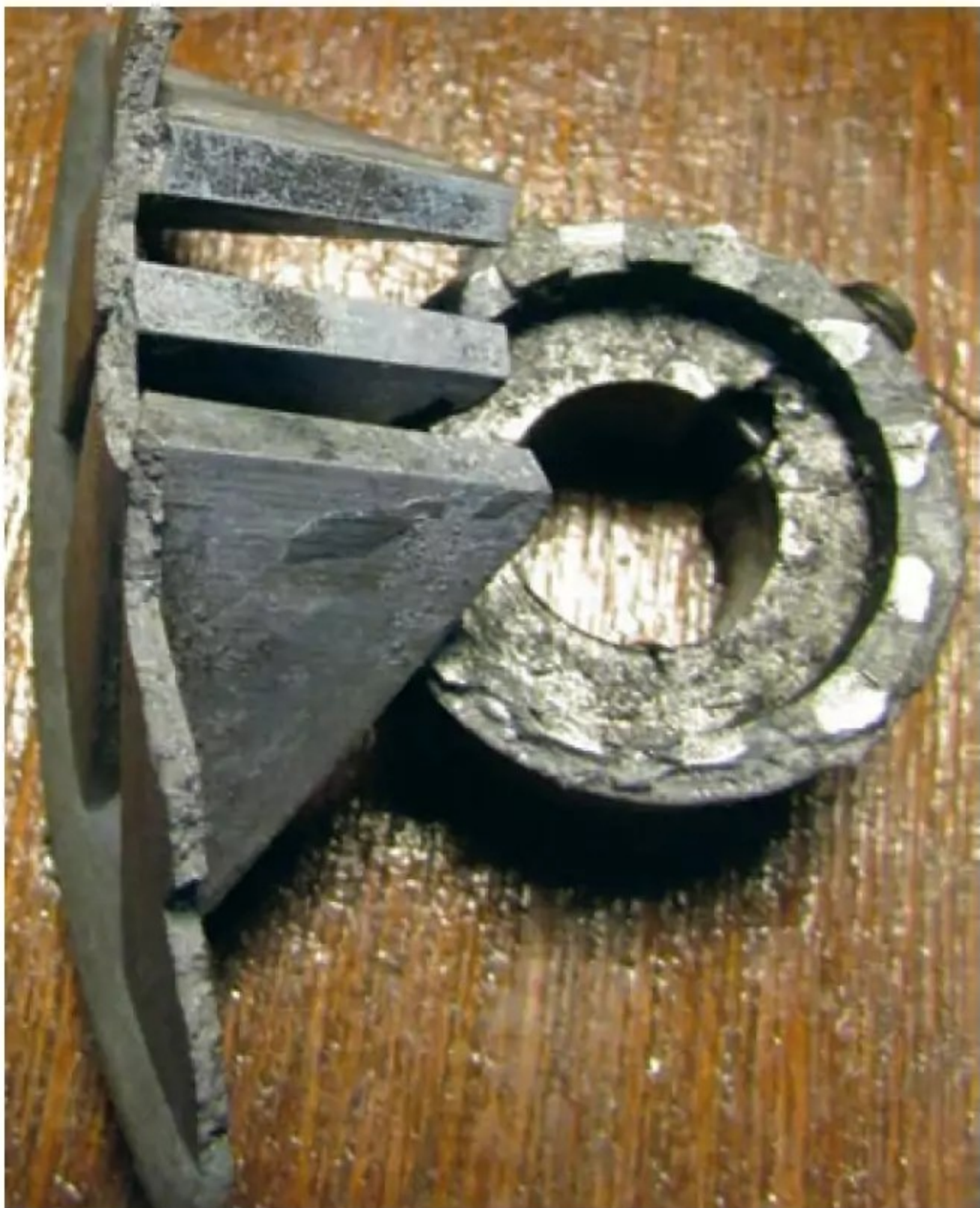
Photo 5: Fracture line visible at left, note the hollow centre – no support for spokes.
