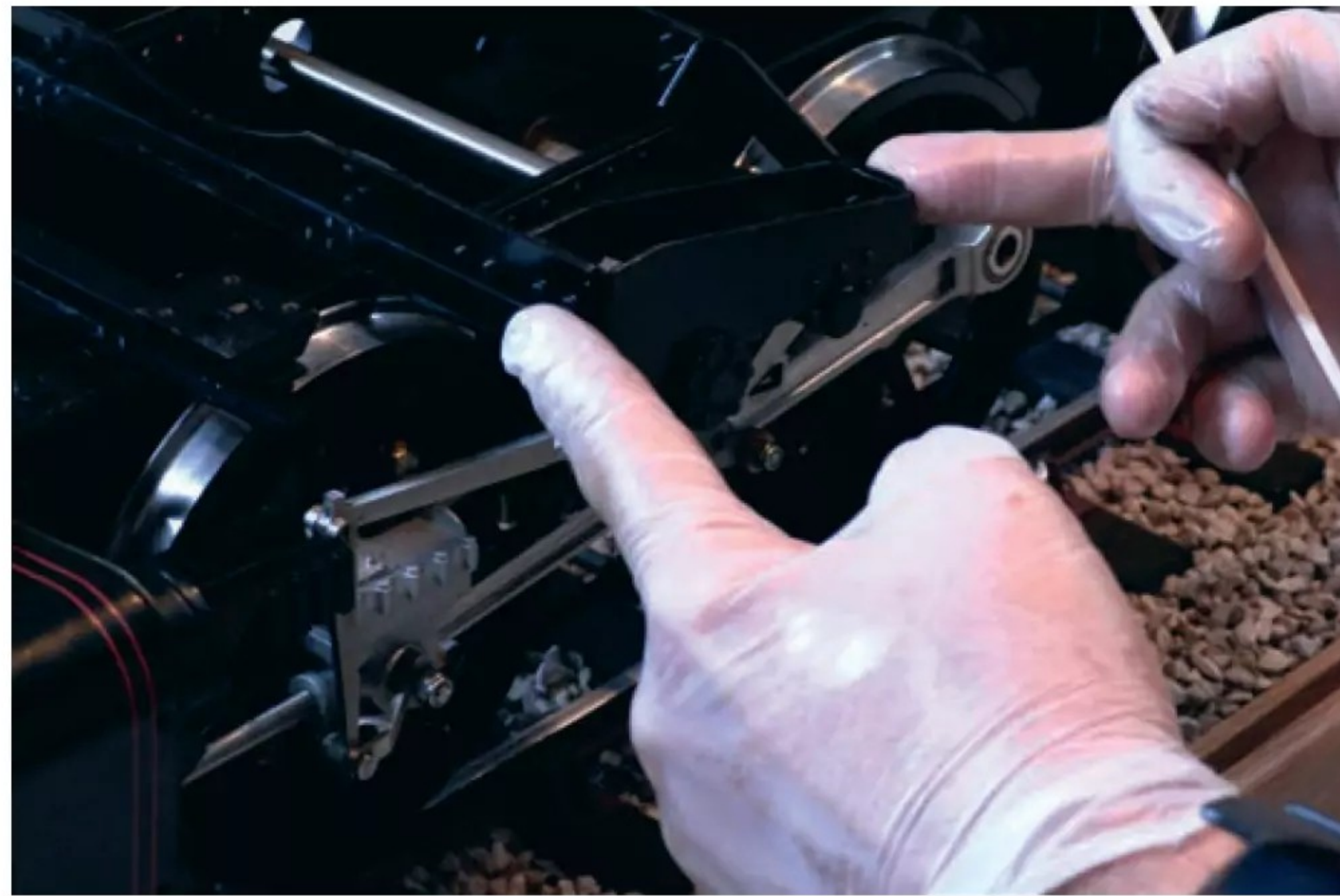
Photo 6: Fitting one of the gear frames.
