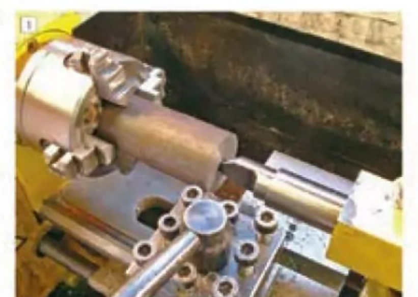
Cast iron bar set up in lathe
