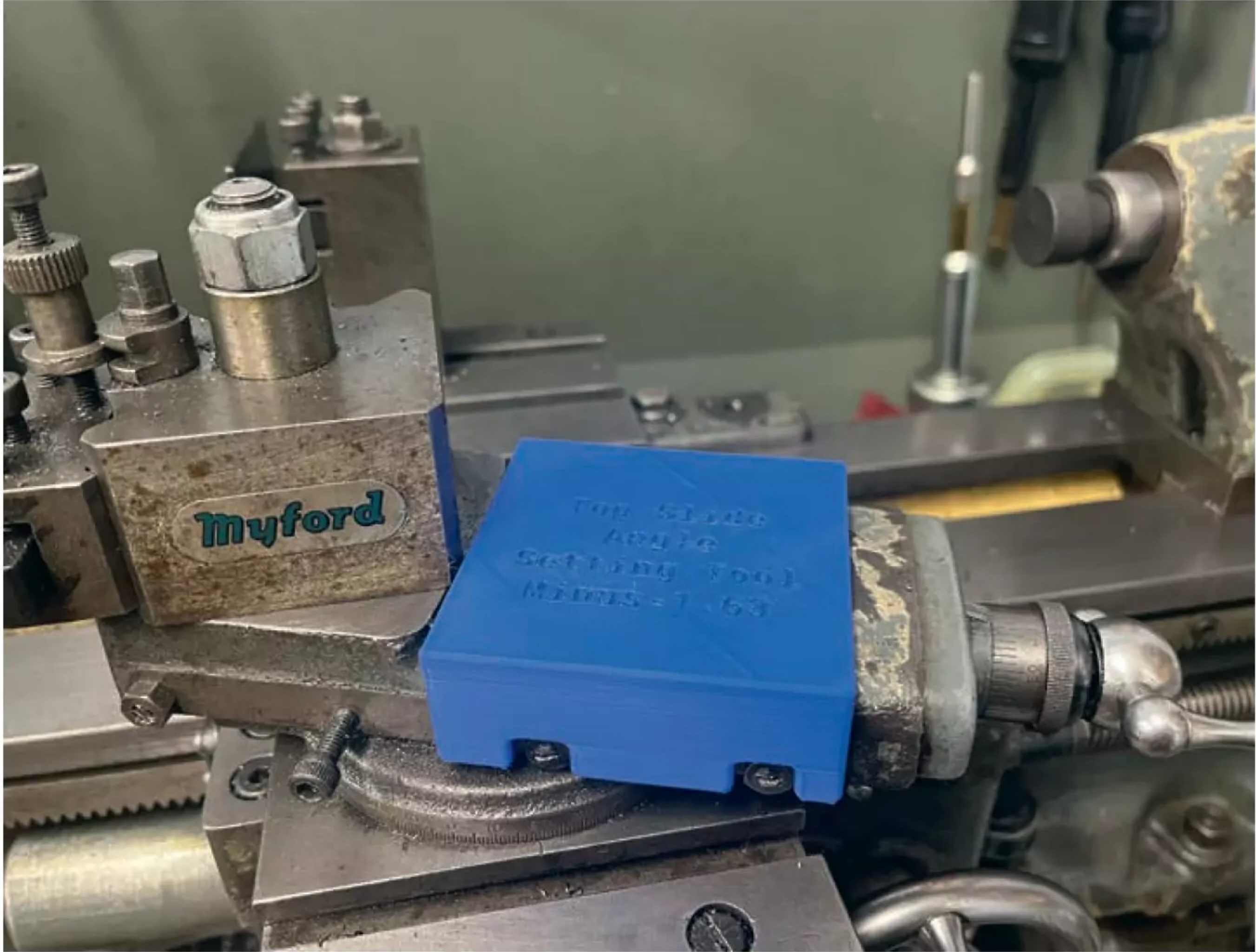
Photo 11: How the aid fits over the gib screws.
