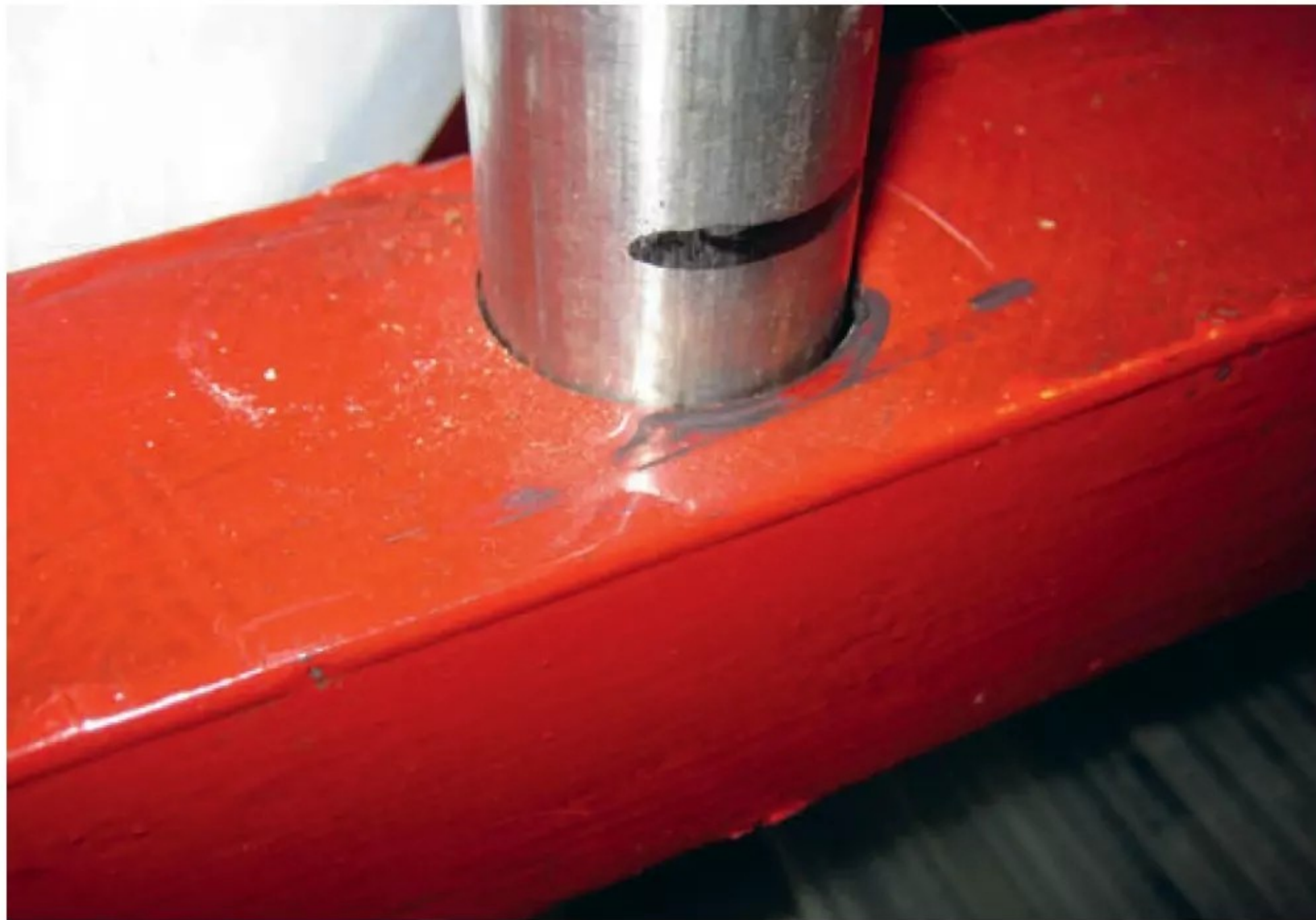
Photo 20: Mark to keep bends the same depth.
