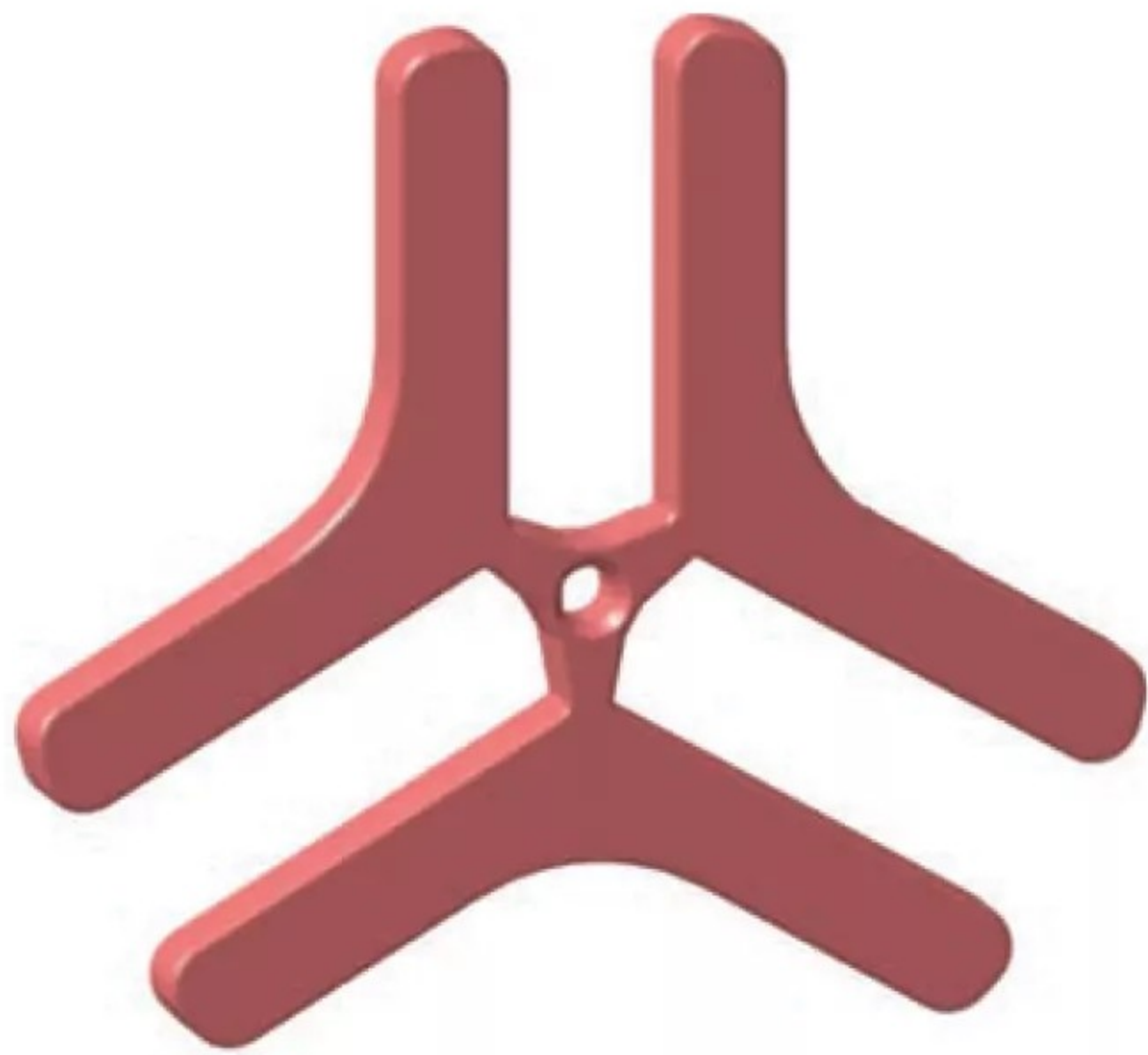
Photo 5: Front view screen grab of a Myford chuck spider.
