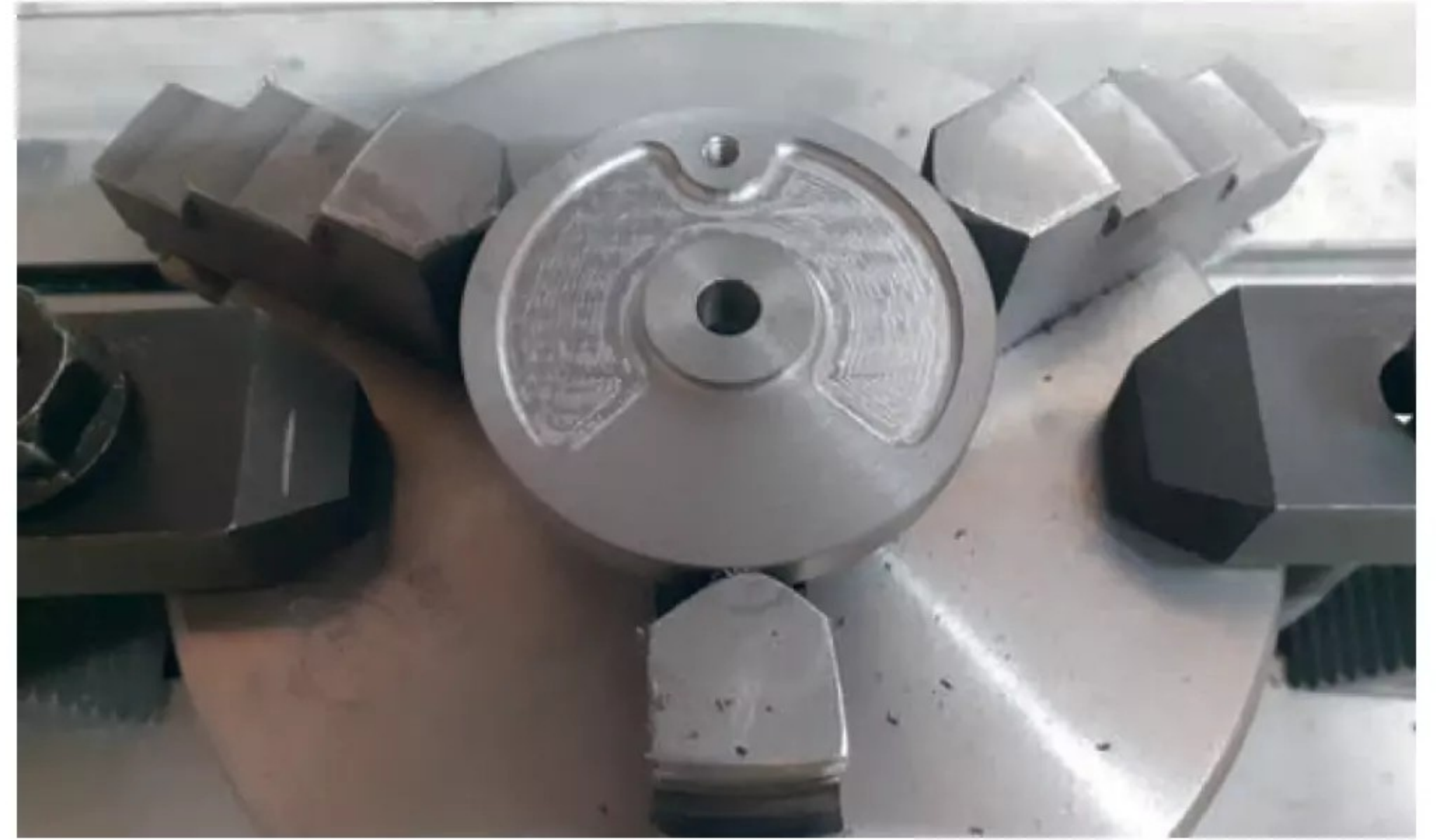
Photo 63: Milling crank disc recess
