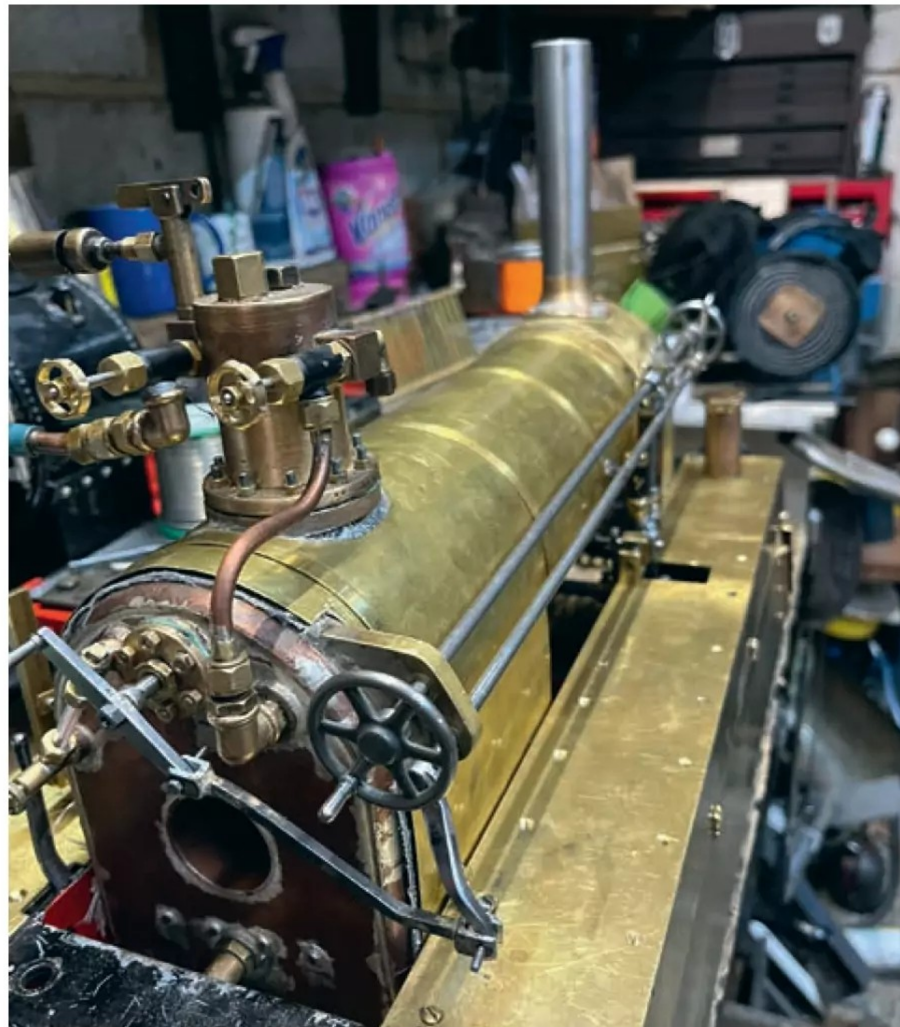
Photo 7: Regulator and reverser rods run the full length of the boiler.
