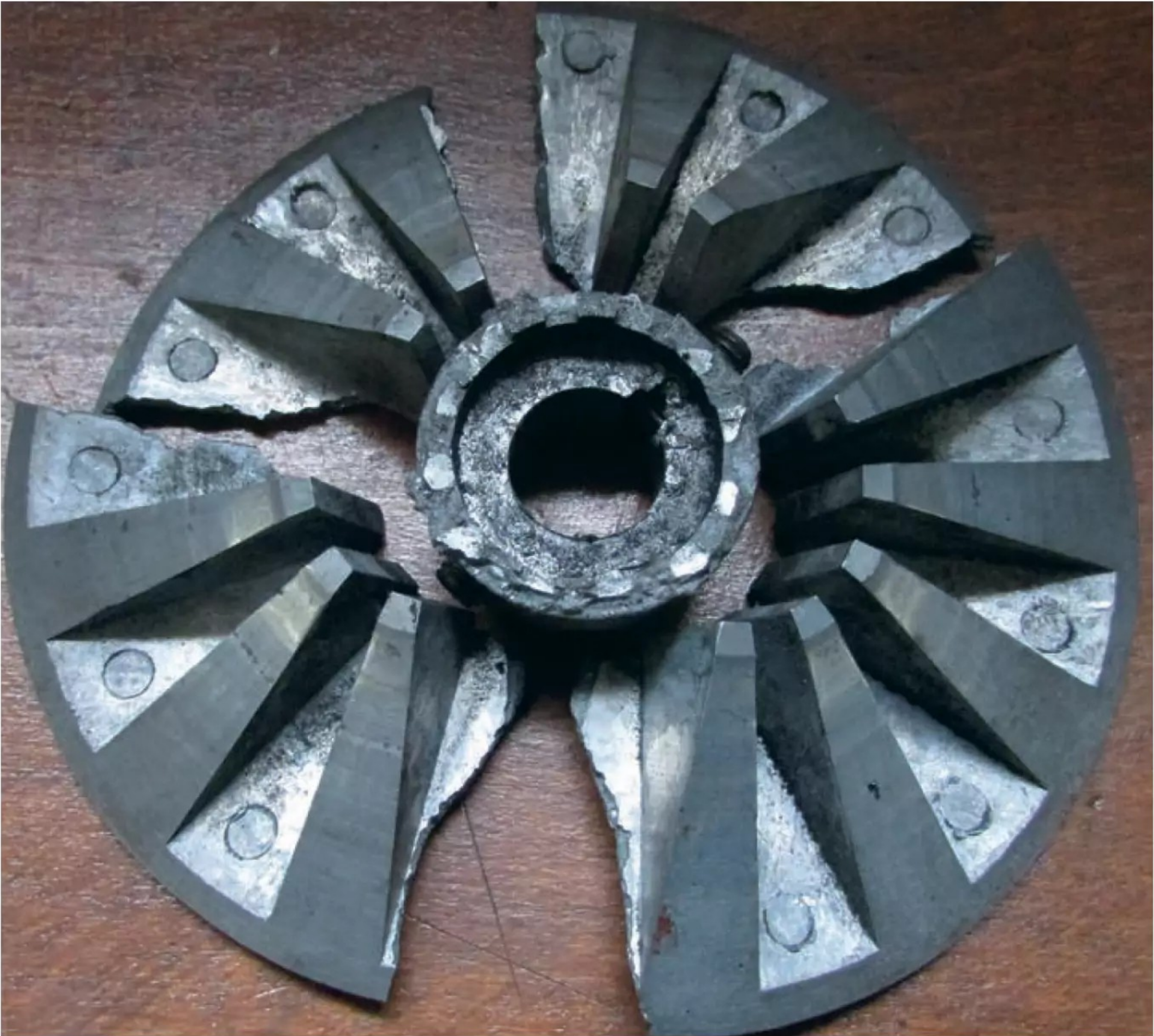
Photo 4: All the parts of the broken pulley half.
