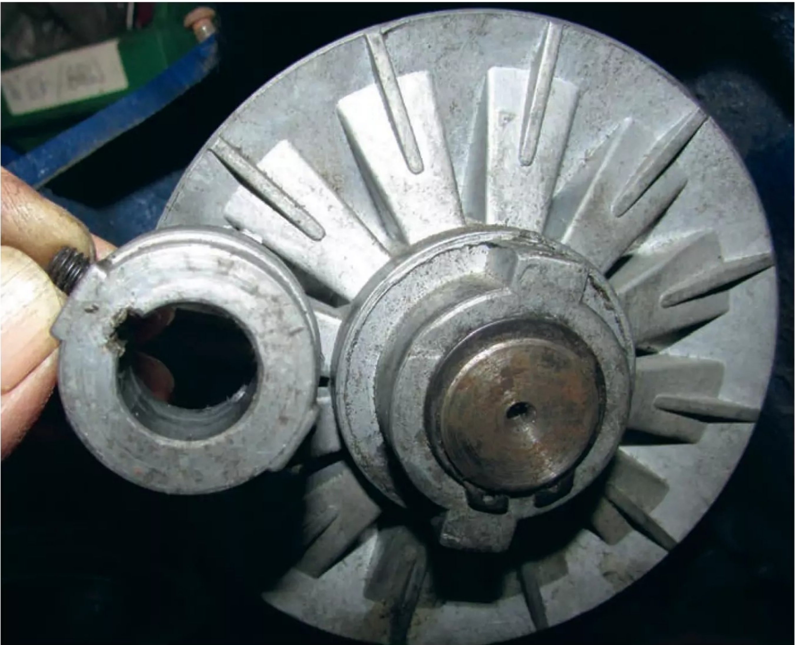
Photo 6: Comparison of the hub diameters of the failed and surviving hollow half pulleys.
