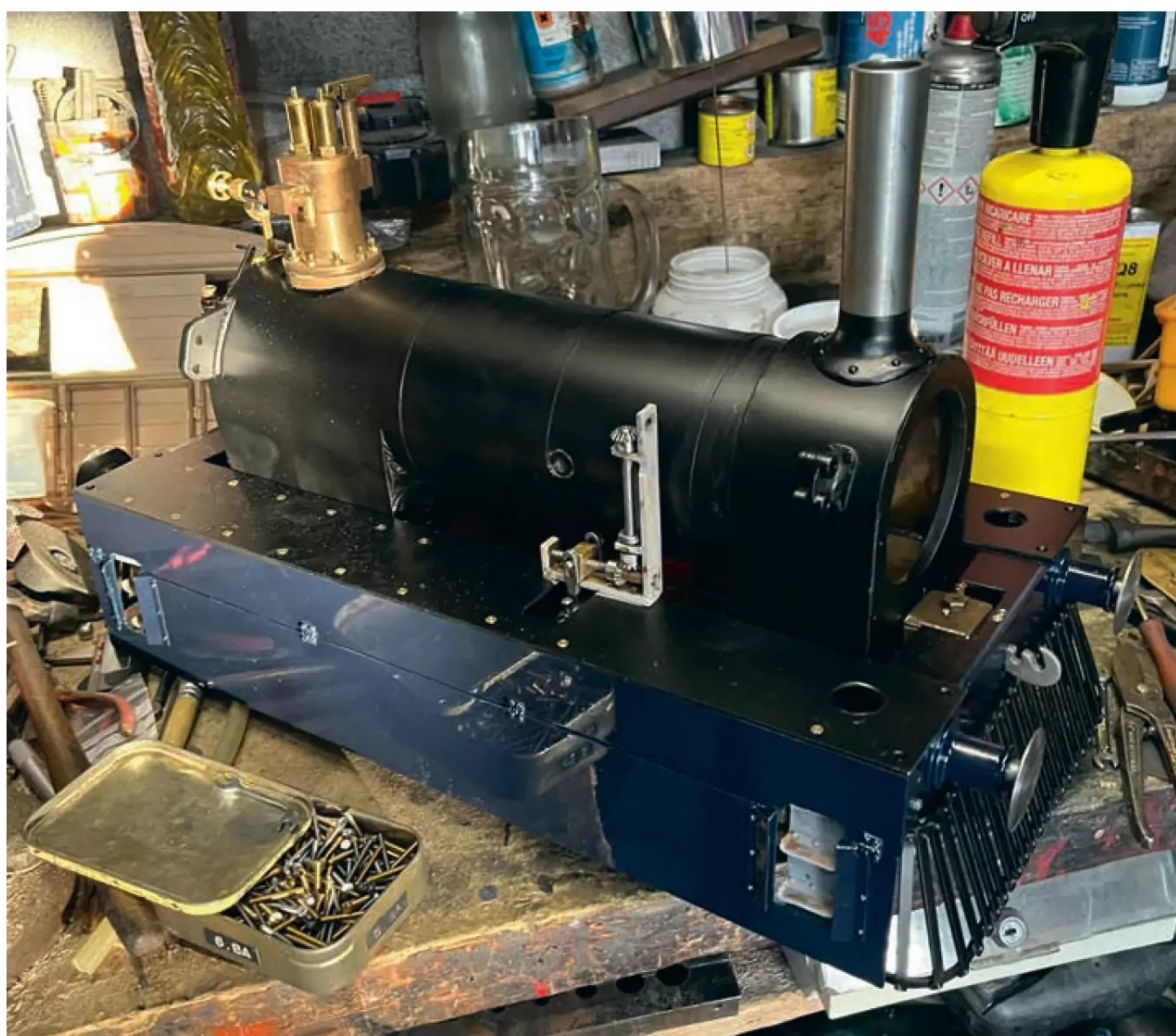
Photo 2: The stretched boiler does not instantly give away its Tich origins.
