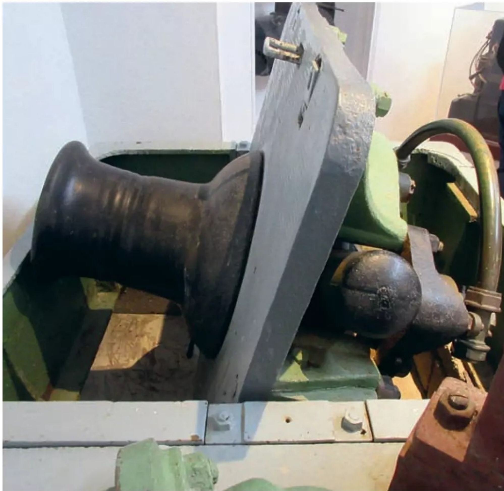
Photo 2: A 1 ton 'turn-over' hydraulic capstan, manufactured 1850.
