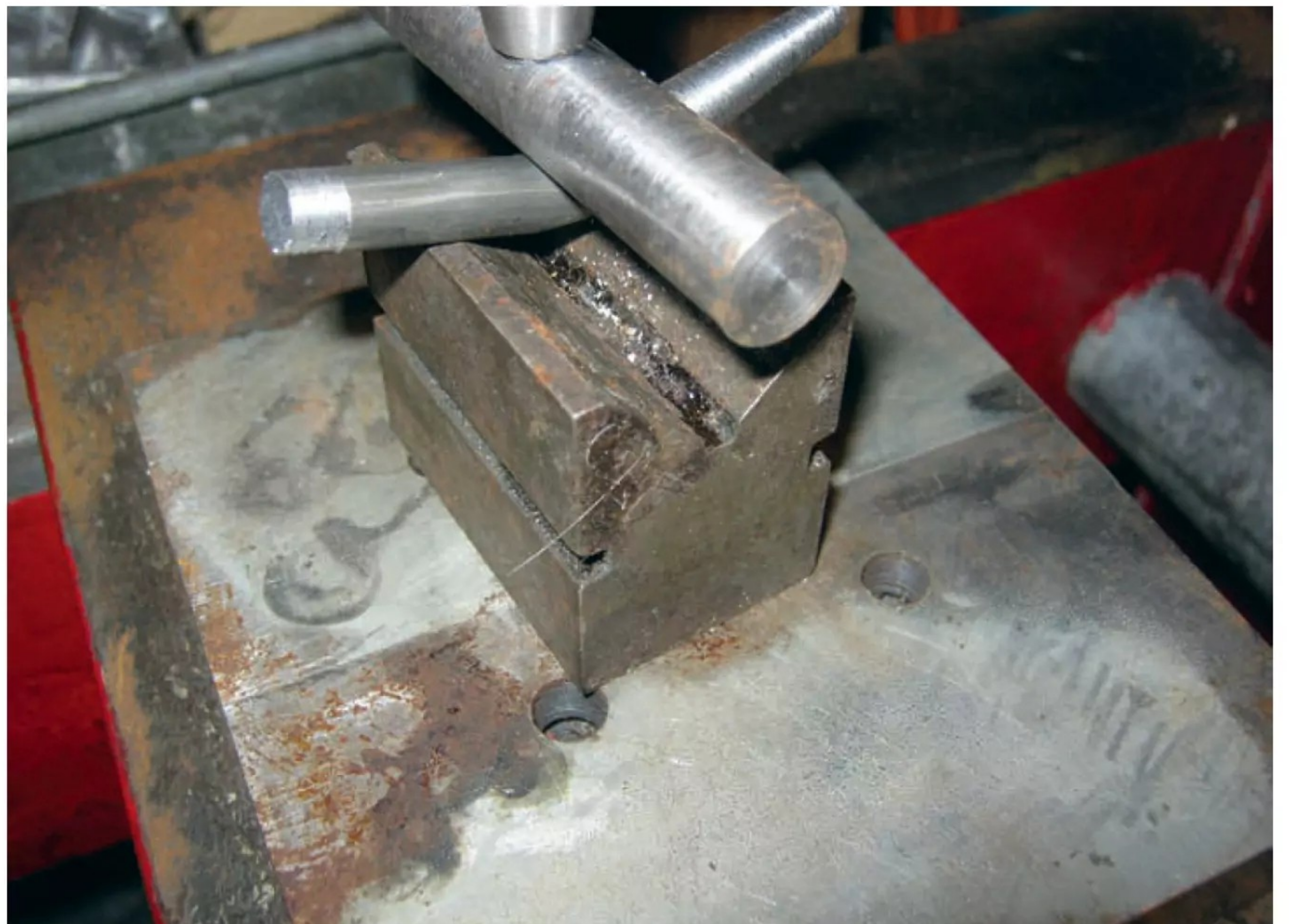
Photo 18: Bending the first tine.
