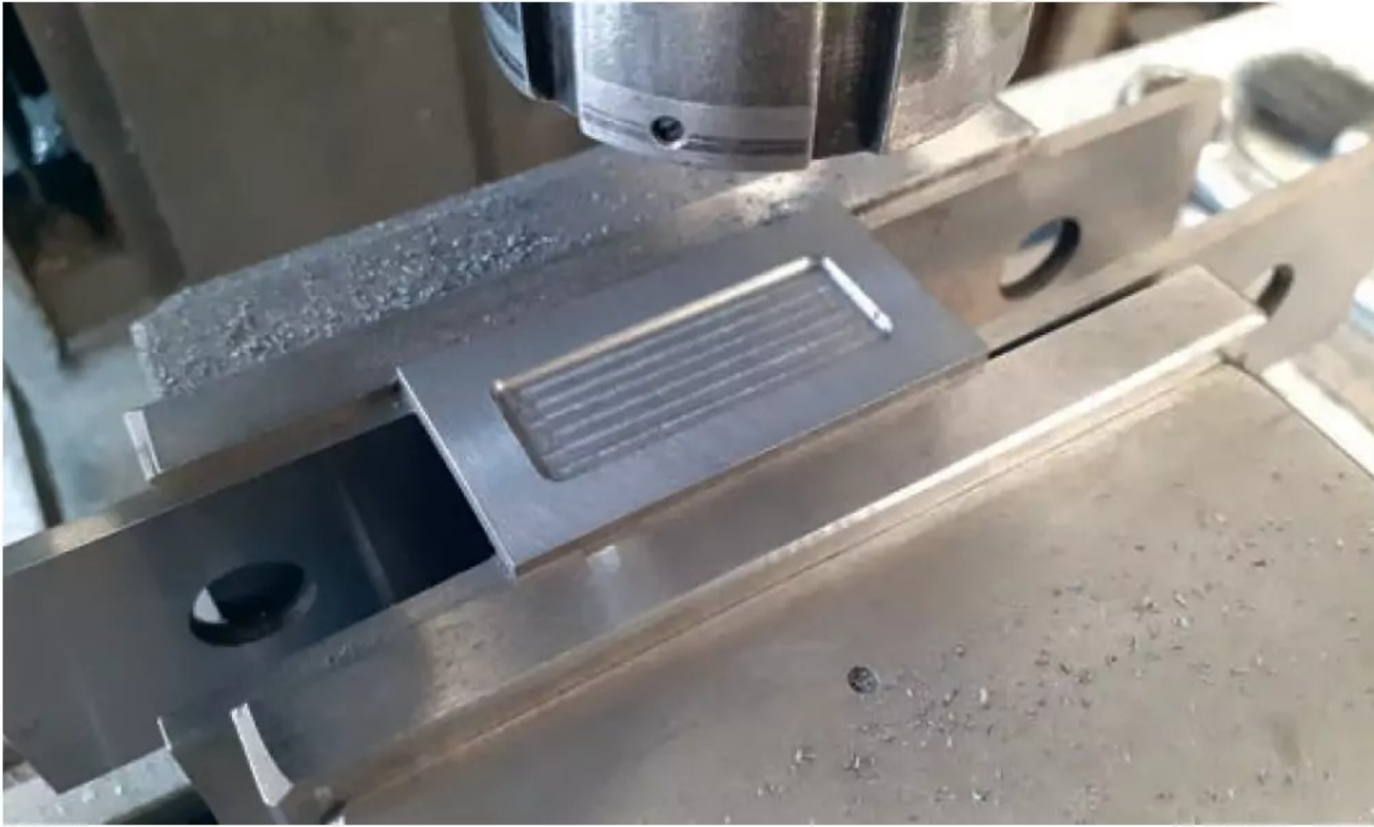
Photo 62: Milling chest valve cover recess
