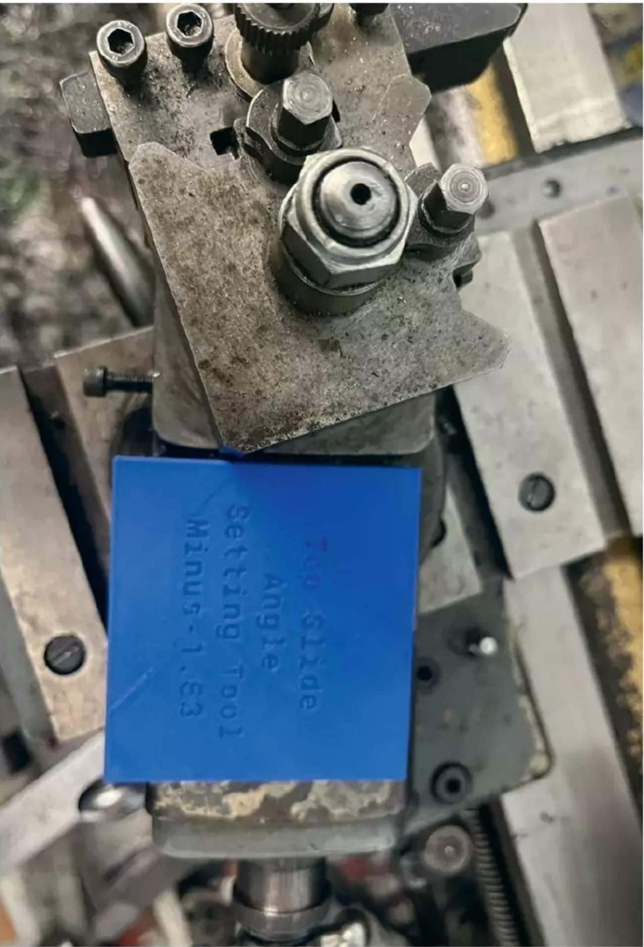
Photo 10: Aid in place prior to setting the correct angle.
