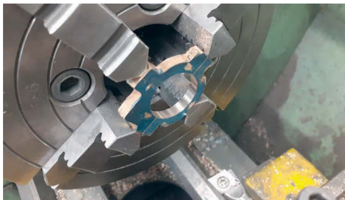
Photo 52: Boring the strap halves screwed together
