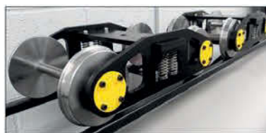
Machined Axle Boxes & Bearings in 5" & 7¼" gauge
