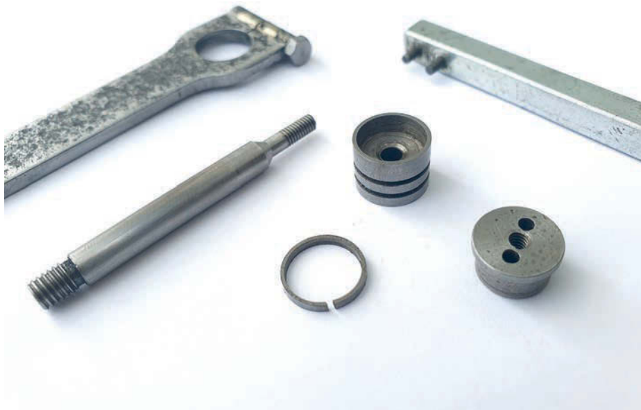
Photo 9: A disassembled piston and its keys.
