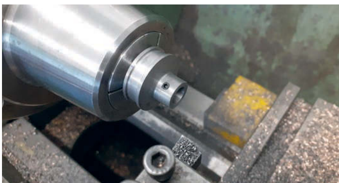
Photo 56: Completing eccentric mounted on arbor
