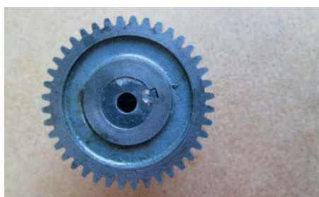
Photo 6: End view of gear mounted with its nice snug key.
