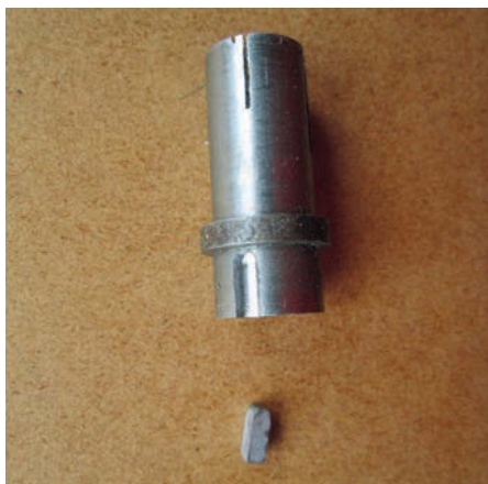
Photo 4: Key and machined mandrel extension ready for soldering.
