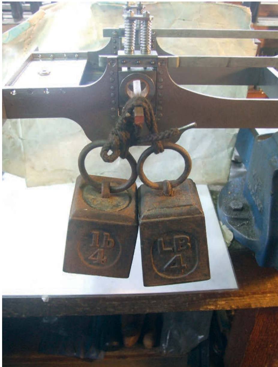
Photo 5: Checking of the spring loading at the axle running position. The collars fitted to the springs can just be seen.
