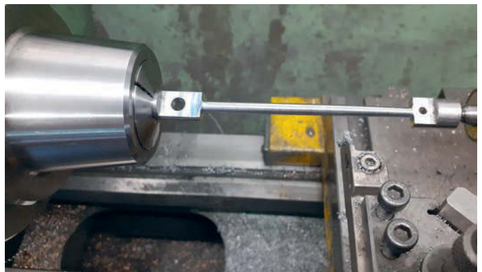
Photo 47: Taper turning conrod with rounded tool
