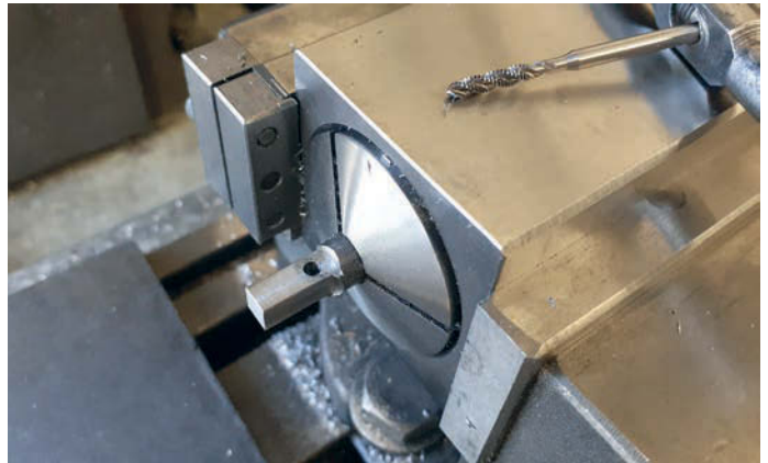
Photo 45: Valve rod clevis milled and drilled
