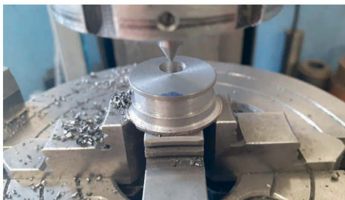
Photo 55: Offset hole reamed & marking high point
