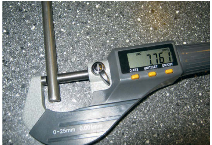
Photo 8: The steel rod was undersize.
