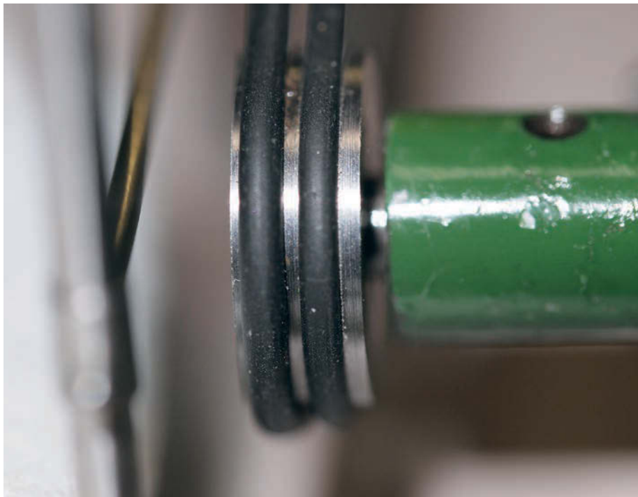
Photo 4: Two millimetre O-ring stock being used as governor drive belts. With smaller pulley diameters these would slip without the grooves.
