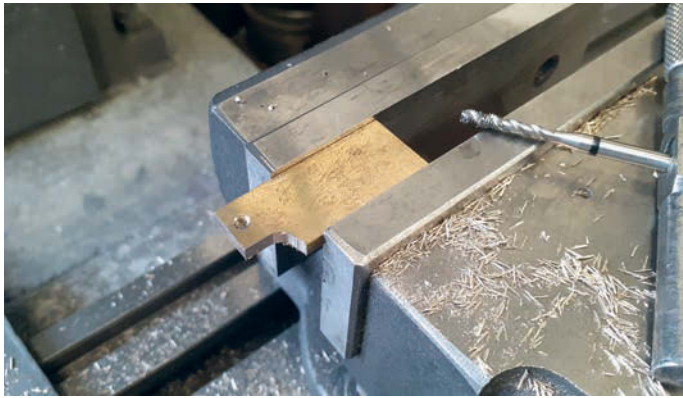
Photo 42: Valve nut machined from larger stock
