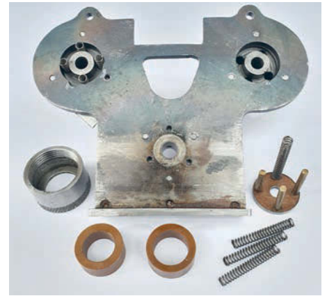
Photo 11: End plate with knob and pressure rings removed. The knobs on the end plates take four springs to apply even contact pressure to the port interface.
