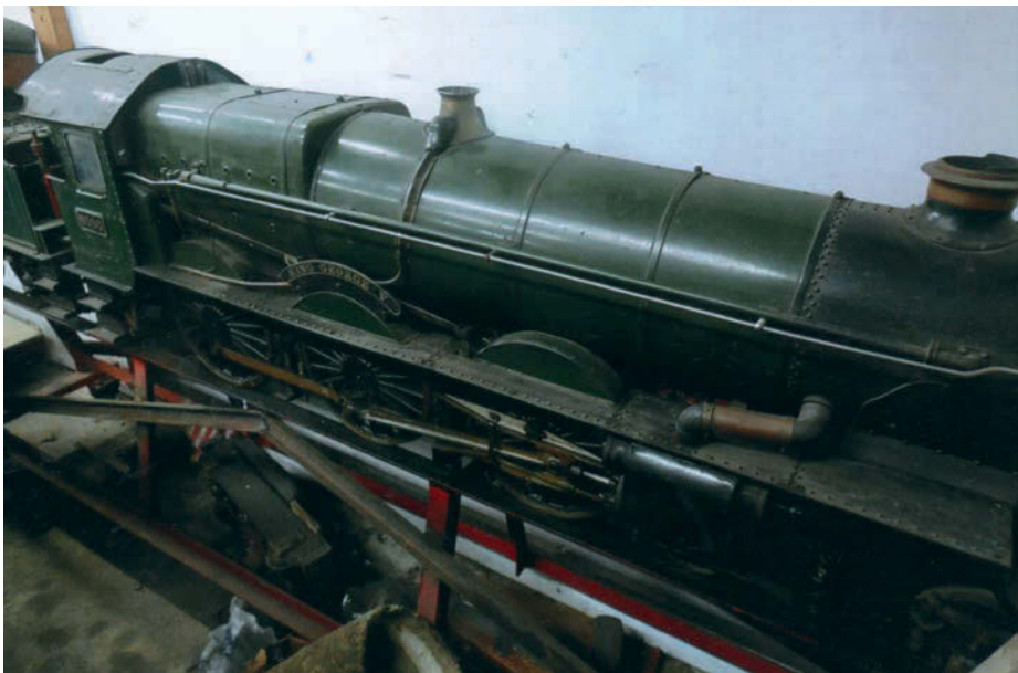
Photo 4: The Wilson-design King in 7 1/4" gauge that I eventually rebuilt, now awaiting a valve rebuild having worked hard for many years.
