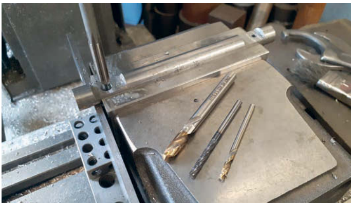
Photo 46: Conrod flats milled, drilled & reamed
