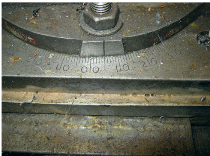
Photo 11: Setting taper angle on the lathe.
