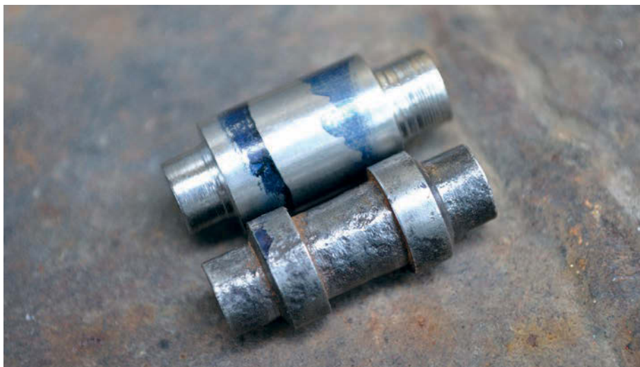
Photo 4: The original was cast iron but I soon turned up a bit of mild steel to suit.
