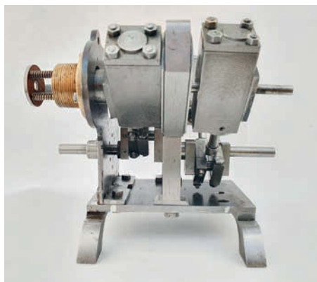
Photo 13: Side view showing cylinders and crankshaft. The right-hand cylinder is pulled back slightly revealing the inboard pivot pin and offset big end on the crank pin.
