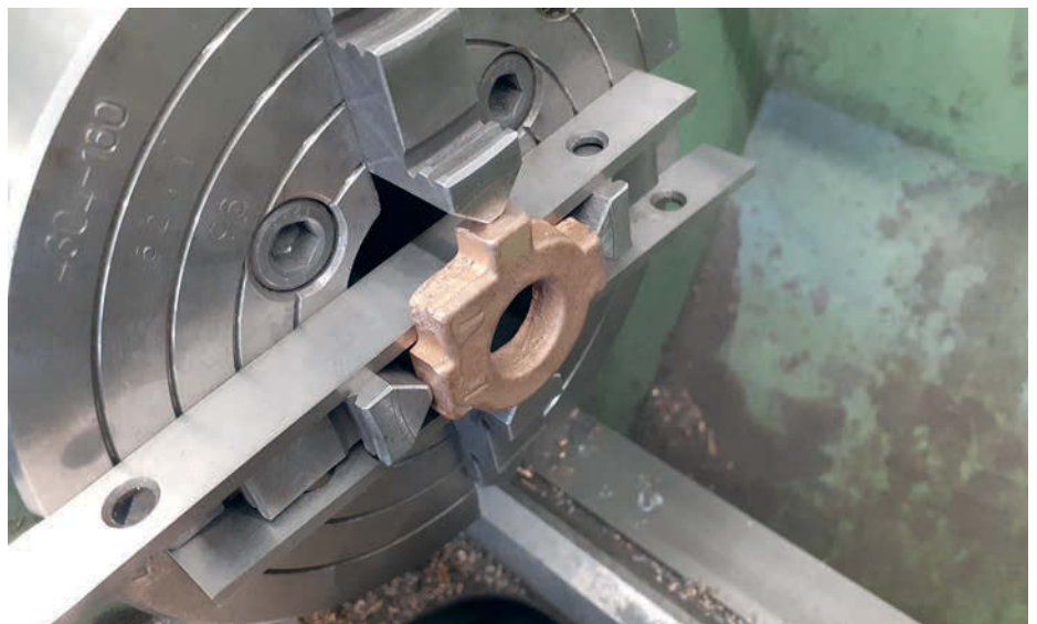
Photo 48: Setting strap to run wobble free with parallels
