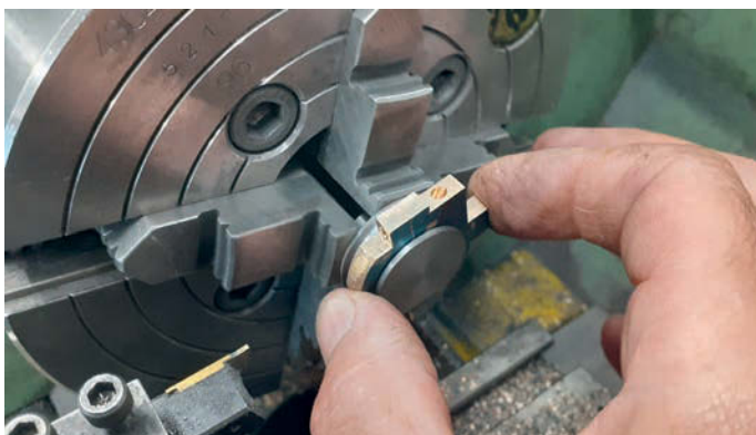
Photo 54: Using strap to gauge size of eccentric
