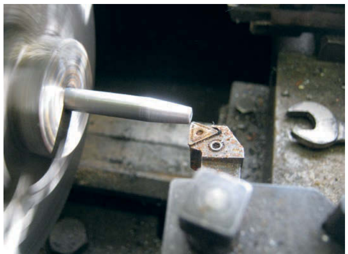
Photo 12: Cutting the taper.
