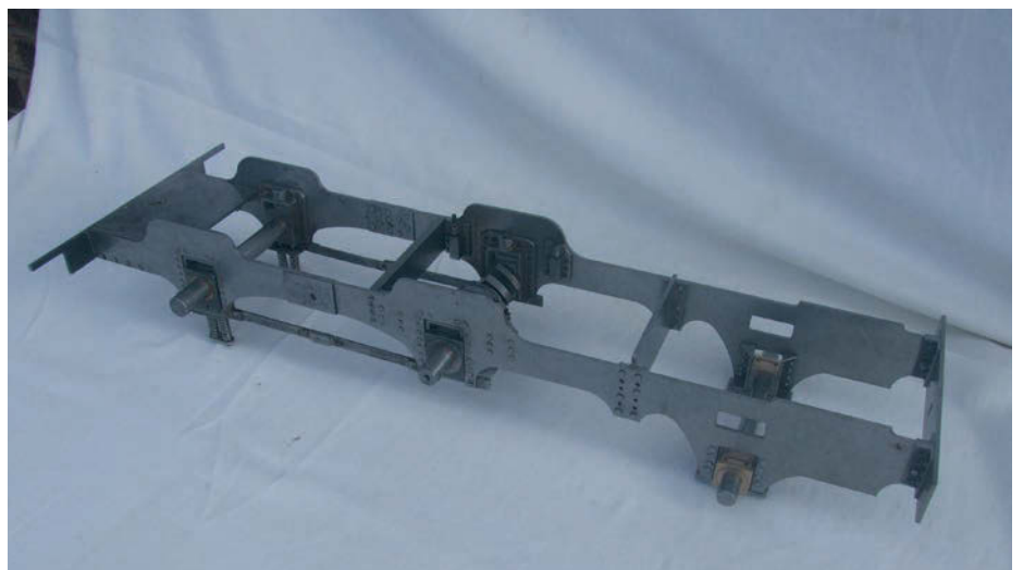
Photo 2: A view showing the current progress with the model development which is ready for the driving wheels and leaf springs to be fitted plus the coupled wheels.
