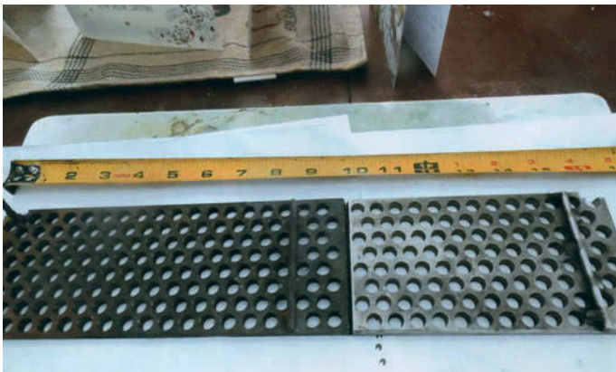
Photo 5: The taper holes in the King grates (upside down) they are fully 16 1/2" long.
