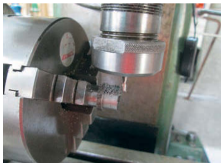
Photo 3: Milling with the work held in a three-jaw chuck.
