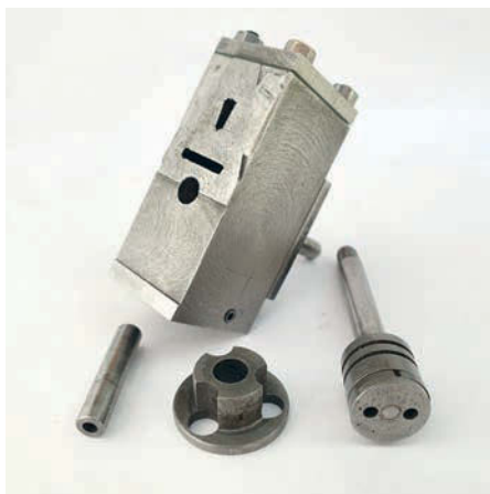
Photo 7: Cylinder, piston, rod guide and pivot pin.
