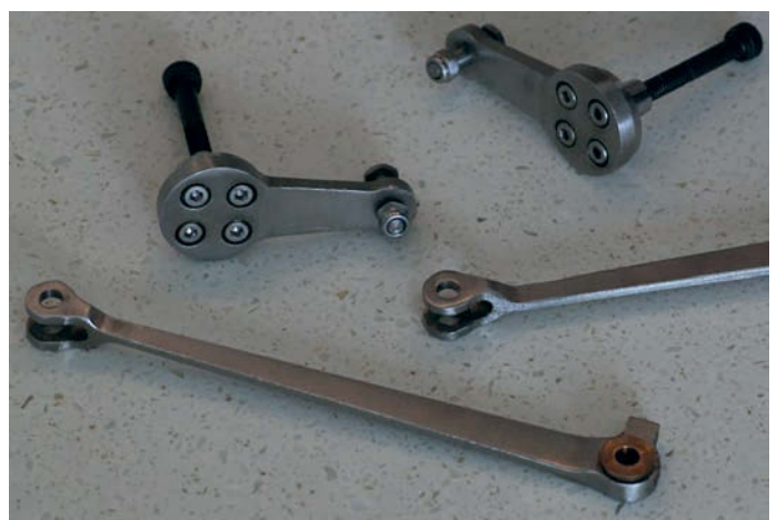
Photo 6: Valve connecting rods, not oiling point at bottom right.
