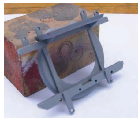
Photo 272: Door frame assembled and primed.
