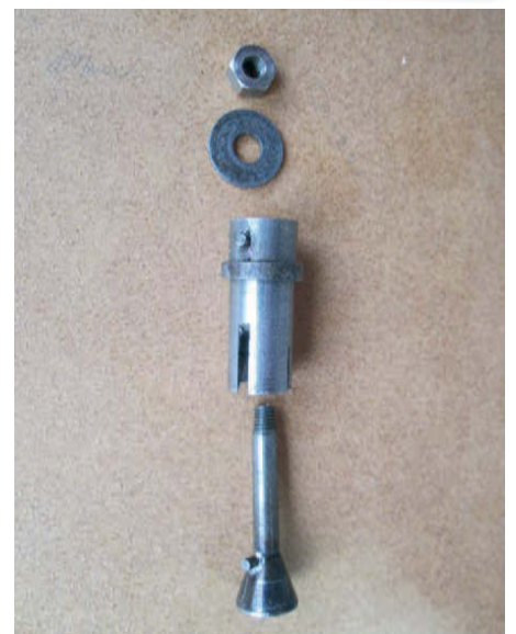
Photo 2: Components of the mandrel extension.
