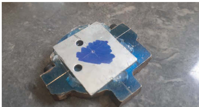
Photo 51: Centre of hole marked on scrap piece
