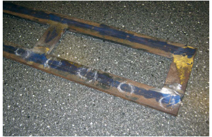
Photo 5: Welded up and marked out for tines.
