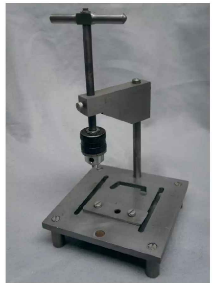
Photo 11: Modifications to this self-designed tapping stand featured in Making And Modifying A Tapping Stand, Engineering in Miniature , Vol 44 issue 11.
