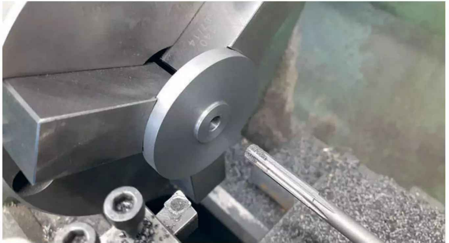
Photo 14: Reaming crank disc after turning
