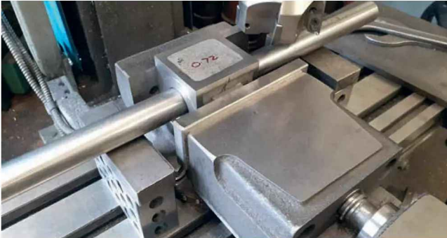
Photo 21: Cylinder base ready for final cut
