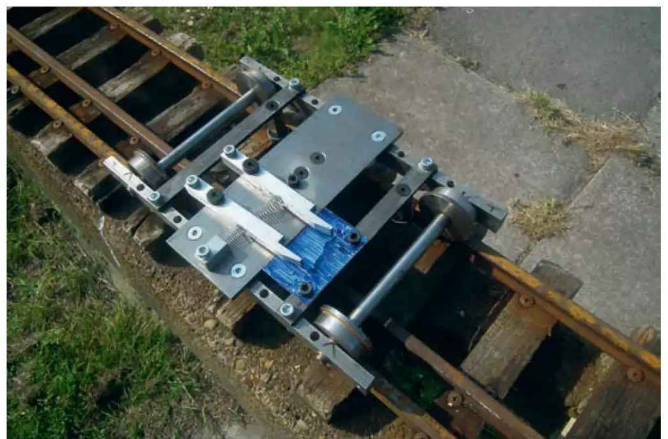
Photo 2: Another interesting device, a rolling track gauge used to check the distances between the rails.
