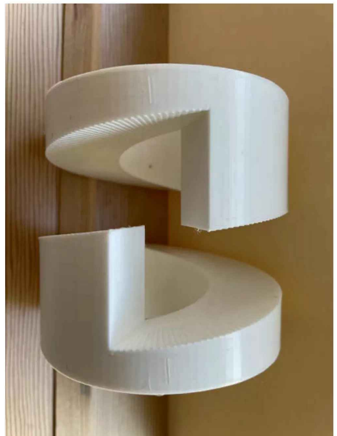
Photo 9: Prototype (before testing) press dies to produce part of a sheet metal helix for a steering chain guide in my traction engine build.
