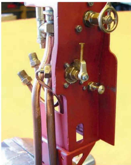
Photo 251: Front view with blower valve
