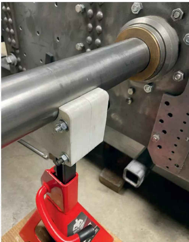
Photo 8: Two piece printed pad to more securely support the main axle on a project, this encloses the smaller top of the support stand column and protects the axle from damage.
