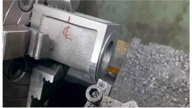
Photo 20: Facing end of cylinder with radius tool
