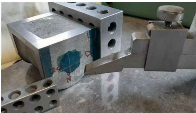
Photo 17: Marking centre of bore
