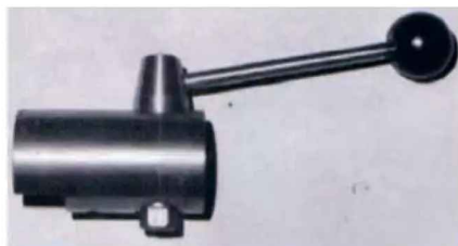
Photo 7: Thrust block with operating lever assembled prior to final mounting.
