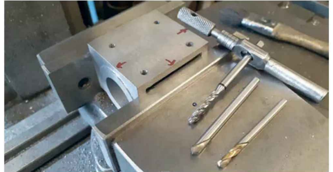
Photo 22: Drilling and tapping cylinder base
