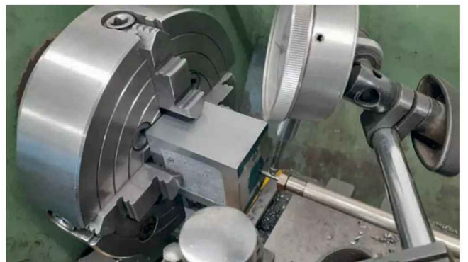
Photo 18: Clocking cylinder centre true in 4-jaw chuck
