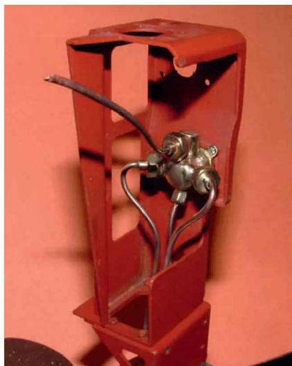
Photo 250: Rear view of valve assembled to pedestal.
