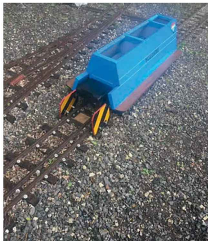
Photo 9: Paul Tanner of York Model Engineers designed this simple but effective device to prevent runaways on to running lines.
