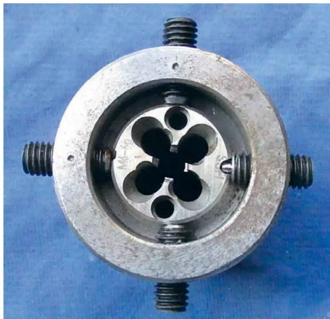
Photo 2: One end of the body uses four screws to centre the die.
