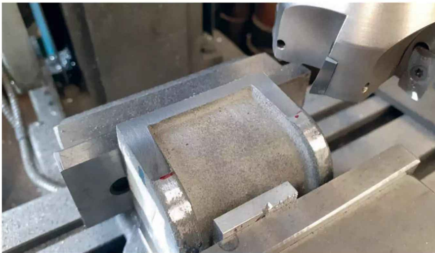
Photo 16: Squaring edge of cylinder upto centre height
