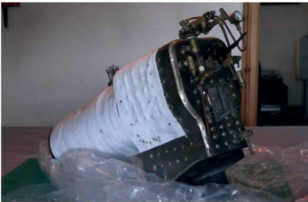
Photo 3: Boiler with backhead fittings loosely attached.
