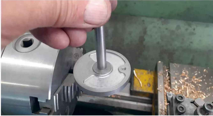
Photo 15: Checking fit of crankshaft spigot in crank
