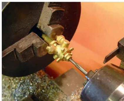
Photo 249: Reaming the valve body.
