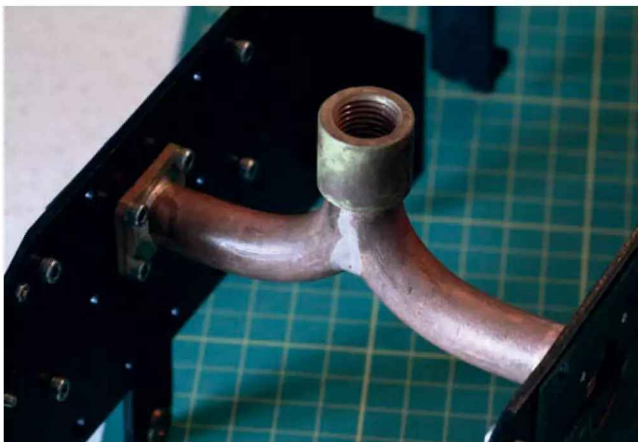
Photo 9: Steam exhaust pipe.
