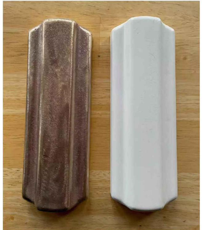
Photo 7: Printed casting pattern (painted white) with included edge draft and shrinkage allowances, resultant cast part shown to the left.
