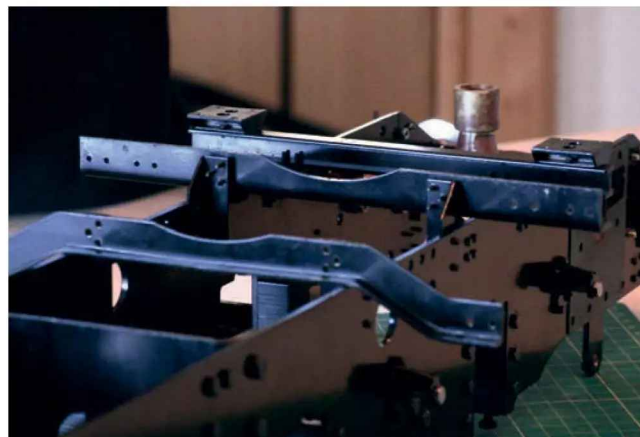
Photo 12: Support beams for boiler and water tank.
