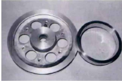
Photo 5: Driving pulley and 'fixed' half of clutch.
