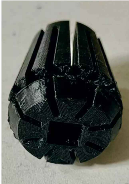
Photo 1: ER32 printed collet for odd sized square stock.
