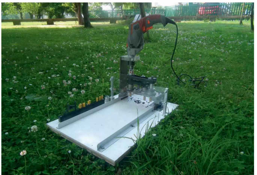
Photo 1: The sleeper groove cutting machine.
