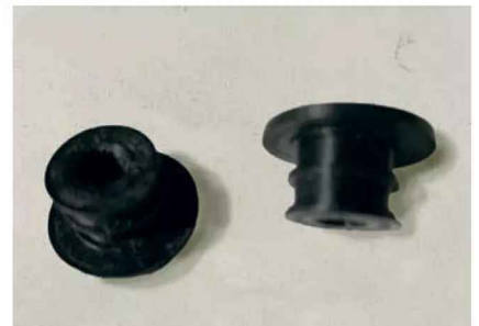
Photo 5: Prototype threaded inserts for cast polyurethane parts.
