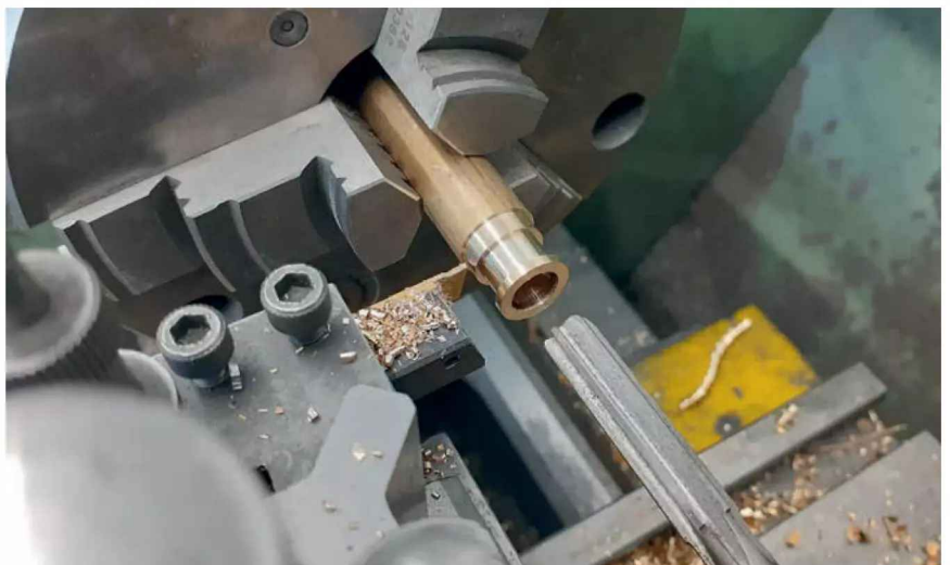
Photo 13: Completed bearing ready to be parted off
