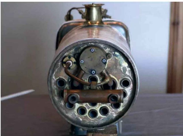
Photo 5: Smokebox end of boiler.
