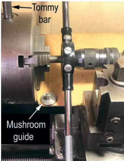
Photo 4: Mushroom guide used to press against the back of a die in a standard die holder.
