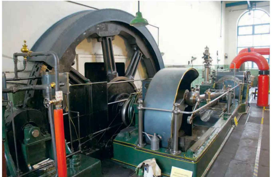
Photo 6: The then working tandem compound engine at Queen Street Mill, Burnley. A Model Engineer article encouraged visitors to go before it closed.
