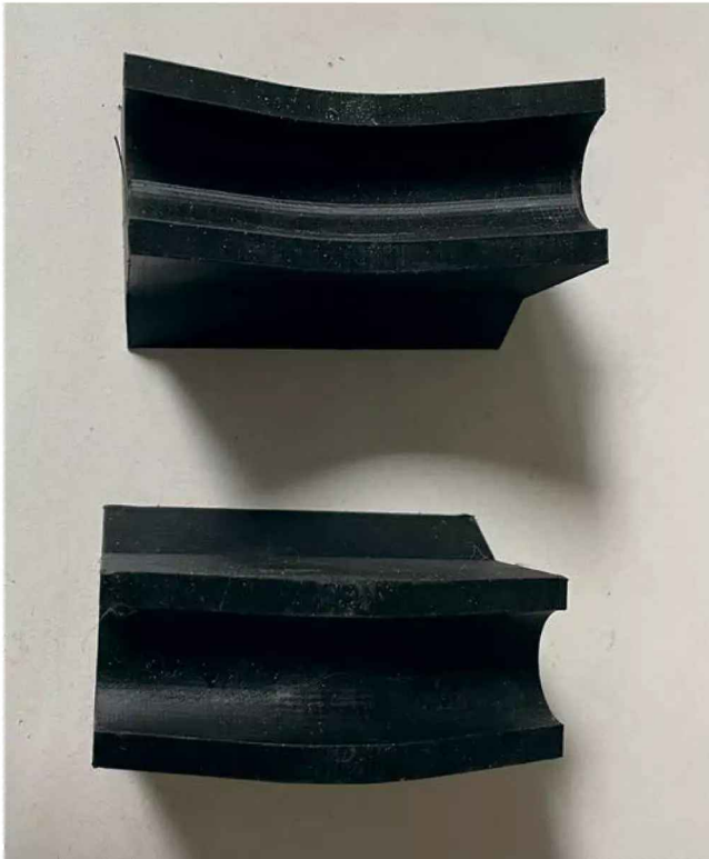
Photo 6: Copper tube bending dies, male and female, diameter specific.
