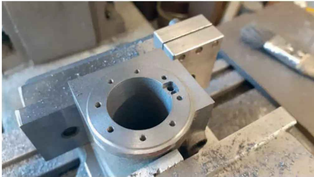
Photo 25: Cylinder ends drilled, tapped and milled
