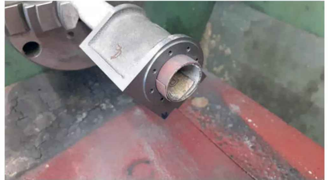
Photo 26: Lapping cylinder with Emery around a tube
