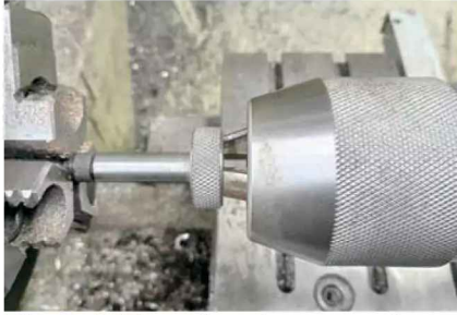
Photo 3: Pressing the extension piece into place.
