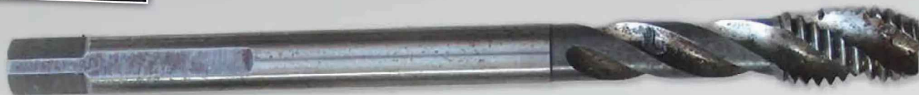
Photo 1: Machine taps modified for positive grip.
