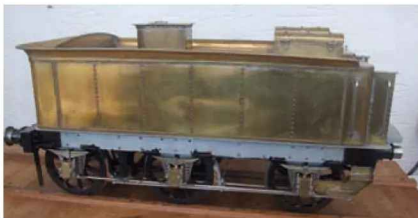
Photo 2: The as yet unfinished tender made by the writer which is the standard tender for the early L&NWR locomotives by Ramsbottom and Webb.
