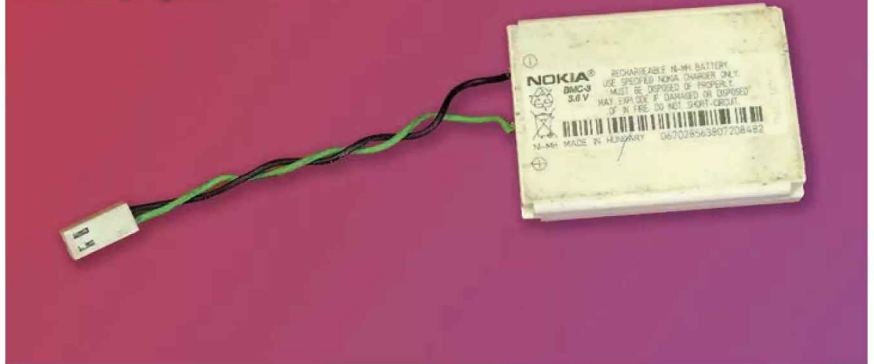
Photo 9: Healthy mobile phone battery fitted with a flying lead for use in a project.
