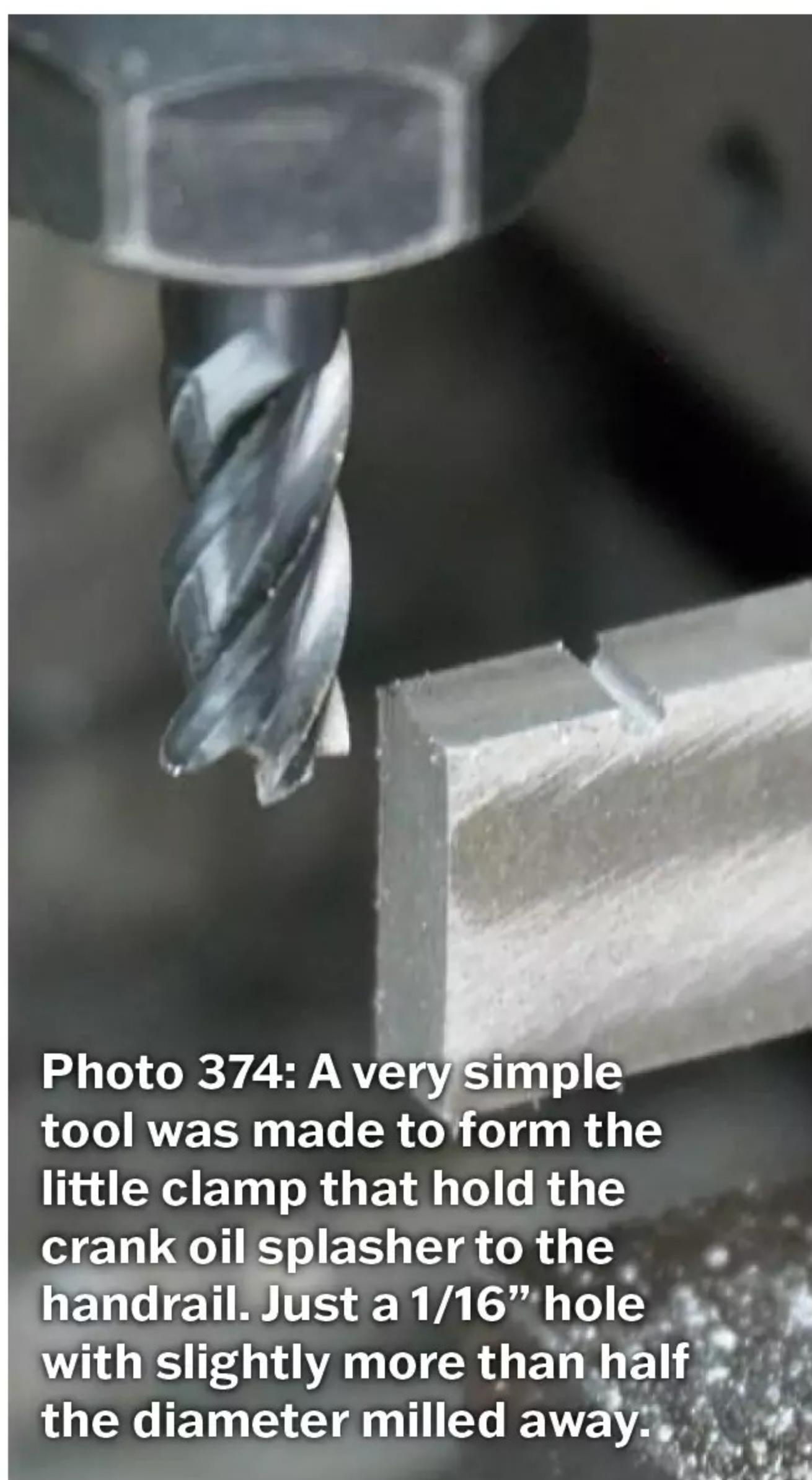
**Photo 374:** A very simple tool was made to form the little clamp that hold the crank oil splasher to the handrail. Just a 1/16" hole with slightly more than half the diameter milled away.
