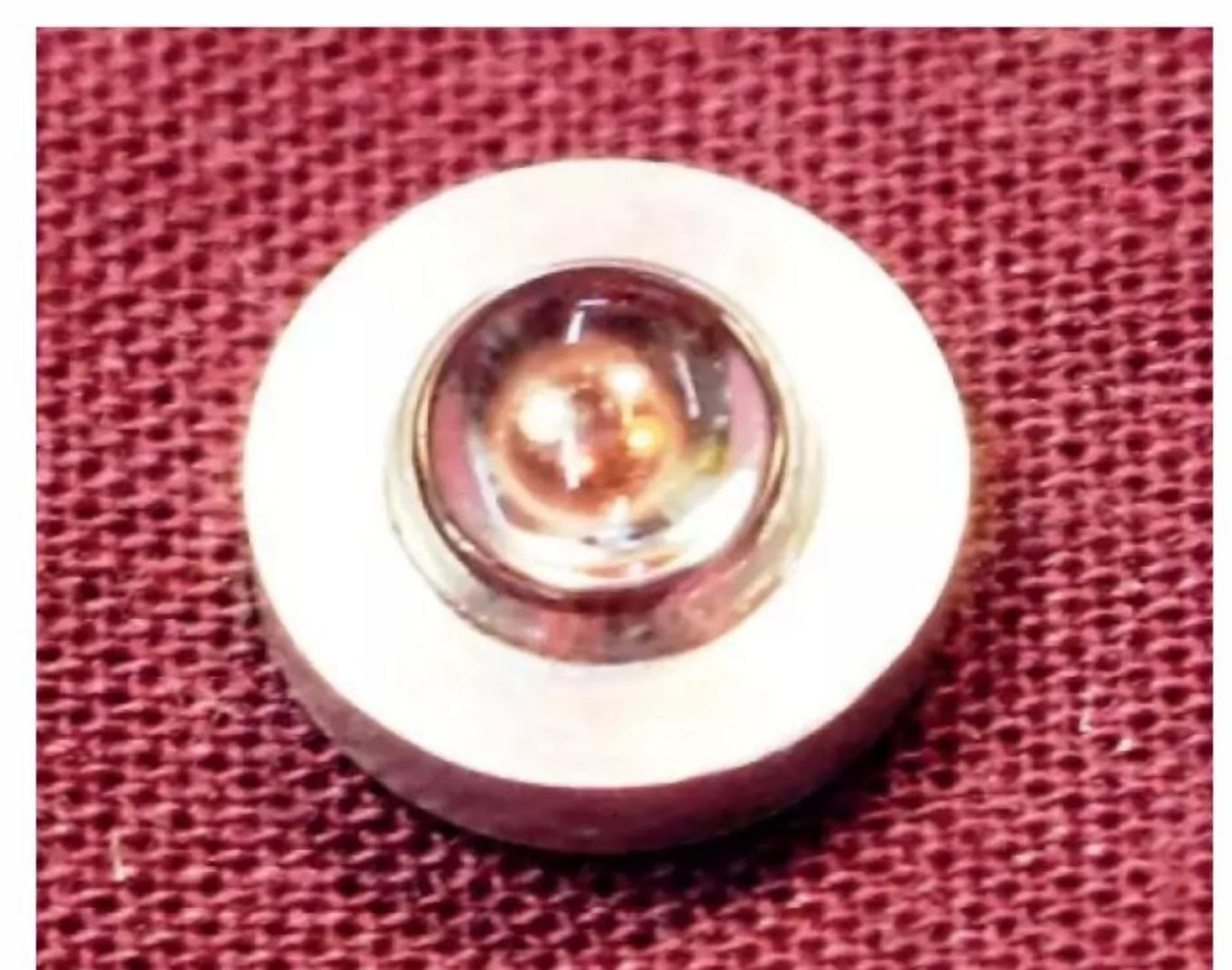
**Photo 28:** Intact MES bulb lens in the metal mount after successfully cutting from the glass envelope.
