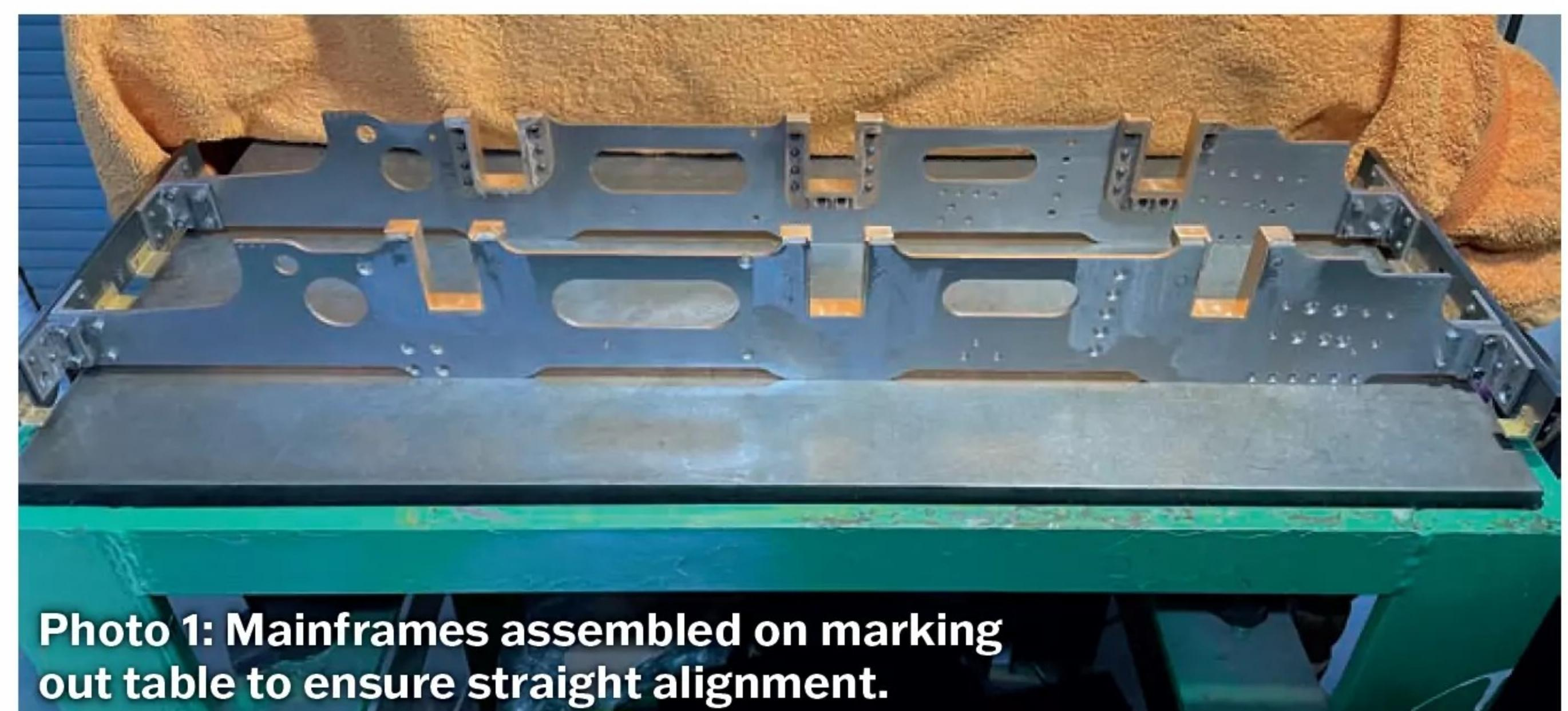
**Photo 1: Mainframes assembled on marking out table to ensure straight alignment.**
