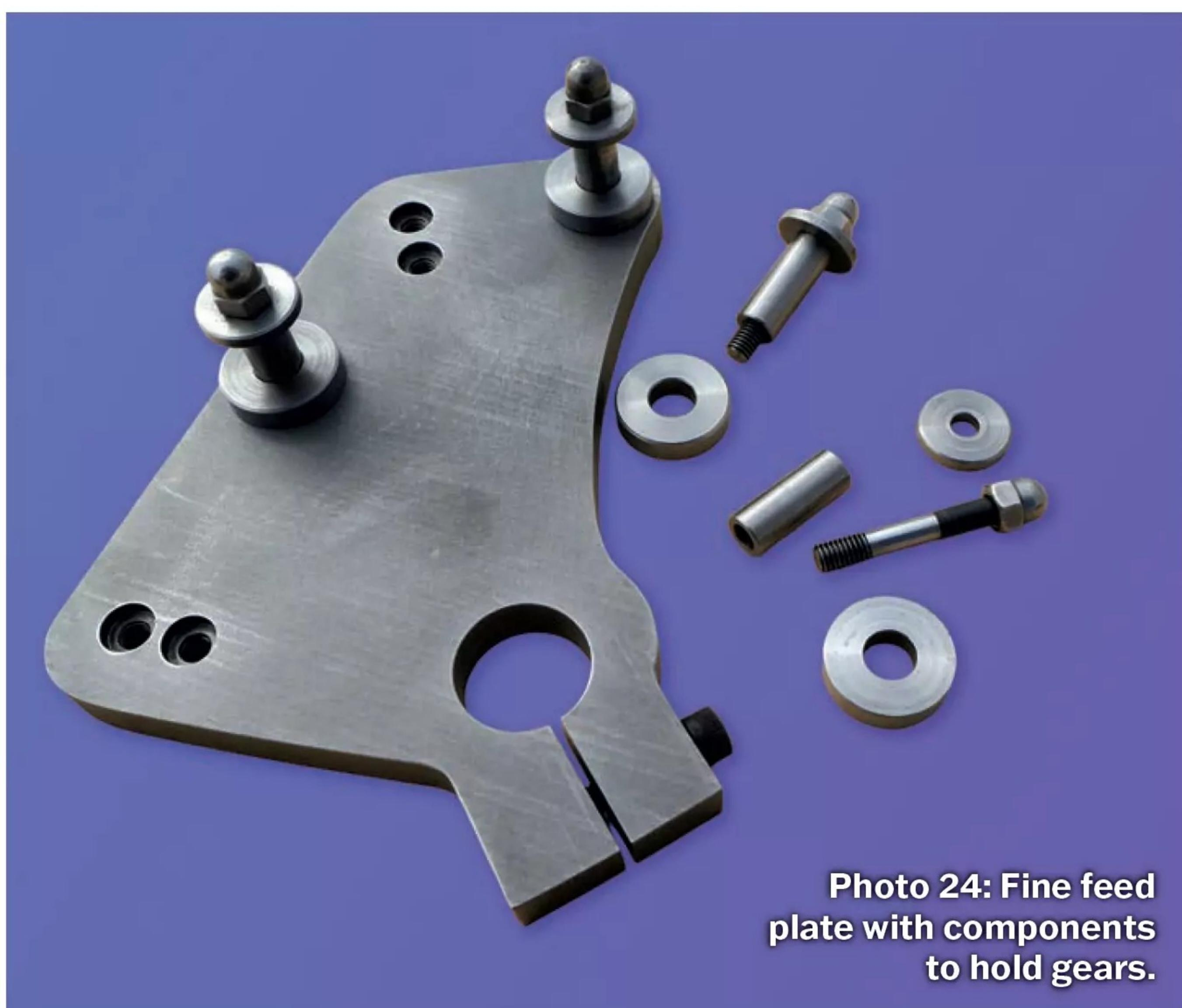
**Photo 24: Fine feed plate with components to hold gears.**
