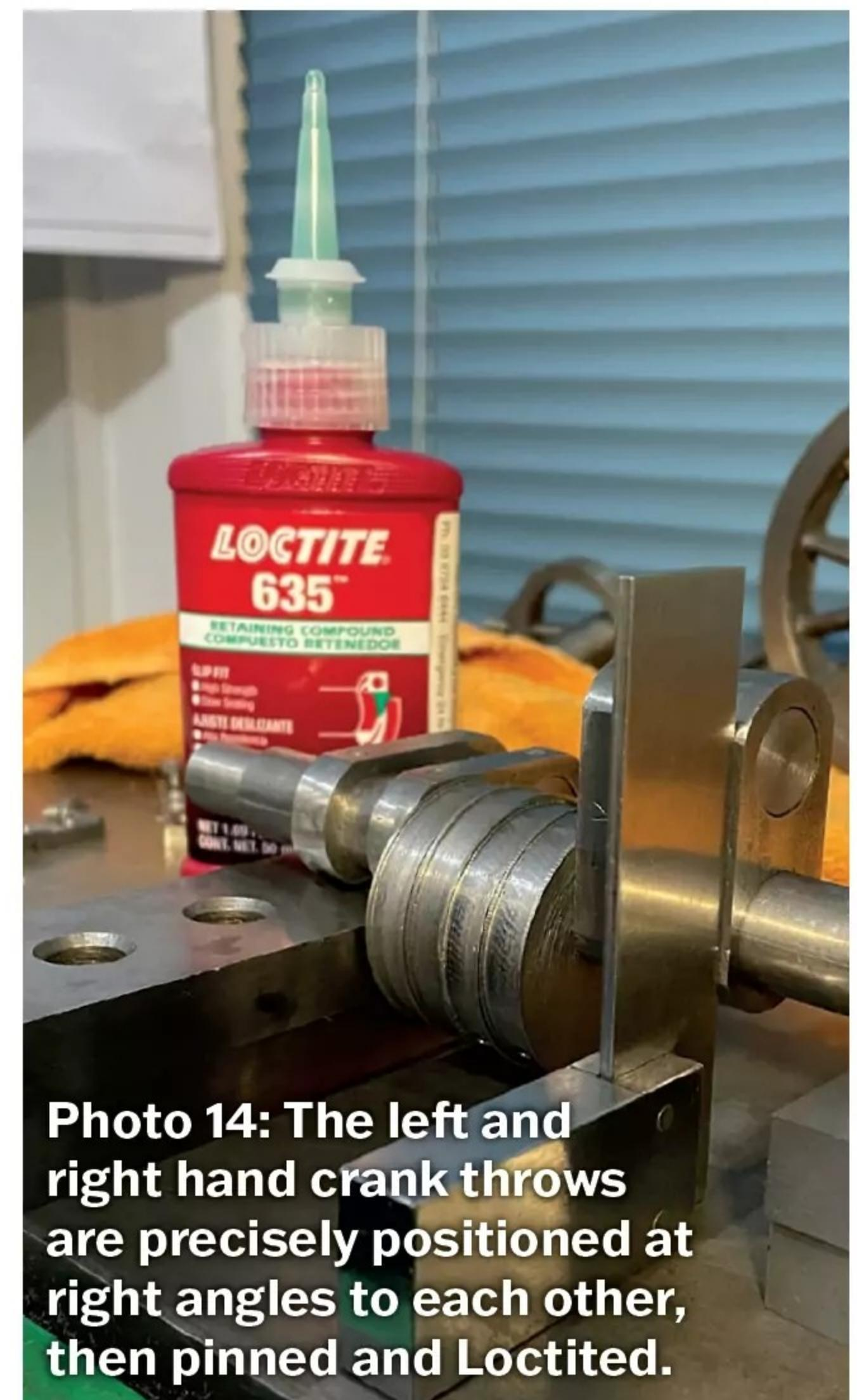
**Photo 14:** The left and right hand crank throws are precisely positioned at right angles to each other, then pinned and Loctited.
