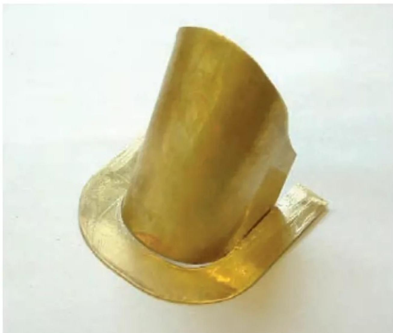
**Photo 230: Steam pipe cover before silver soldering.**
