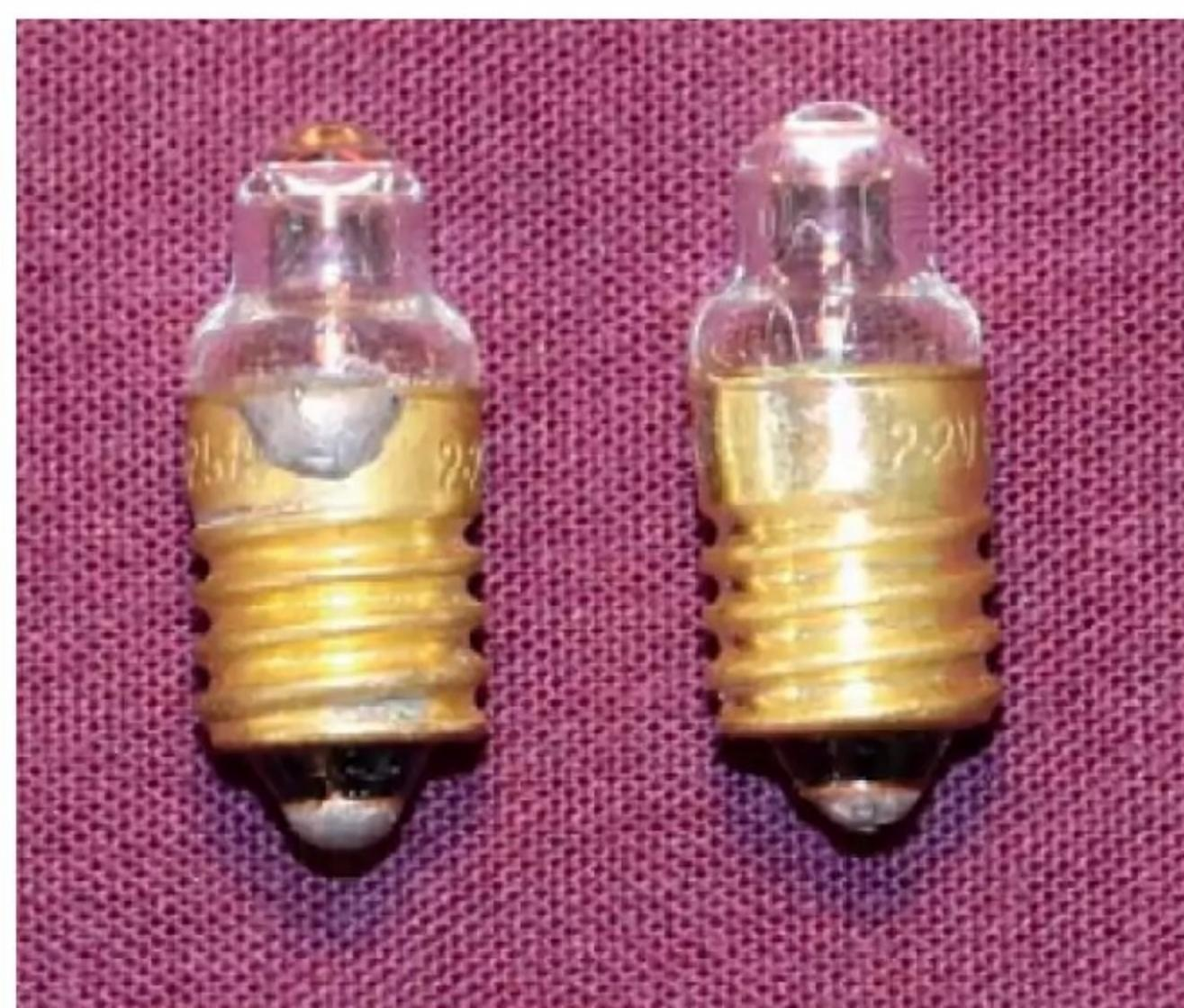
**Photo 22:** A pair of old MES lensed torch bulbs found in my scrap collection. New copies are still available and appear to be identical, with the exception that the threads are chrome plated.
