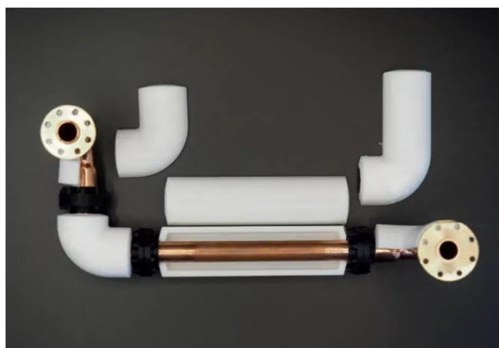
**Photo 379: The pipe run from the HP to LP cylinders under construction. The dummy flanges have been slipped onto the pipe before making the joints and the 3D printed pipe lagging is ready to glue together.**
