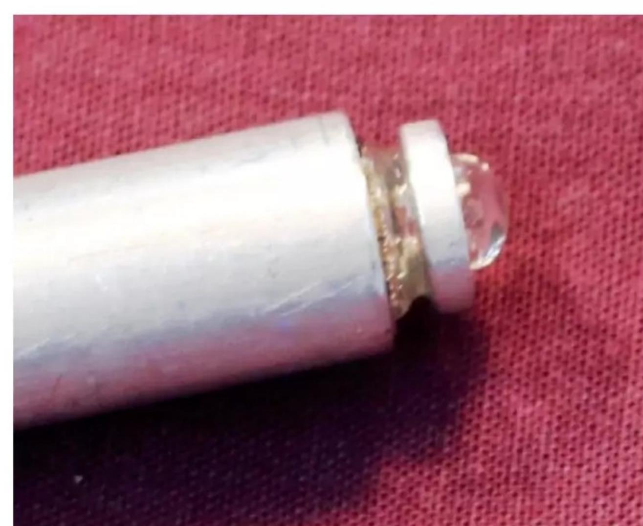
**Photo 27:** The solution to the bulb shattering was to bond a metal ring to the bulb before cutting to restrain the glass stresses.
