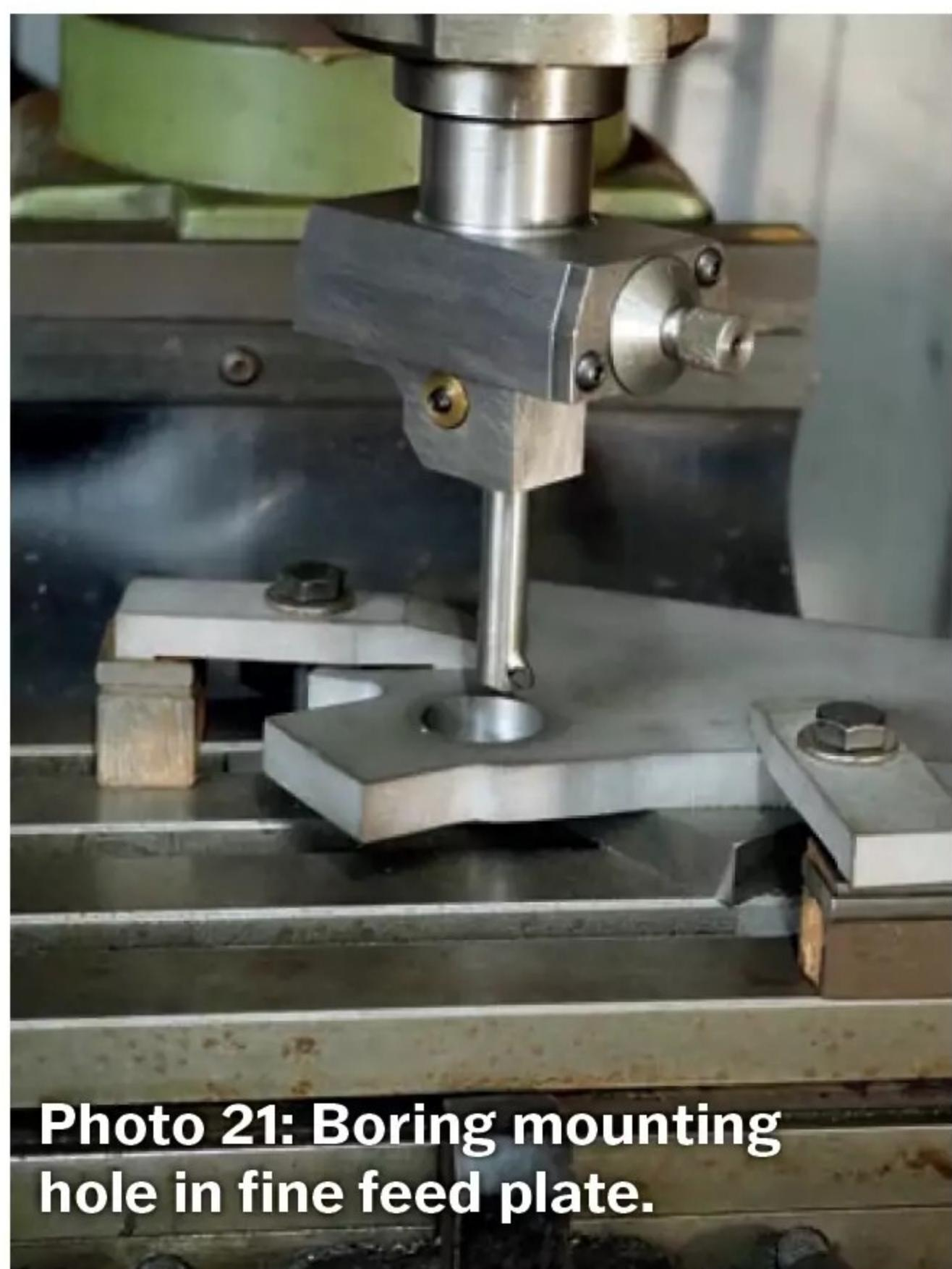
**Photo 21:** Boring mounting hole in fine feed plate.
