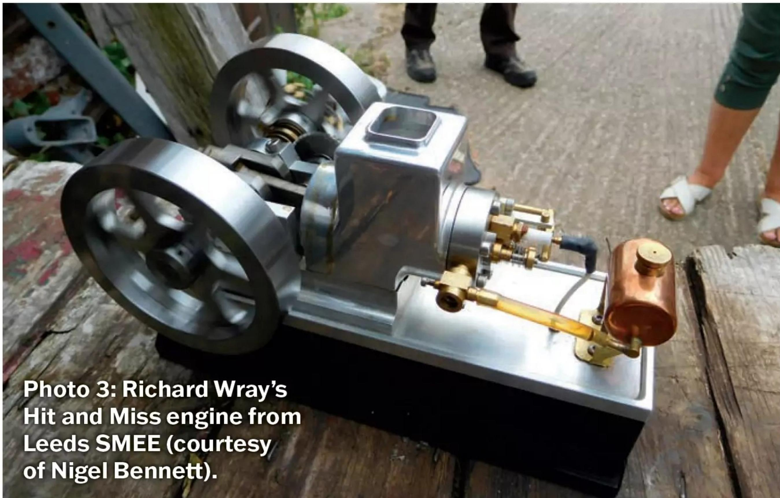
**Photo 3: Richard Wray's Hit and Miss engine from Leeds SMEE (courtesy of Nigel Bennett).**
