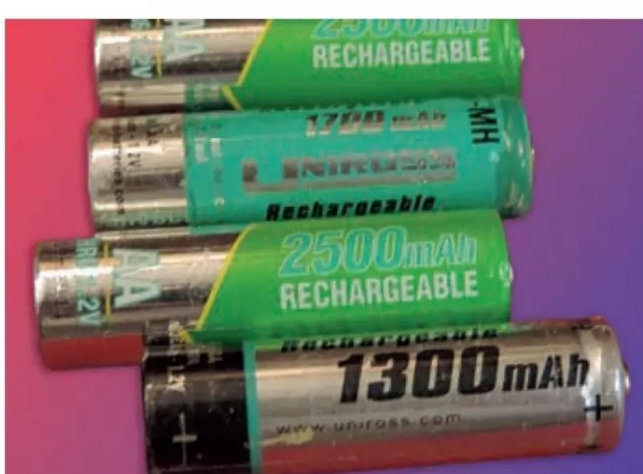
**Photo 1:** AA NiMH cells with capacities from 1300mAh to 2500mAh.
