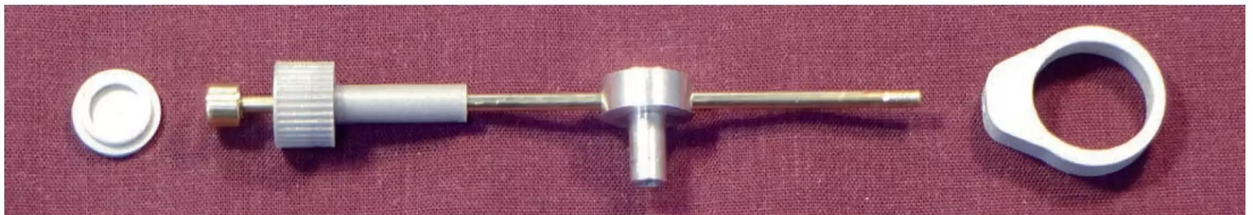
**Photo 31:** The beam and rotor assembly that allows movement of the specimen holder, right, in both the X and Y directions. Specimens are held in the rotor right and the brass beam slides through, and pivots in, the baseplate on the aluminium bush. The knob, left, is sheathed in a Helliman rubber and rolls over the baseplate to provide fine movement.
