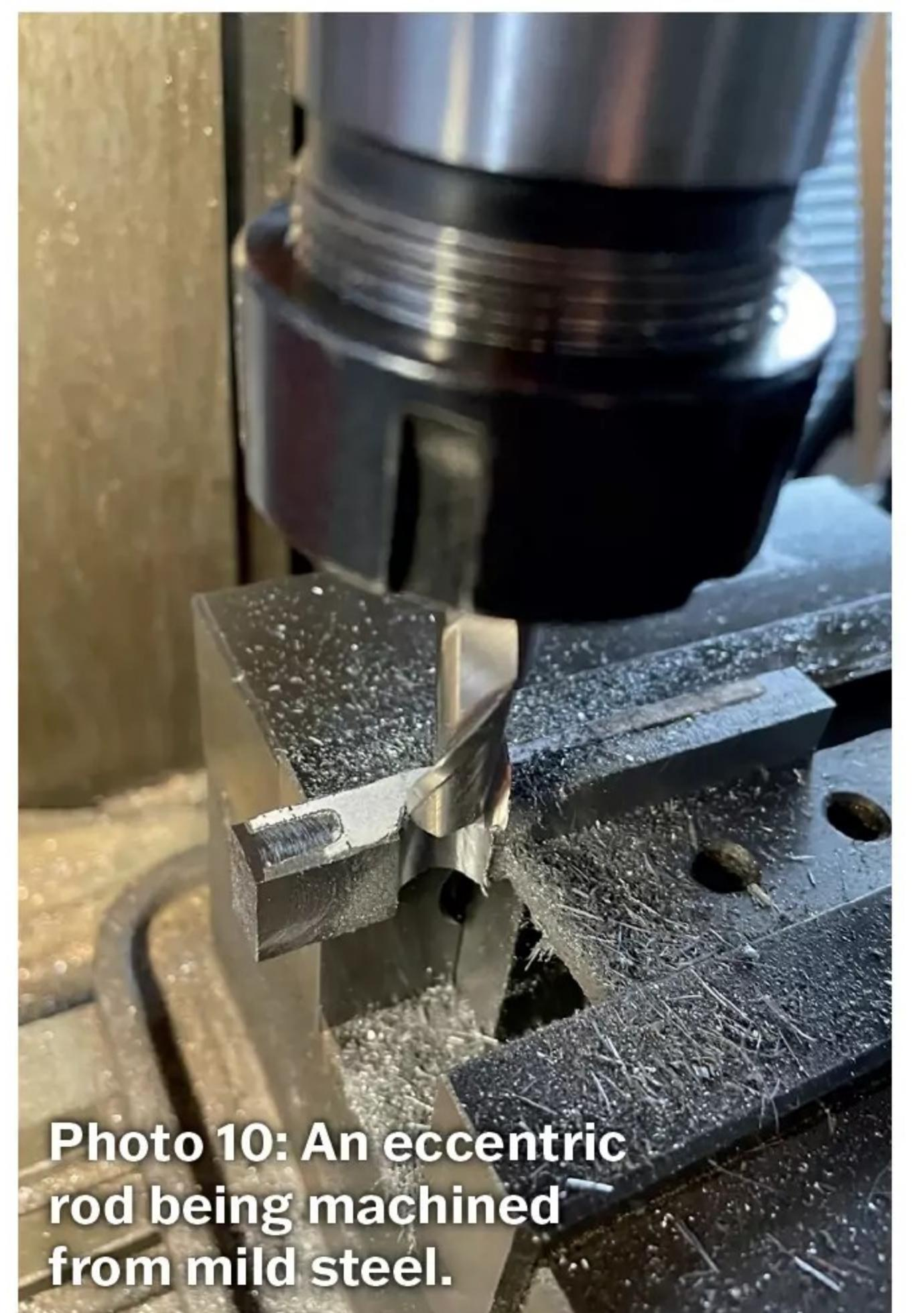
**Photo 10: An eccentric rod being machined from mild steel.**
