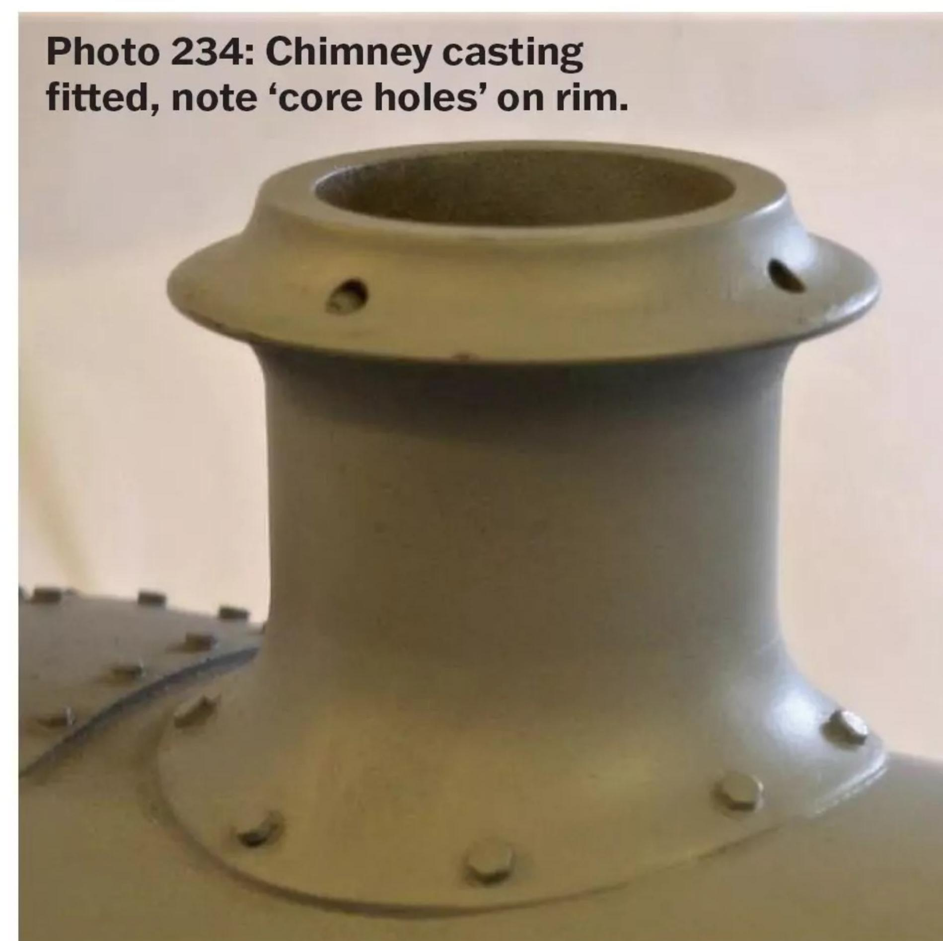
**Photo 234: Chimney casting fitted, note 'core holes' on rim.**
