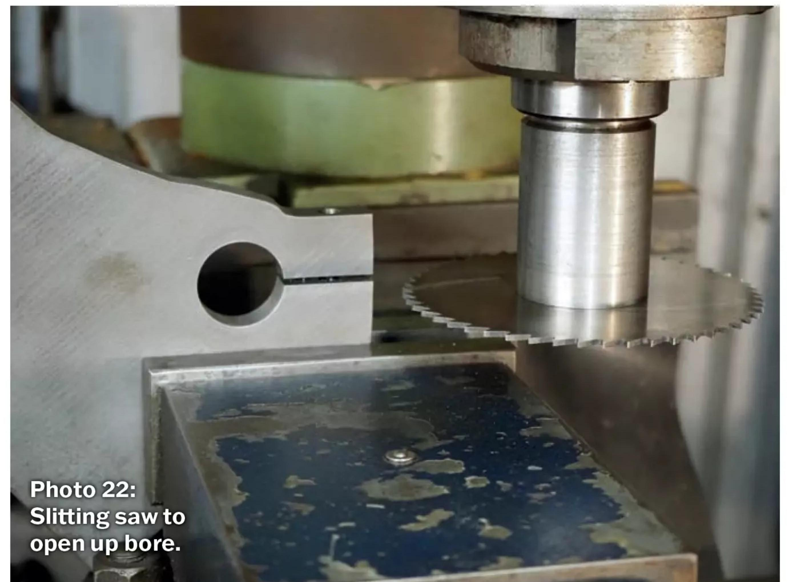
**Photo 22:** Slitting saw to open up bore.
