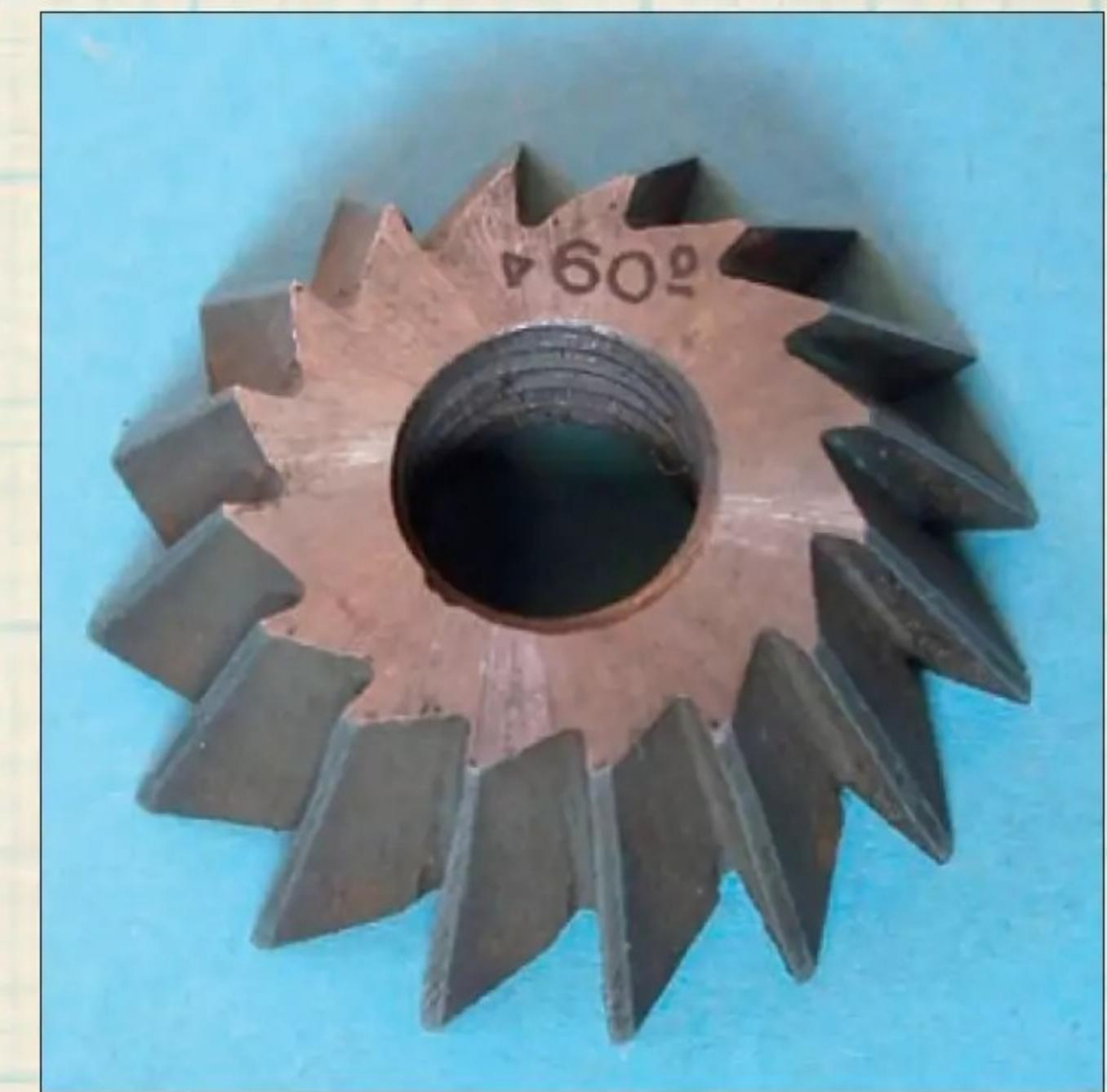
**Photo 1: Internally threaded dovetail cutter.**
