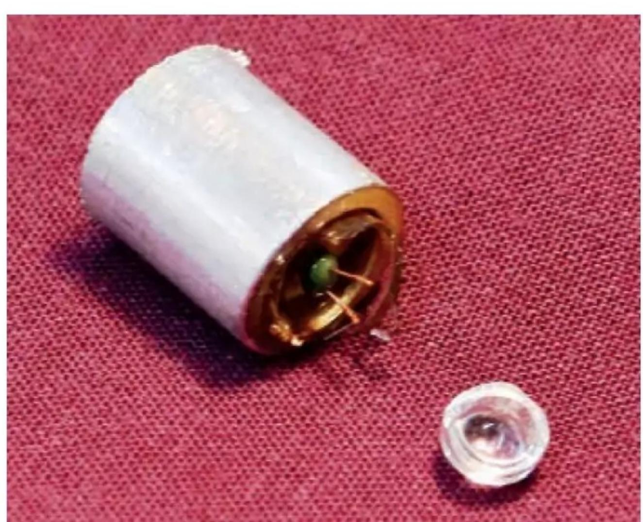
**Photo 26:** The MES bulb shattered when the cutter was only part way through owing to stress being unlocked in the glass envelope.
