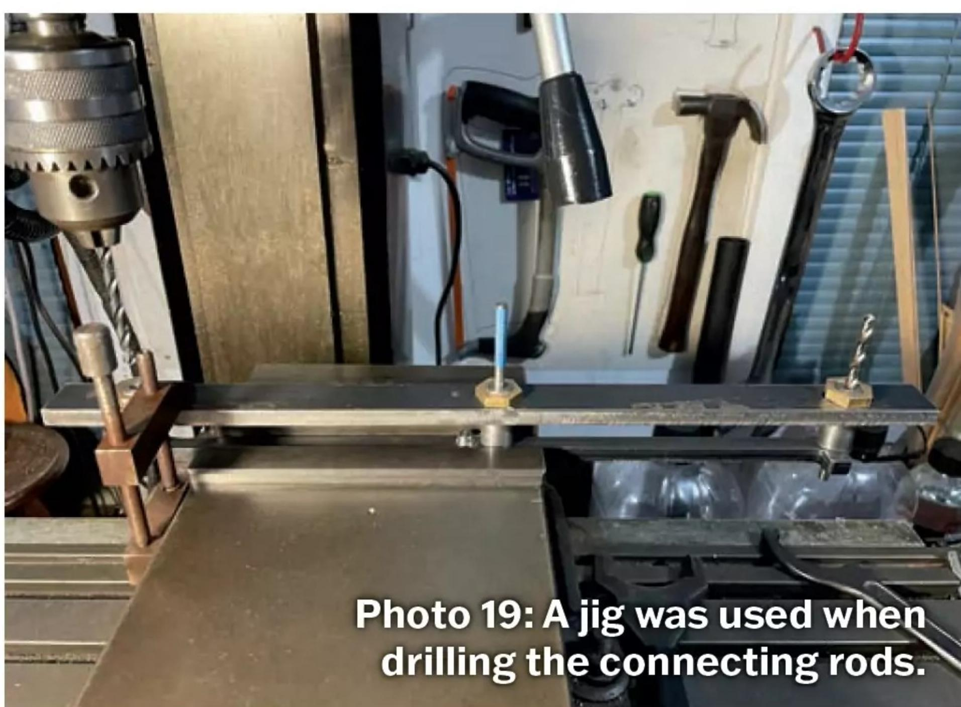
**Photo 19:** A jig was used when drilling the connecting rods.
