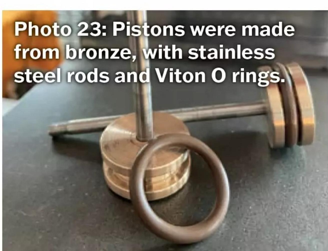
**Photo 23:** Pistons were made from bronze, with stainless steel rods and Viton O rings.
