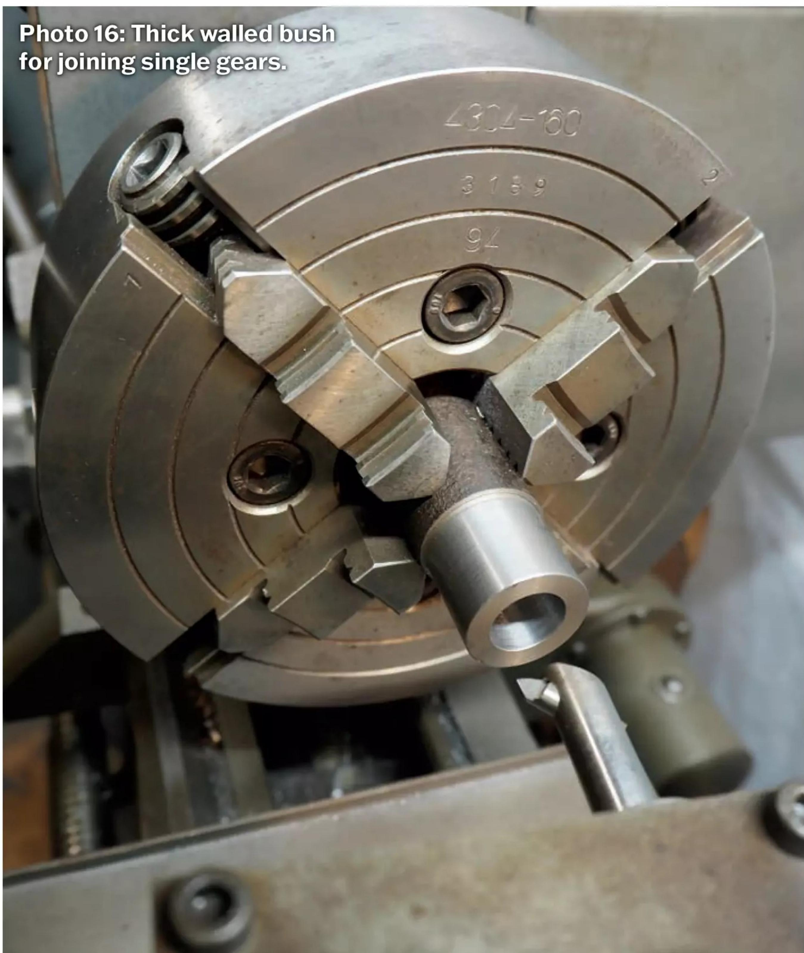
**Photo 16:** Thick walled bush for joining single gears.
