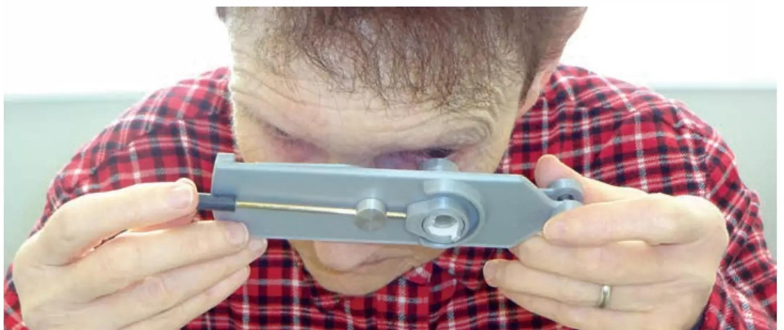
**Photo 35:** The microscope in use: the pair of fingers on the left hand is adjusting the focus, while the right hand is moving the roller knob and beam to move the sample in the X and Y directions.
