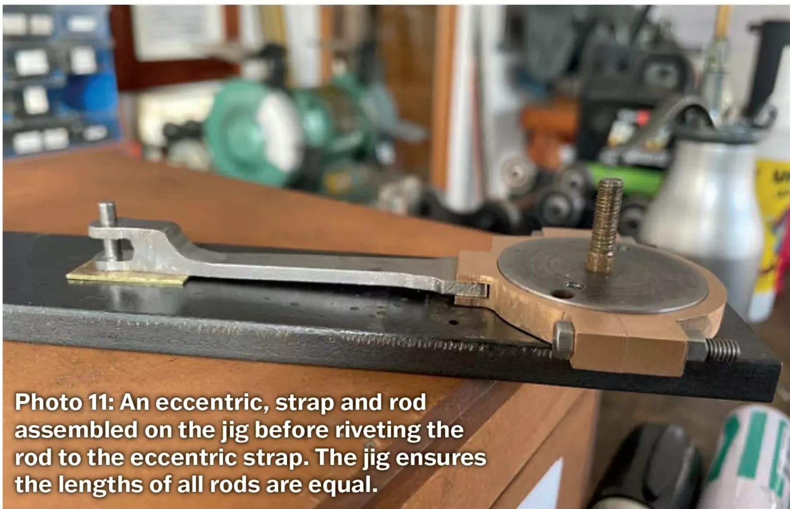
**Photo 11:** An eccentric, strap and rod assembled on the jig before riveting the rod to the eccentric strap. The jig ensures the lengths of all rods are equal.
