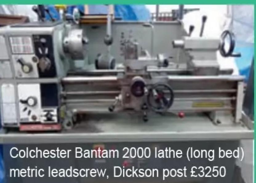
Colchester Bantam 2000 lathe (long bed)
