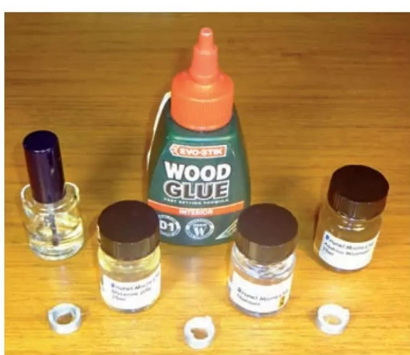
**Photo 34:** Fluids for mounting specimens: PVA glue, clear nail varnish and professional mountant media from Brunel Microscopes. At the front are three completed specimen holders containing bees' wings and pollen.
