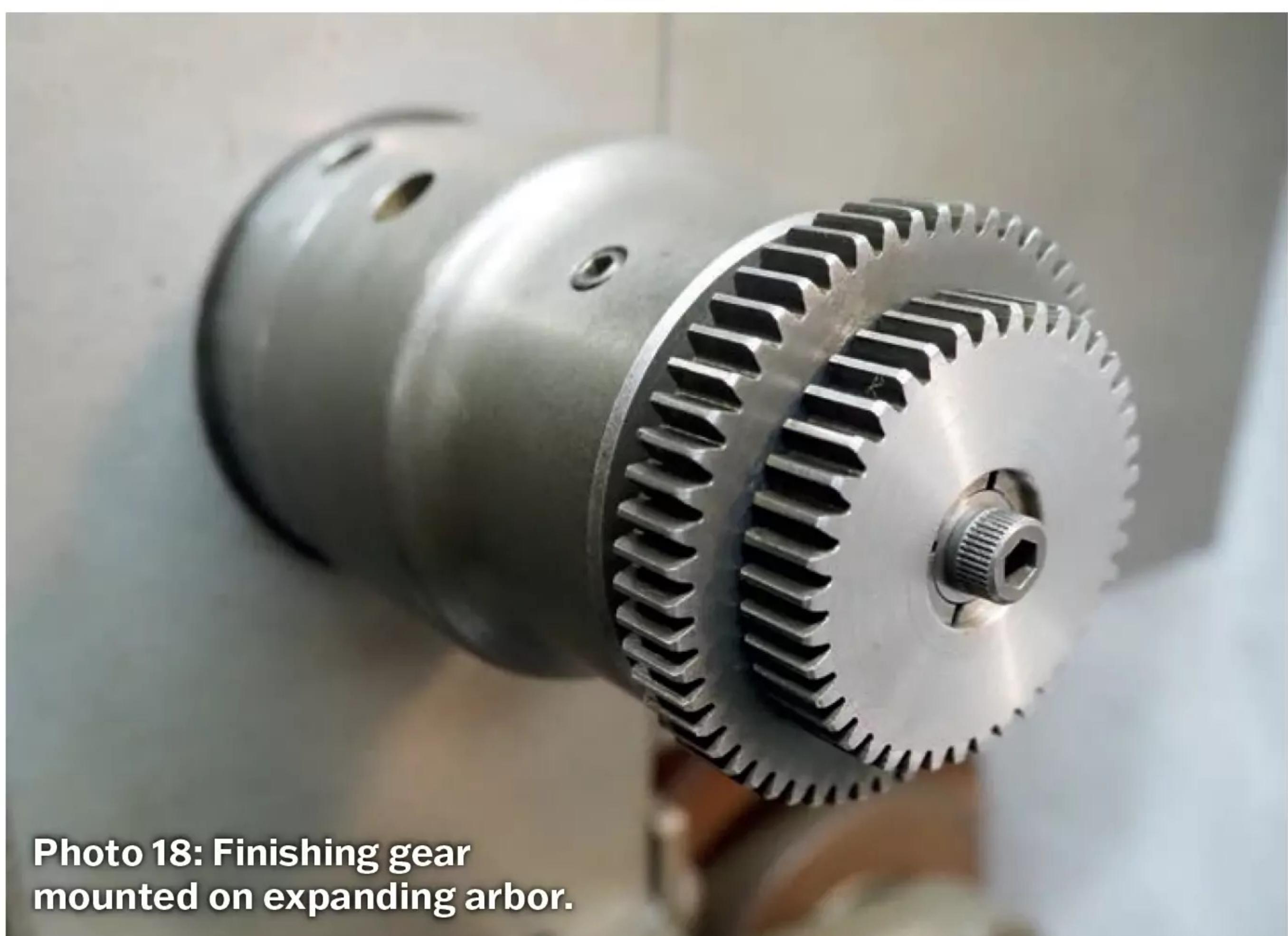
**Photo 18: Finishing gear mounted on expanding arbor.**
