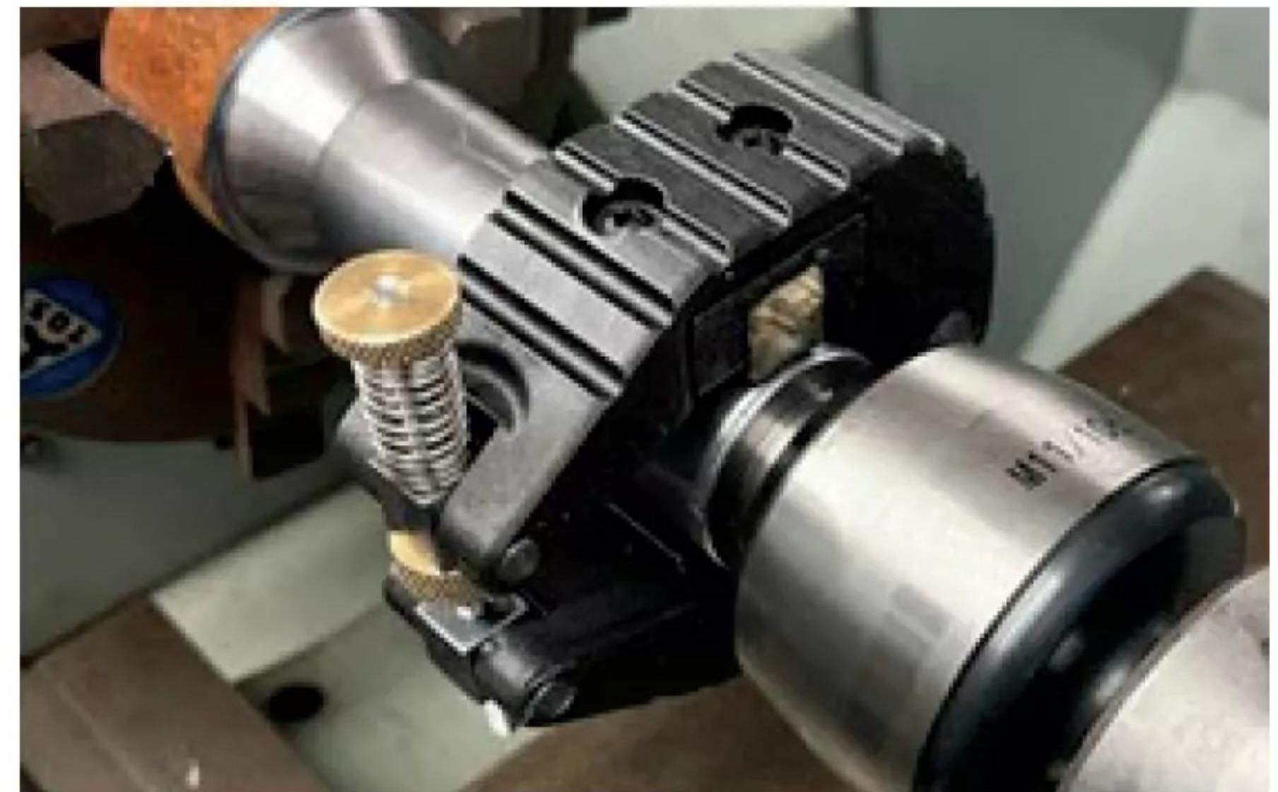
**Photo 8:** A clearer view of how the stone is held against the work.
