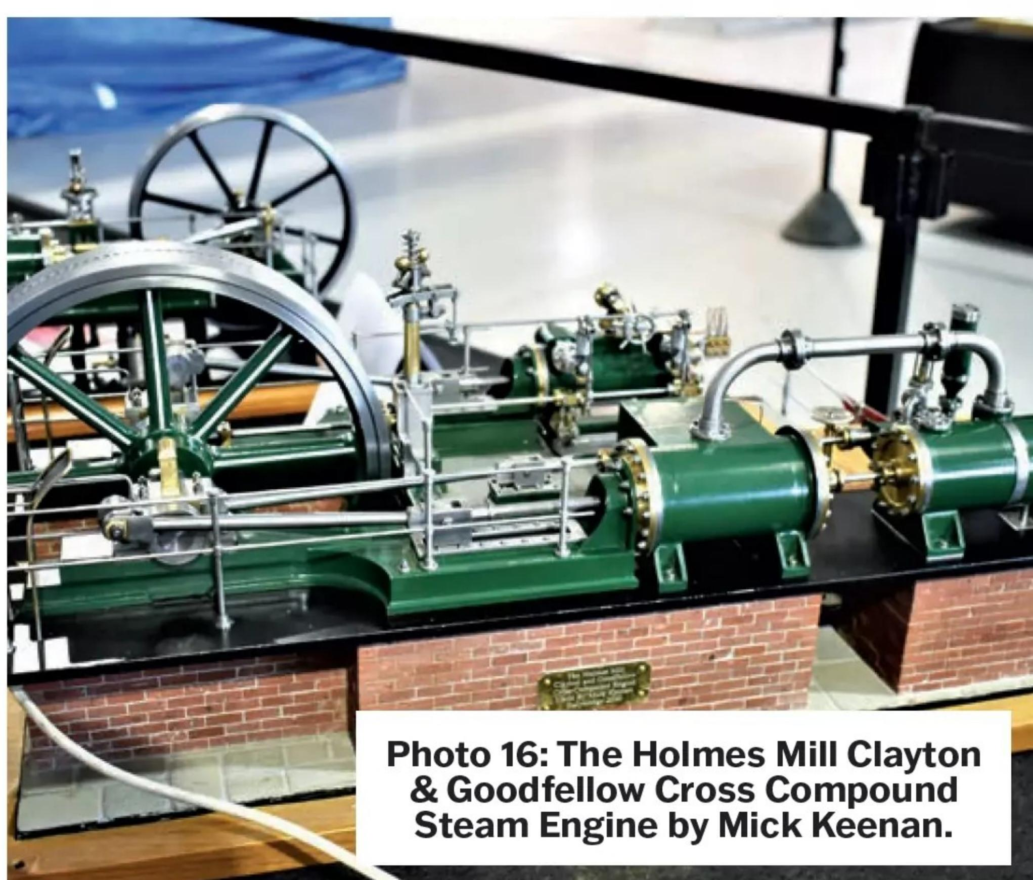
**Photo 16:** The Holmes Mill Clayton & Goodfellow Cross Compound Steam Engine by Mick Keenan.
