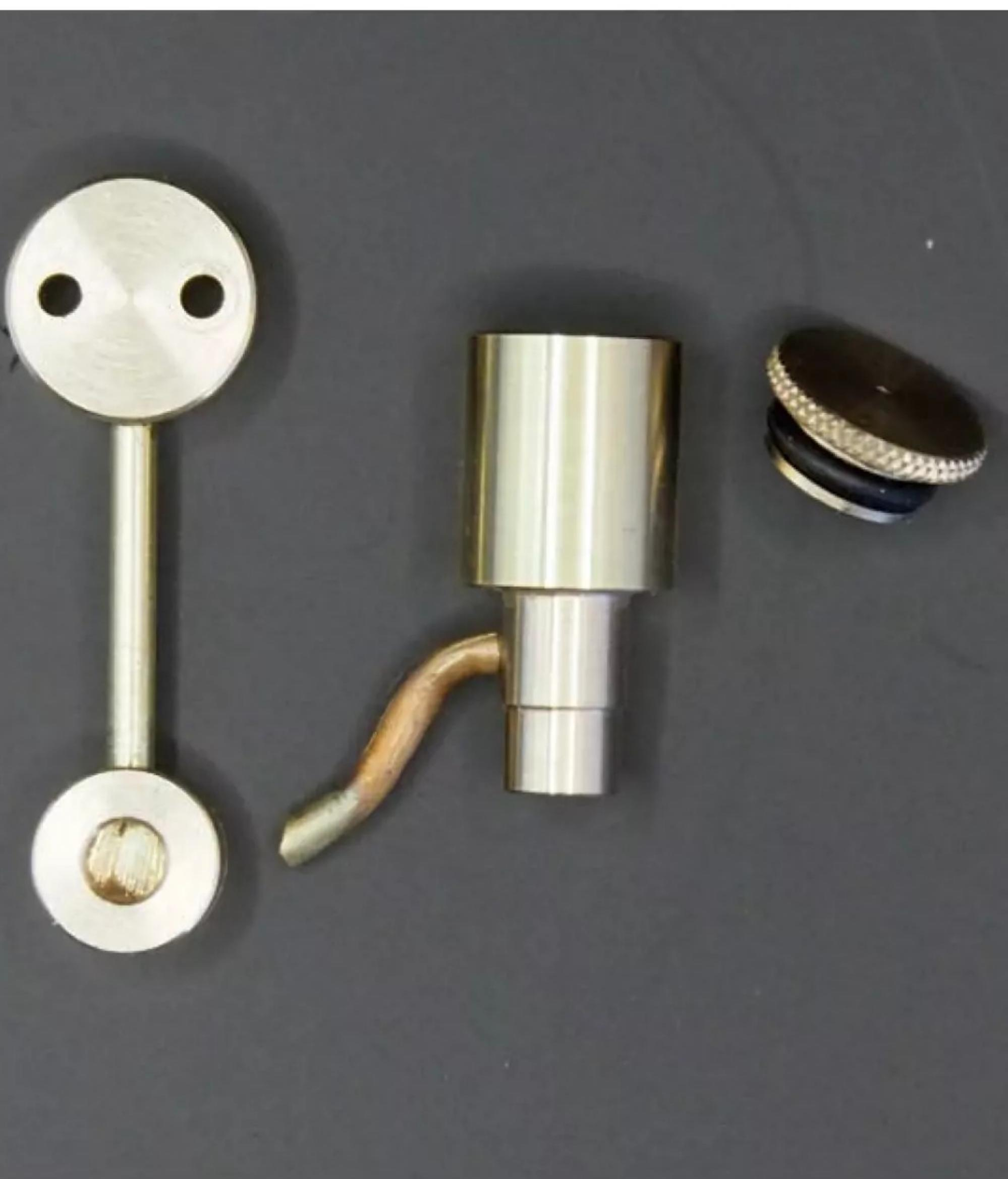
**Photo 376: The parts for the crankpin oil pot and the banjo that carried the oil in.**
