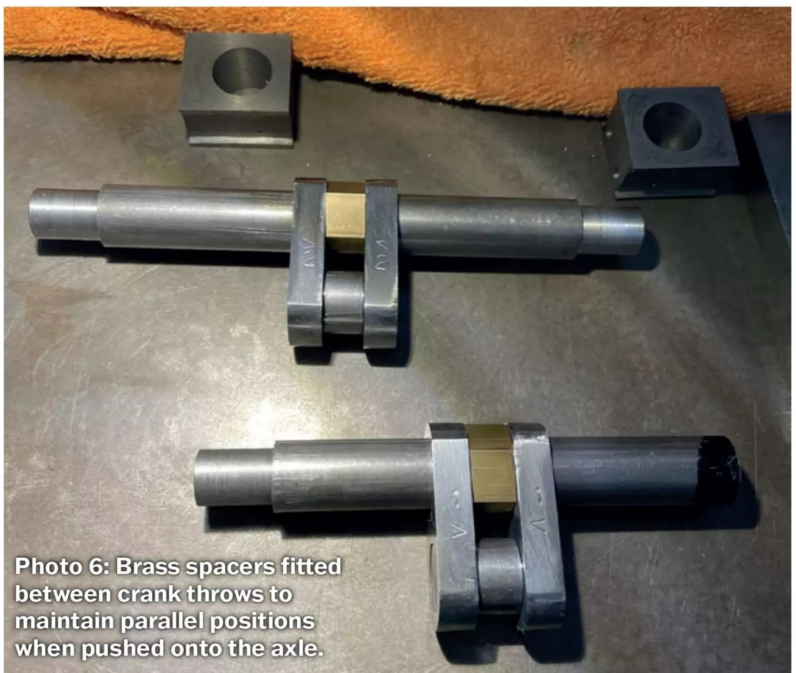
**Photo 6:** Brass spacers fitted between crank throws to maintain parallel positions when pushed onto the axle.
