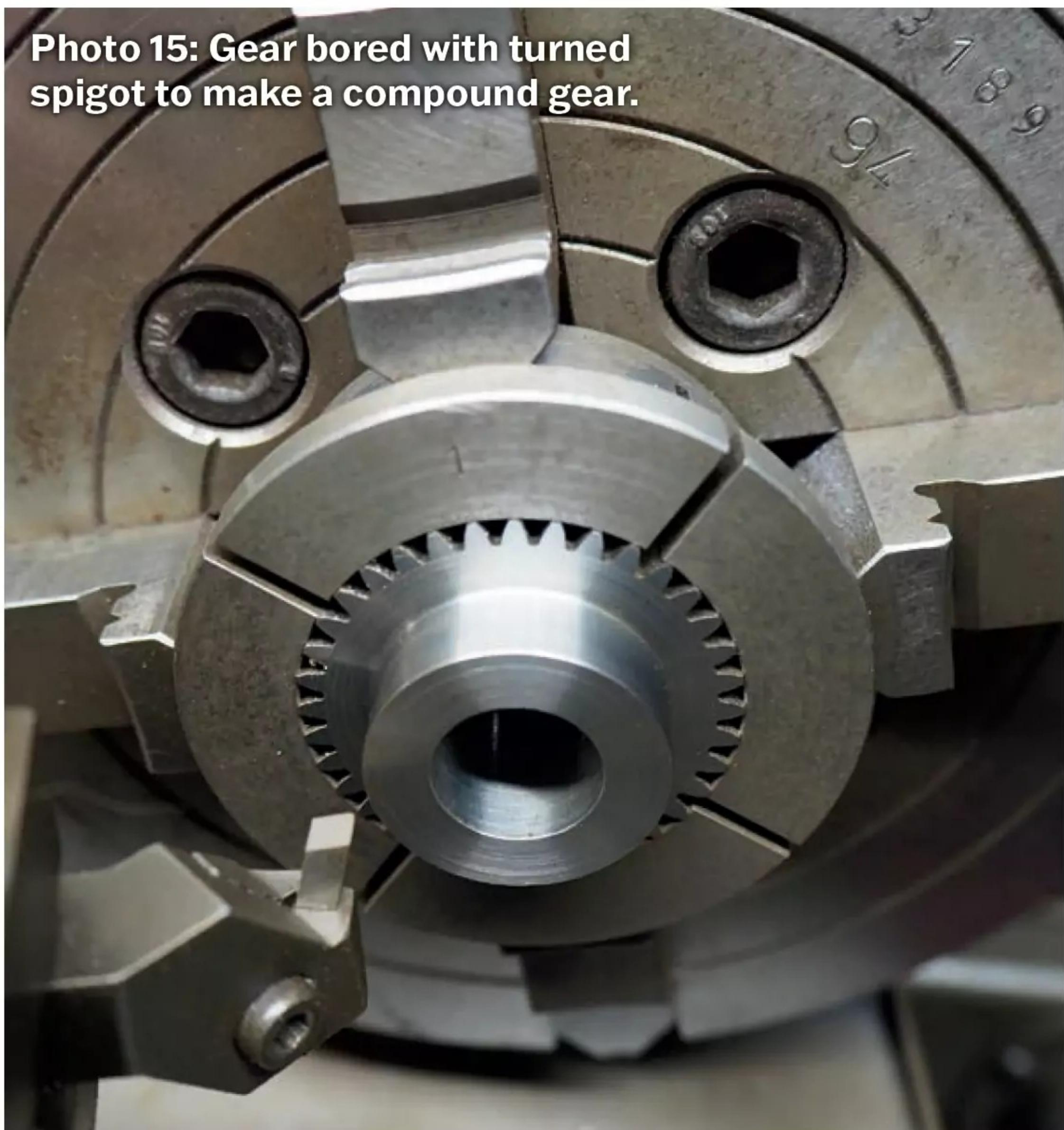
**Photo 15:** Gear bored with turned spigot to make a compound gear.
