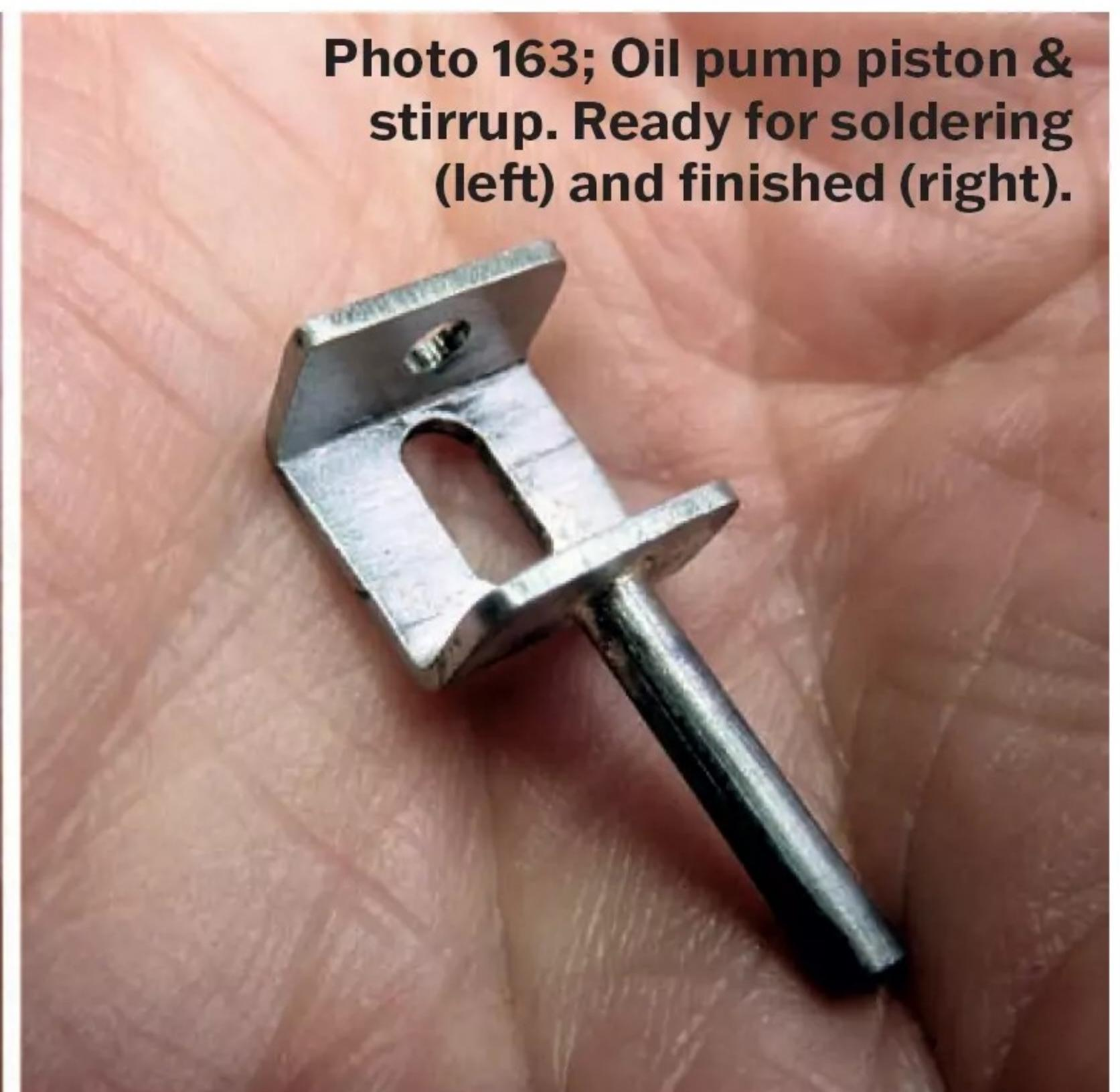
**Photo 163; Oil pump piston & stirrup. Ready for soldering (left) and finished (right).**
