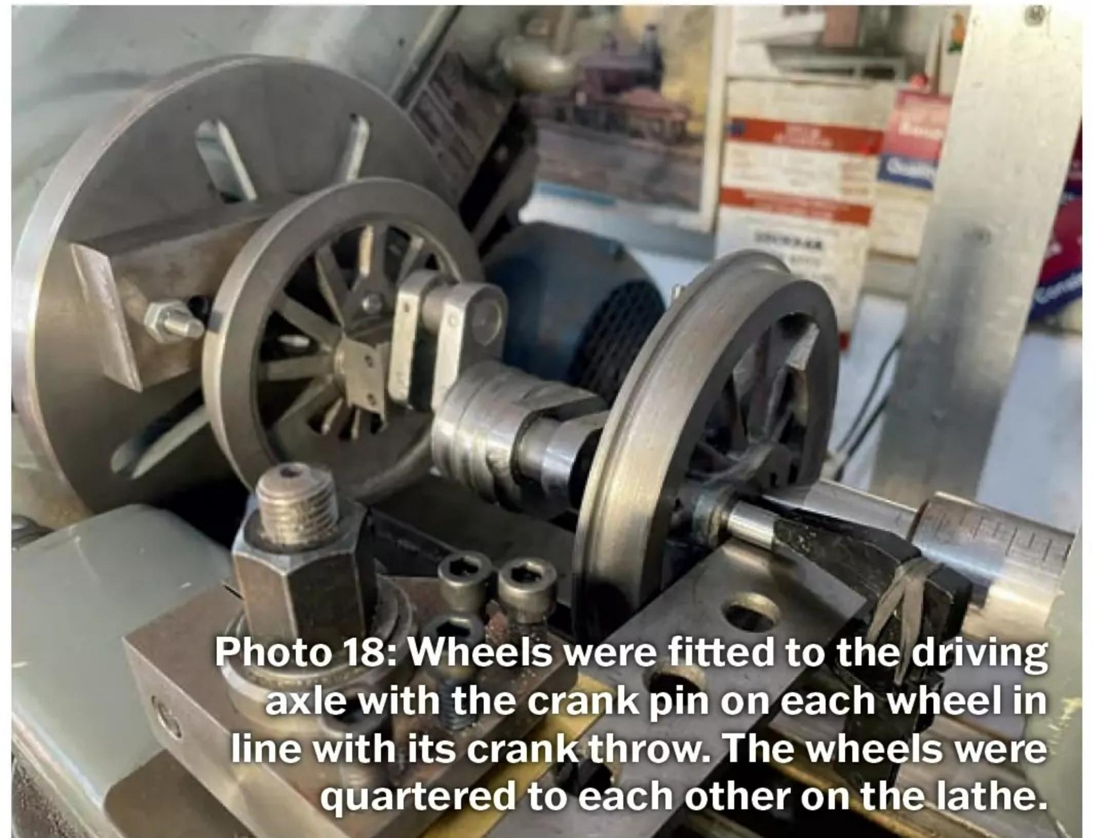
**Photo 18:** Wheels were fitted to the driving axle with the crank pin on each wheel in line with its crank throw. The wheels were quartered to each other on the lathe.
