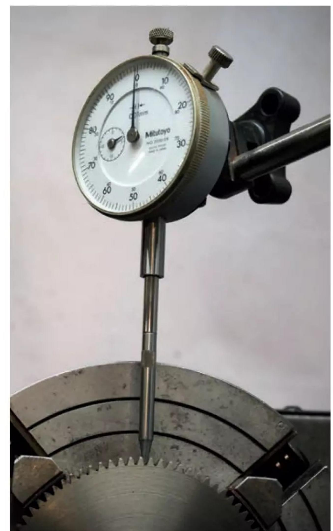
**Photo 14:** Setting up gear using pointed extension fitted to dial indicator.
