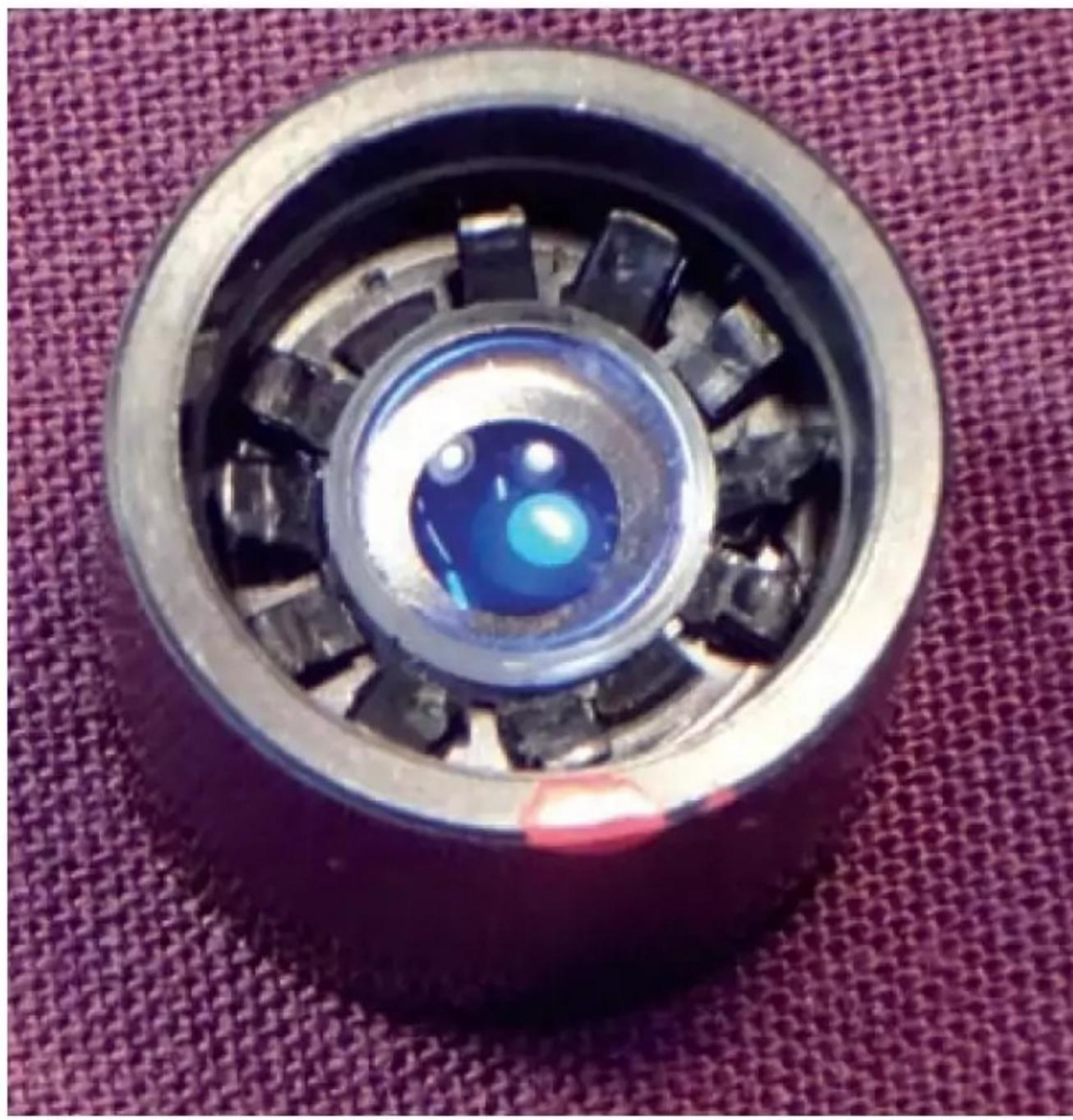
**Photo 20:** Close up of a scanner module showing how the lens is held with plastic fingers that are easily bent back to release the lens. The blue cast demonstrates that it has an anti-reflection coating.
