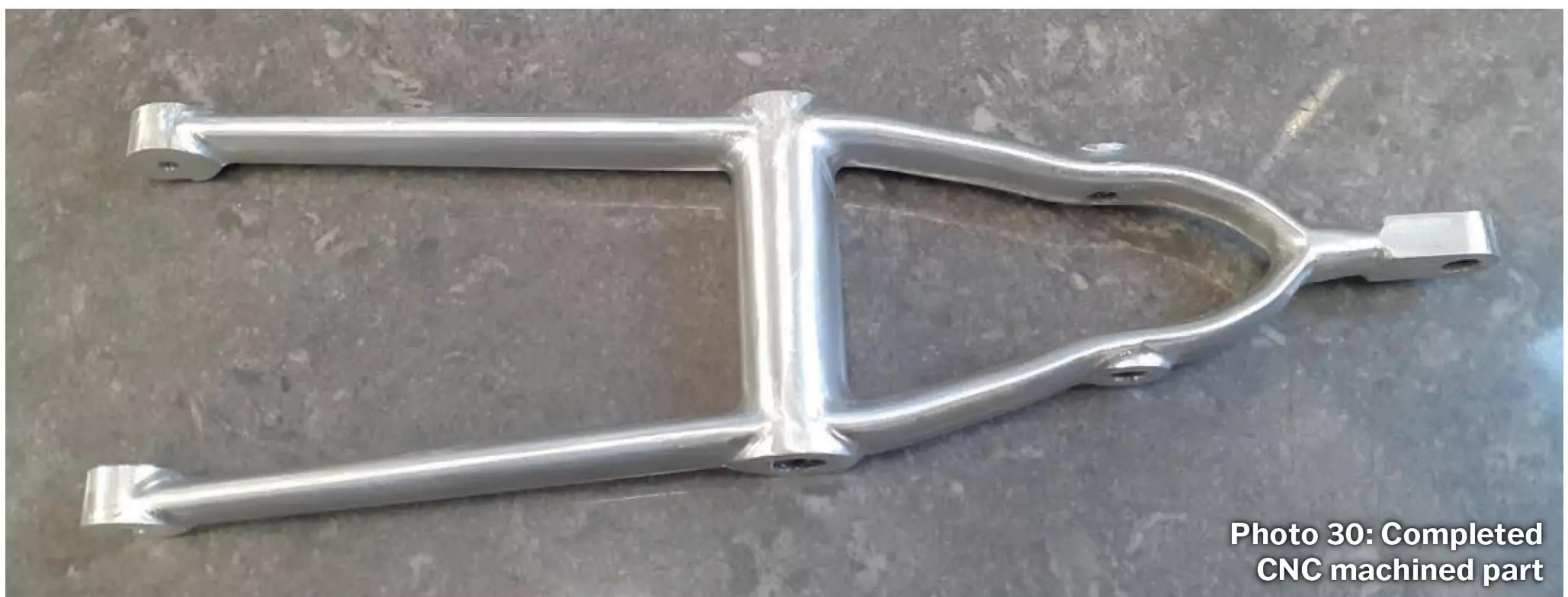
**Photo 30: Completed CNC machined part**
