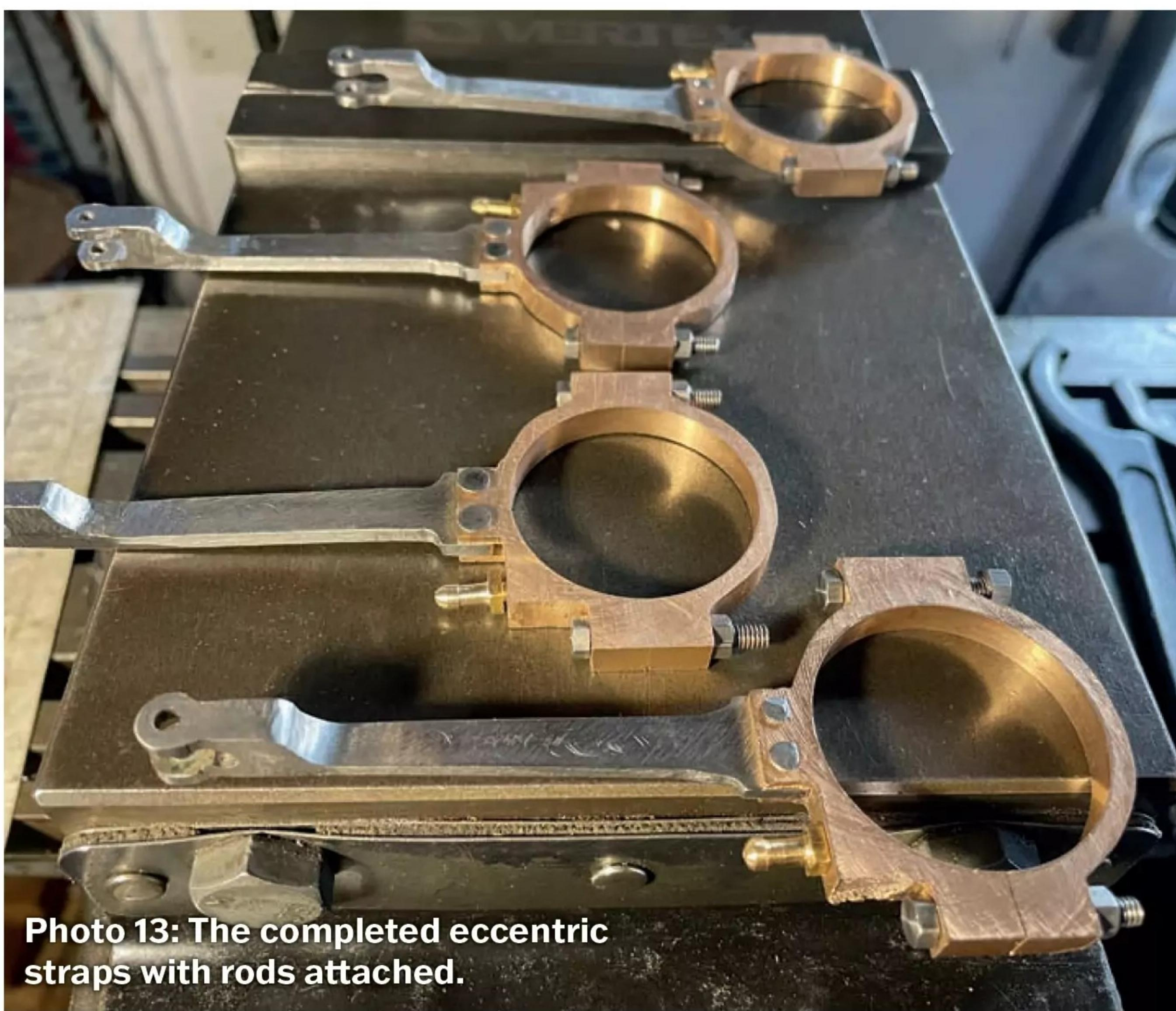
**Photo 13:** The completed eccentric straps with rods attached.
