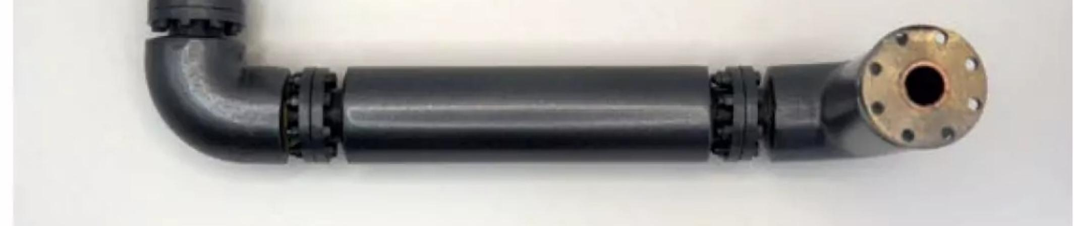
**Photo 381: The exhaust pipe run after painting (and an accidental drop that exposed the insides).**
