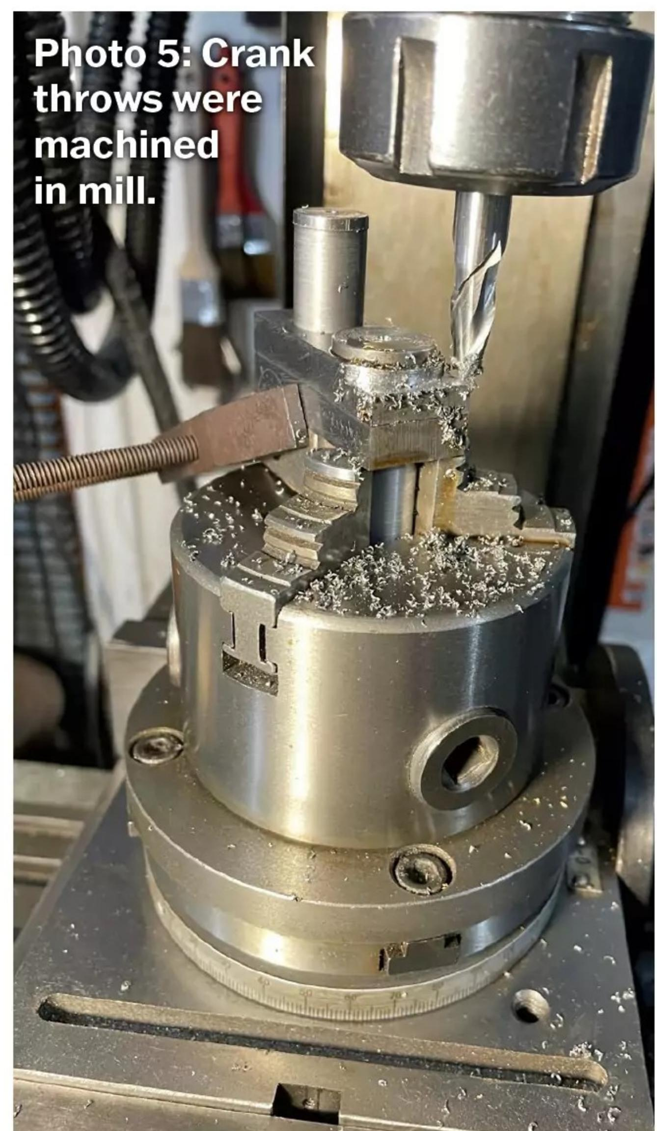
**Photo 5:** Crank throws were machined in mill.
