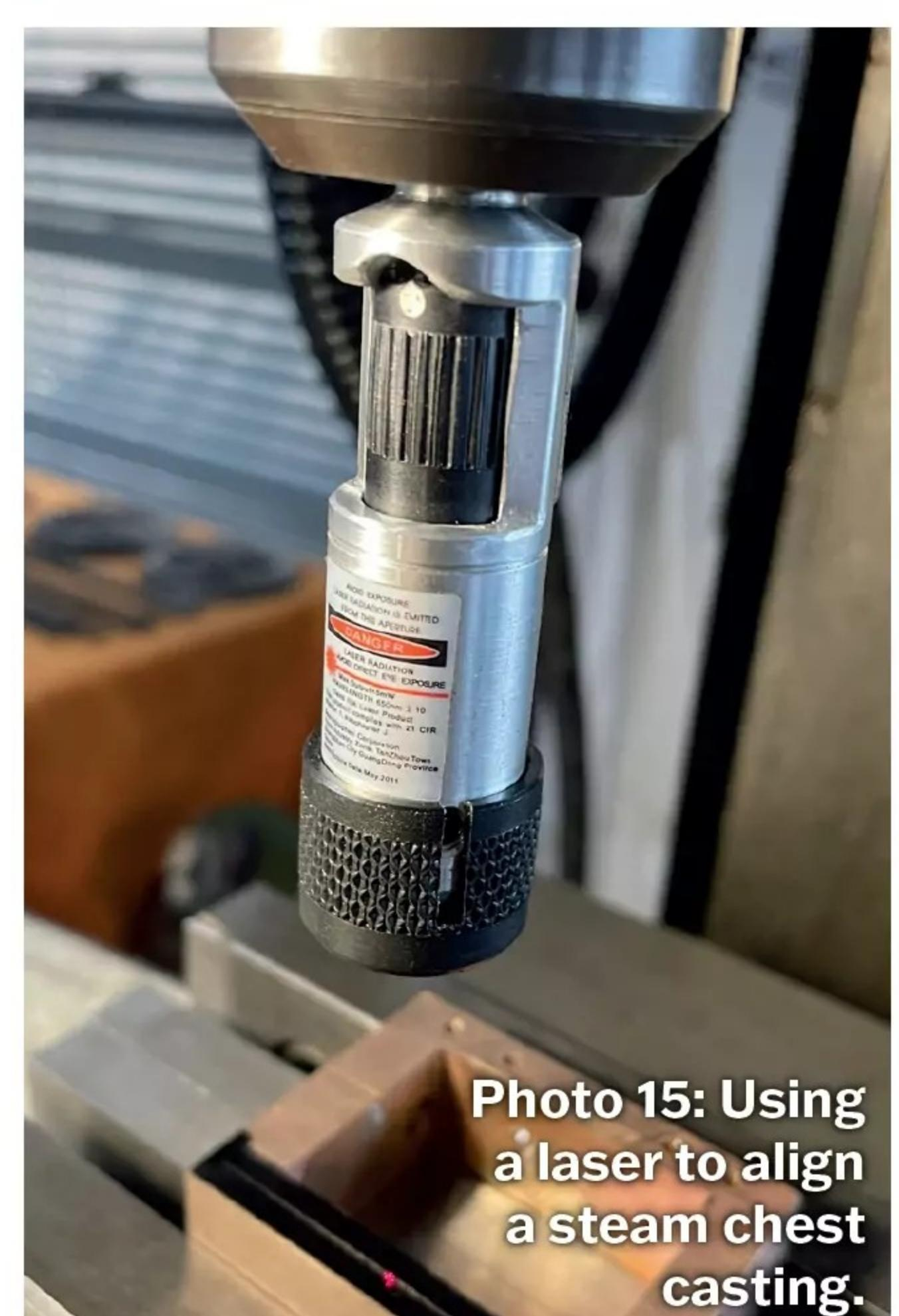
**Photo 15:** Using a laser to align a steam chest casting.
