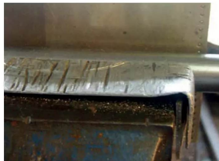
Photo 4: Holding a prepared piece of plate for a tender corner so the bend can be formed after the lower row of simulated rivets has been made.
