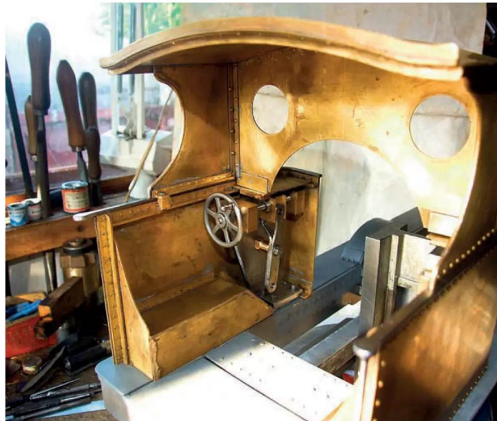
Photo 12: The front cab plate being used for the shape needed for the angle attaching it to the roof. The model needs two similar sections, one for the underside and one representing a rain-strip on top.
