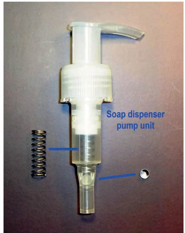
Photo 17: The pump mechanism of a disposable soap dispenser. These typically have a 5mm glass ball and a nice chrome plated spring acting as the one-way valve.
