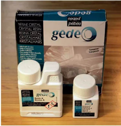
Photo 3: Gedeo Crystal Resin used in my experiments to cast miniature bi-convex lenses.
