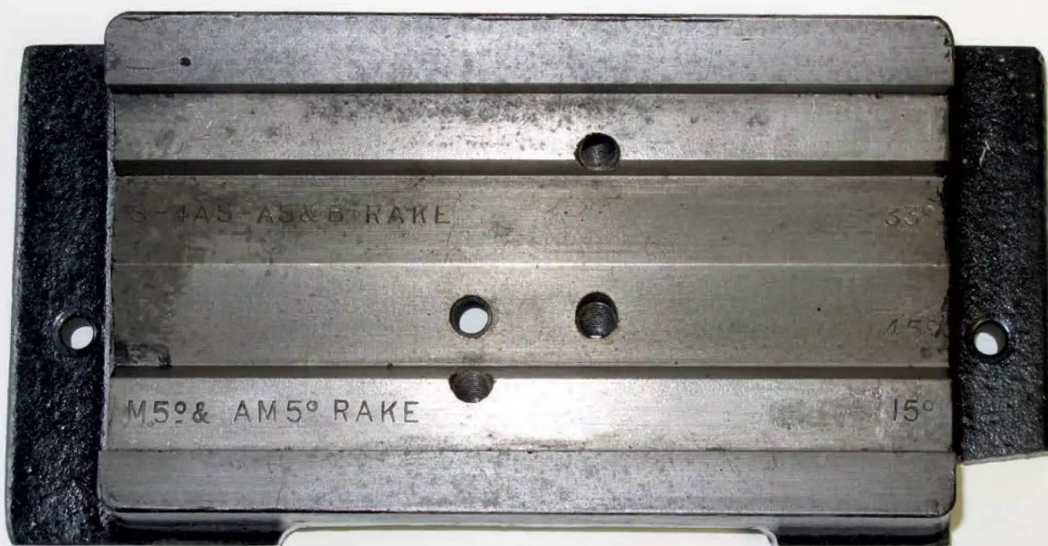
Photo 6: Base of the 3/8" - 1/2" jig with marked flats for angling the upper part of the jig.
