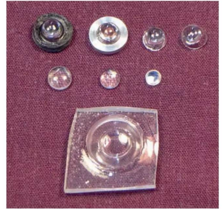
Photo 9: A selection of home-made lenses. Top row: lenses cut from MES bulbs both mounted left, and broken off, right. Middle row: three cast resin lenses. Bottom: An attempt to create a lens by hot-pressing in 3mm thick Perspex.
