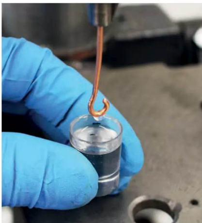
Photo 6: Thoroughly mixing Gedeo resin with a simple hook stirrer on the drill press.
