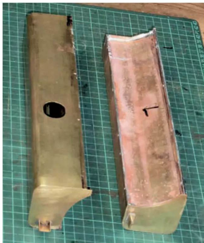
Photo 157: The basic tanks soldered shut.
