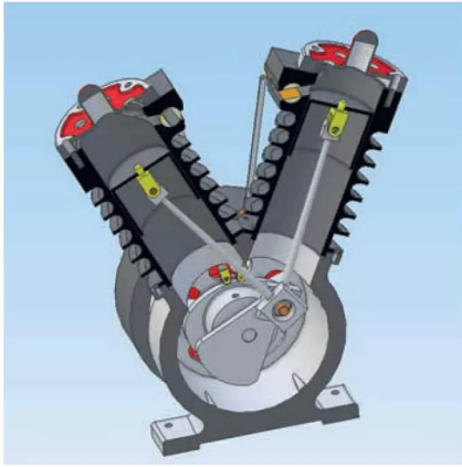
Photo 4: Final design assembly - section view
