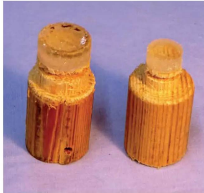
Photo 14: After the clear resin had cured the edges of each lens were exposed by turning back the enclosing wood dowels.
