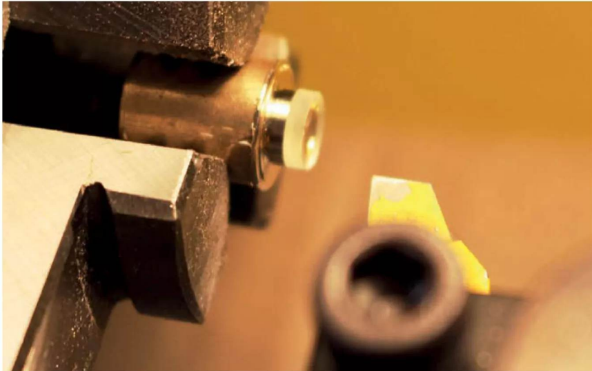
Photo 8: Once the Gedeo resin had cured each brass cup was turned back to expose the rim of the cast lens which could then easily be popped out of the mould.
