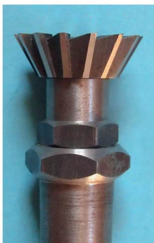
Jacques Maurel explains how to make an adaptor to hold threaded end mills.
