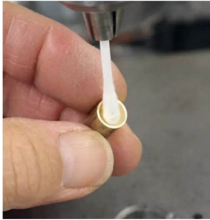
Photo 4: Polishing one of the brass casting cups with Brasso and a Cotton Bud.
