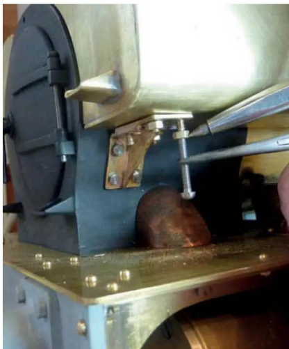
Photo 158: How to coax small nuts into place with a scribe.
