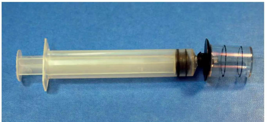
Photo 7: Crude vacuum pump used to remove bubbles from the Gedeo resin. The syringe is sealed to the cup containing the resin and the plunger retracted and held for several minutes. All the parts were found in my scrap box. Black rings on the cup were guides for combining hardener and resin volumes in the ratio 1:2.
