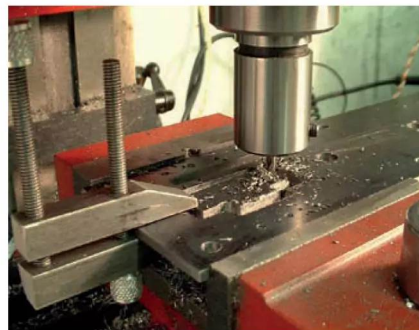
Photo 8: Milling out the 'crankshaft pit'.
