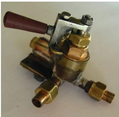
Photo 199: Finished actuating valve.
