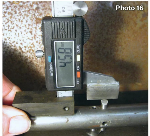
Photo 14: Initially setting the cutter to rather less than 5mm.
