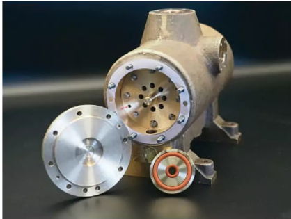
Photo 350: Rear view of the air pump/condenser with the rear delivery plate exposed along with the valve and the rear cylinder cover.
