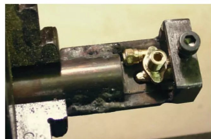
Photo 196: Casting in jig for boring.
