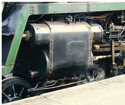
Photo 205: Bolt on relief valve on front cylinder cover.
