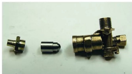
Photo 195: One of Geoff's drain cocks disassembled.
