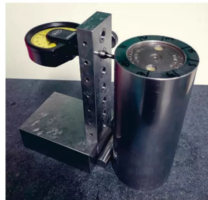
Photo 8: Surveying the cylindrical master square for errors relative to a true square.
