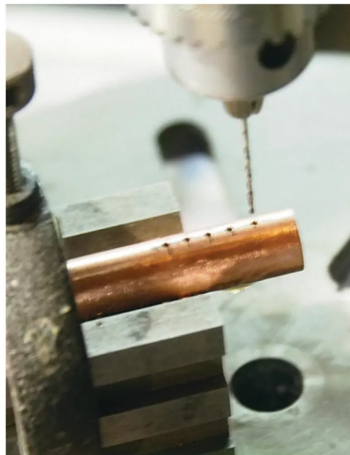
Photo 356: The spray bar is just a length of copper pipe with a brass plug soldered into the end.
