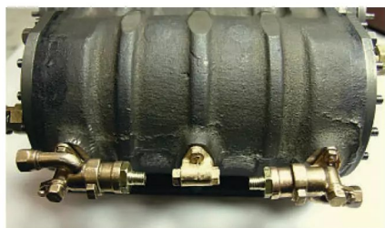
Photo 194: Close up of drain cocks.
