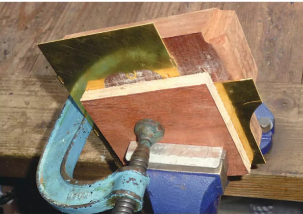
Photo 145: Cab side clamped for forming the rear corner.
