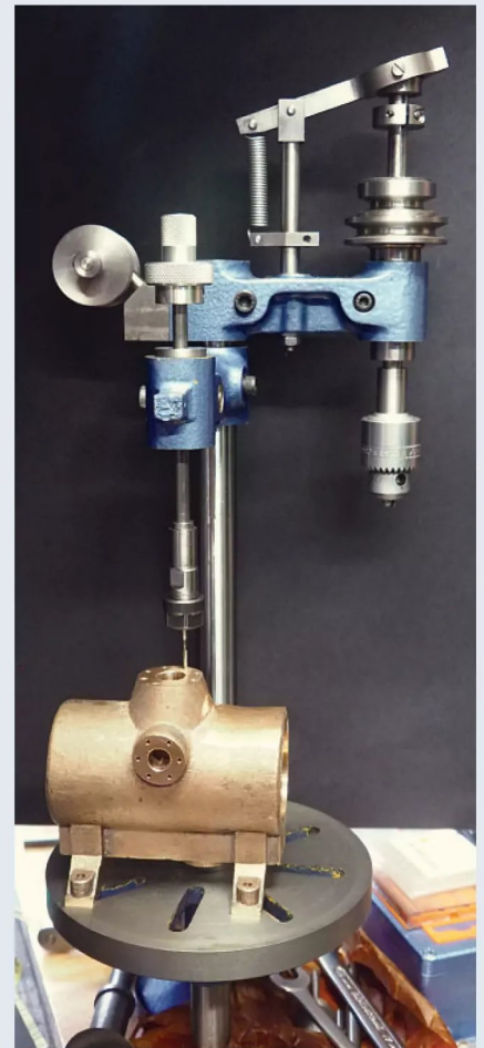
Photo 342: Just to emphasise that some sort of guide is essential for tapping the stud holes (46 of them I think).
