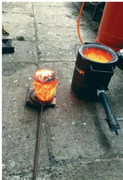
Photo 3: All aglow. Ready to start pouring.
