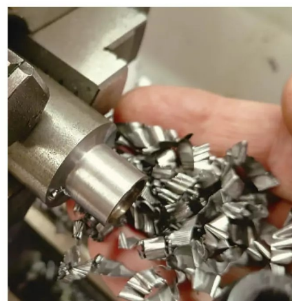
Photo 9: The result of a heavy 5mm deep cut in steel.
