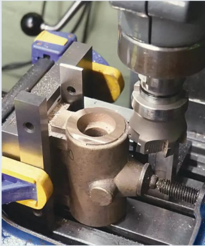
Photo 336: A nest of angle plates and parallels located the casting for machining the ends.
