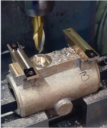
Photo 335: The holes were drilled at the same setting; the last one was the condensate exhaust.
