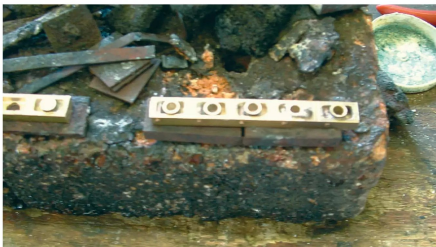
Photo 185: Making valve guide die blocks.
