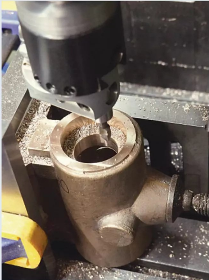
Photo 337: Boring the first end.
