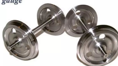
5" gauge 3 Hole Disc Wheels with profiled face
