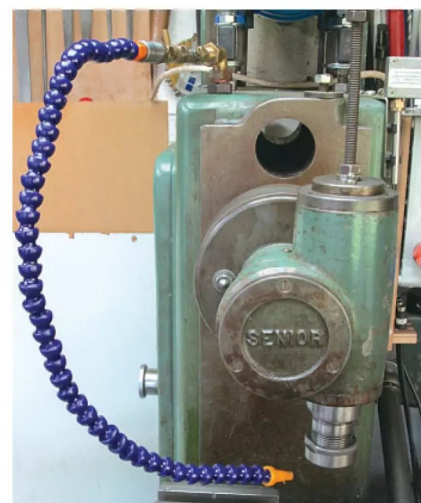
Photo 22: New discharge pipe to cutter.
