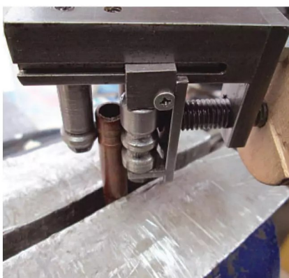
Photo 21: Shop made tool for rolling groove in pipe.
