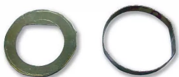
Photo 168: Embryo cylinder end cover cleading.
