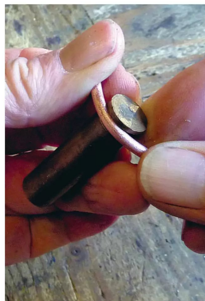
Photo 122: My home-made pipe bending tool.
