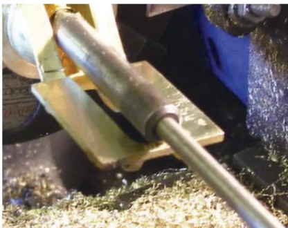
Photo 174: My extended pin drill in action.
