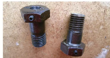
Photo 18: M16 pipe locating bolts.
