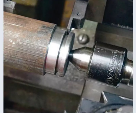
Photo 323: After first facing the end and turning to diameter, I put in the groove for the O-ring packing.
