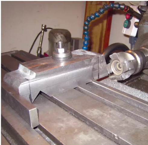
Photo 8: Milling the edges of the base of the steady.
