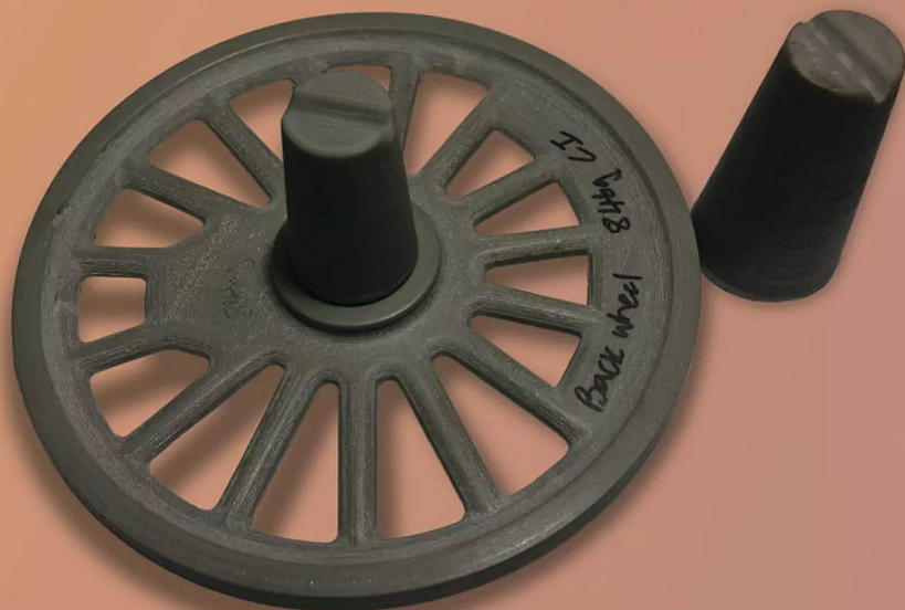
Photo 2: Spoked wheel pattern and risers.
