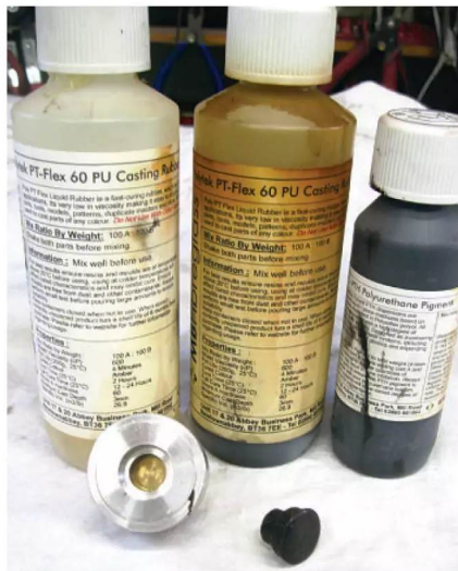
Photo 14: Mould and product made in cold moulded polyurethane rubber.
