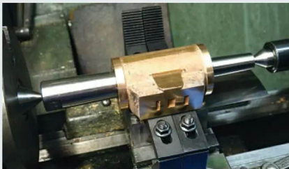
Photo 298: Not everything went exactly to plan and a bit of very thin shim was needed to get the height right before clamping down. Bringing the casting across from the mill, still on the expanding mandrel, was a part of the plan.
