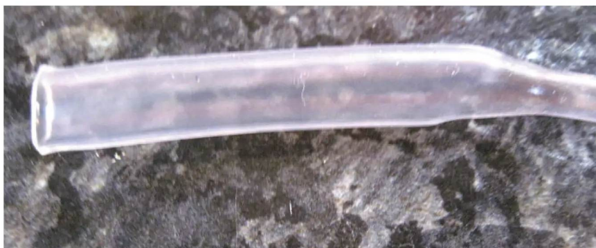
Photo 16: Soaking PVC tubing in methyl ethyl ketone.
