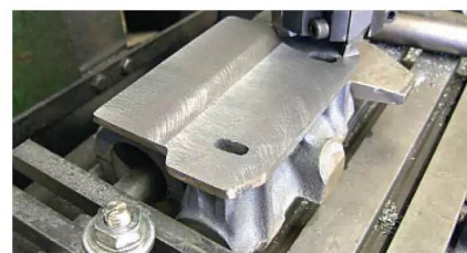
Photo 156: A slab milling cutter faces the back plate.
