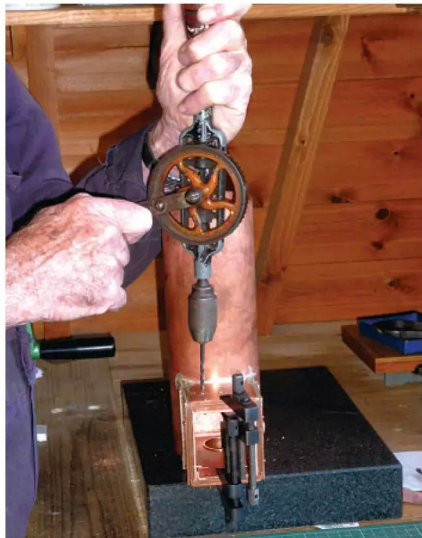
Photo 108: Spotting through by hand due to the confines of the throatplate.
