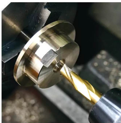
Photo 311: ...then they were moved to a collet to finish the internal details. This is the rear cover having the clearance for the piston nut machined.
