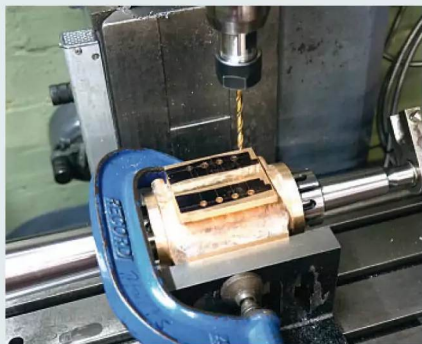
Photo 302: The expanding mandrel was checked for burrs then used to re-mount the cylinder for drilling the securing holes. The machined valve face was used for angular location.
