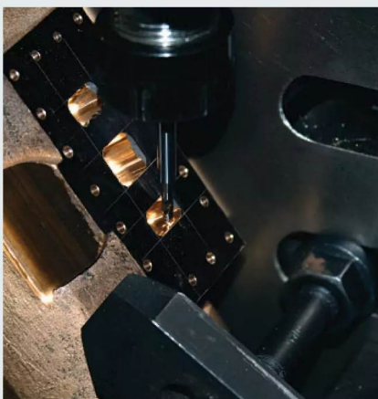
Photo 306: Starting the steam passages with a slot drill...
