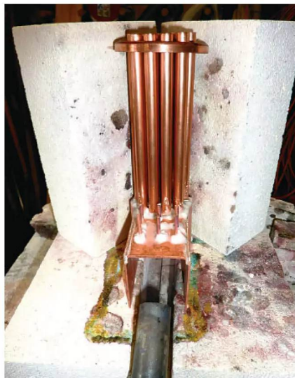
Photo 110: Heat is applied inside the firebox.
