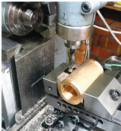
Photo 308: Drilling through for the exhaust.
