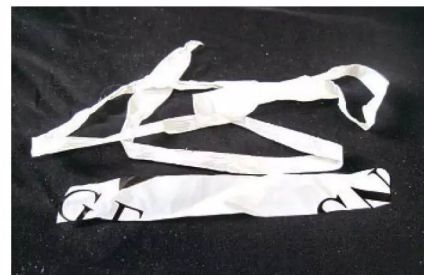
Photo 12: Plastic deformation of polymer film. The un-stretched film and the drawn one.
