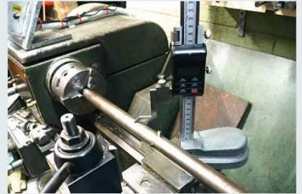
Photo 296: Measuring the height of the lathe centre above the after-market boring table.
