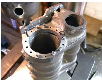
Photo 161: Tapping for the cylinder covers.
