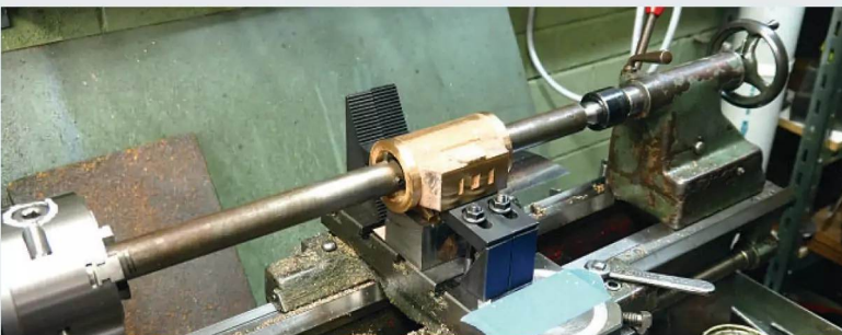
Photo 300: The clamps were set to bear on the upper surface of the base to avoid any chance of distorting the cylinder. Standard mill clamps just made it for size, but some one-offs wouldn't be difficult to make.
