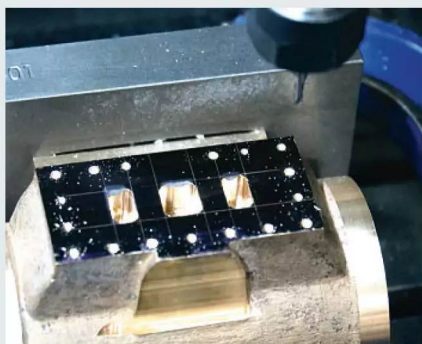
Photo 305: The JB Weld used to correct the port edges can be seen here. The ports have been machined and the stud holes are being spotted out.
