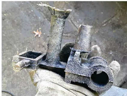
Photo 5: Gunmetal cylinder and valve chest as removed from the sand.
