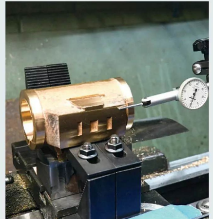
Photo 299: The sanity check with the indicator was encouraging.
