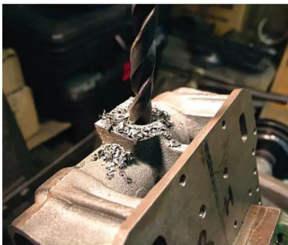
Photo 160: Machining the steam inlet.
