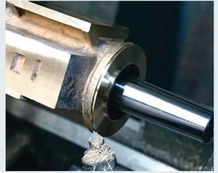
Photo 293: One end of the cylinder could now be brought to length and diameter.
