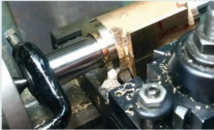
Photo 294: And then the other. Unlike most of the other castings there was plenty of machining allowance on this one.
