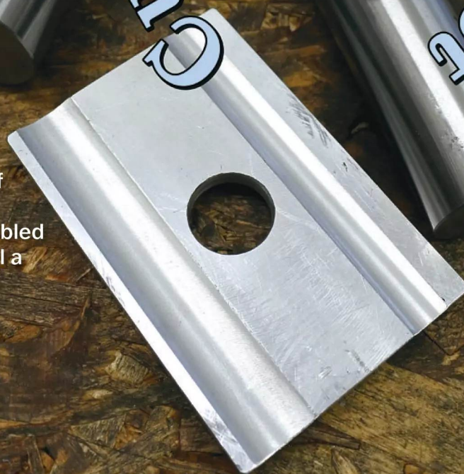
Photo 1: Sample plate with two circular slots milled into it.
