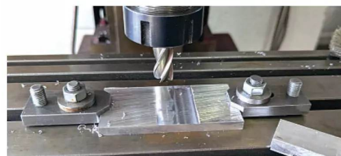
Photo 6: The fixture is clamped to the mill table and skimmed flat where the workpiece will be attached.
