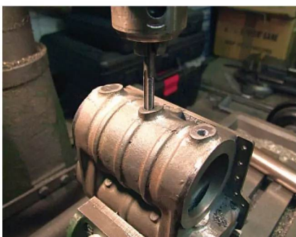
Photo 162: Tapping the drain cock holes.
