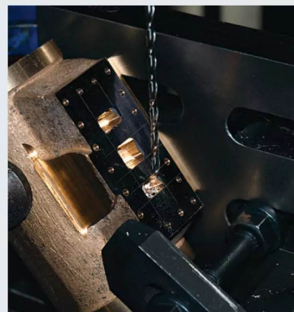
Photo 307: ...and finishing with a long series drill.
