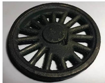
Photo 3: Casting inclusion when no riser is used.
