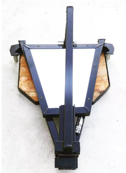
Photo 7: The delta unit lies mostly between the two platforms when folded.
