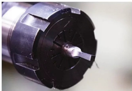
Photo 261: The valve levers need a close fitting square hole to go over the end of the spindles. The first job is to make a broach to go in the Hemingway rotary broach.
