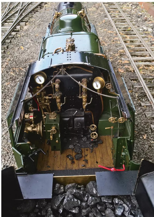
Photo 138: Additional universal joints bring operation closer to the driver.
