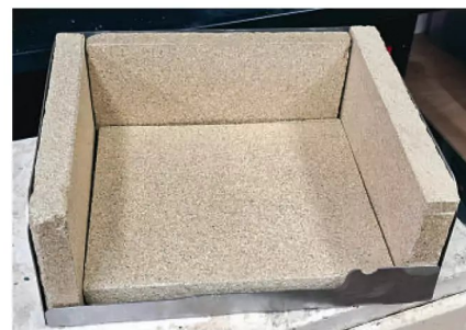
Photo 5: Frame with vermiculite blocks in place.
