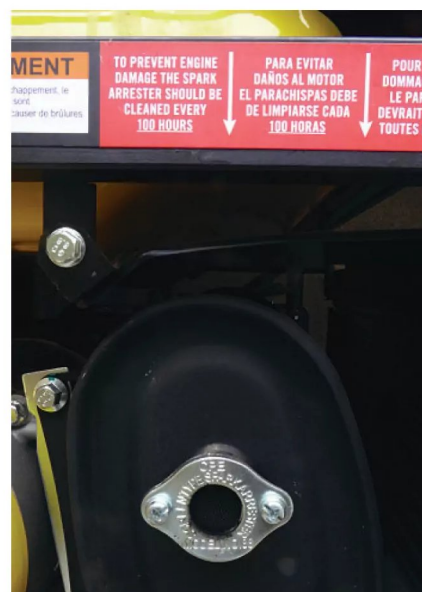
Photo 1: Mesh spark arrester with cleaning warning.
