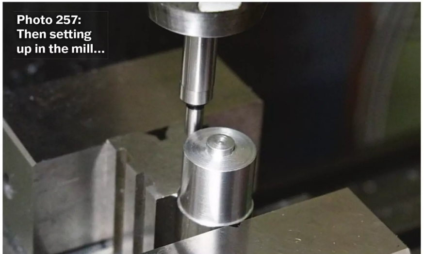
Photo 258: ...in order to drill the mounting hole through both parts.
