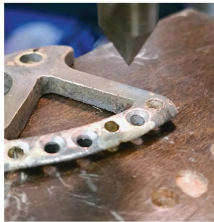
Photo 10: Countersinking a re-drilled hole.
