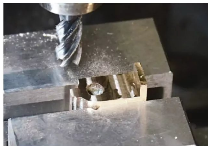
Photo 245: Where the bronze had poured well the dashpot body machined very nicely. The metal had flowed well around the cylinder core.
