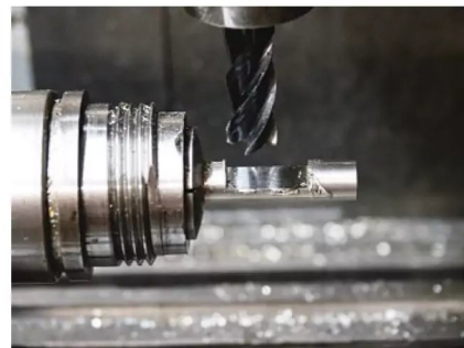
Photo 251: ...and then the flat is milled at the same setting.
