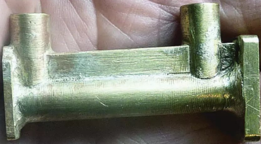
Photo 92: Water pump soldered assembly
