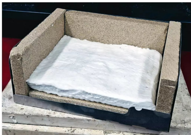
Photo 6: Kaolin wool blanket in base of hearth.
