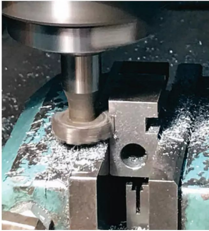
Photo 4: Machining guide block with a T-cutter.
