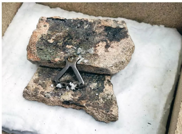
Photo 7: Fluxed string retainer ready for heating.
