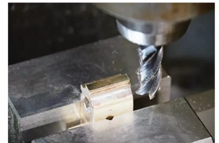
Photo 246: The profile of the front of the dashpot is complex and would be difficult to fabricate.
