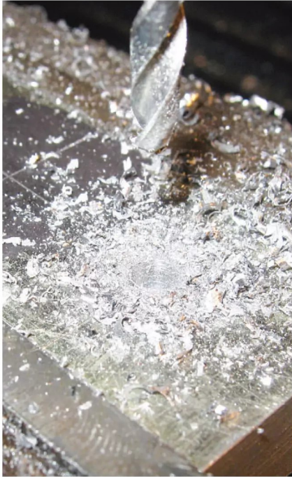
Photo 10: Drilling locating holes.
