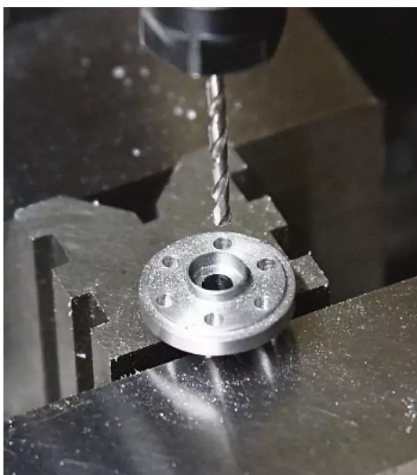
Photo 259: With the body still parallel it's back to the mill to drill the mounting holes.
