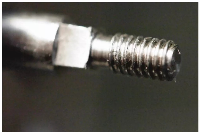
Photo 255: The outer part of the spindle is turned down and threaded.
