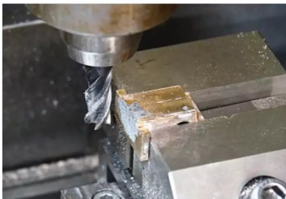
Photo 244: Machining the dashpot body to size. There was a bit of JB Weld used as filler but none of it in a vital place.
