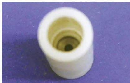
Photo 3: The drill jig used to position the hole for pinning the leg
