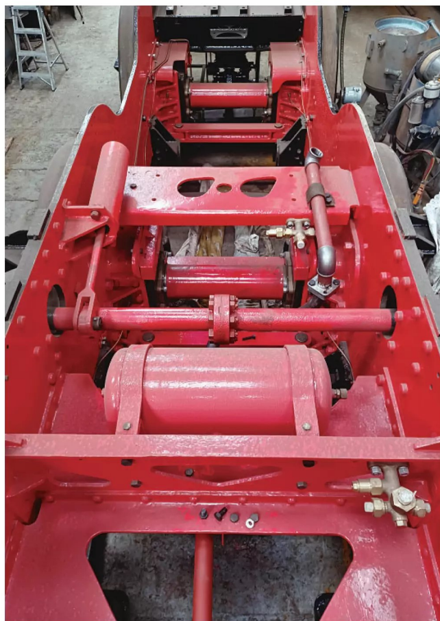
Photo 140: The vacuum reservoir in situ .
