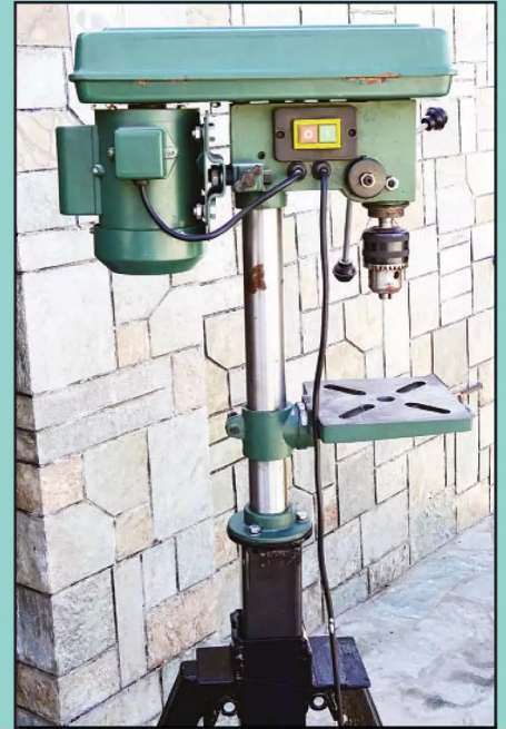
Photo 2: Pillar drill mounted on the stand.
