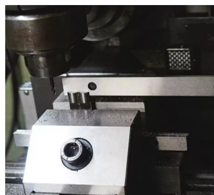
Photo 253: A good result with a 1/8" parallel sitting firmly in the slot.
