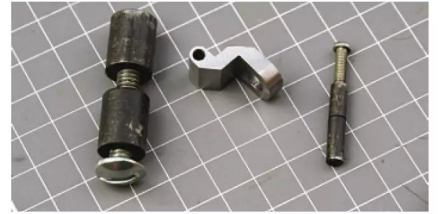
Photo 236: The completed bracket with the filing buttons used to round over the ends.
