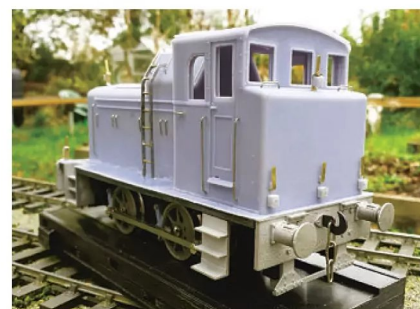
Photo 5: 3-D printing in metal, a Class 01 shunter. (Picture courtesy of Norman Millier.)
