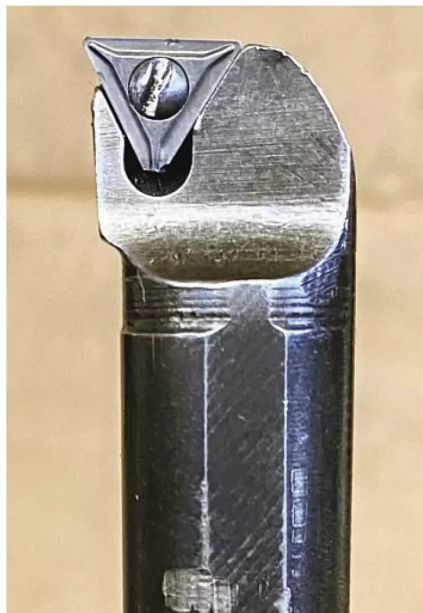
Photo 47: Tip of the inserted carbide tool.
