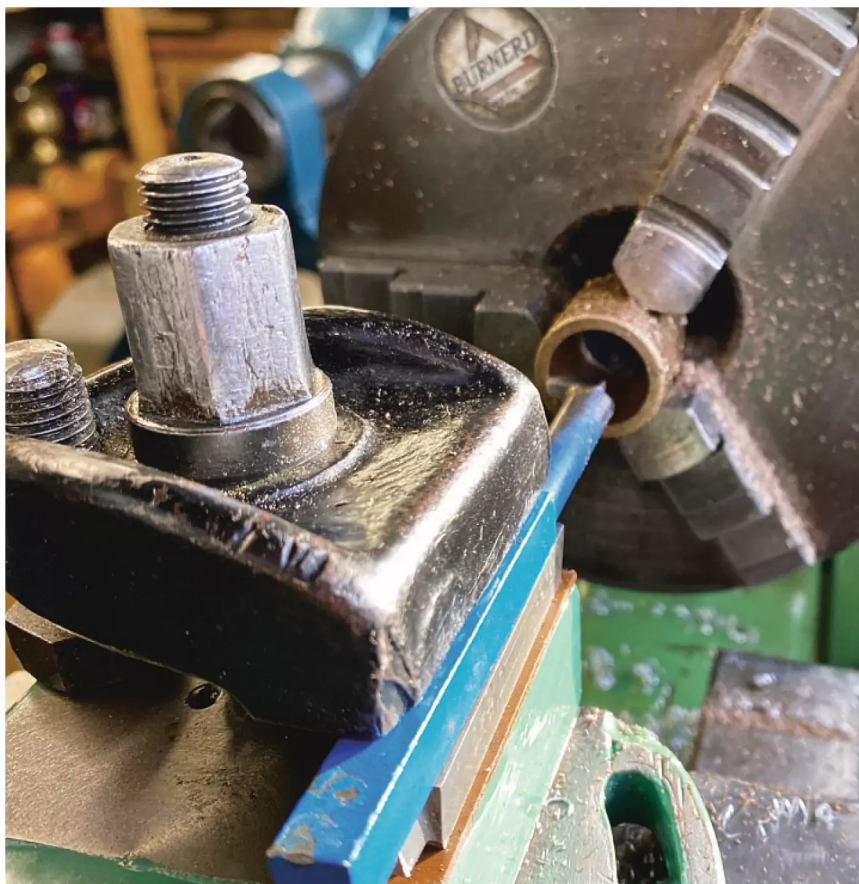
Photo 45: Typical boring setup.
