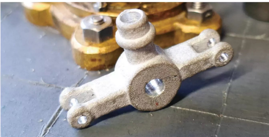
Photo 4: The crosshead with all holes drilled.
