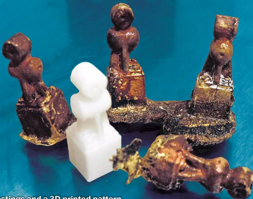
Photo 1: Lost-PLA brass castings and a 3D printed pattern.
