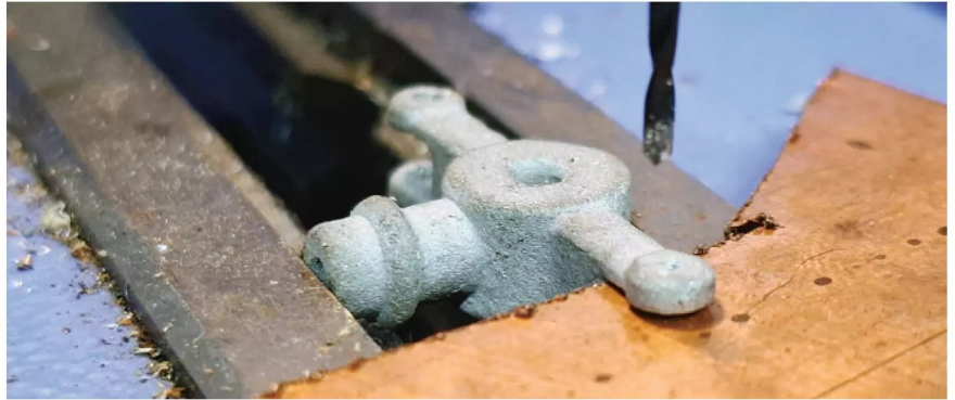
Photo 3: The 3D printed aluminium crosshead, supported for drilling.
