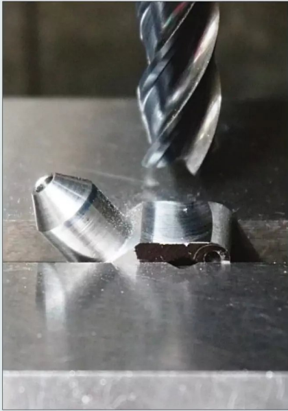
Photo 221: Machining the bevels on the head. The ends have been rounded over using filing buttons.
