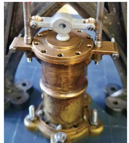
Photo 5: The crosshead with rollers fitted, offered up to the model.
