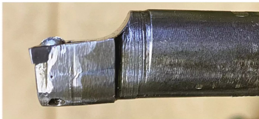
Photo 50: The tip is angled down to increase front clearance.
