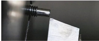
Photo 239: Short lengths of round bar were milled to hexagonal in the dividing head then the glut pins formed on the ends in a 3-jaw Griptru chuck.
