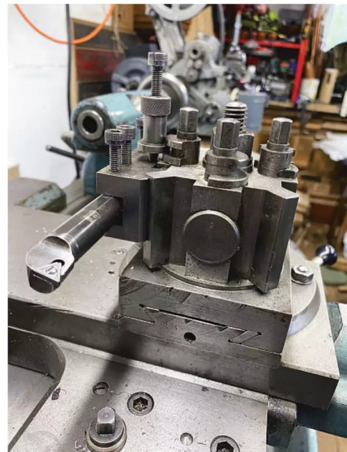
Photo 46: Demonstrating overhang with an inserted carbide tool.
