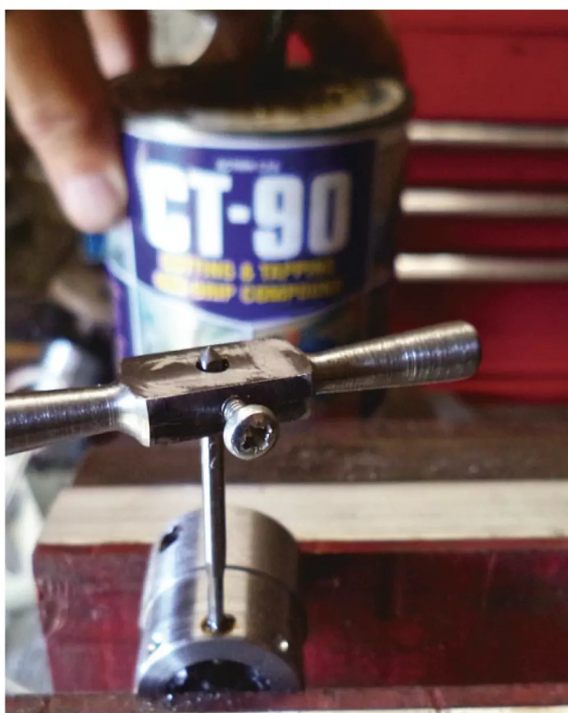
Photo 13: Taping die holder with small wrench. Note use of cutting CT90 cutting fluid and the tap not gripped on the square.
