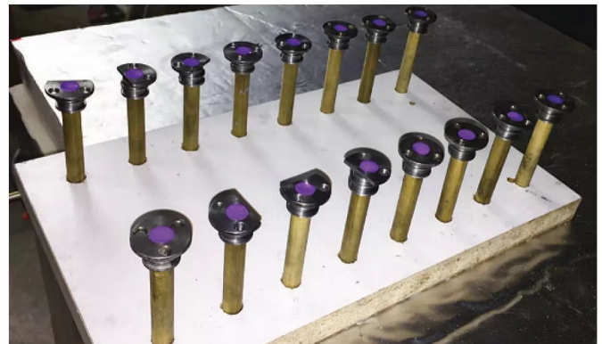
Photo 10: Degreased inserts ready for two coats of unwaxed shellac, three inserts per strake have a partially trimmed edge to maintain clearance on tapered strake side (my mistake).
