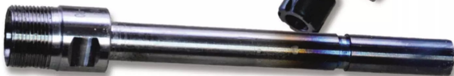
Photo 11: ER 11 chuck heat treated prior to thread cutting.
