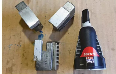
Photo 15: Aluminium soft jaws bonded to the chuck jaws, ensuring they are supported by the shoulders on the jaws.
