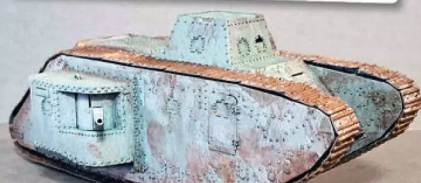
Photo 17: 3D resin printed A7V tank, designed in Alibre Atom 3D.
